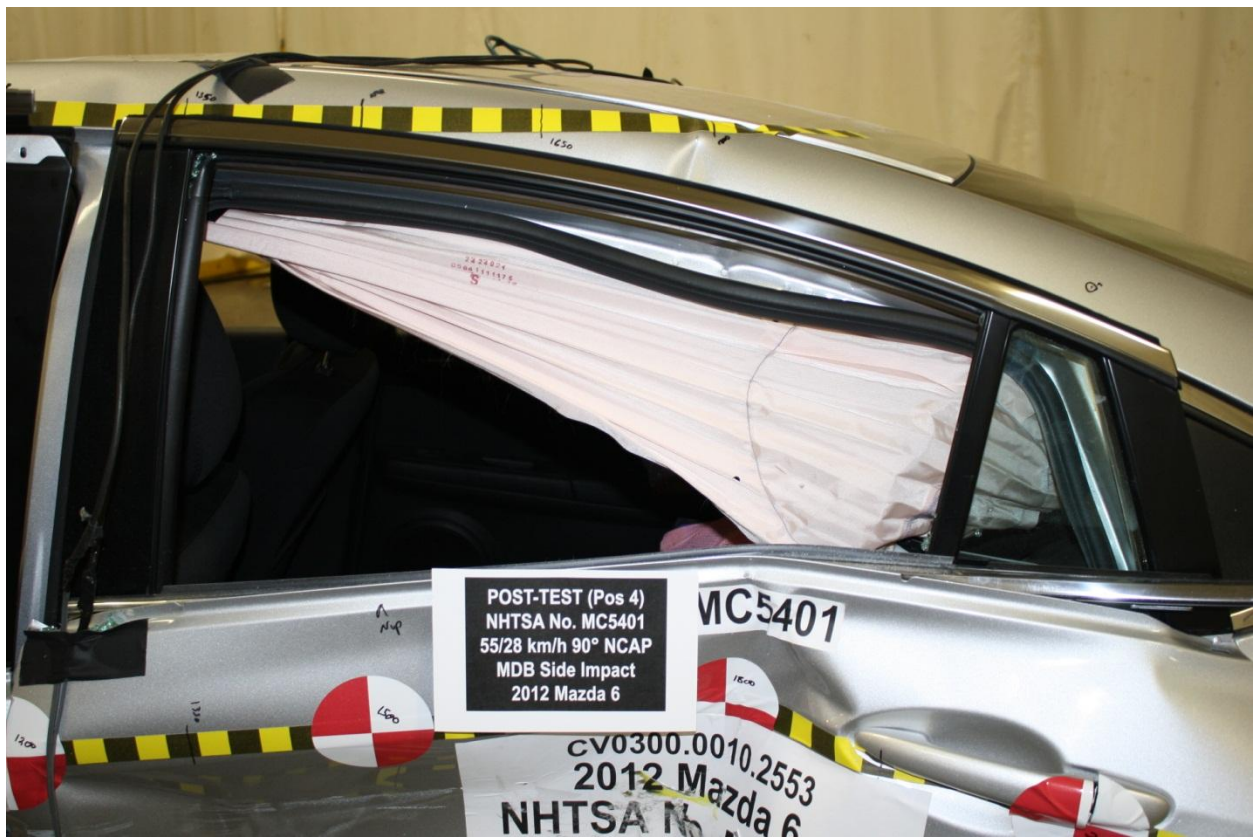
Figure A-56: Post-Test Left Side View of Passenger Dummy Shoulder and Door Top View
