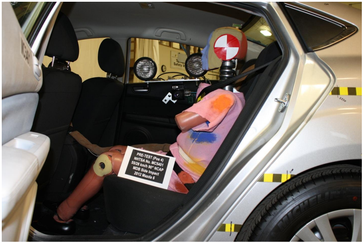
Figure A-54: Pre-Test Left Side View of Passenger Dummy Showing Belt and Chalking
