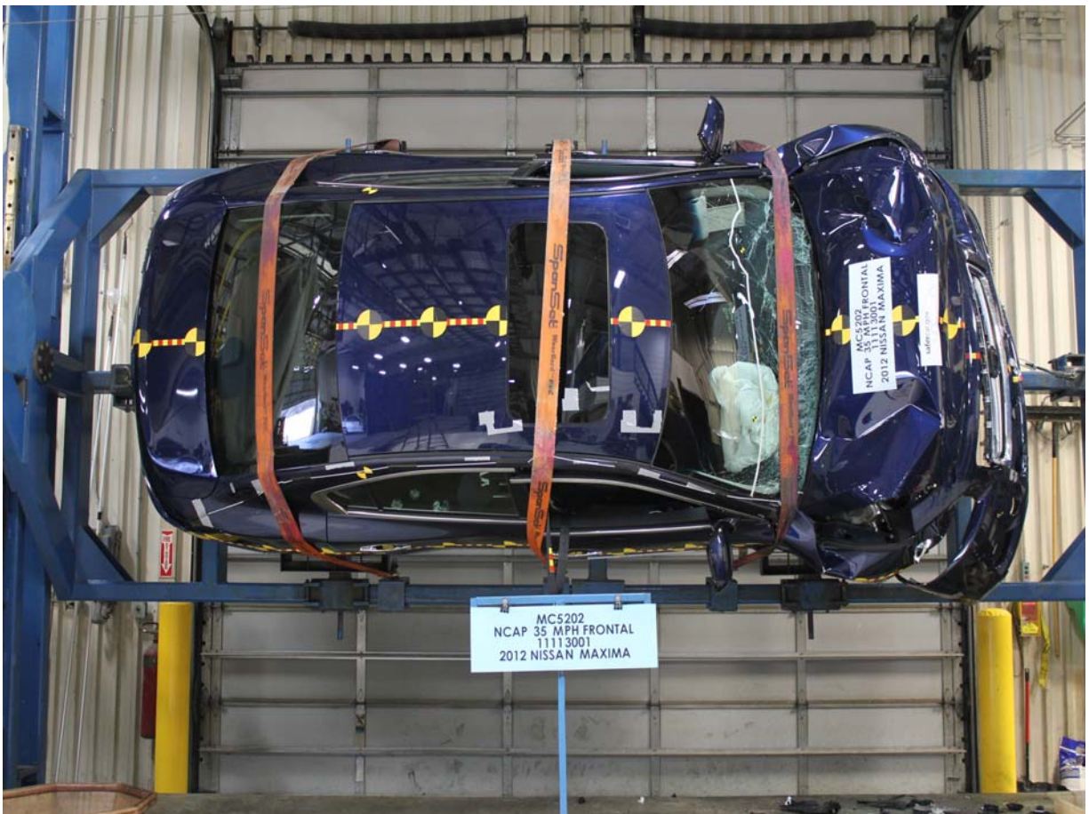
Vehicle at 270 Degrees on Static Rollover Device
