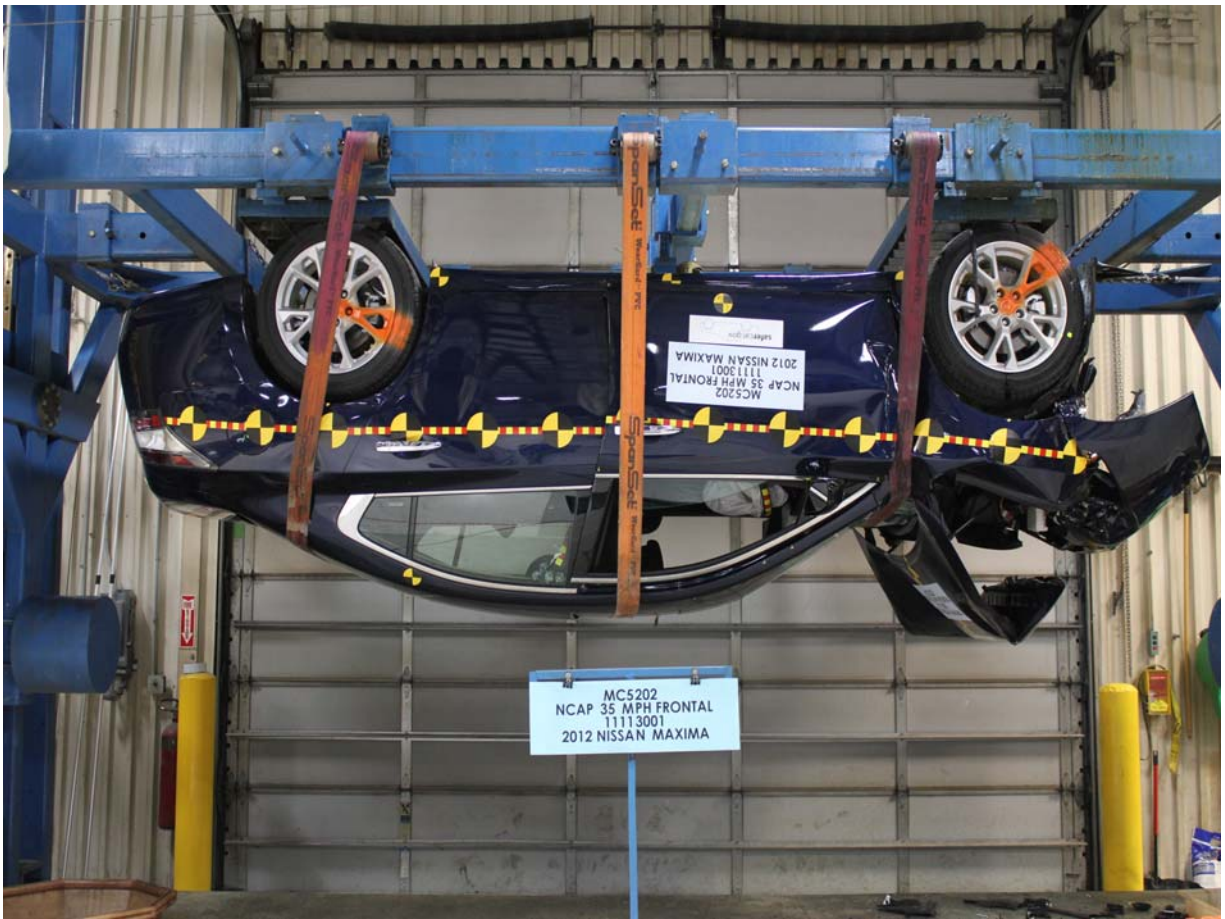
Vehicle at 180 Degrees on Static Rollover Device
