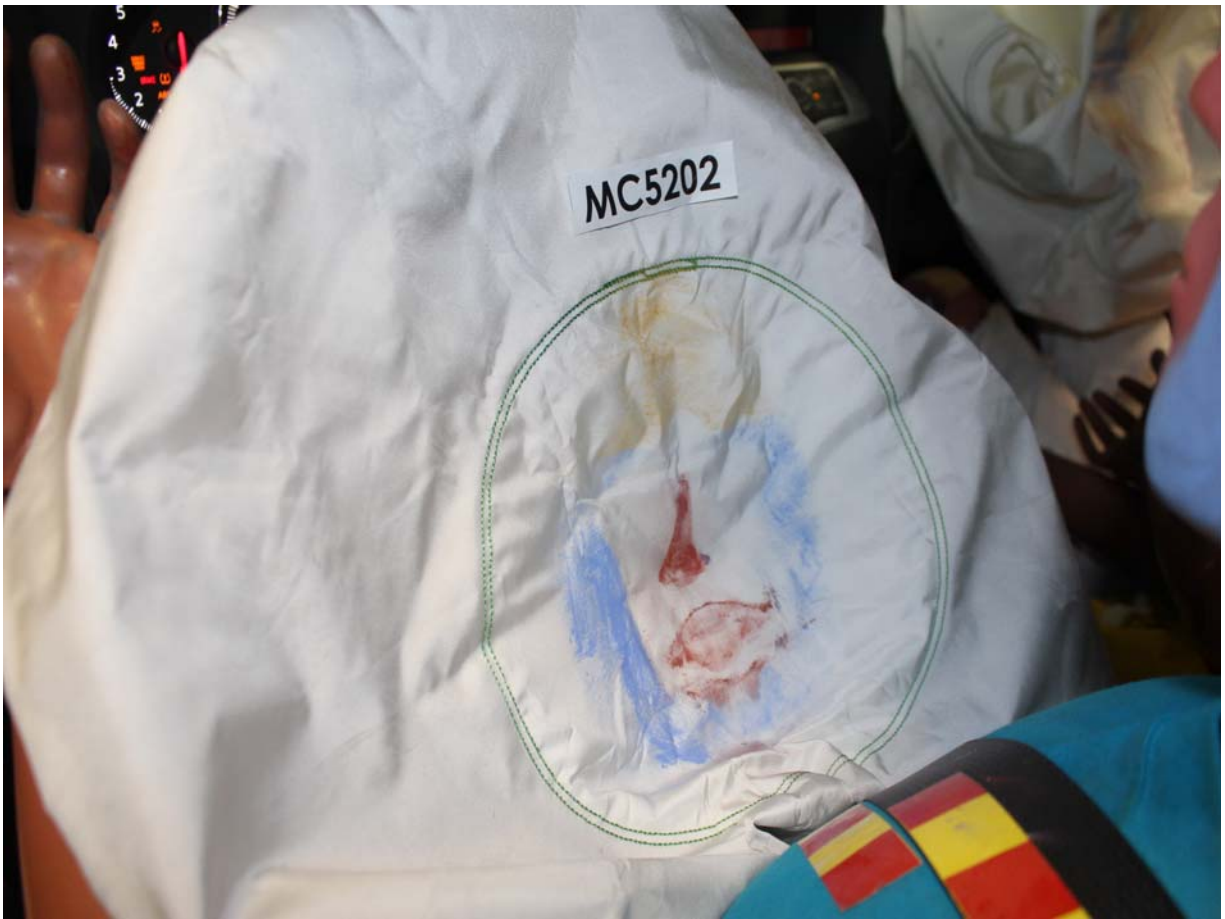
Post-Test Driver Dummy Contact with Airbag
