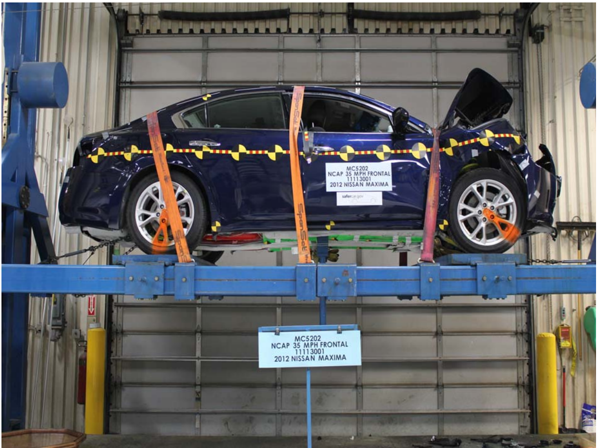
Vehicle at 360 Degrees on Static Rollover Device
