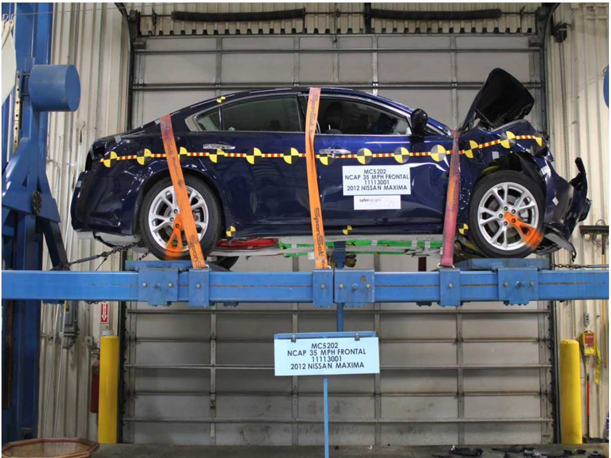
Vehicle at 0 Degrees on Static Rollover Device
