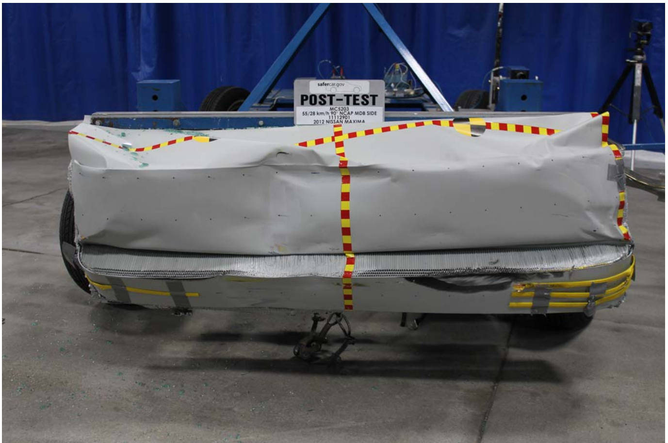
Post-Test Front View of MDB Impactor Face
