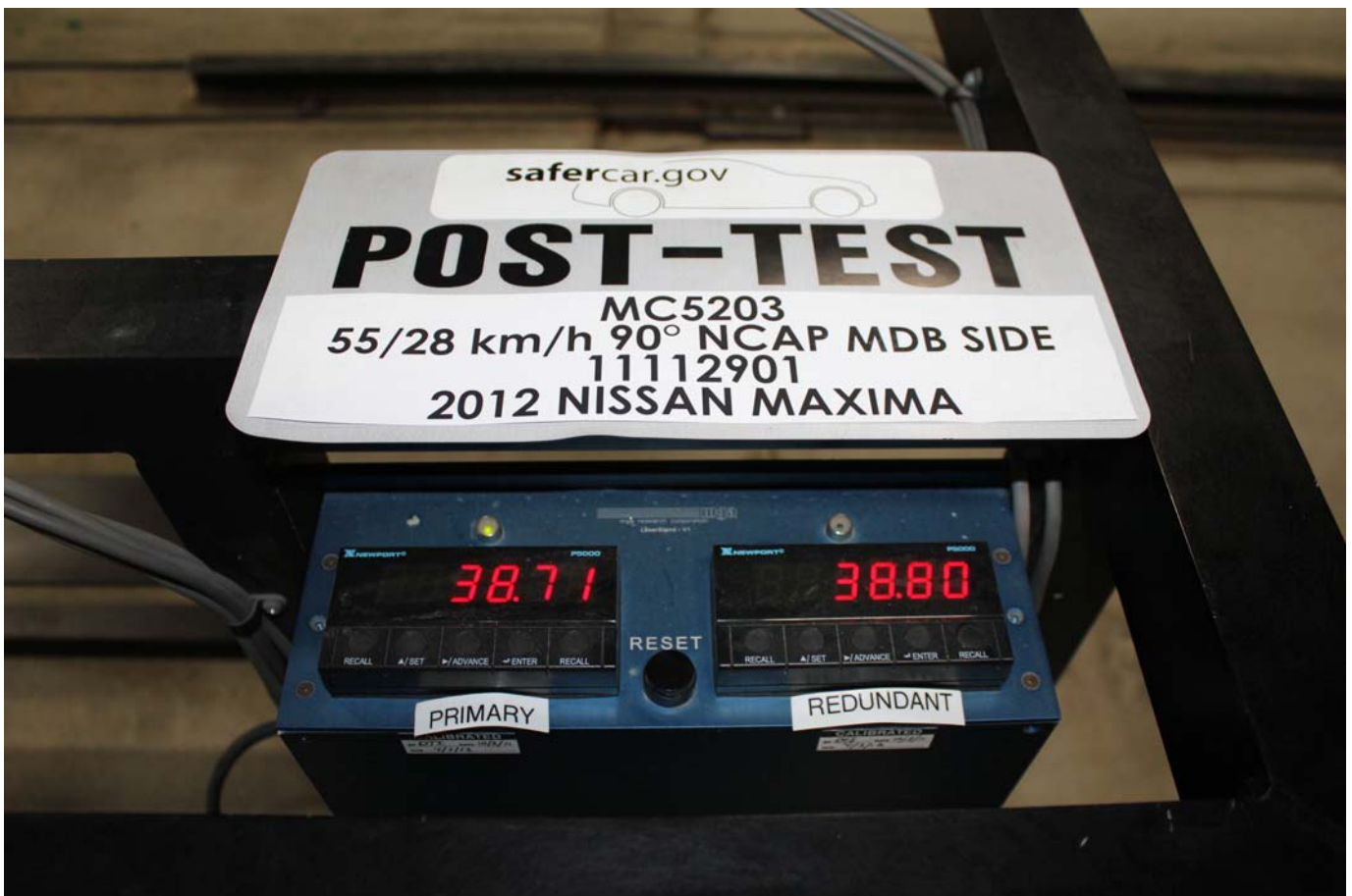
Post-Test Primary and Redundant Speed Trap Read-Out
