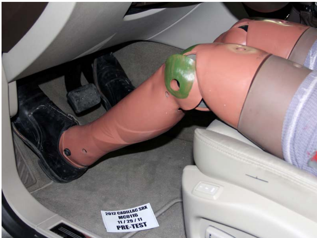
FIGURE 34. Pre-Test Placement of Driver Dummy's Feet
