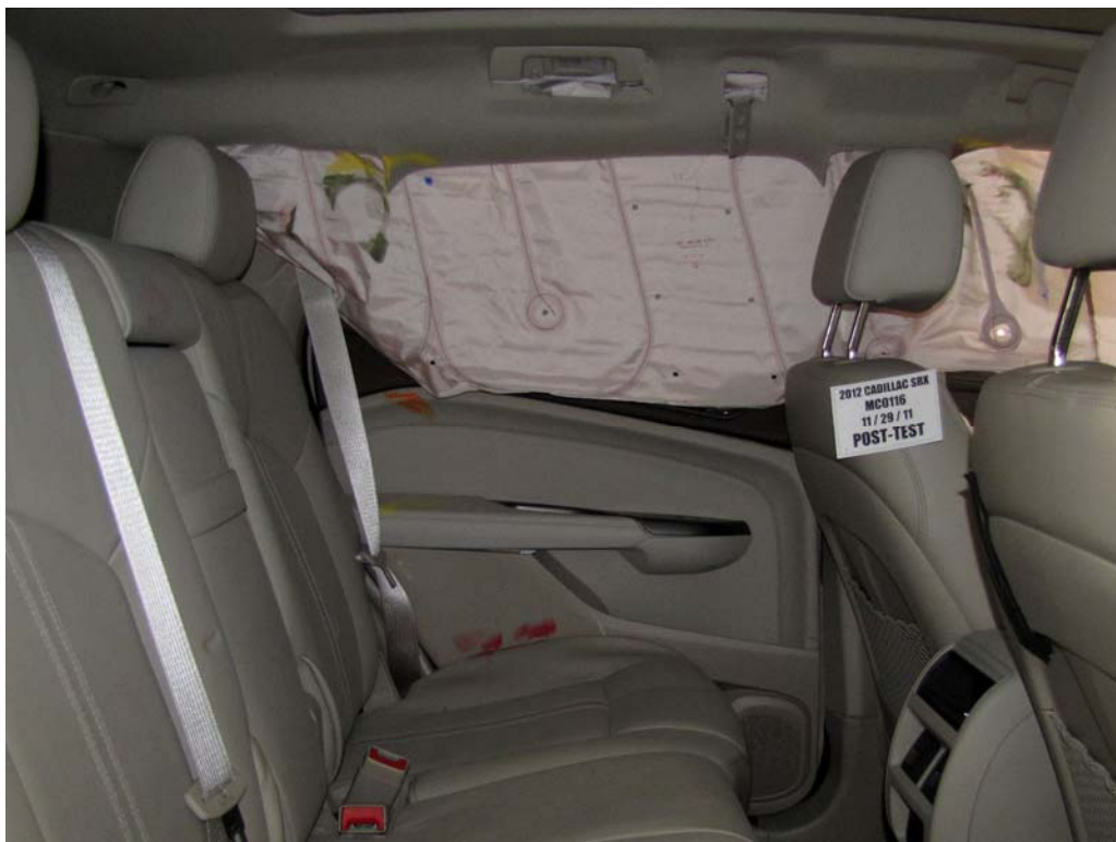
FIGURE 73. Post-Test Rear Passenger Inner Door Panel View
