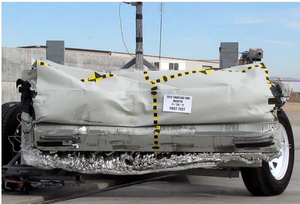
FIGURE 83. Post-Test Front View of MDB Impactor Face
