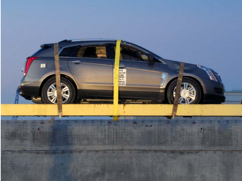
FIGURE 98. FMVSS No. 301 Static Rollover 360 Degrees
