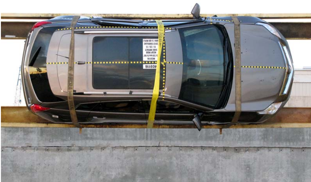
FIGURE 95. FMVSS No. 301 Static Rollover 90 Degrees
