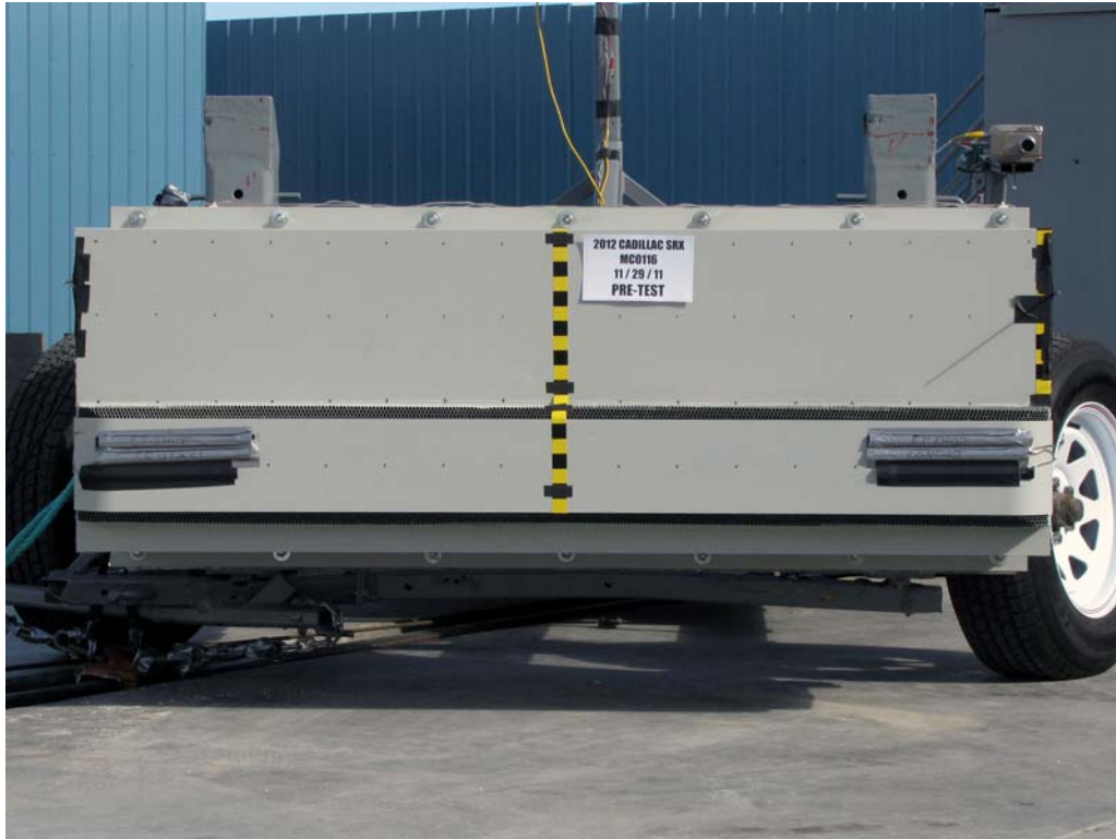
FIGURE 82. Pre-Test Front View of MDB Impactor Face
