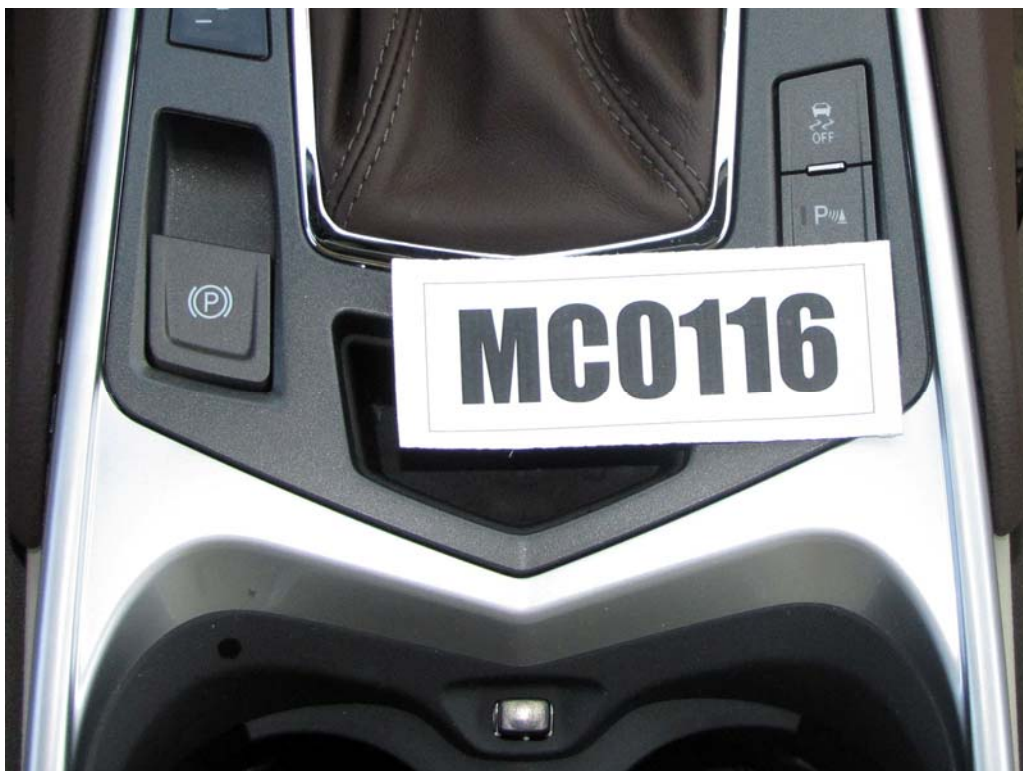
FIGURE 37a. View of Parking Brake Button
