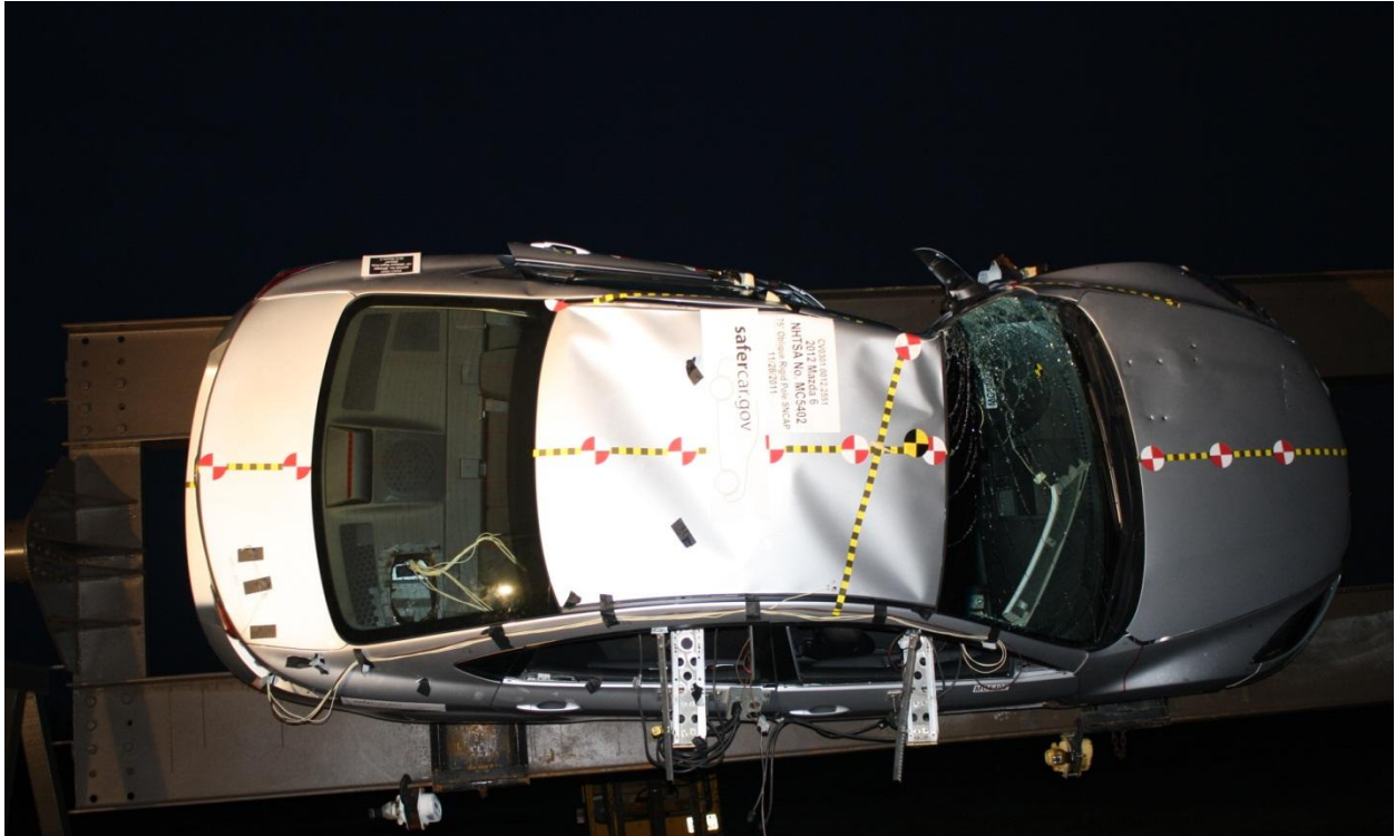
Figure A-65: FMVSS No. 301 Static Rollover 270 Degrees
