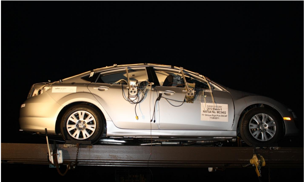
Figure A-66: FMVSS No. 301 Static Rollover 360 Degrees
