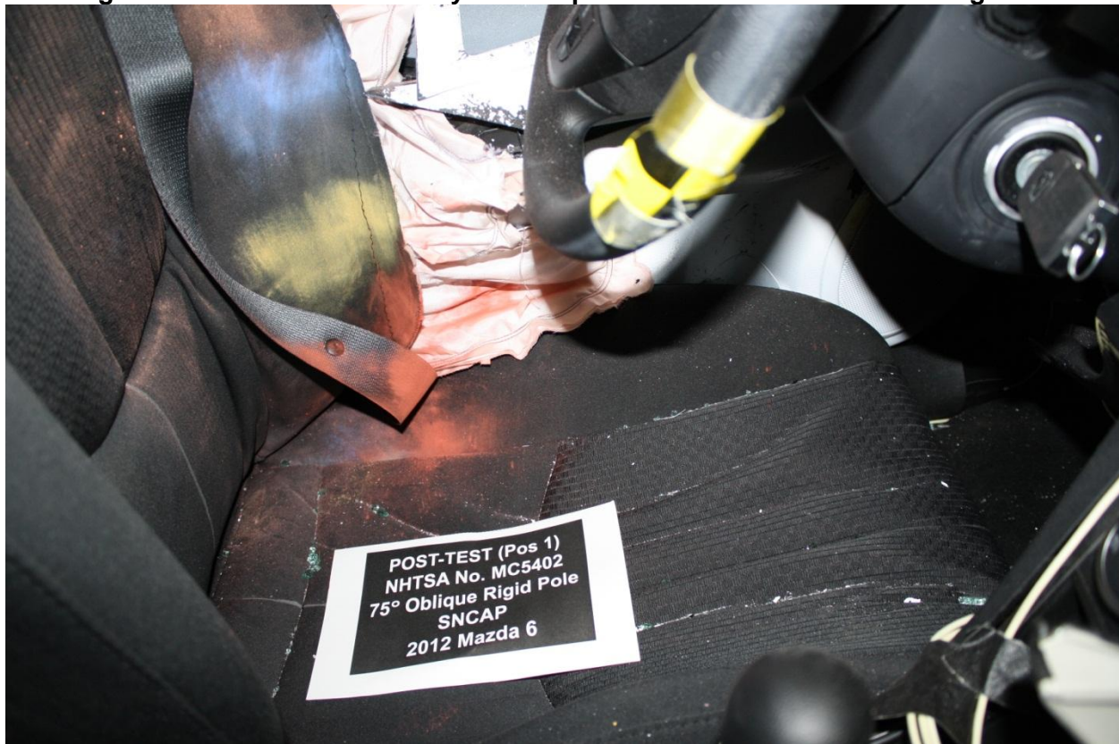
Figure A-50: Post-Test Dummy Close-Up Pelvis Contact With Vehicle Interior
