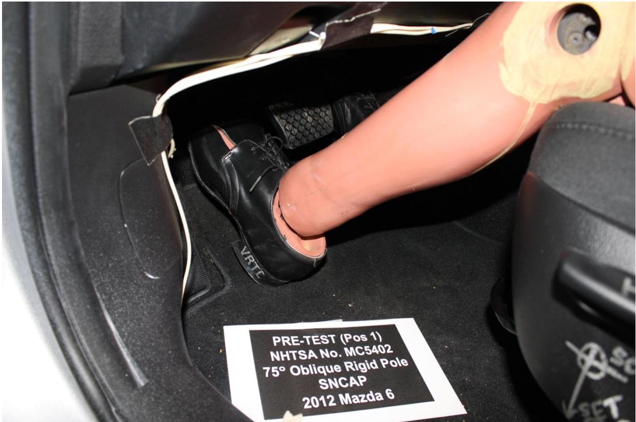
Figure A-32: Pre-Test Placement of Dummy's Feet
