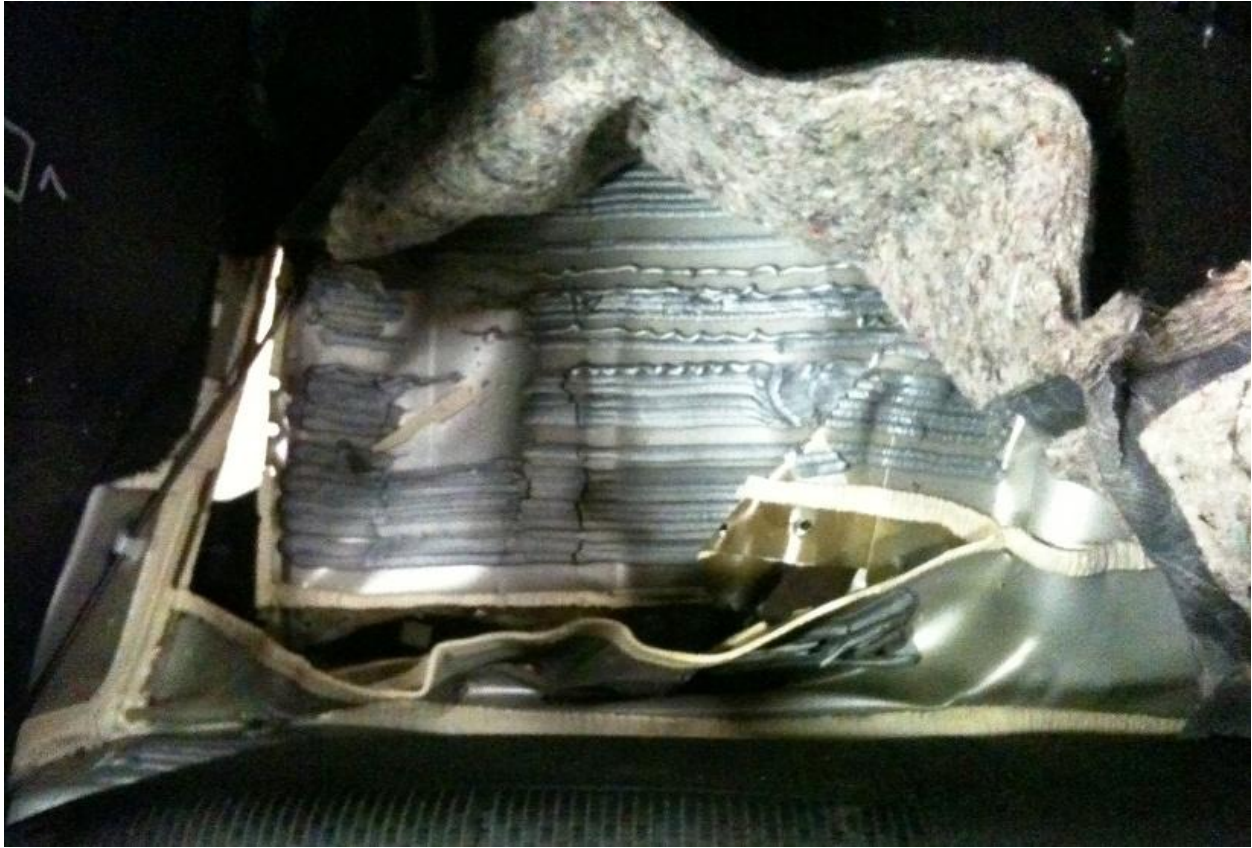
Figure A-71: Post-Test Left Rear Passengers Floor Pan Separation
