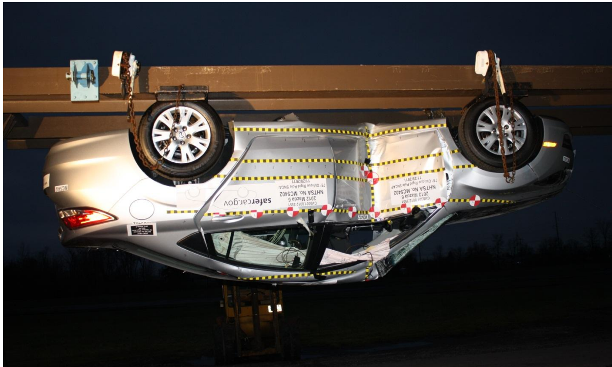
Figure A-64: FMVSS No. 301 Static Rollover 180 Degrees
