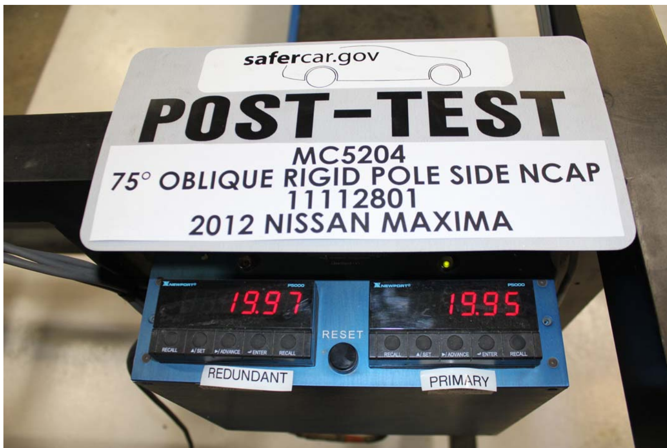
Post-Test Primary and Redundant Speed Trap Read-Out
