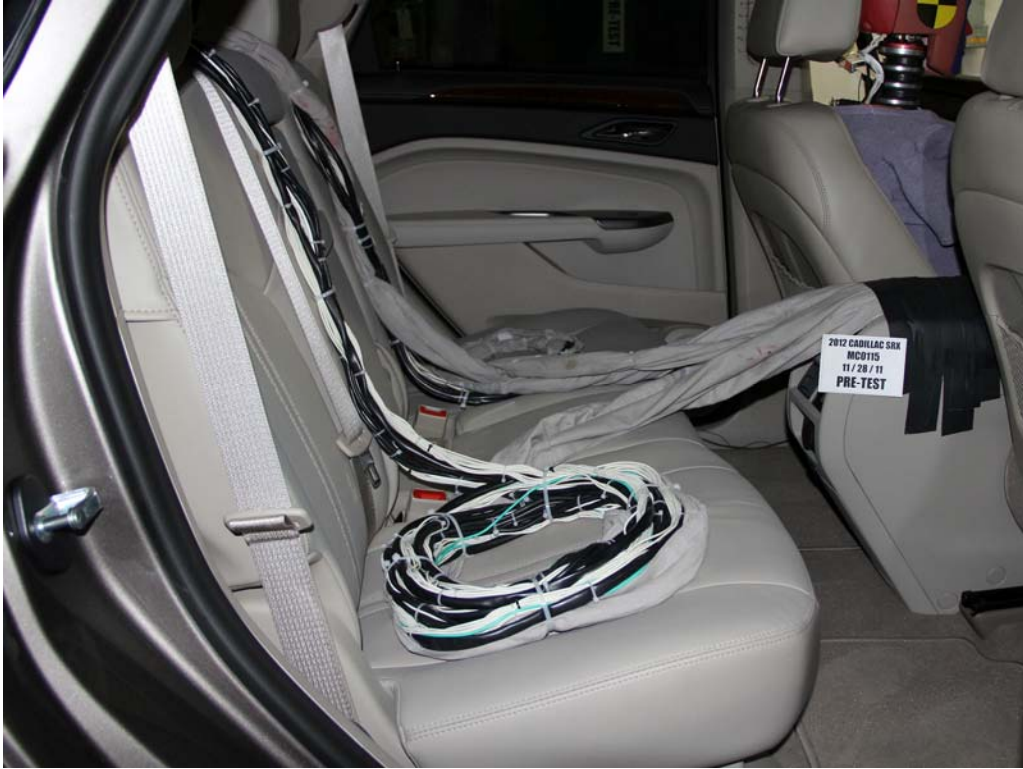
FIGURE 27. Pre-Test Dummy Cable Routing
