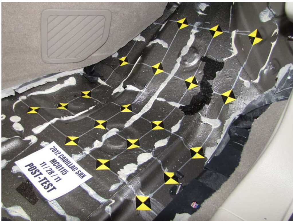
FIGURE 61. Post-Test Passenger's Side Floorpan
