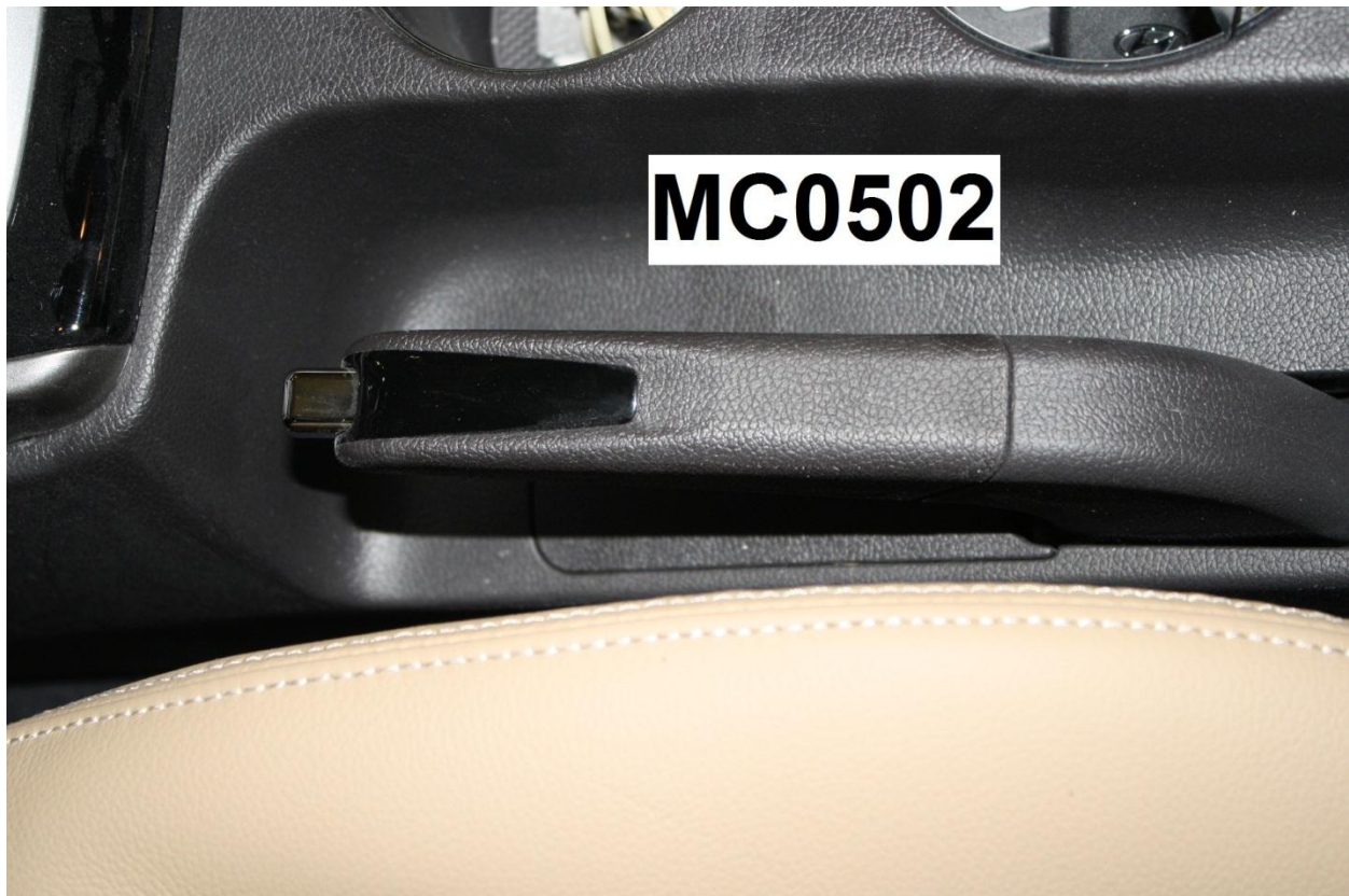
Figure A-35: View of Disengaged Parking Brake
