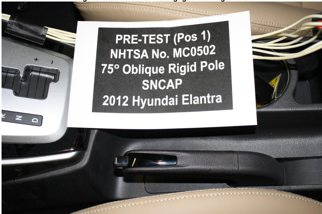
Figure A-36: Pre-Test View of Parking Brake (Should be engaged see video for verification)
