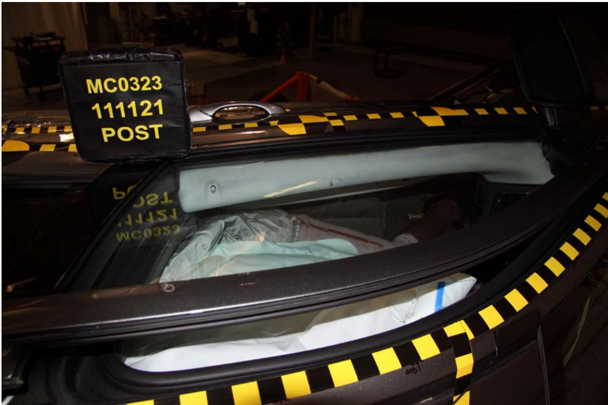
043 Post-Test Driver Dummy and Door Clearance View
