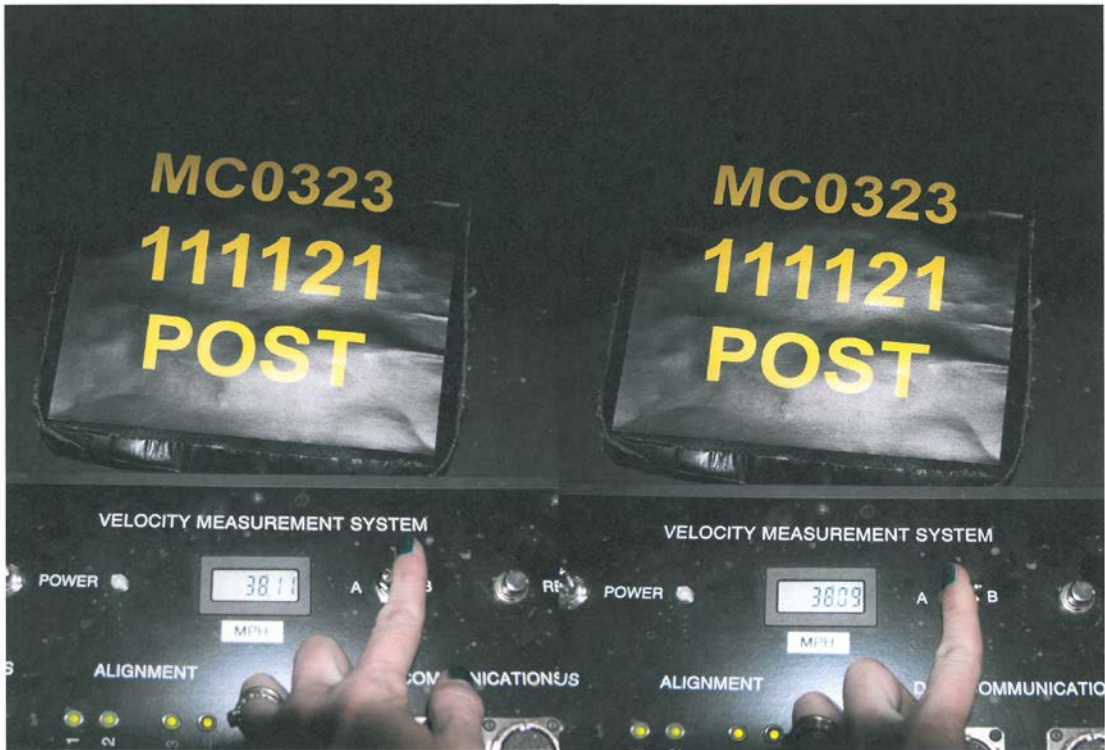
093 Post-Test Primary Speed Trap Read-Out
