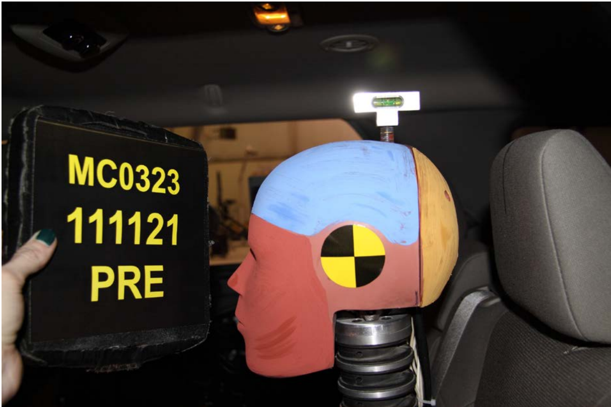
062 Pre-Test View of Rear Passenger Dummy's Head Showing Dummy's Head is Level
