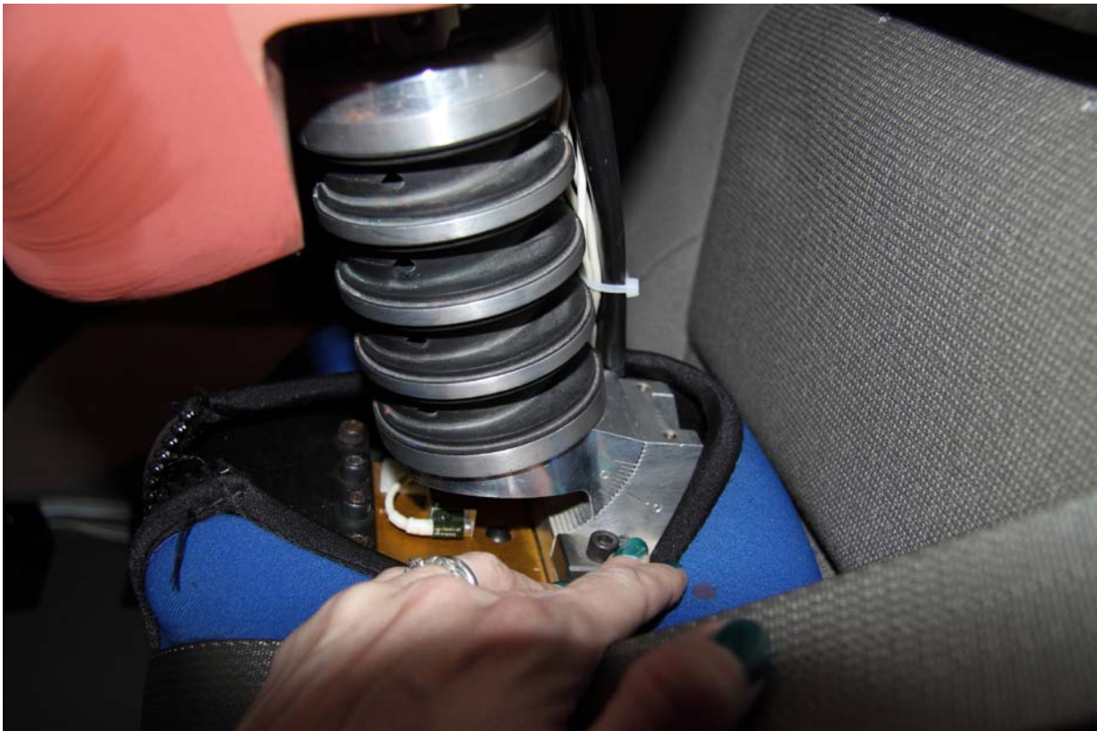
061 Pre-Test View of Rear Passenger Dummy's Neck Showing Position of Adjustable Neck Bracket
