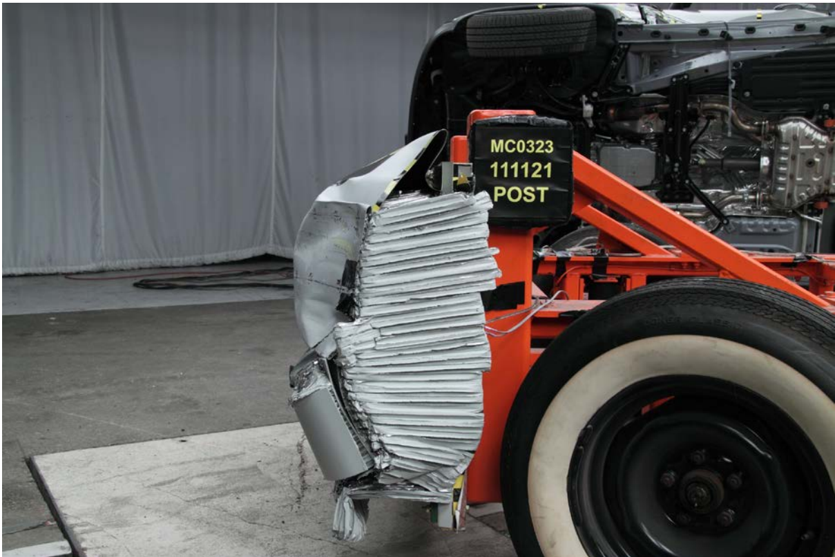
087 Post-Test Left Side View of MDB Impactor Face
