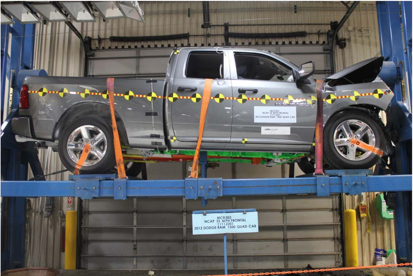
Vehicle at 0 Degrees on Static Rollover Device
