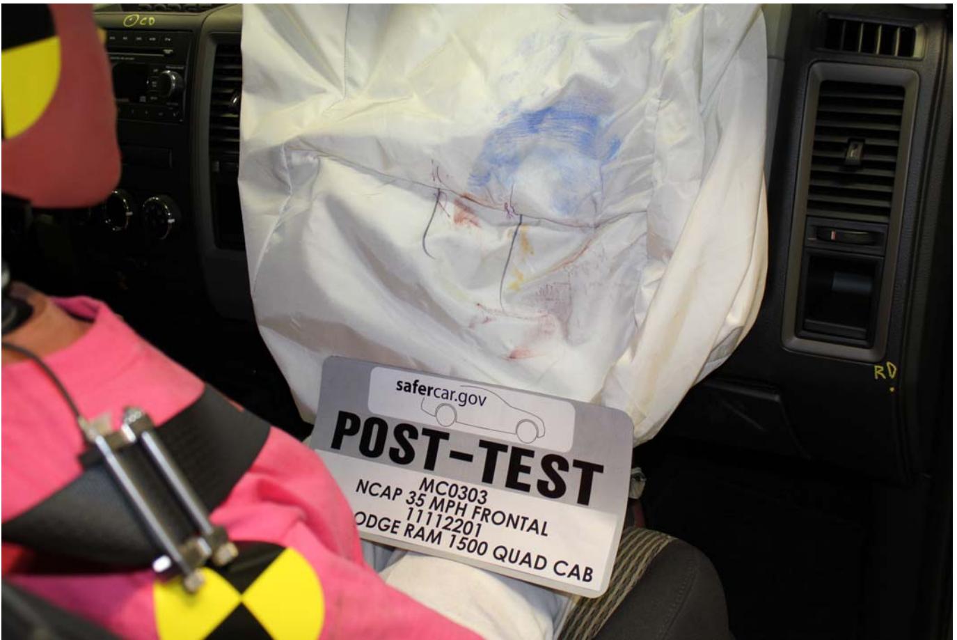
Post-Test Passenger Dummy Contact with Airbag
