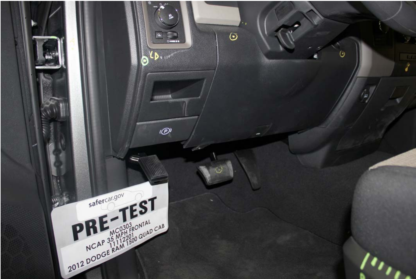
Pre-Test Driver's Side Knee Bolster (without dummy)
