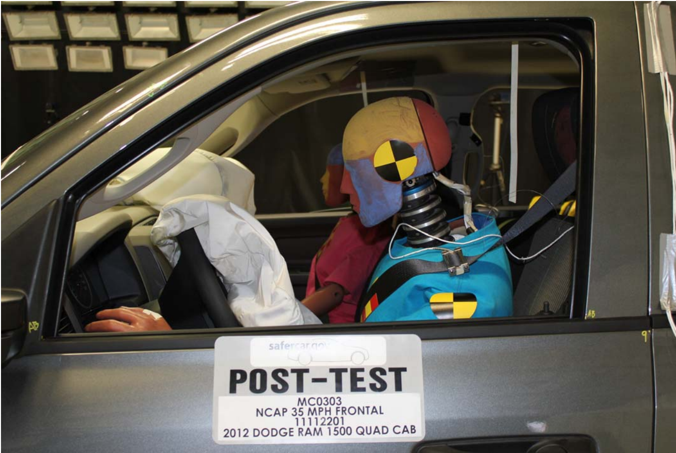
Post-Test Driver Dummy Window View
