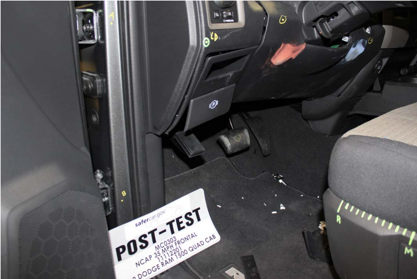
Post-Test Driver's Side Knee Bolster (without dummy)
