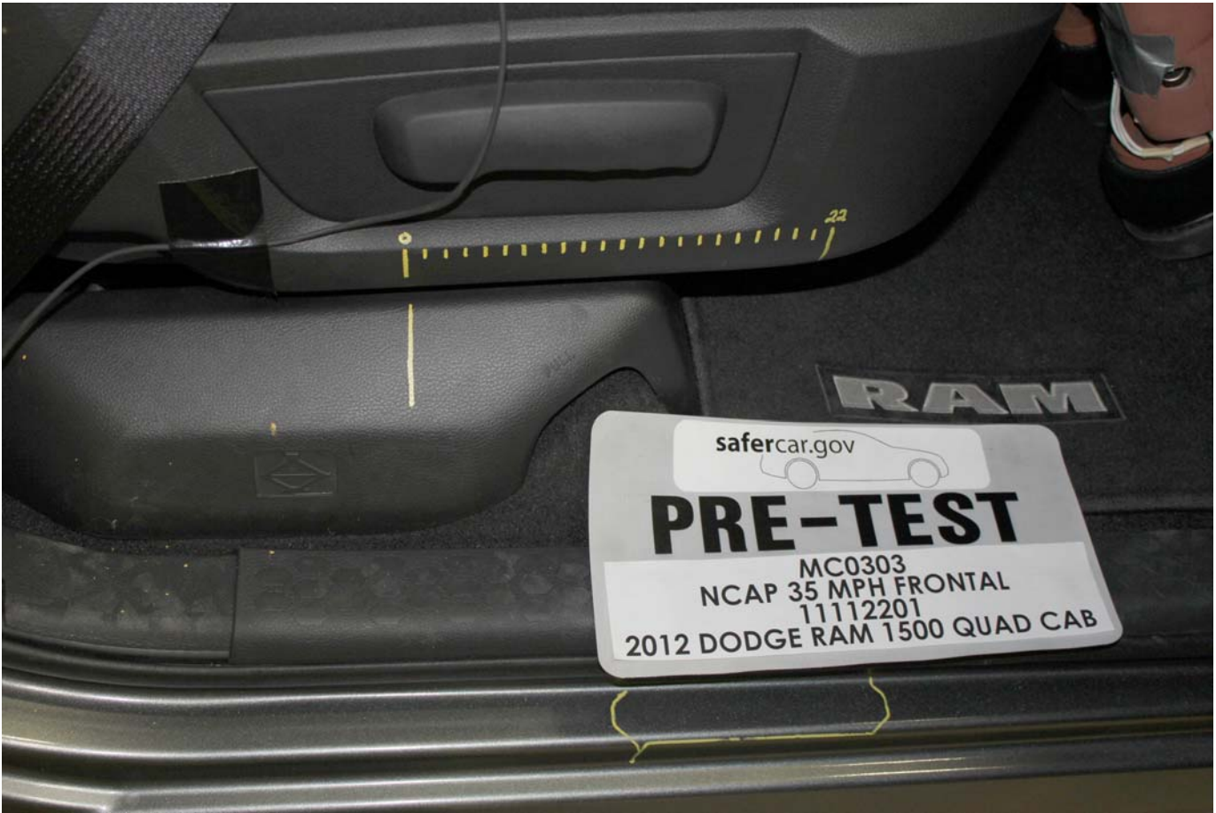
Pre-Test Passenger's Seat Fore-Aft Markings
