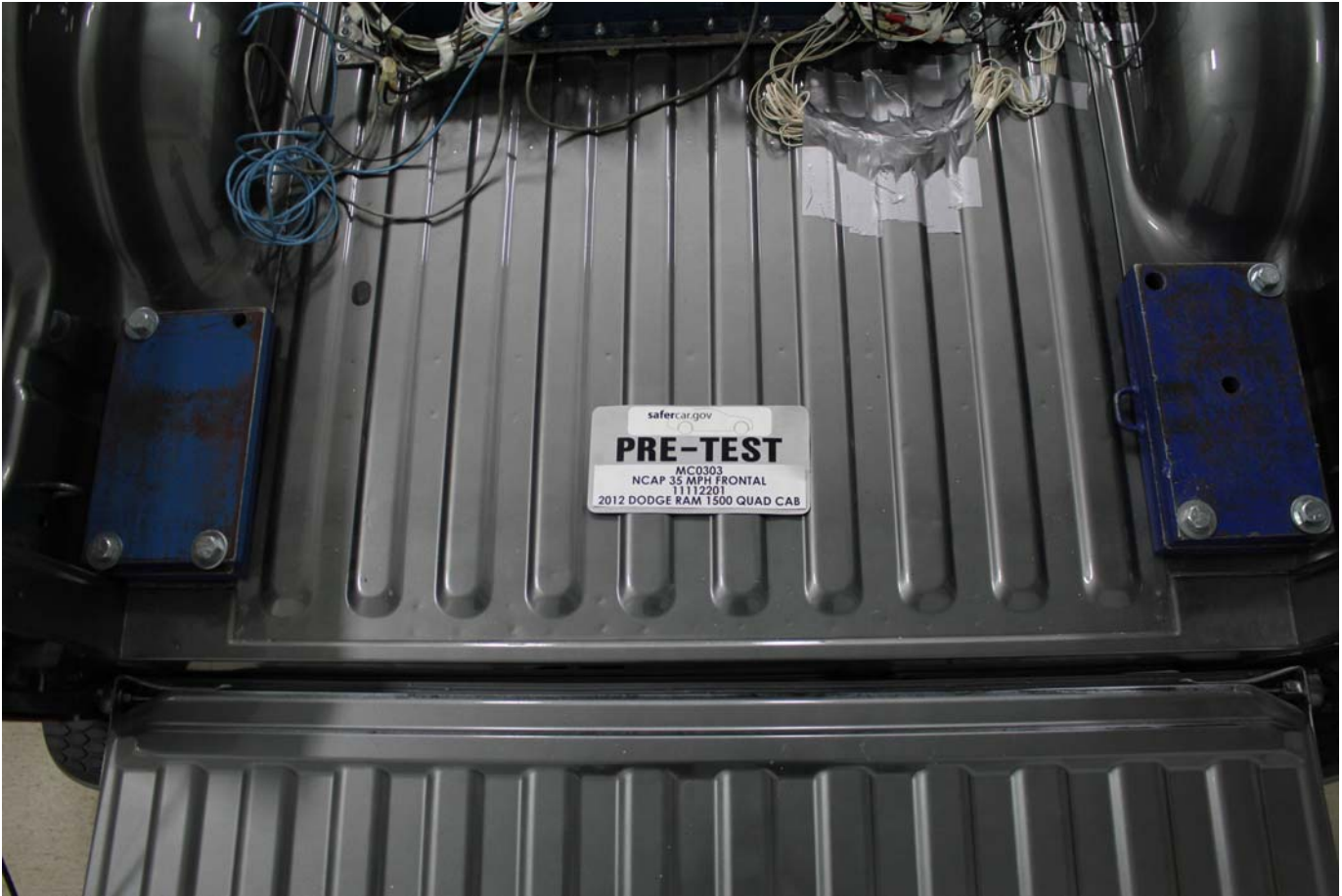
Ballast Installed in Vehicle
