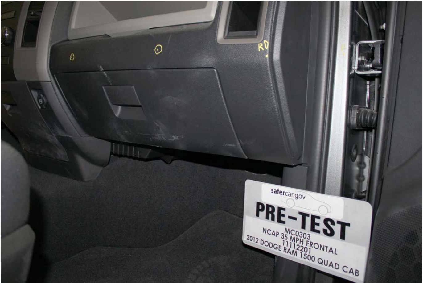
Pre-Test Passenger's Side Knee Bolster (without dummy)
