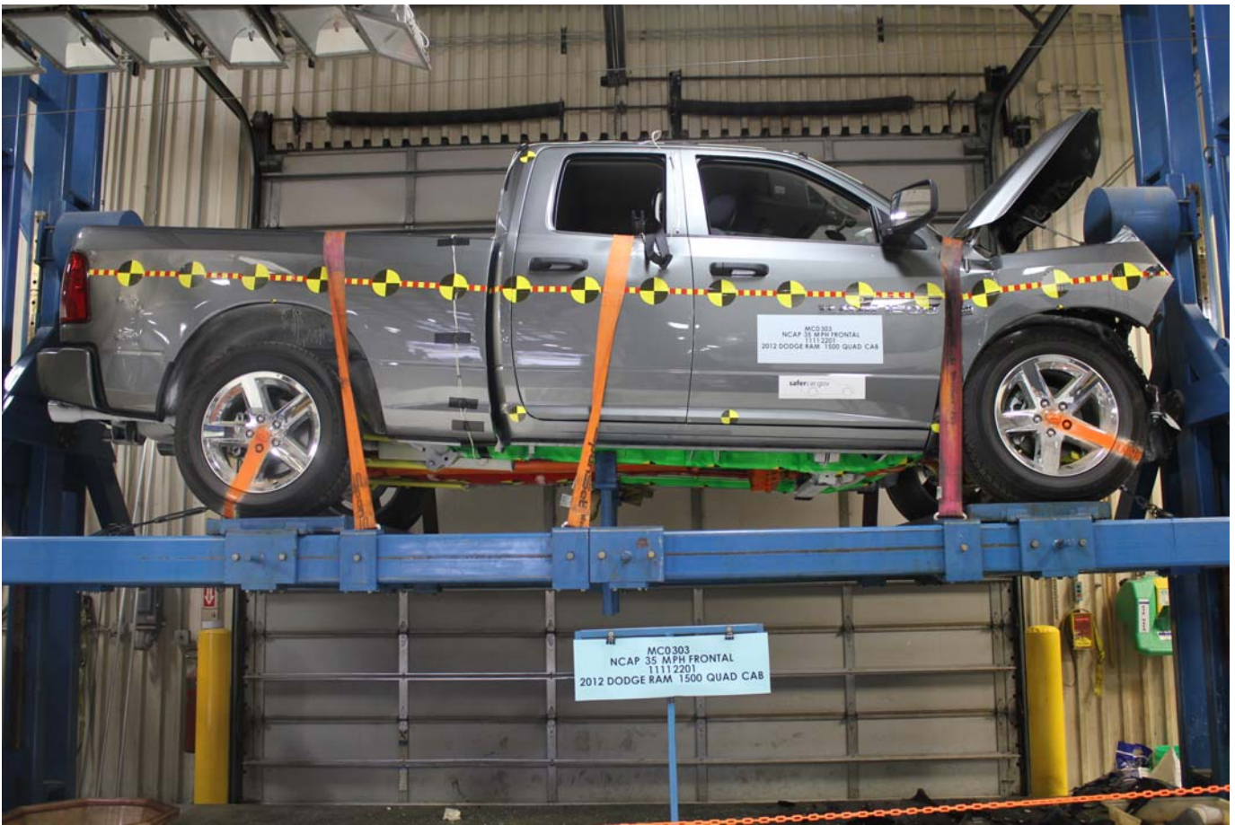
Vehicle at 360 Degrees on Static Rollover Device
