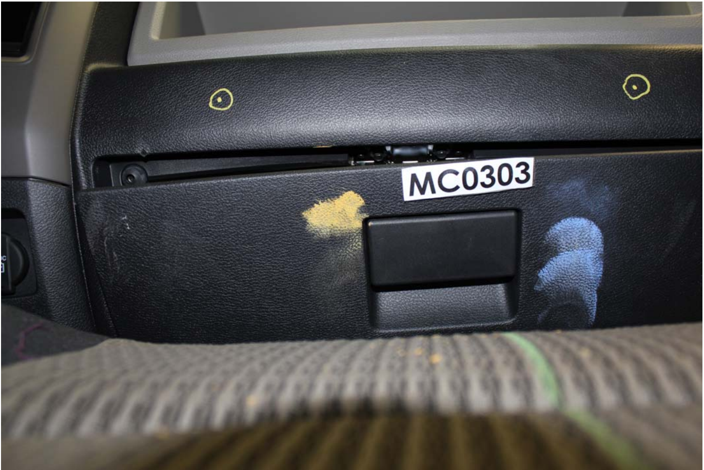
Post-Test Passenger Dummy Contact with Glovebox
