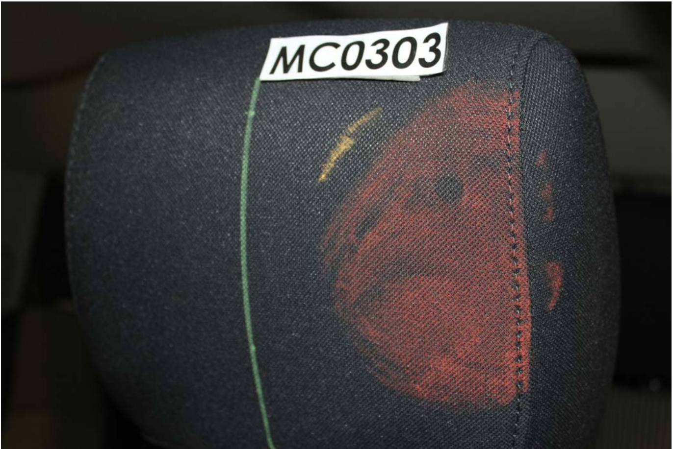
Post-Test Driver Dummy Contact with Headrest
