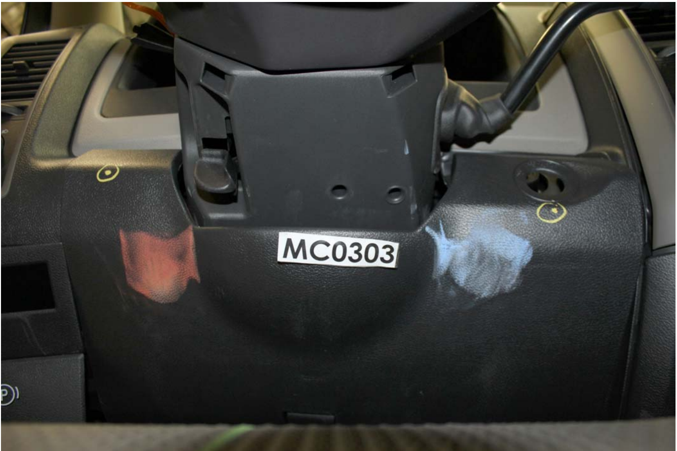
Post-Test Driver Dummy Contact with Knee Bolster
