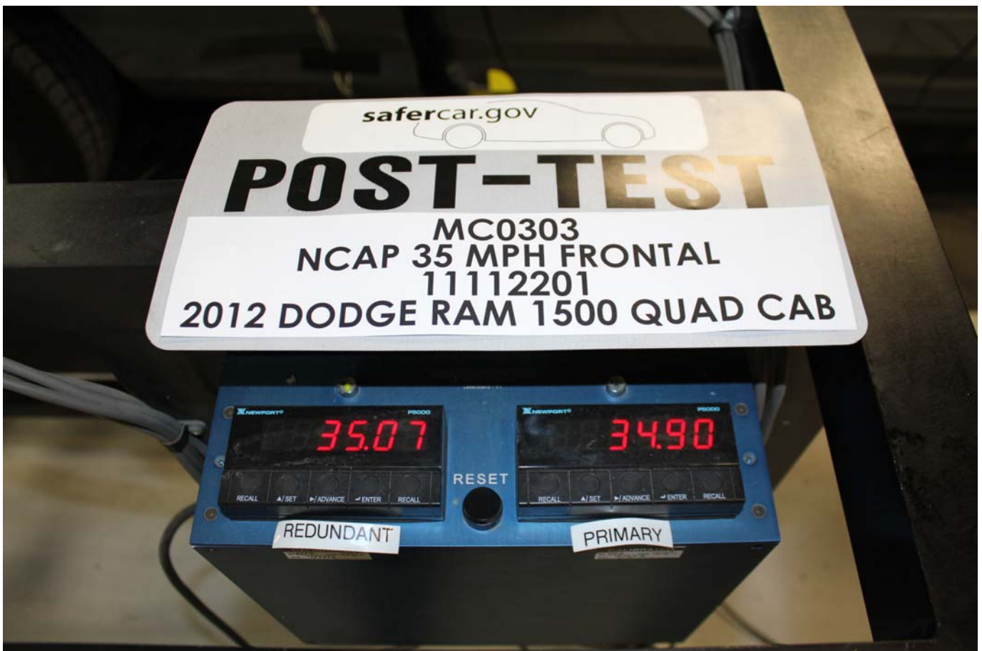
Post-Test Speed Trap Read-Out
