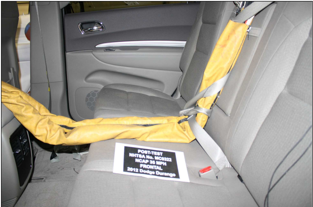
Figure A-28: Post-Test Dummy Cable Routing
