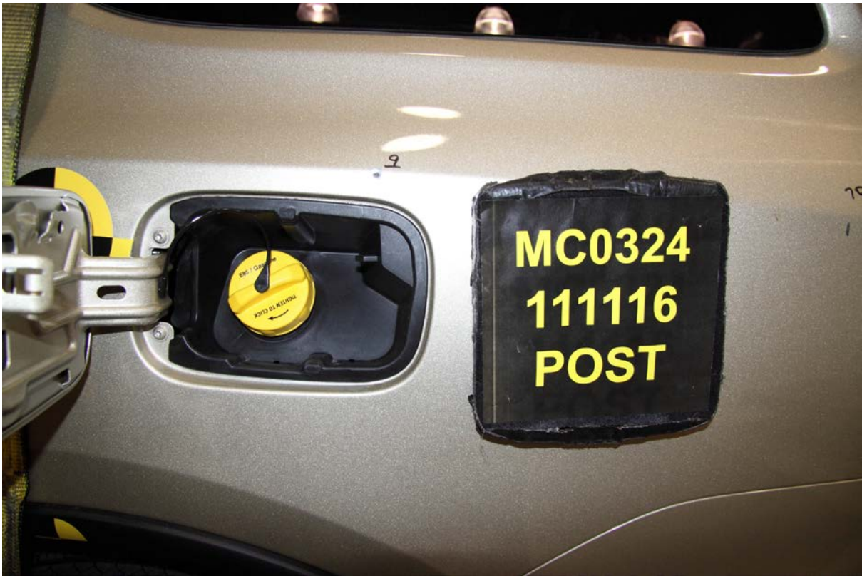
53 Post-Test View of Fuel Filler Cap or Fuel Filler Neck
