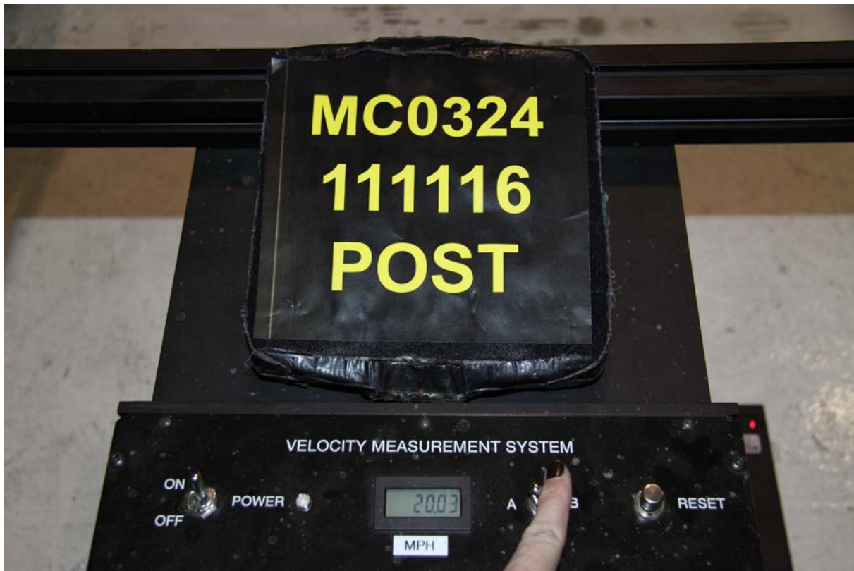
61 Post-Test Primary and Redundant Speed Trap Read-Out
