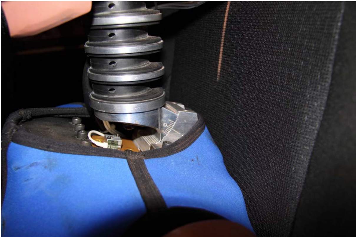
30 Pre-Test Left Side View of Dummy's Neck Showing Position of Adjustable Neck Bracket
