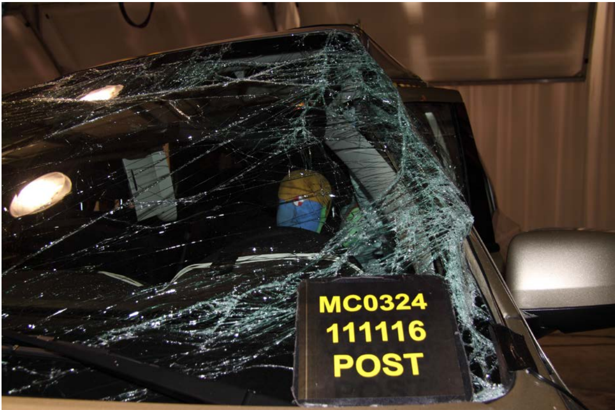
22 Post-Test Front Close-Up View of Dummy
