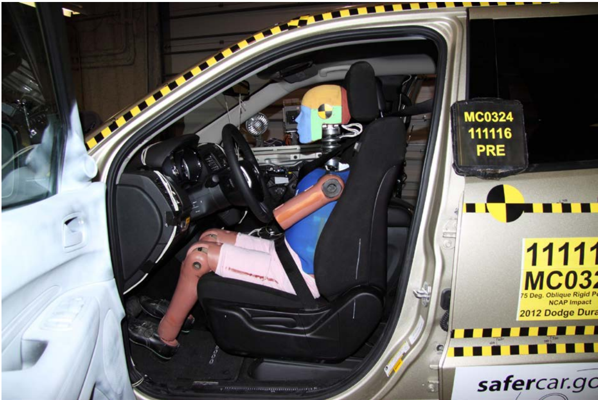
23 Pre-Test Left Side View of Dummy Showing Belt and Chalking
