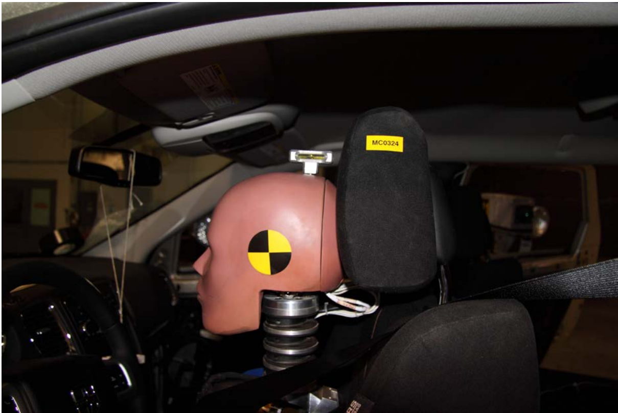
27 Pre-Test Front View of Dummy Head and Shoulders in Relation to Head Restraint
