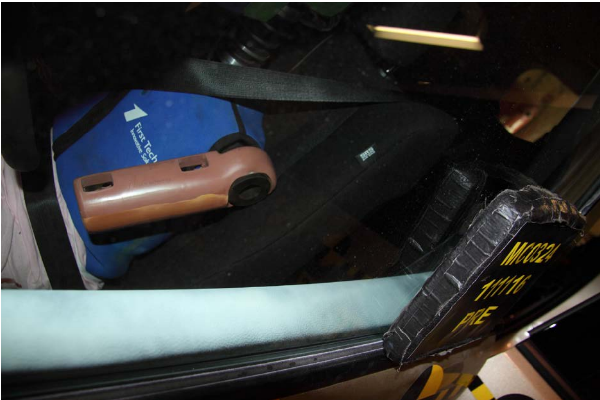
40 Pre-Test Dummy and Door Clearance View
