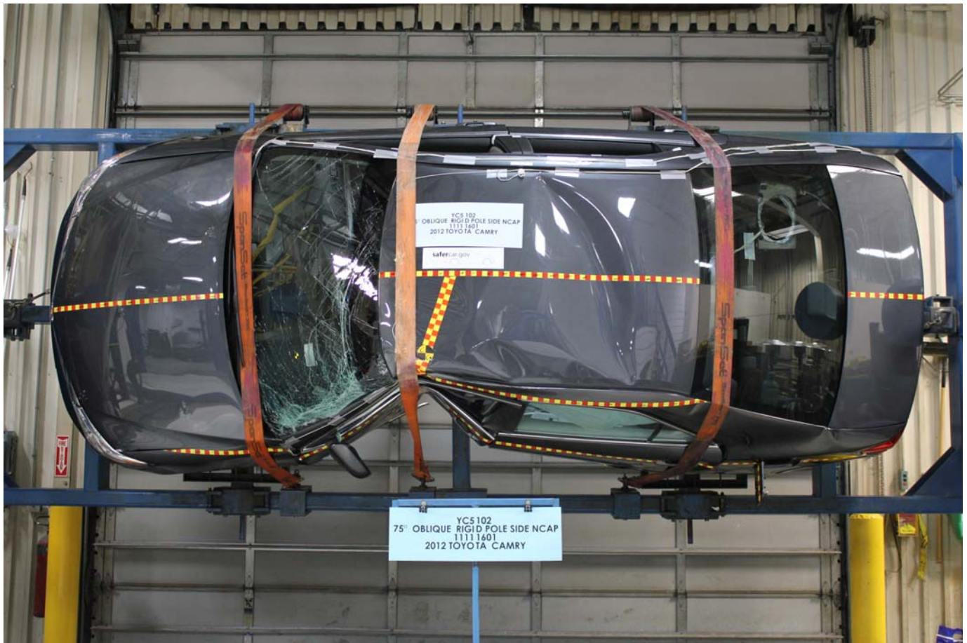
FMVSS No. 301 Static Rollover 90 Degrees
