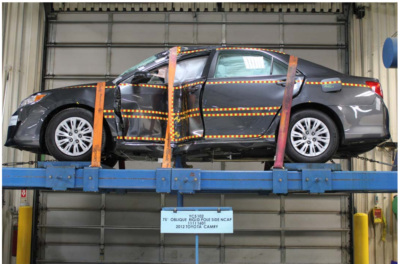
FMVSS No. 301 Static Rollover 0 Degrees
