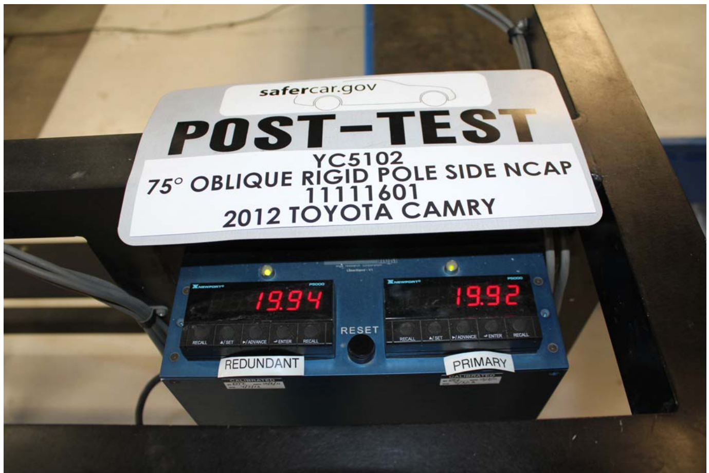
Post-Test Primary and Redundant Speed Trap Read-Out
