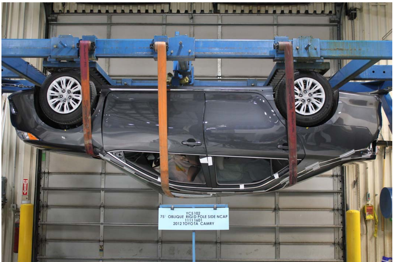
FMVSS No. 301 Static Rollover 180 Degrees
