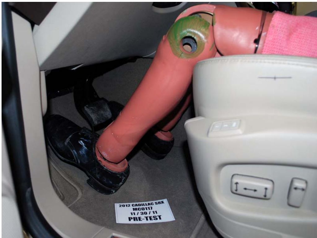
FIGURE 32. Pre-Test Placement of Dummy's Feet
