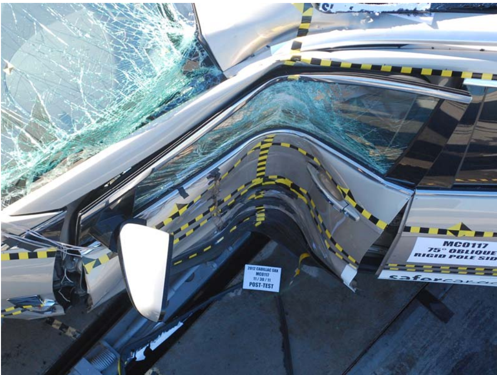
FIGURE 41. Post-Test Driver Dummy and Door Clearance
