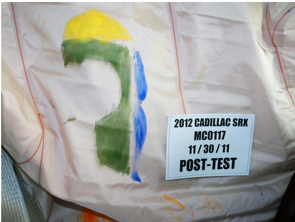
FIGURE 47. Post-Test Dummy Close-Up Head Contact with Side Airbag View
