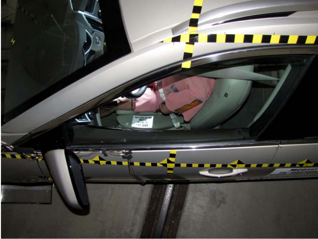
FIGURE 40. Pre-Test Driver Dummy and Door Clearance
