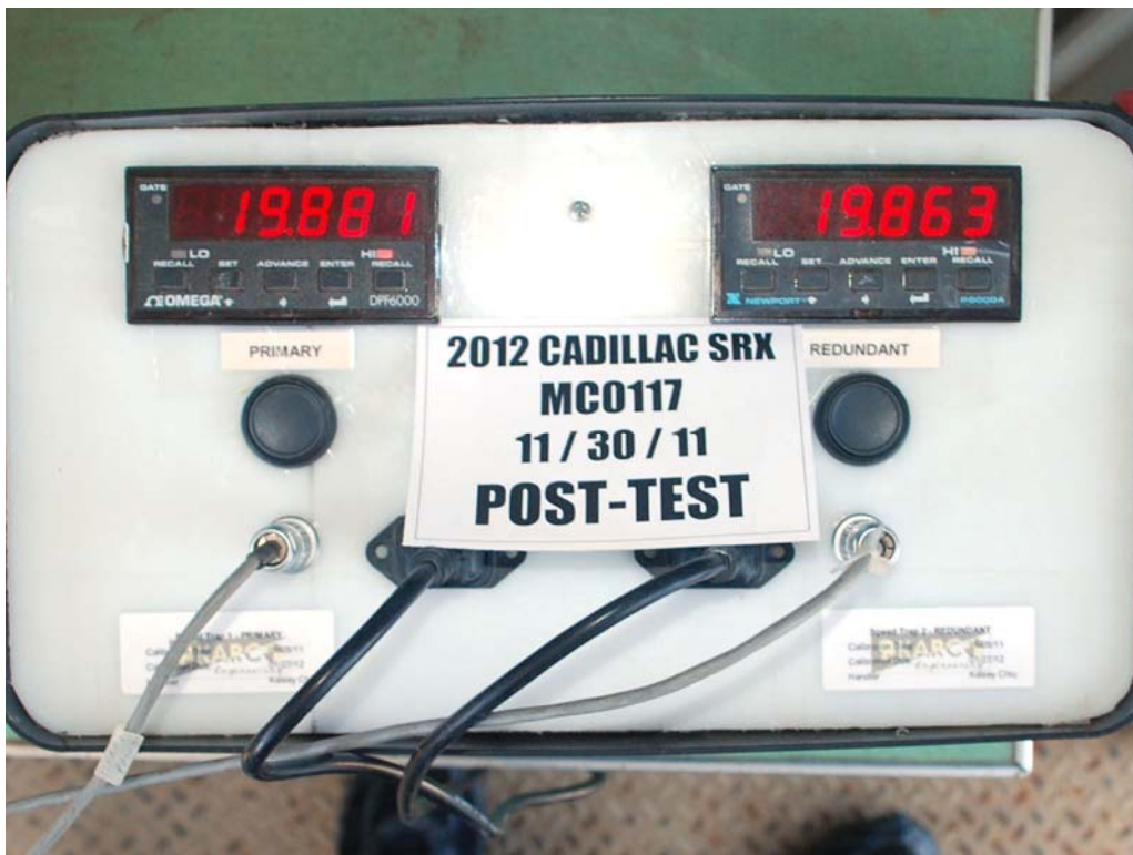
FIGURE 61. Post-Test Primary and Redundant Speed Trap Read-Out
