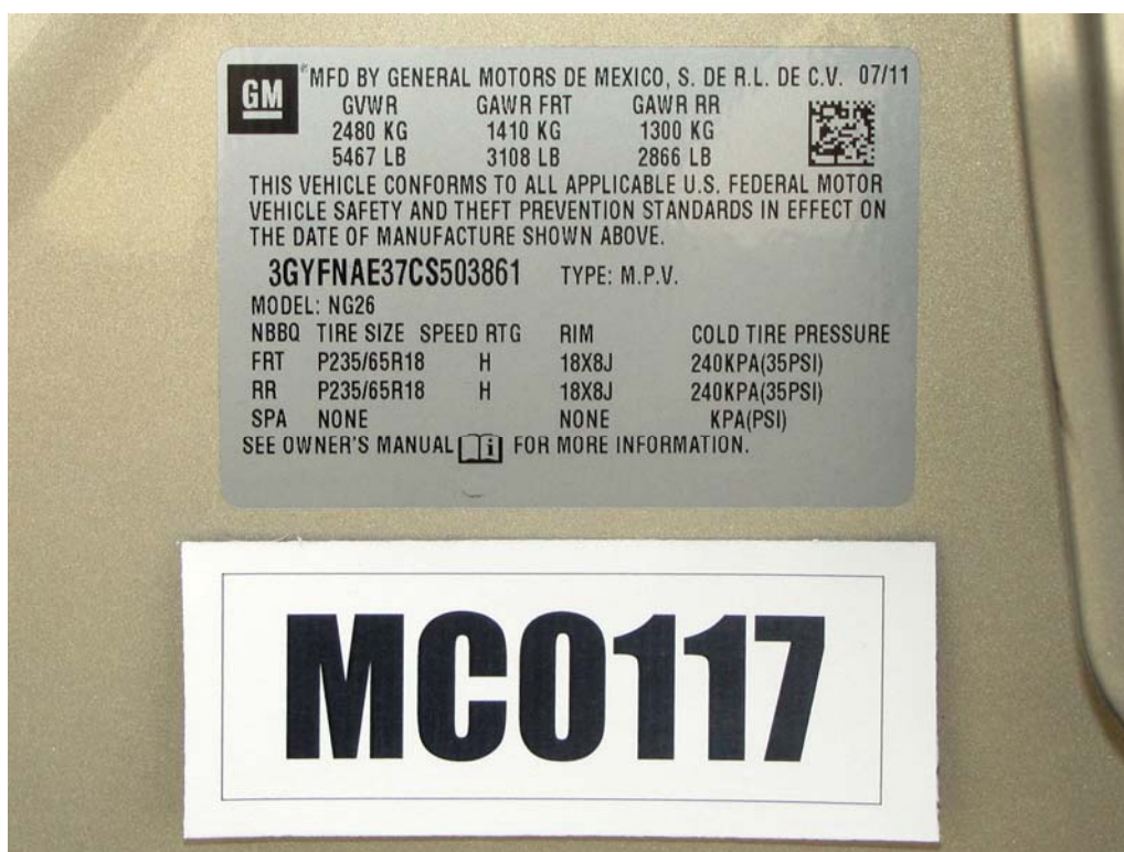
FIGURE 54. Close-Up View of Vehicle's Certification Label
