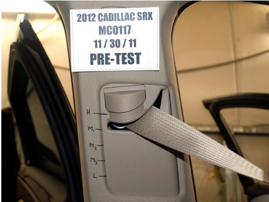
FIGURE 33. Pre-Test View of Belt Anchorage for Dummy
