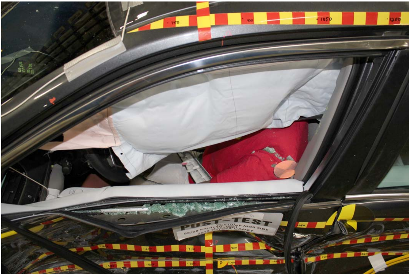
Post-Test Driver Dummy and Door Clearance View
