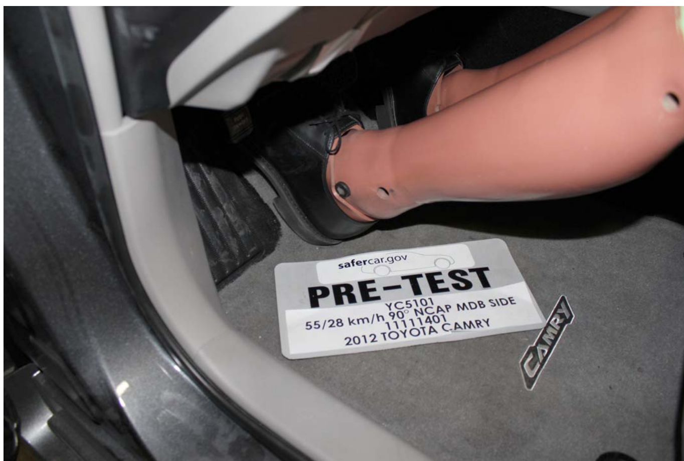
Pre-Test Placement of Driver Dummy's Feet
