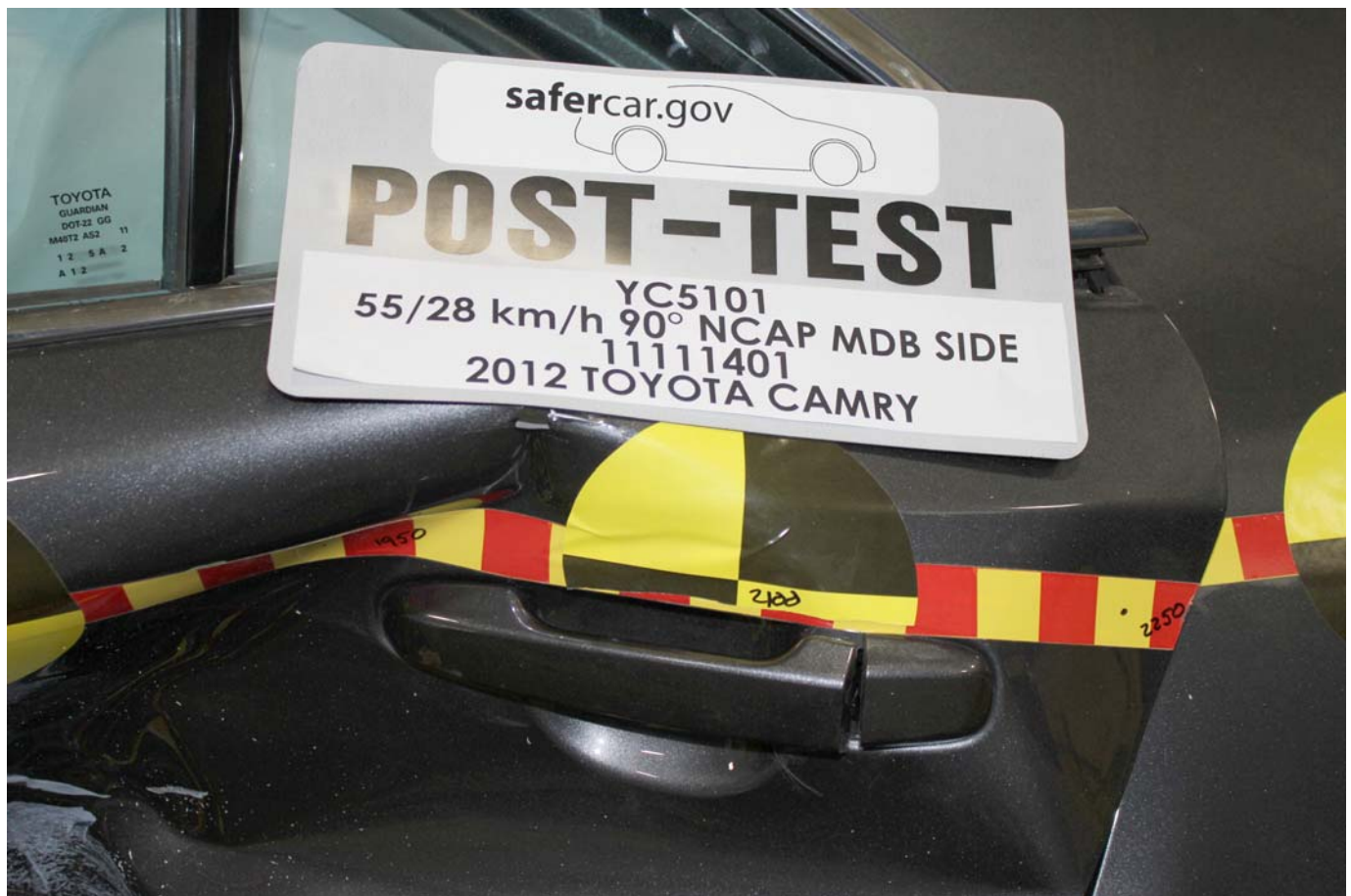
Post-Test Left Rear Door Latch Close-Up
