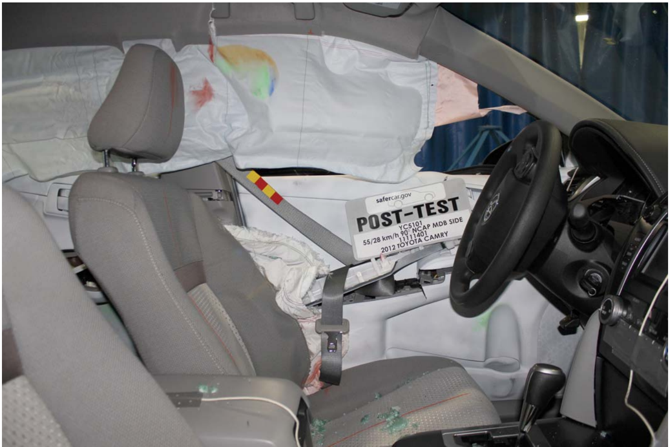
Post-Test Driver Inner Door Panel View
