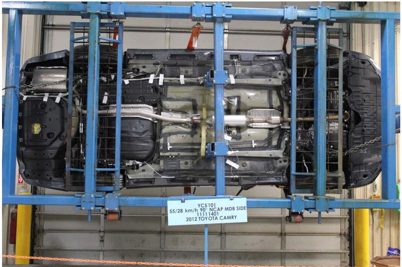
FMVSS No. 301 Static Rollover 90 Degrees
