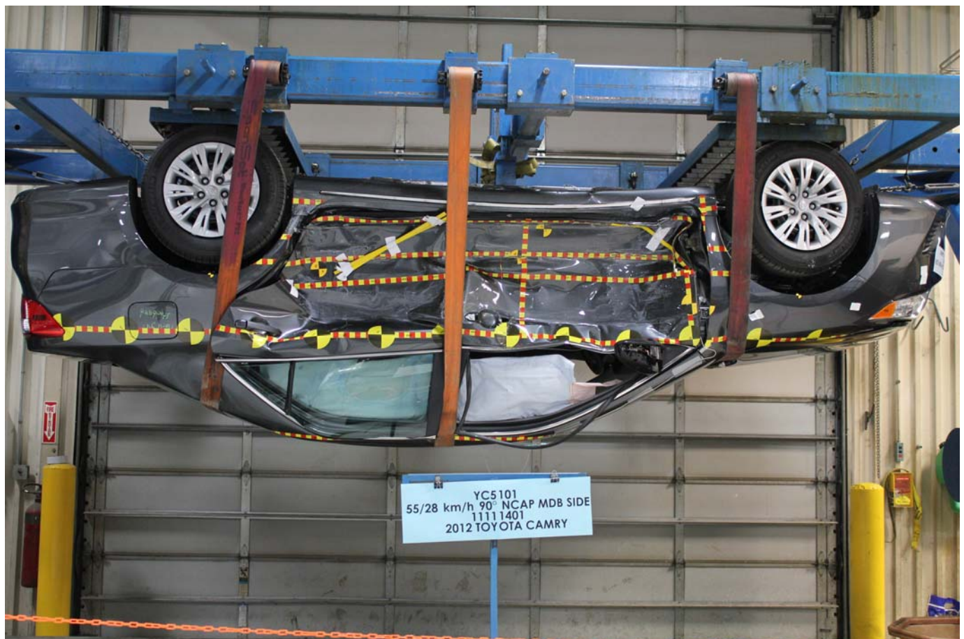
FMVSS No. 301 Static Rollover 180 Degrees
