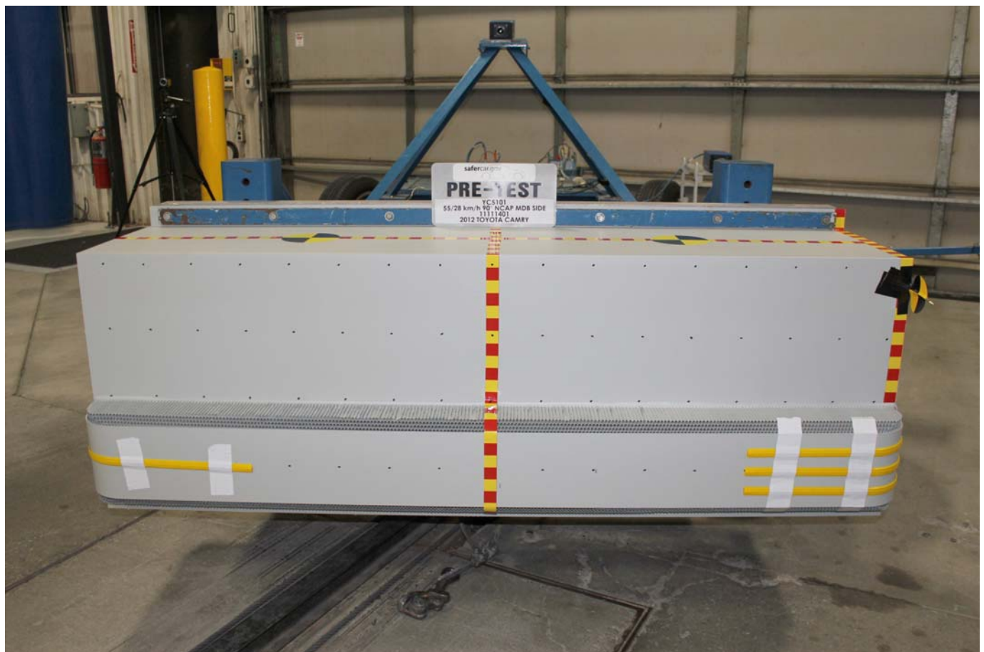
Pre-Test Front View of MDB Impactor Face
