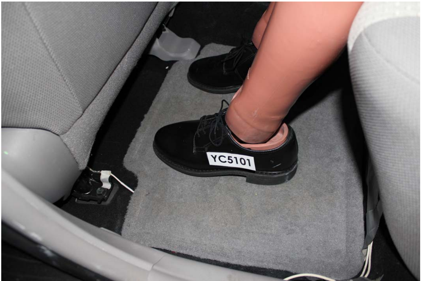
Pre-Test Placement of Rear Passenger Dummy's Feet
