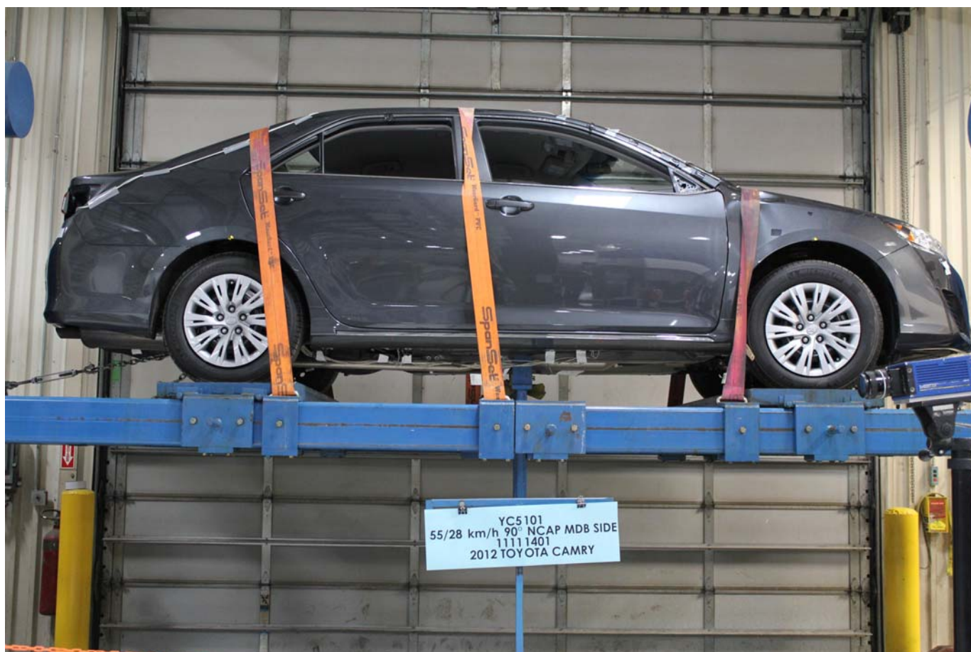
FMVSS No. 301 Static Rollover 360 Degrees
