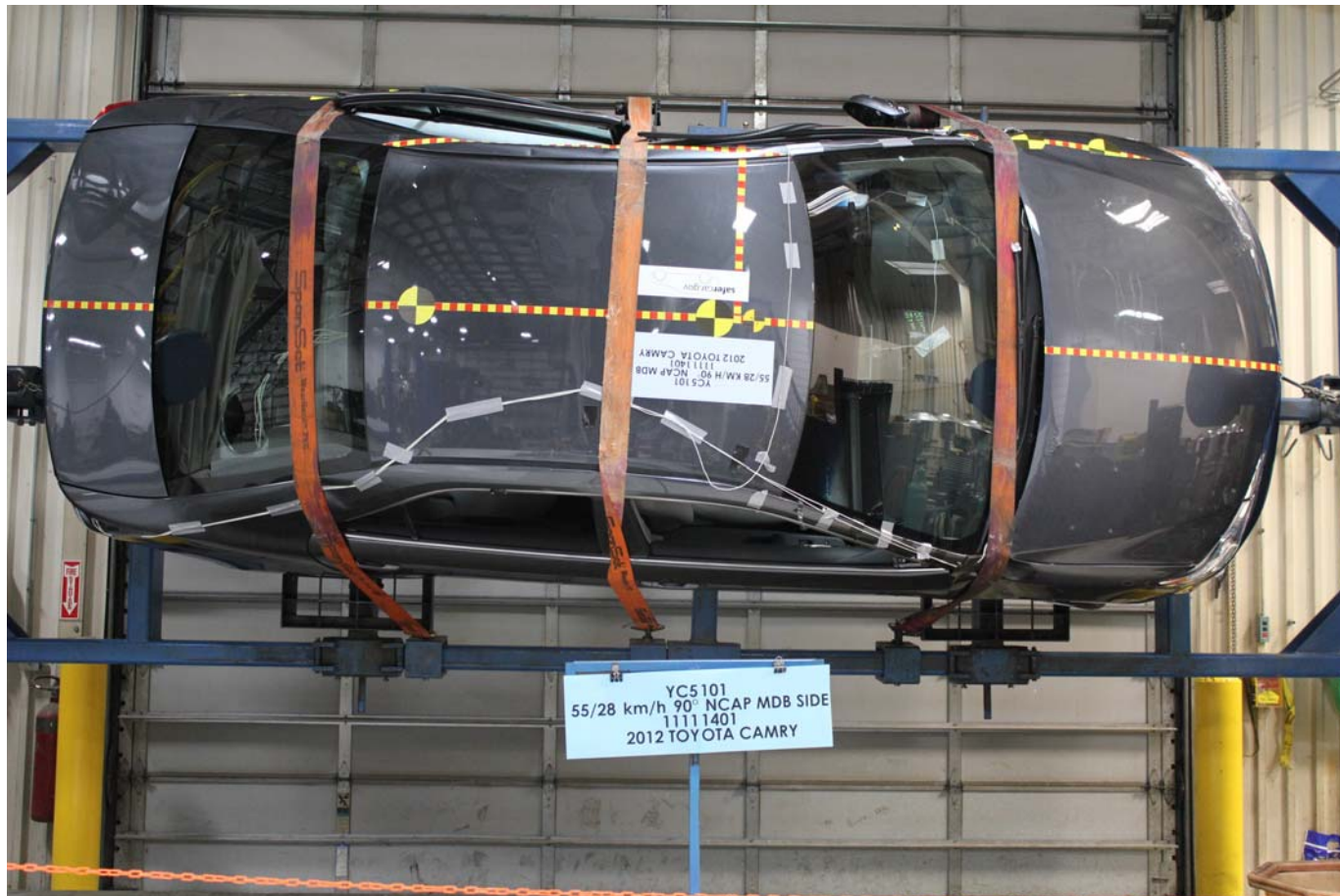
FMVSS No. 301 Static Rollover 270 Degrees
