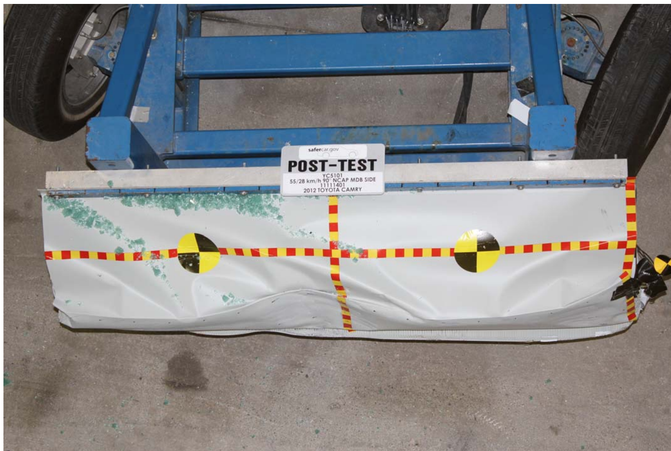
Post-Test Top View of MDB Impactor Face
