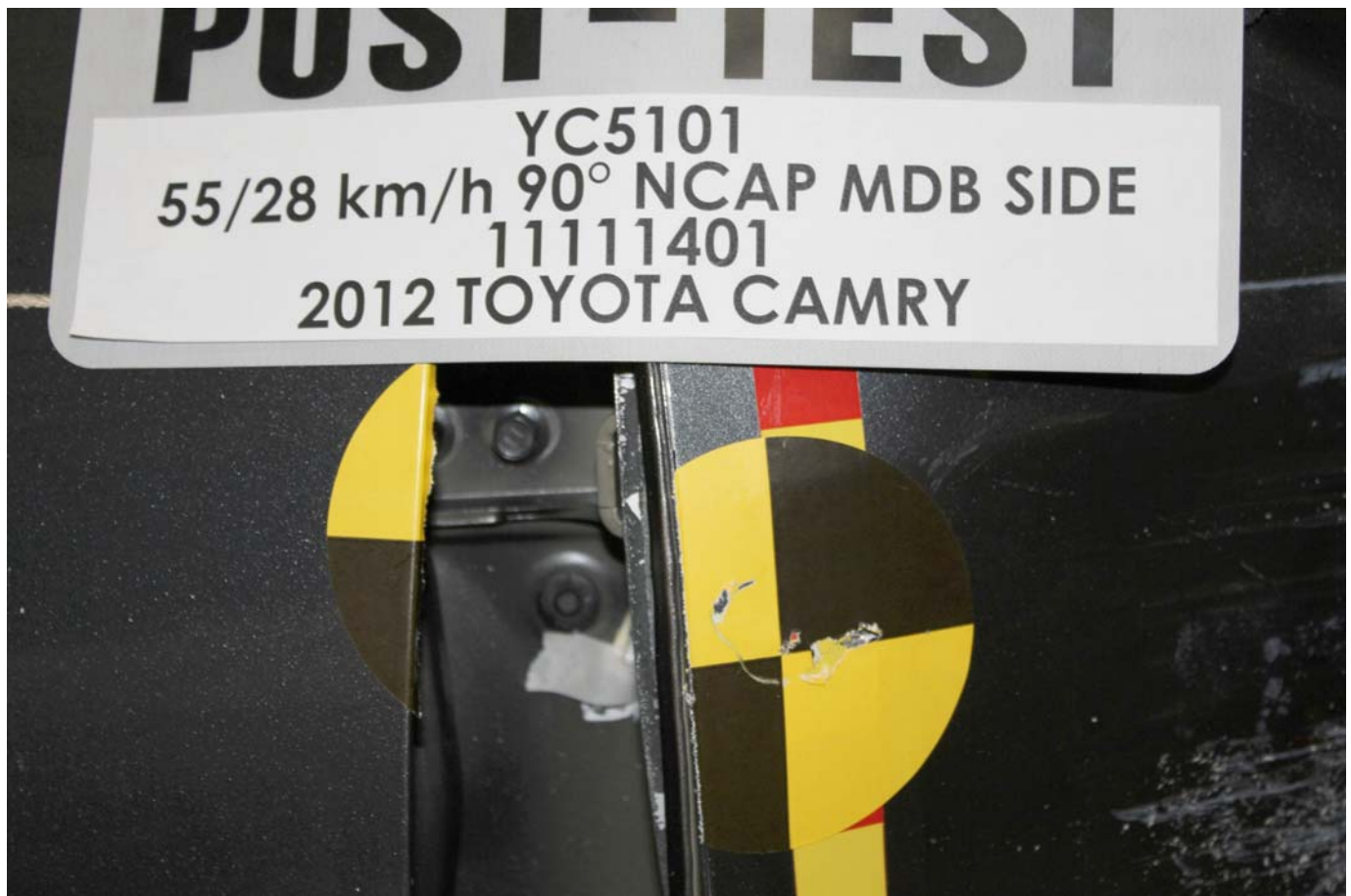
Post-Test Close-Up View of Impact Point Target
