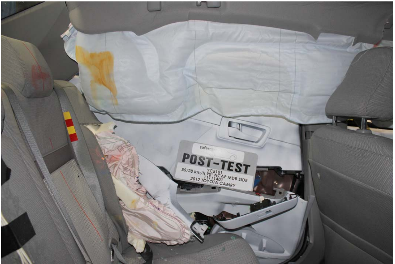
Post-Test Rear Passenger Inner Door Panel View
