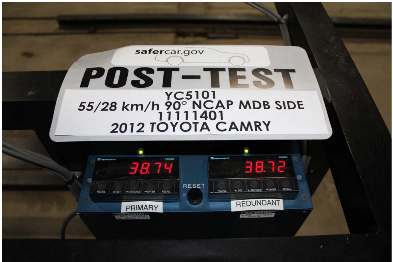
Post-Test Primary and Redundant Speed Trap Read-Out
