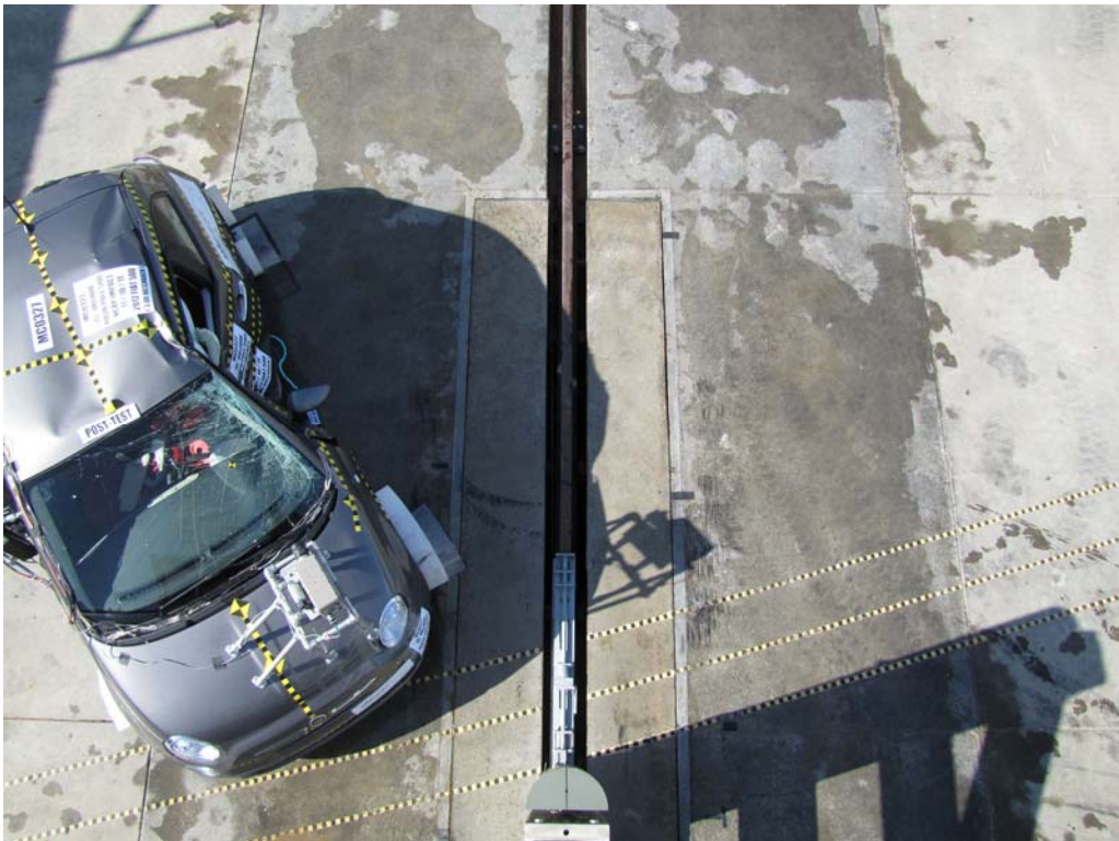
FIGURE 16. Post-Test Overhead View of Test Vehicle and Pole
