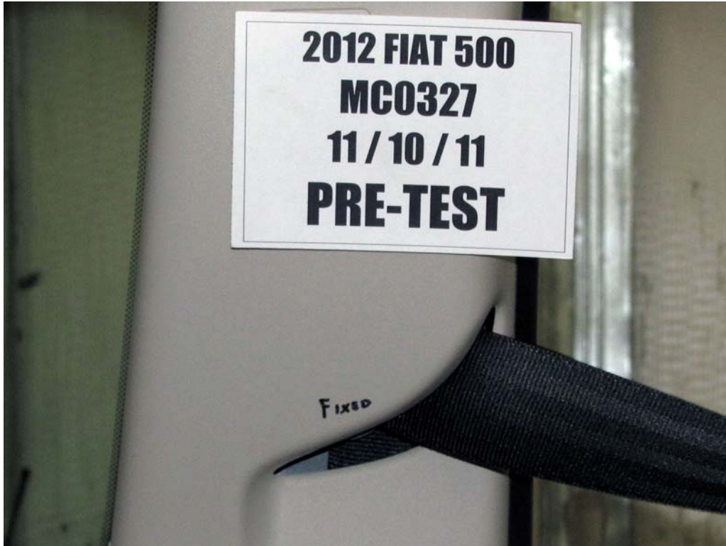
FIGURE 33. Pre-Test View of Belt Anchorage for Dummy
