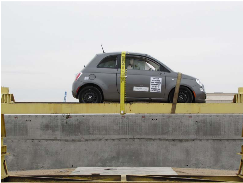
FIGURE 62. FMVSS No. 301-305 Rollover 0 Degrees
