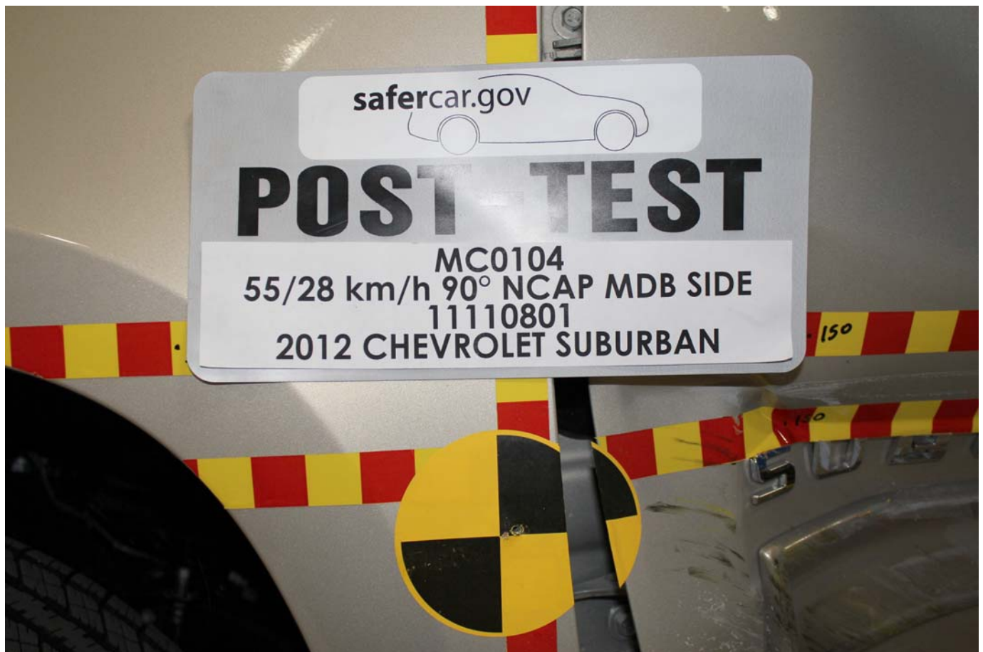
Post-Test Close-Up View of Impact Point Target
