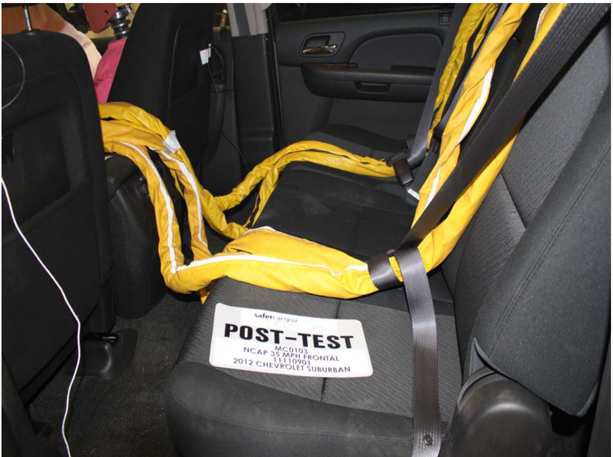
Post-Test Dummy Cable Routing
