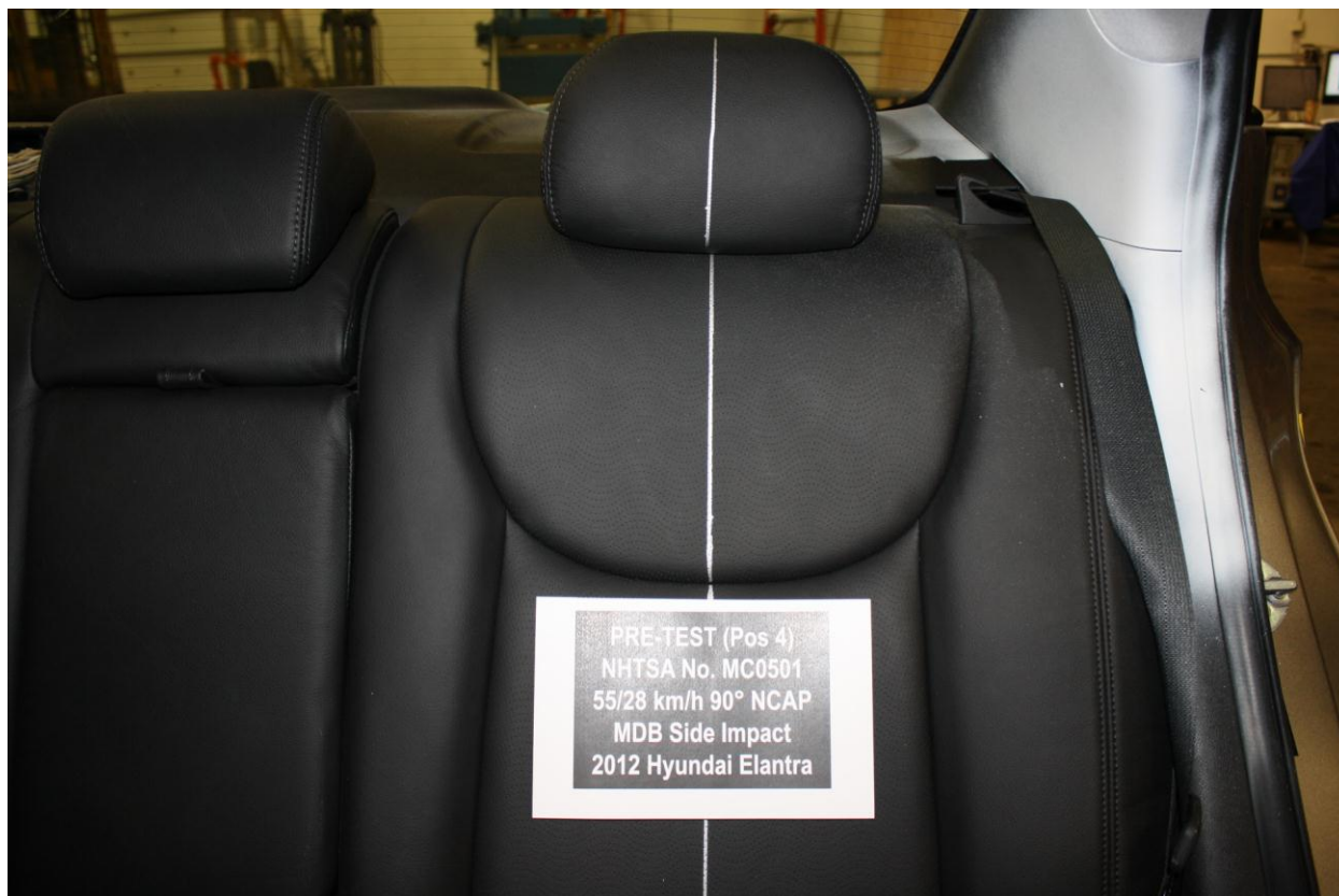
Figure A-57: Pre-Test Frontal View of Rear Passenger Seat Back Prior to Dummy Positioning
