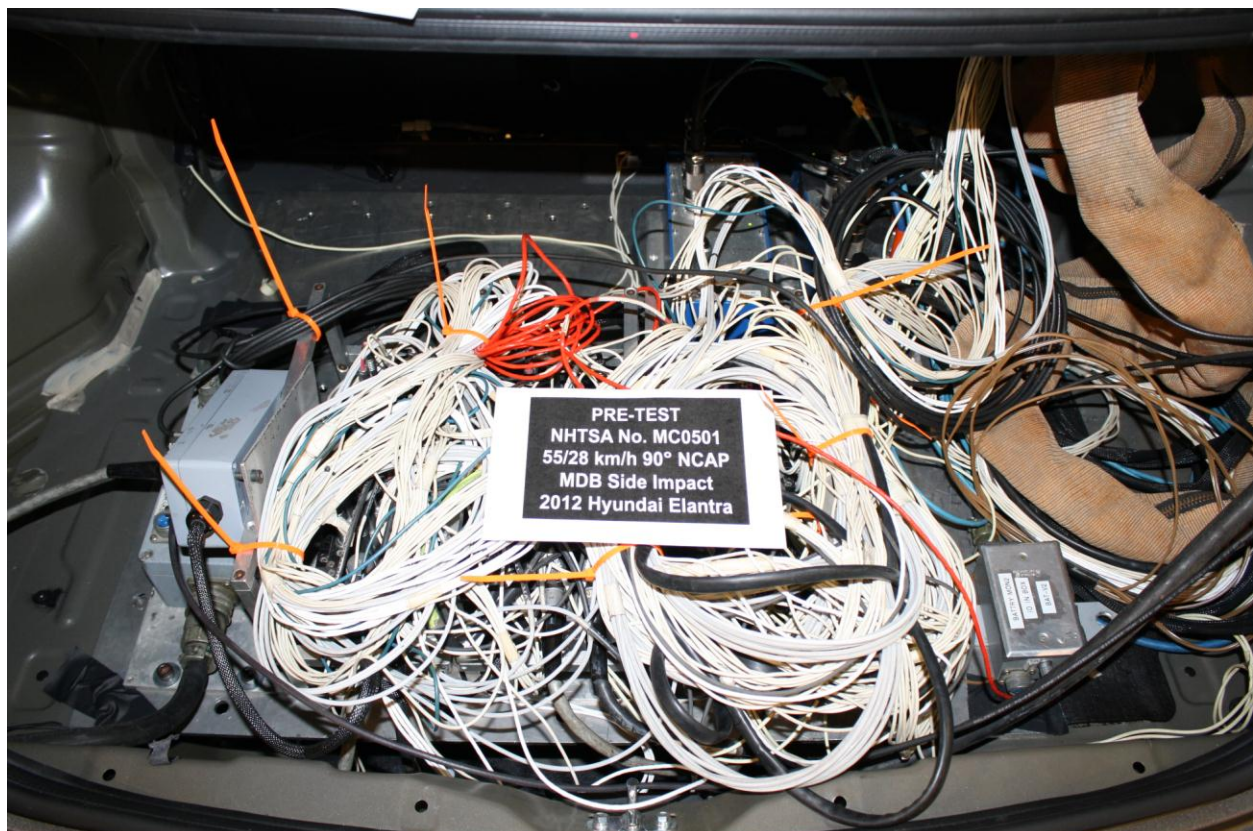
Figure A-92: Pre-Test Ballast View
