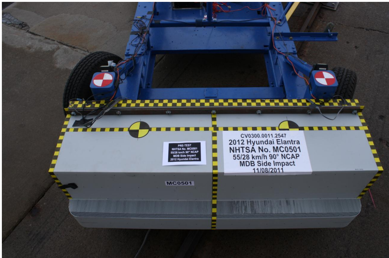
Figure A-84: Pre-Test Top View of MDB Impactor Face
