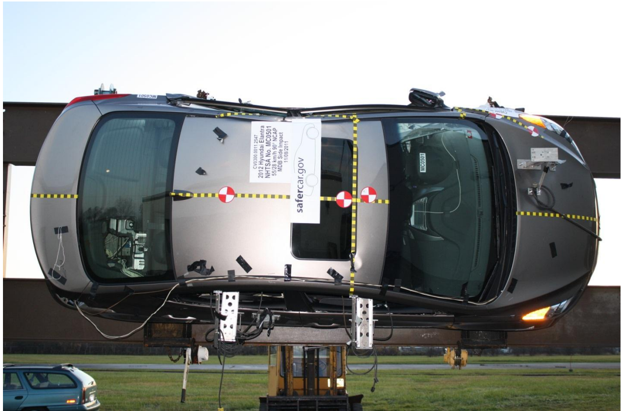
Figure A-97: FMVSS No. 301 Static Rollover 270 Degrees
