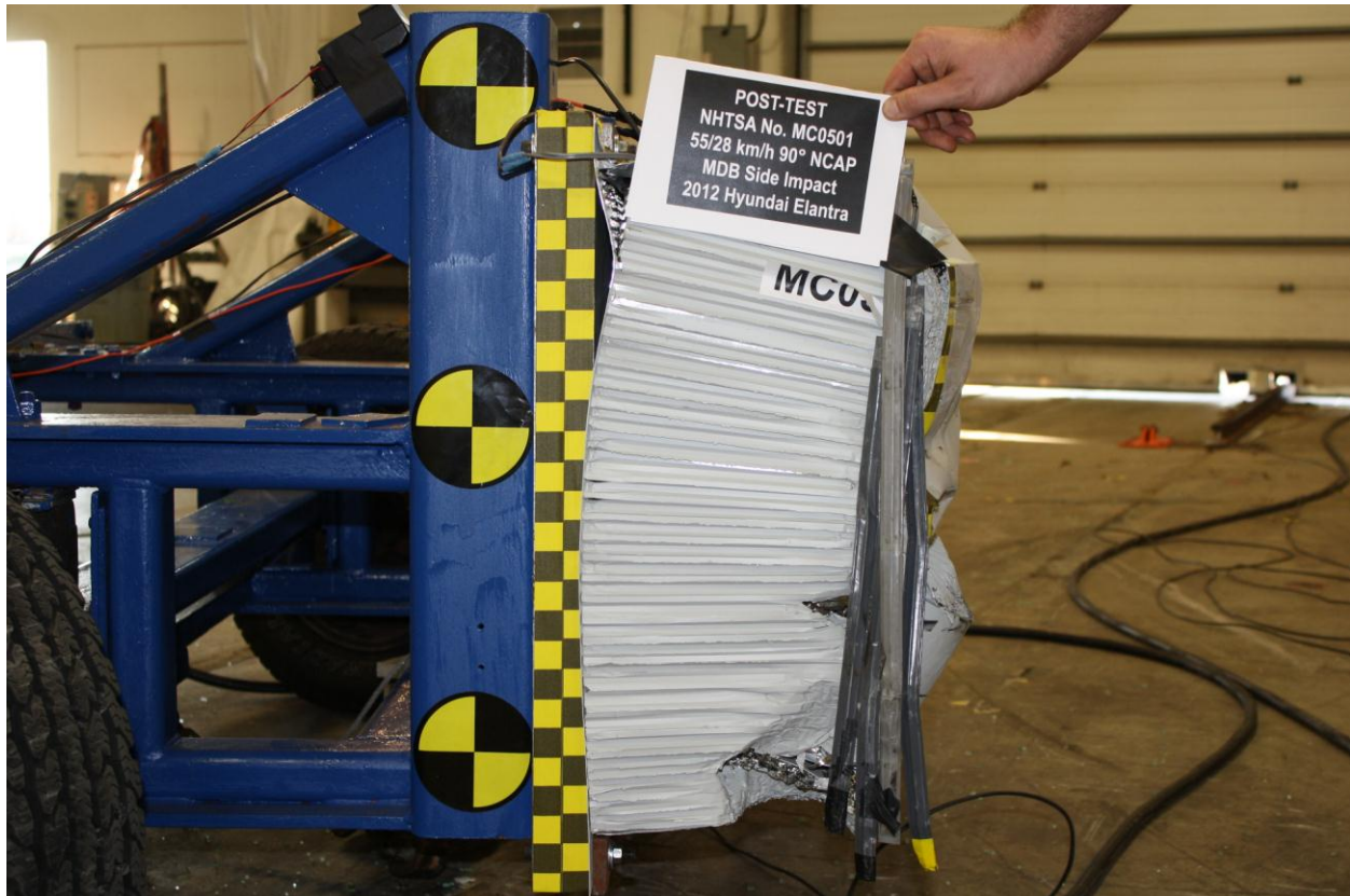
Figure A-89: Post-Test Right Side View of MDB Impactor Face
