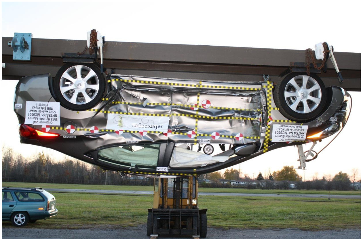
Figure A-96: FMVSS No. 301 Static Rollover 180 Degrees
