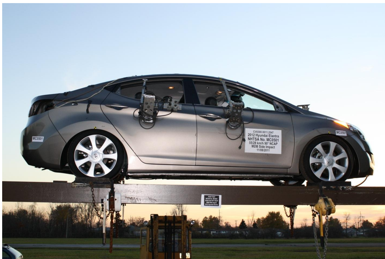
Figure A-94: FMVSS No. 301 Static Rollover 0 Degrees
