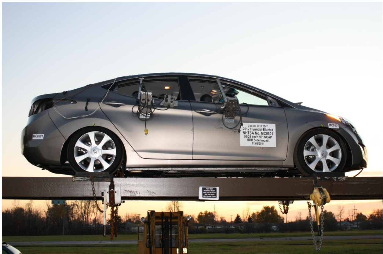
Figure A-98: FMVSS No. 301 Static Rollover 360 Degrees
