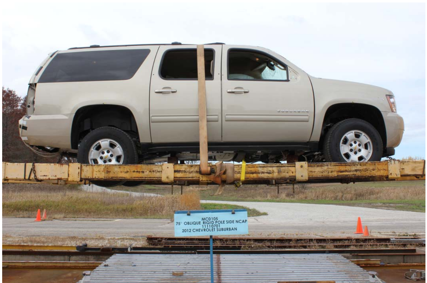
FMVSS No. 301 Static Rollover 0 Degrees
