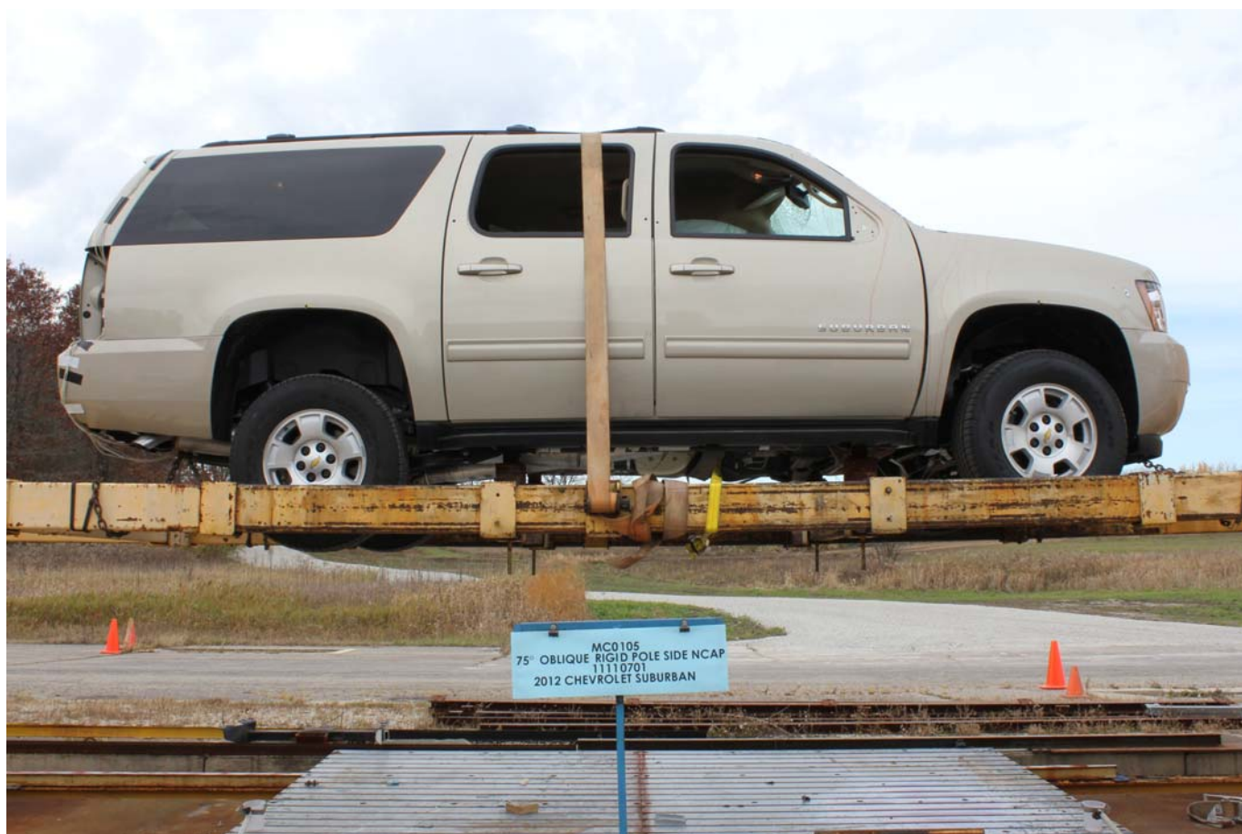
FMVSS No. 301 Static Rollover 360 Degrees
