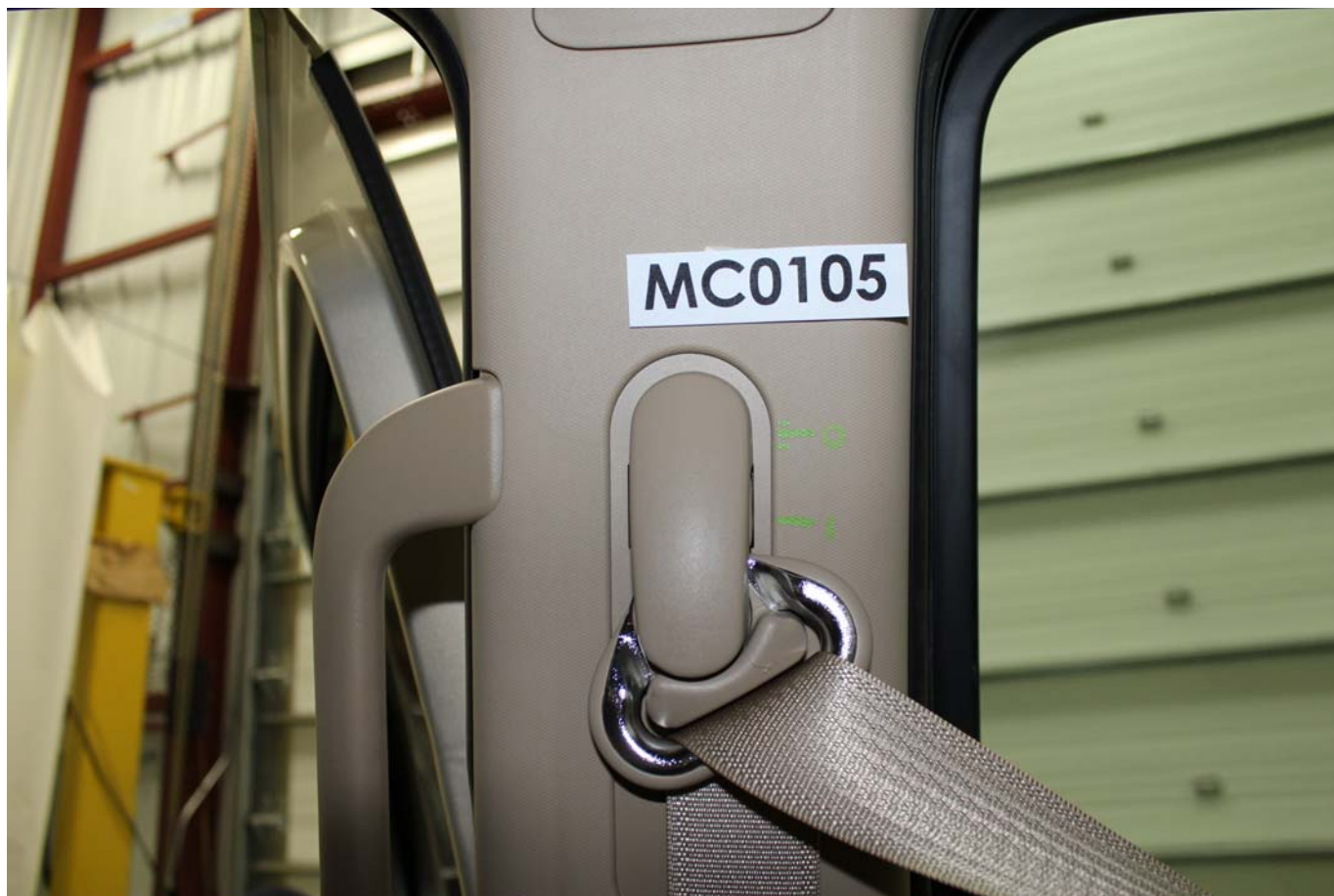
Pre-Test View of Belt Anchorage for Dummy
