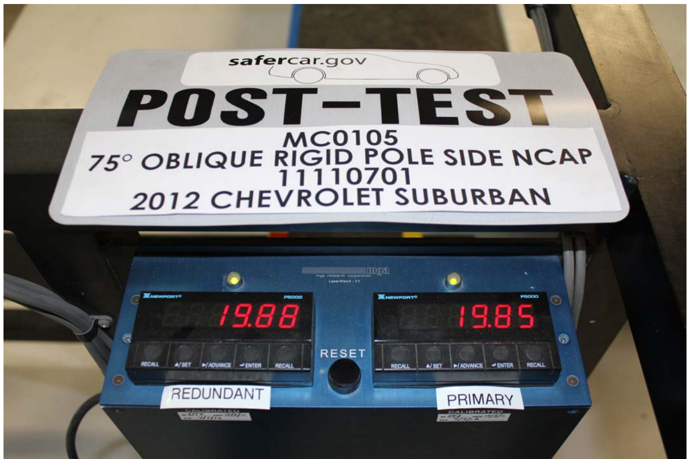
Post-Test Primary and Redundant Speed Trap Read-Out
