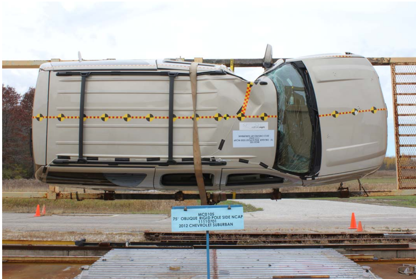
FMVSS No. 301 Static Rollover 270 Degrees
