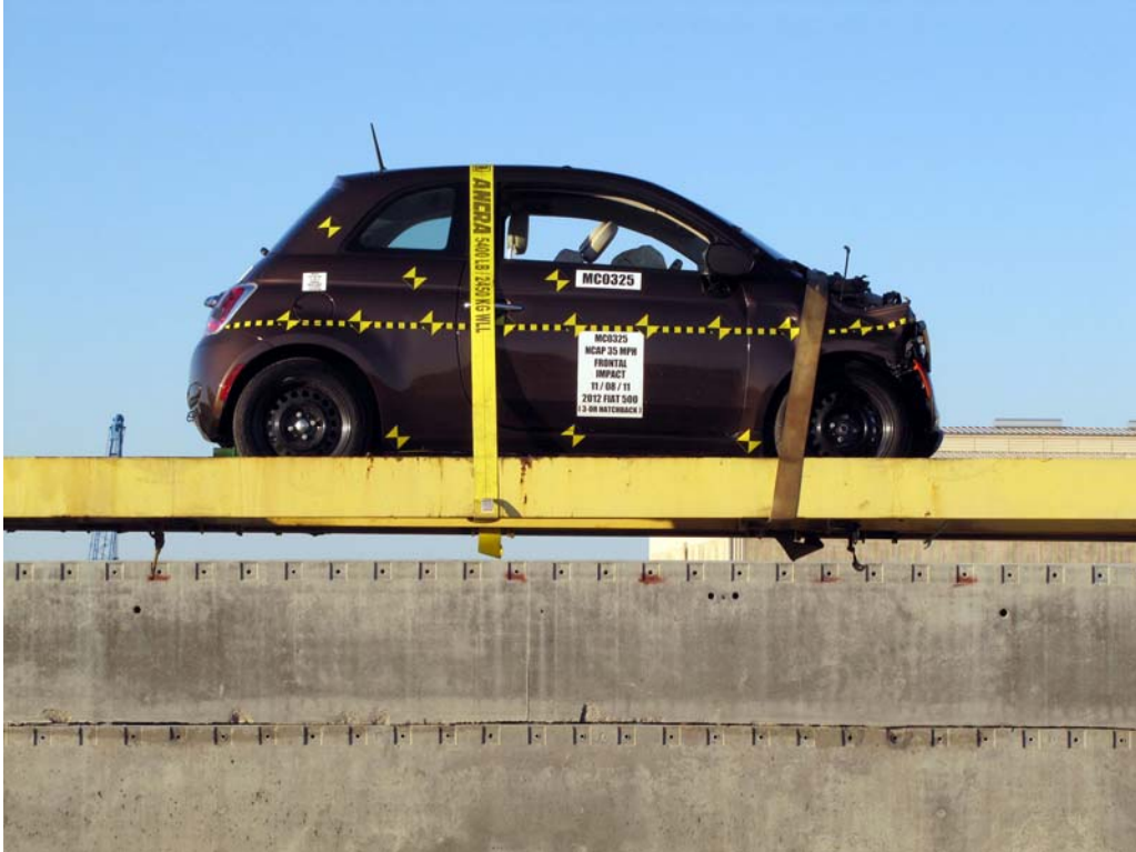
FIGURE 70. Vehicle at 360° on Static Rollover Device
