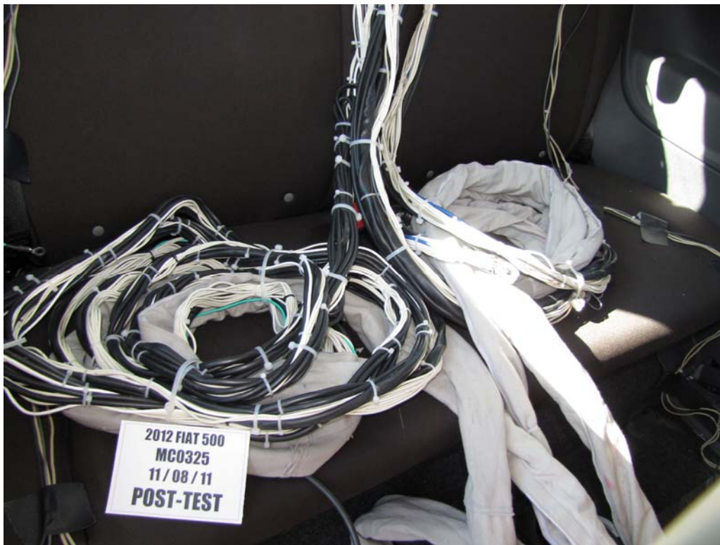
FIGURE 28. Post-Test Dummy Cable Routing
