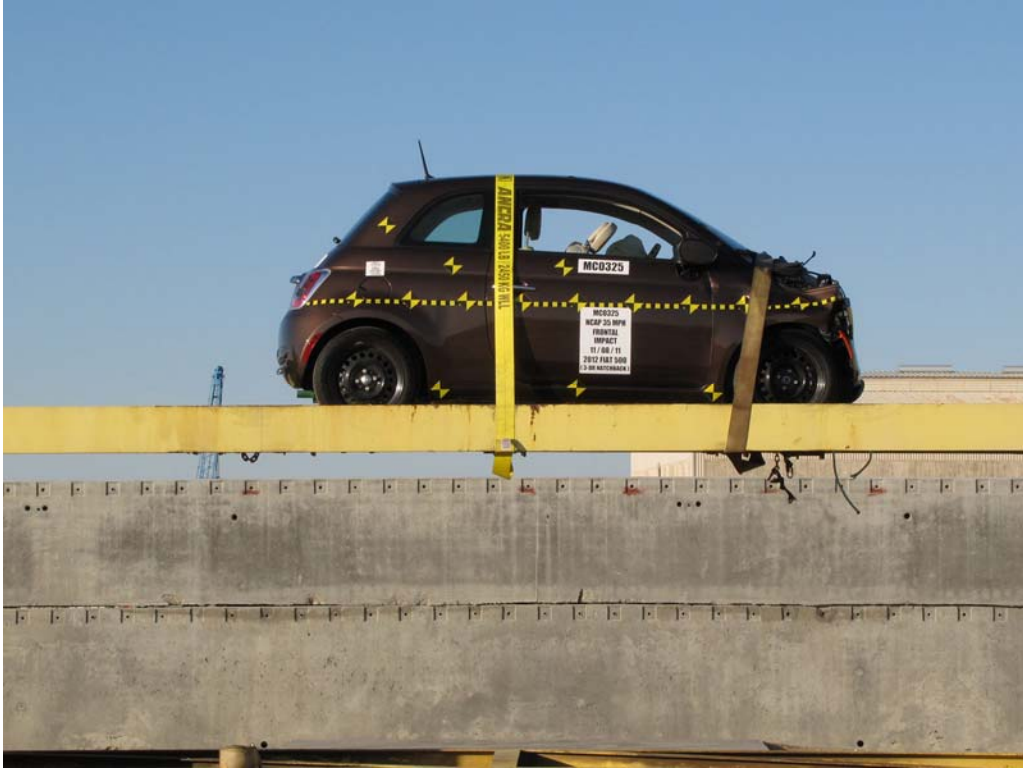
FIGURE 66. Vehicle at 0°on Static Rollover Device
