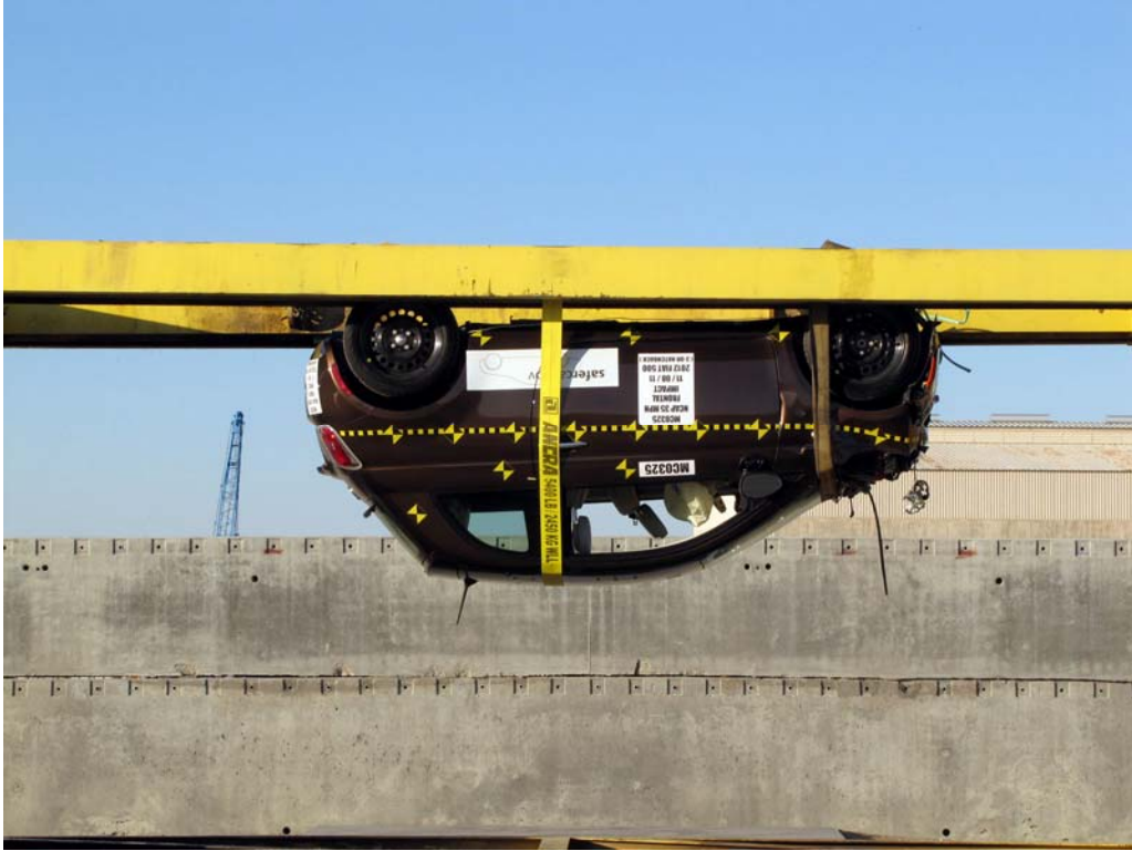
FIGURE 68. Vehicle at 180° on Static Rollover Device
