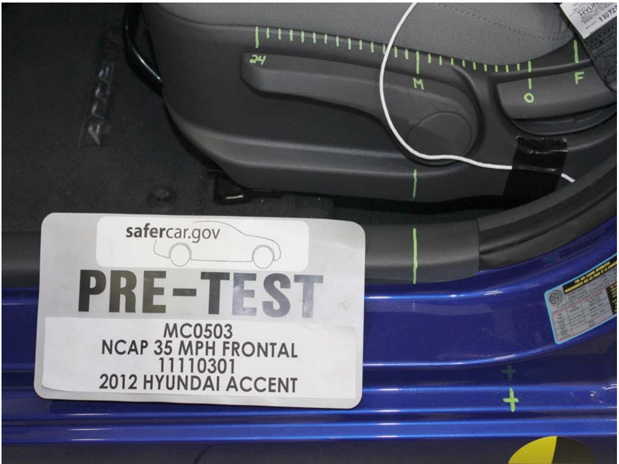
Pre-Test Driver's Seat Fore-Aft Markings
