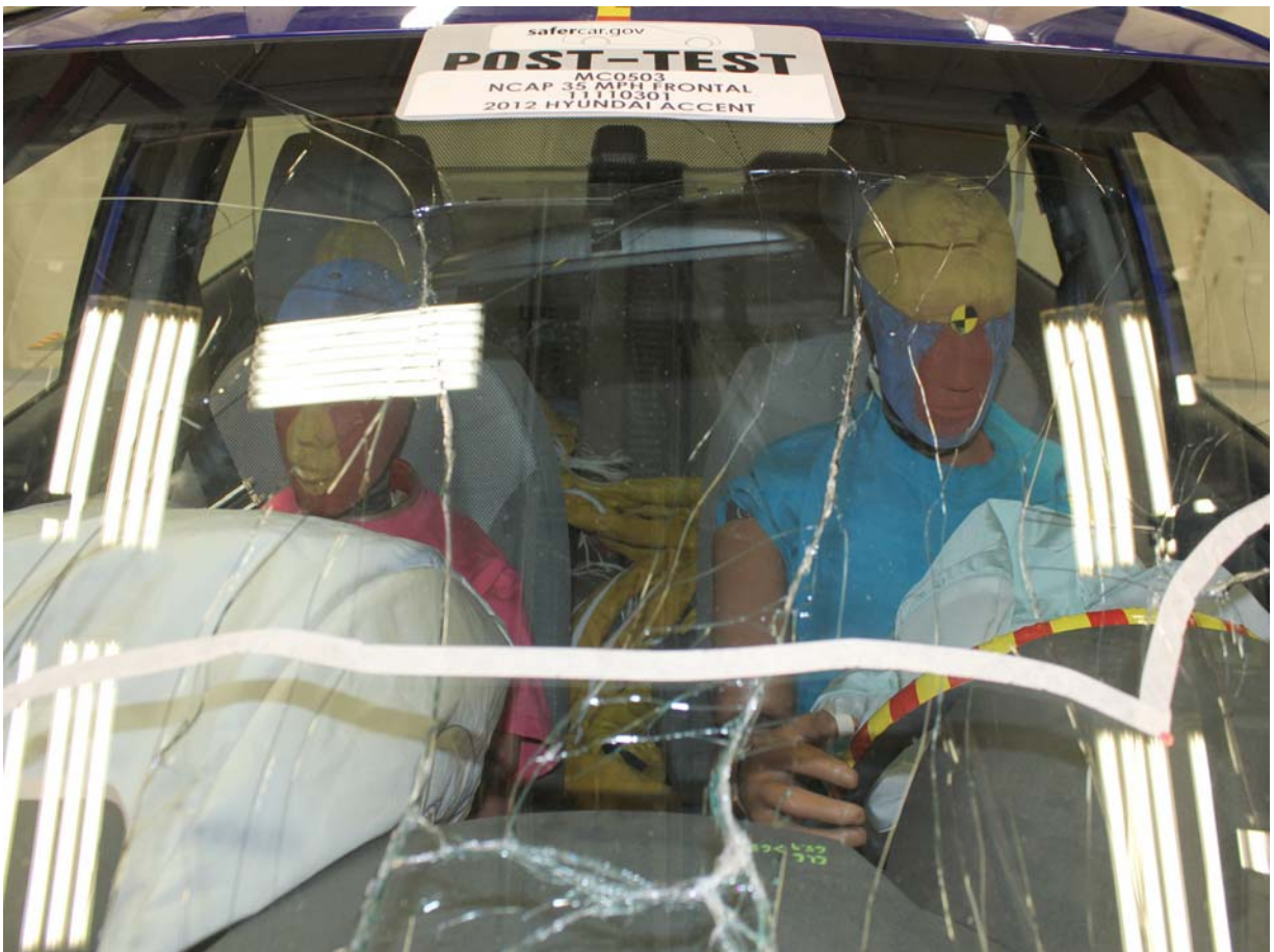
Post-Test Windshield View
