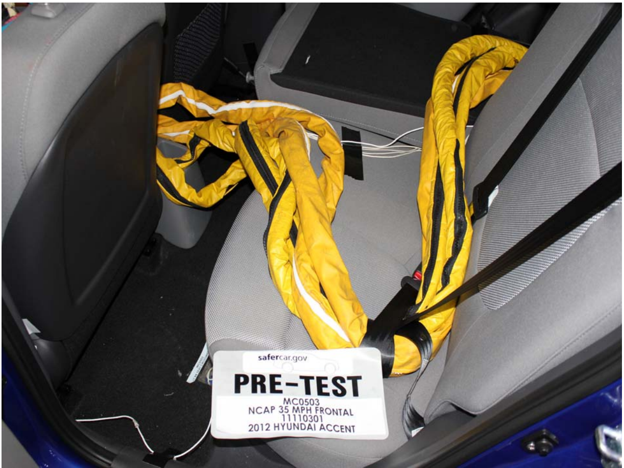
Pre-Test Dummy Cable Routing
