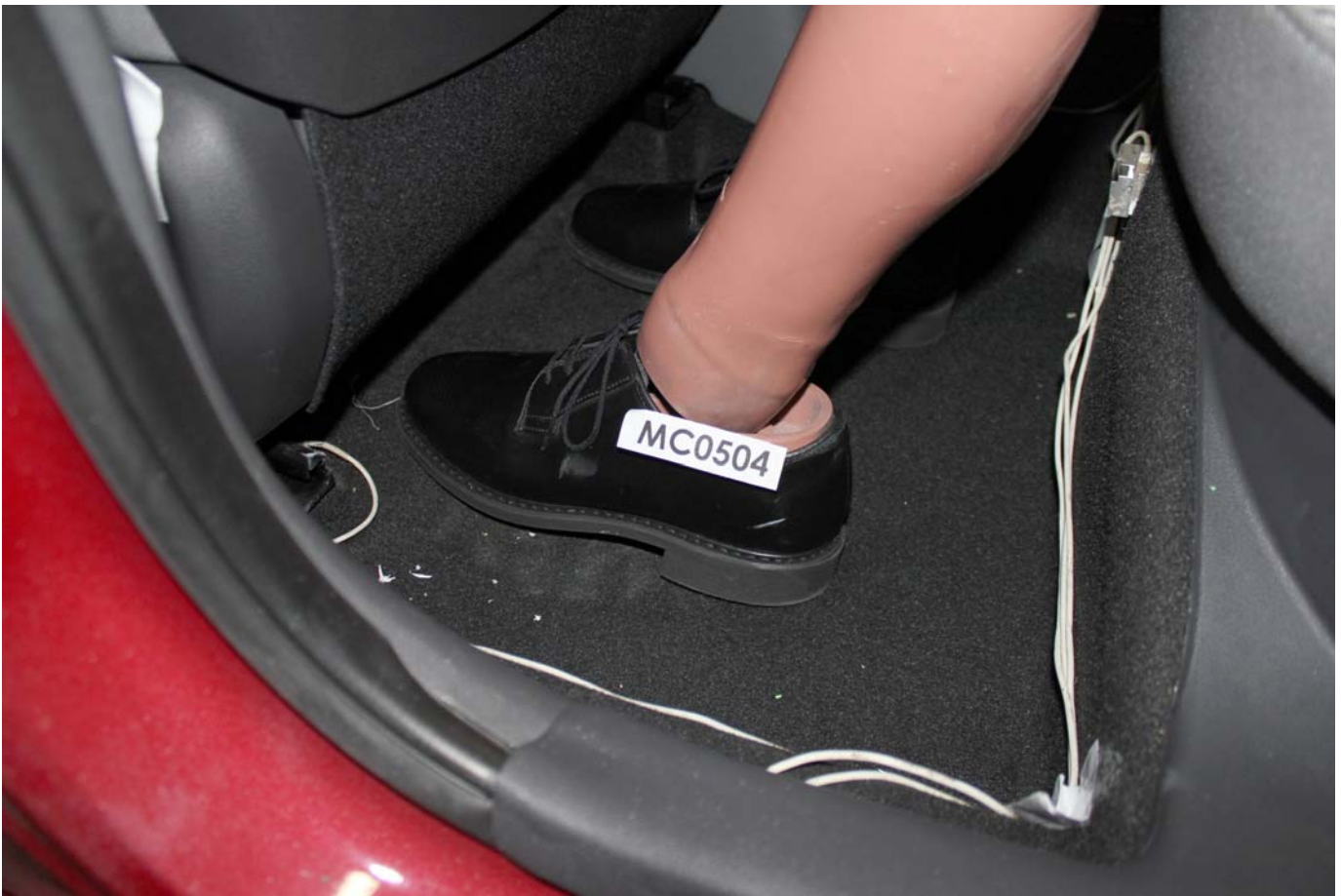
Pre-Test Placement of Rear Passenger Dummy's Feet
