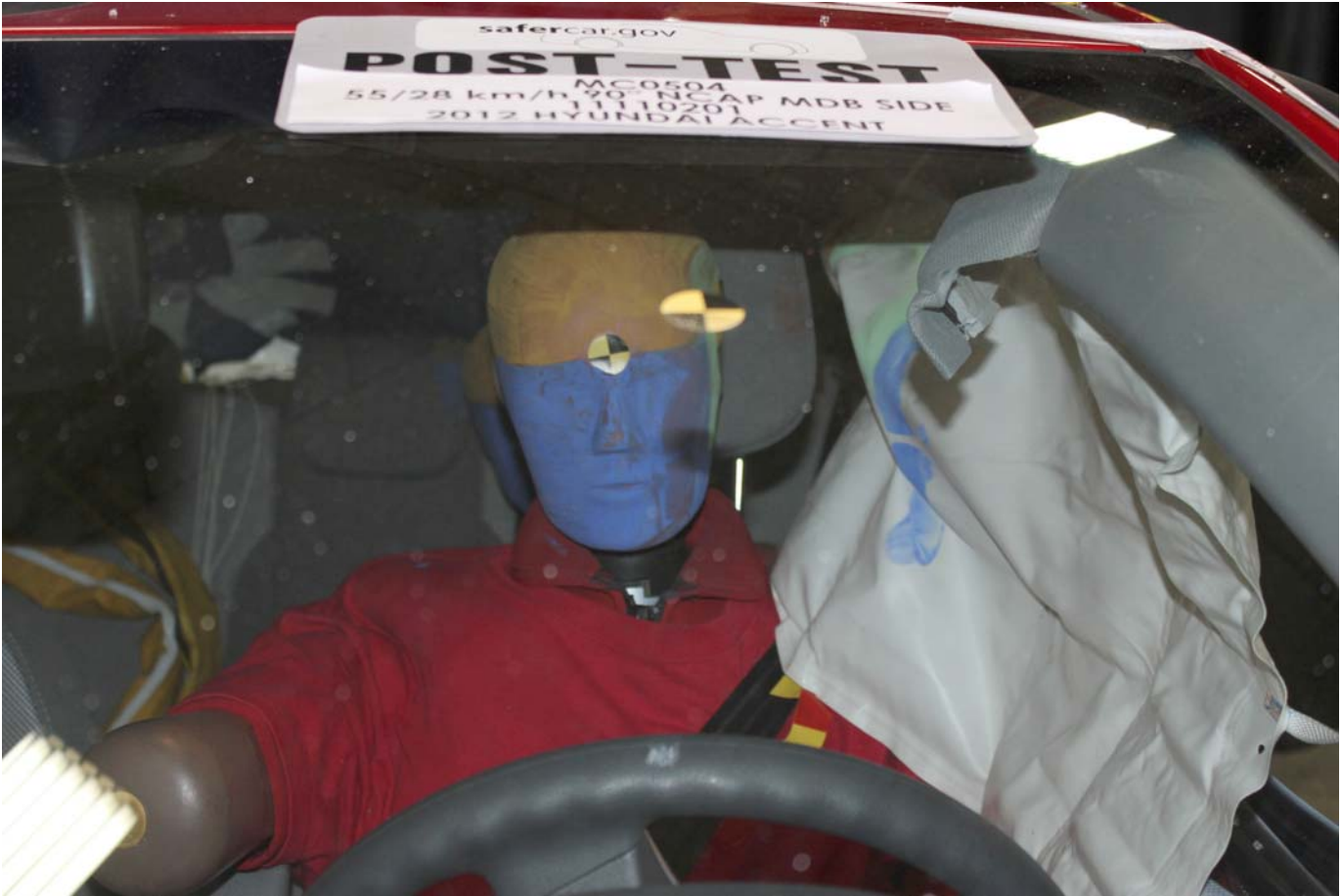
Post-Test Front Close-Up View of Driver Dummy
