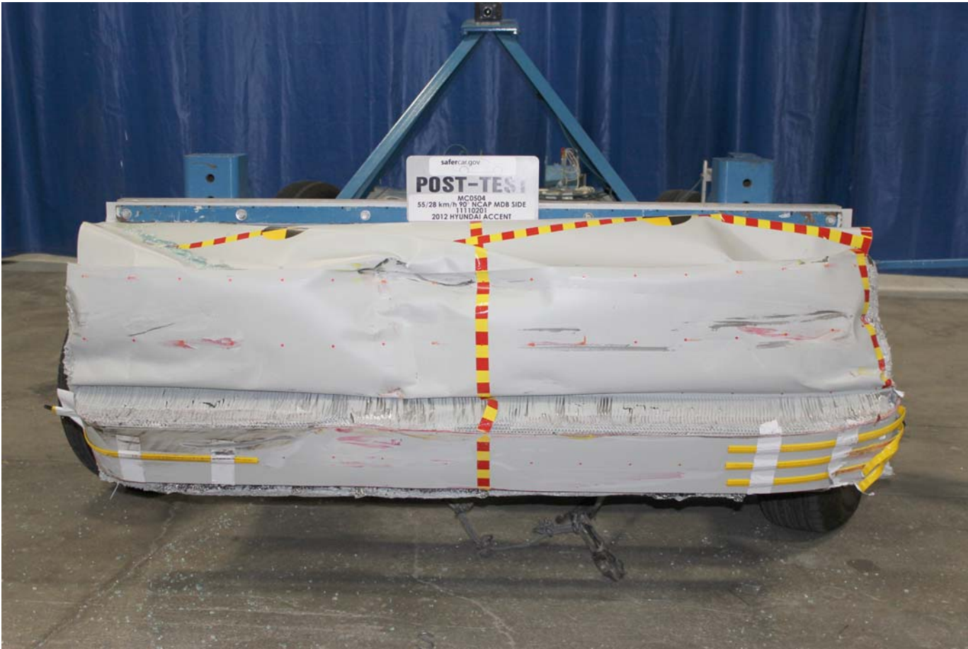
Post-Test Front View of MDB Impactor Face
