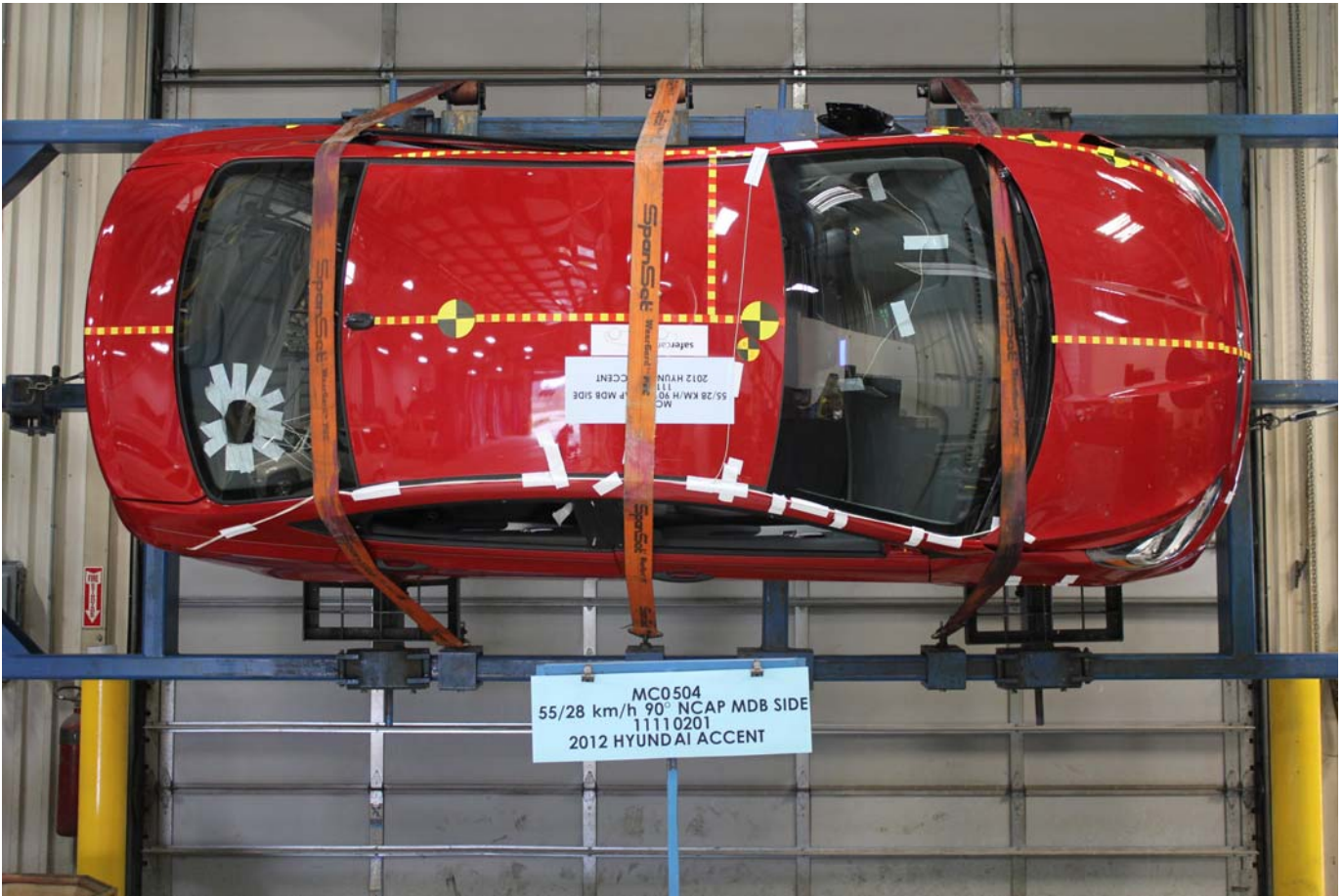
FMVSS No. 301 Static Rollover 270 Degrees
