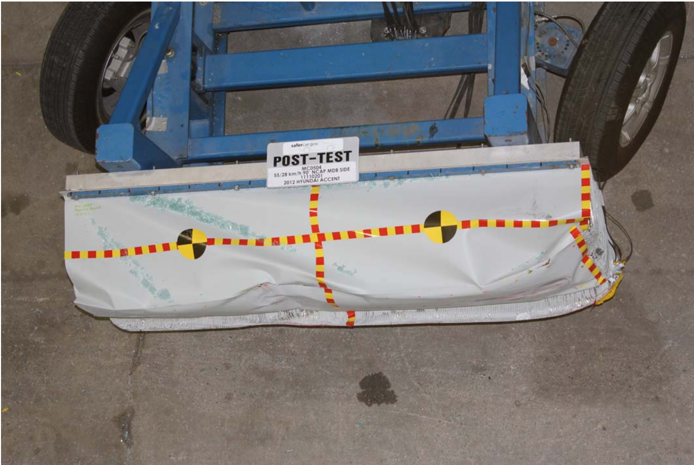
Post-Test Top View of MDB Impactor Face
