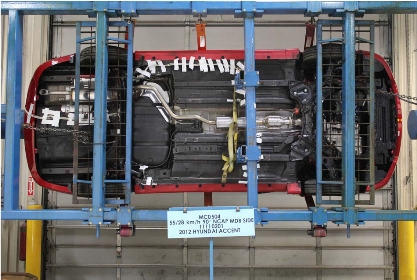
FMVSS No. 301 Static Rollover 90 Degrees
