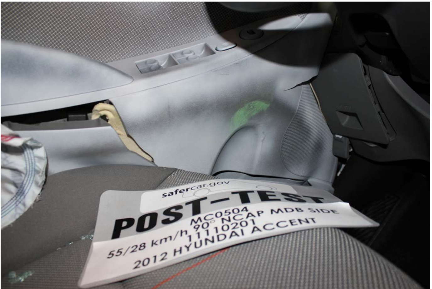
Post-Test Driver Dummy Close-up Knee Contact with Vehicle Interior View
