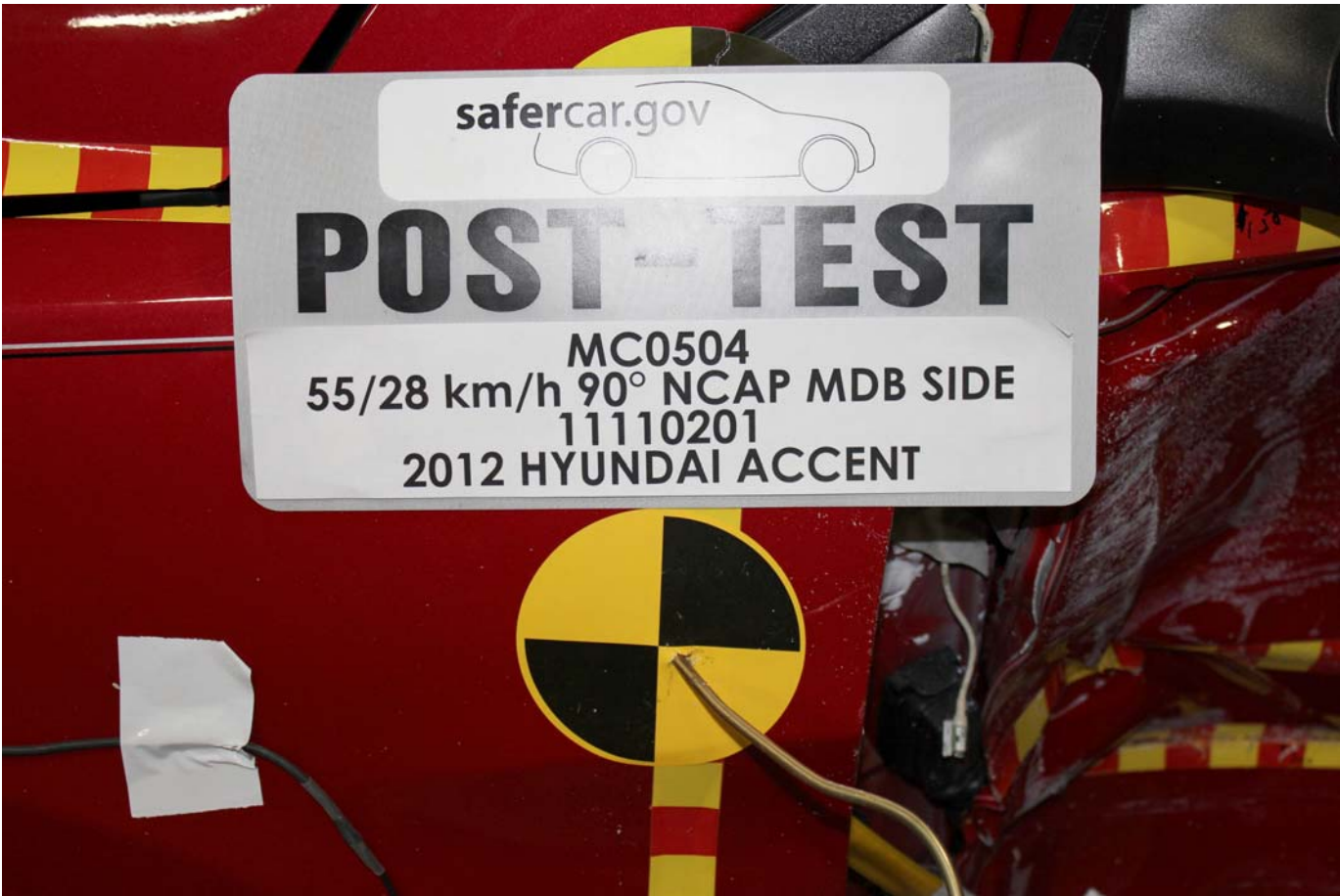
Post-Test Close-Up View of Impact Point Target
