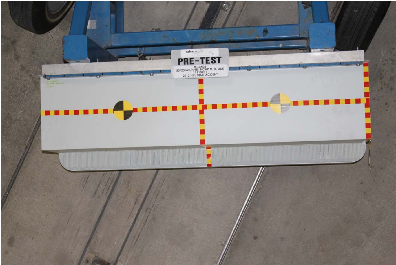
Pre-Test Top View of MDB Impactor Face
