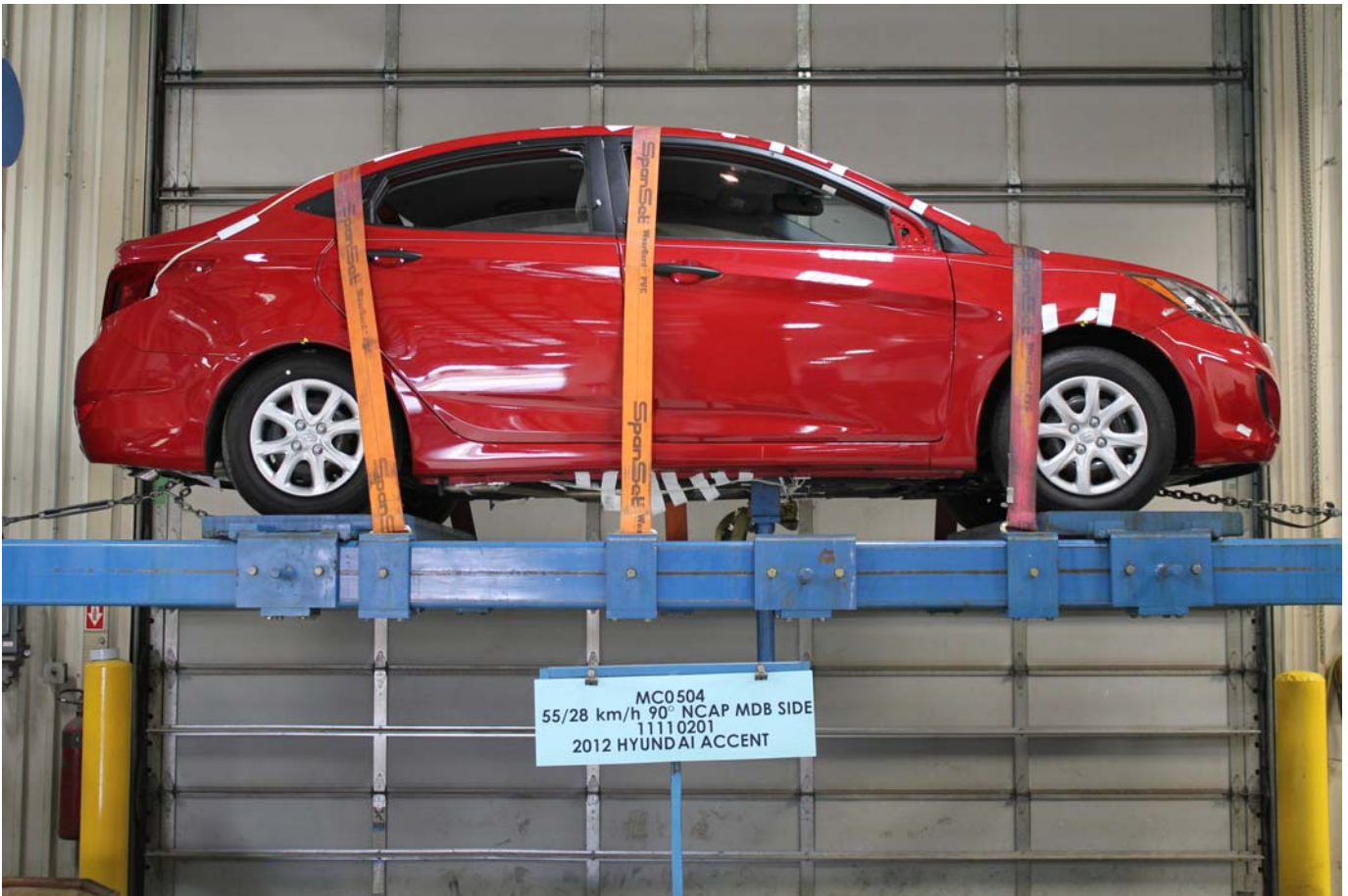
FMVSS No. 301 Static Rollover 360 Degrees
