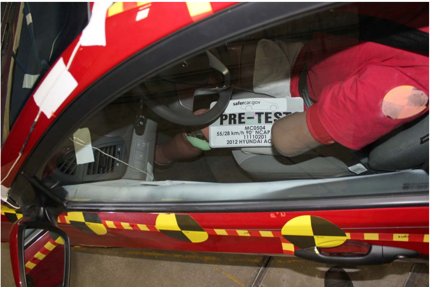
Pre-Test Driver Dummy and Door Clearance View
