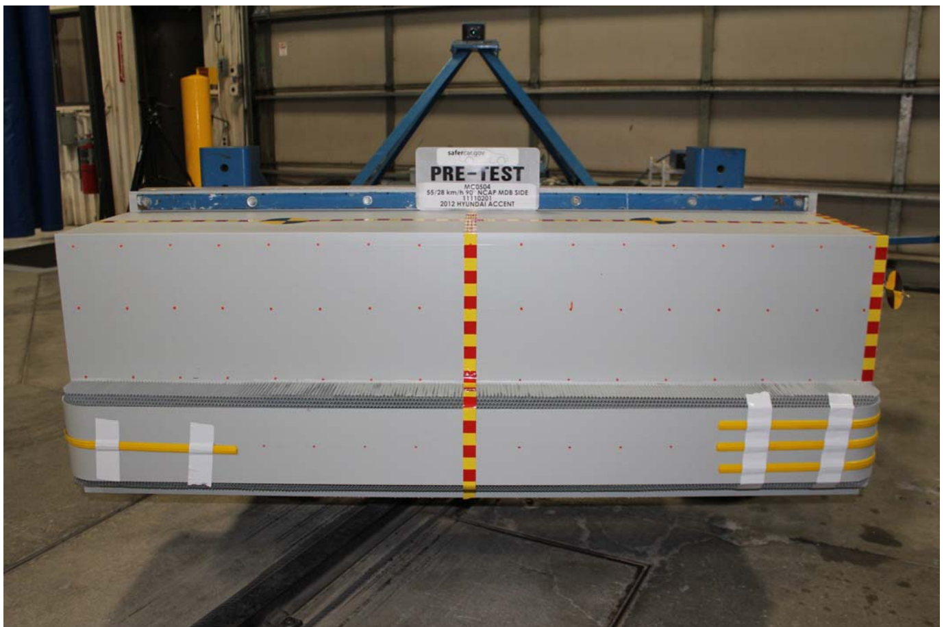
Pre-Test Front View of MDB Impactor Face
