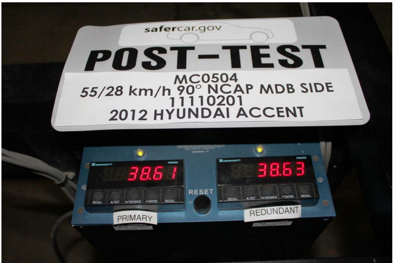
Post-Test Primary and Redundant Speed Trap Read-Out
