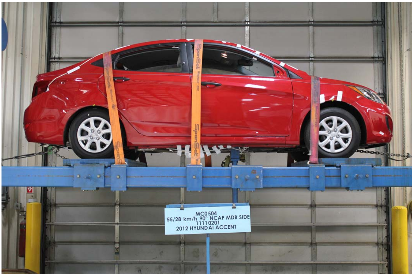
FMVSS No. 301 Static Rollover 0 Degrees
