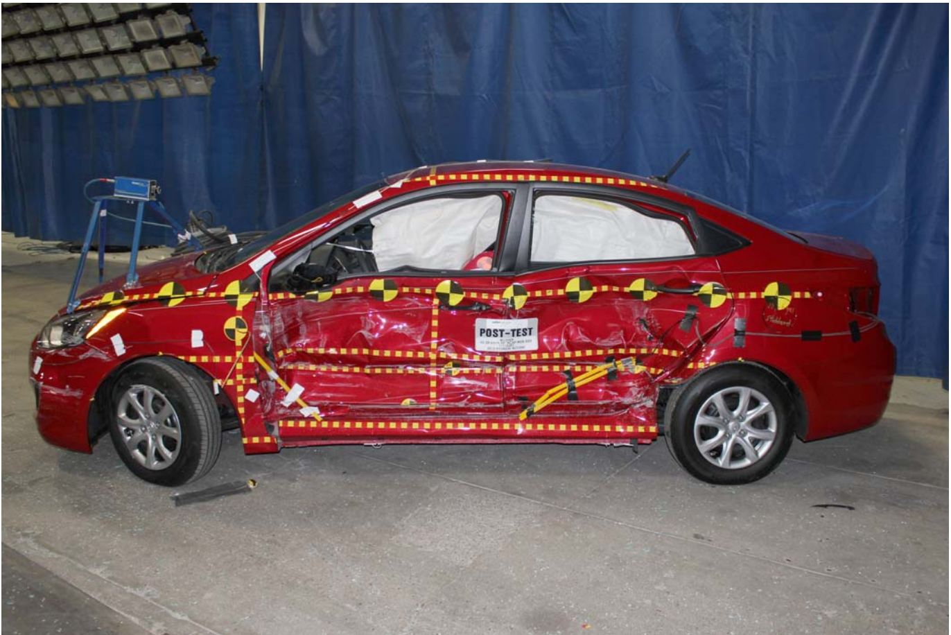
Post-Test Left Side View of Test Vehicle
