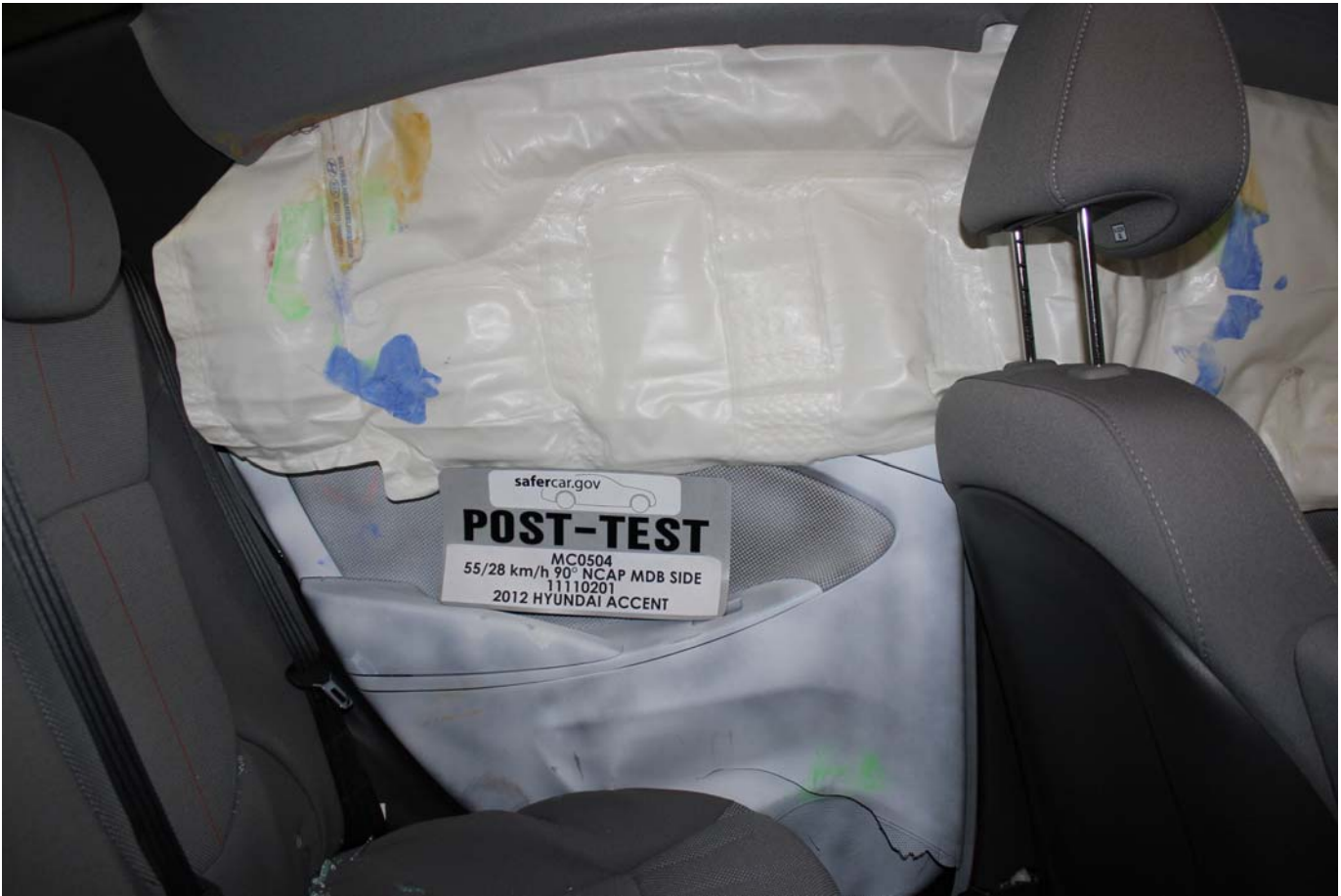
Post-Test Rear Passenger Inner Door Panel View
