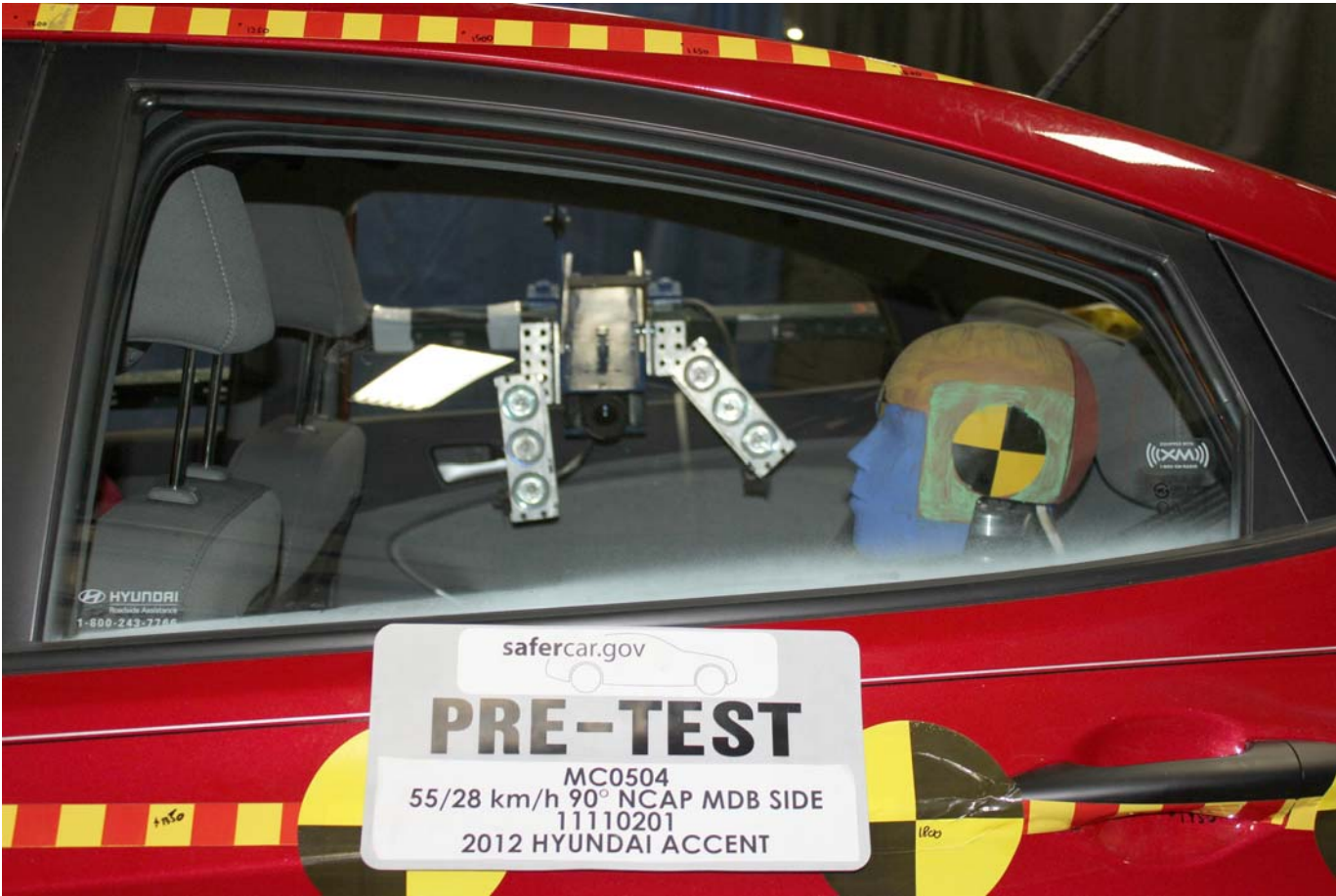
Pre-Test Left Side View of Rear Passenger Dummy Shoulder and Door Top View
