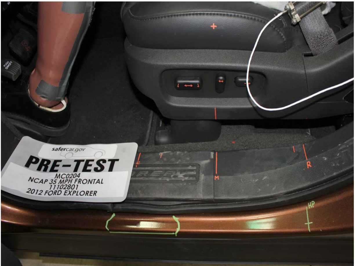
Pre-Test Driver's Seat Fore-Aft Markings
