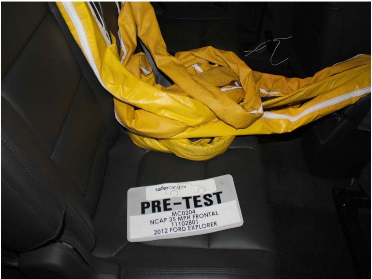
Pre-Test Dummy Cable Routing
