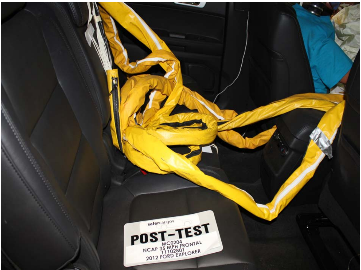
Post-Test Dummy Cable Routing
