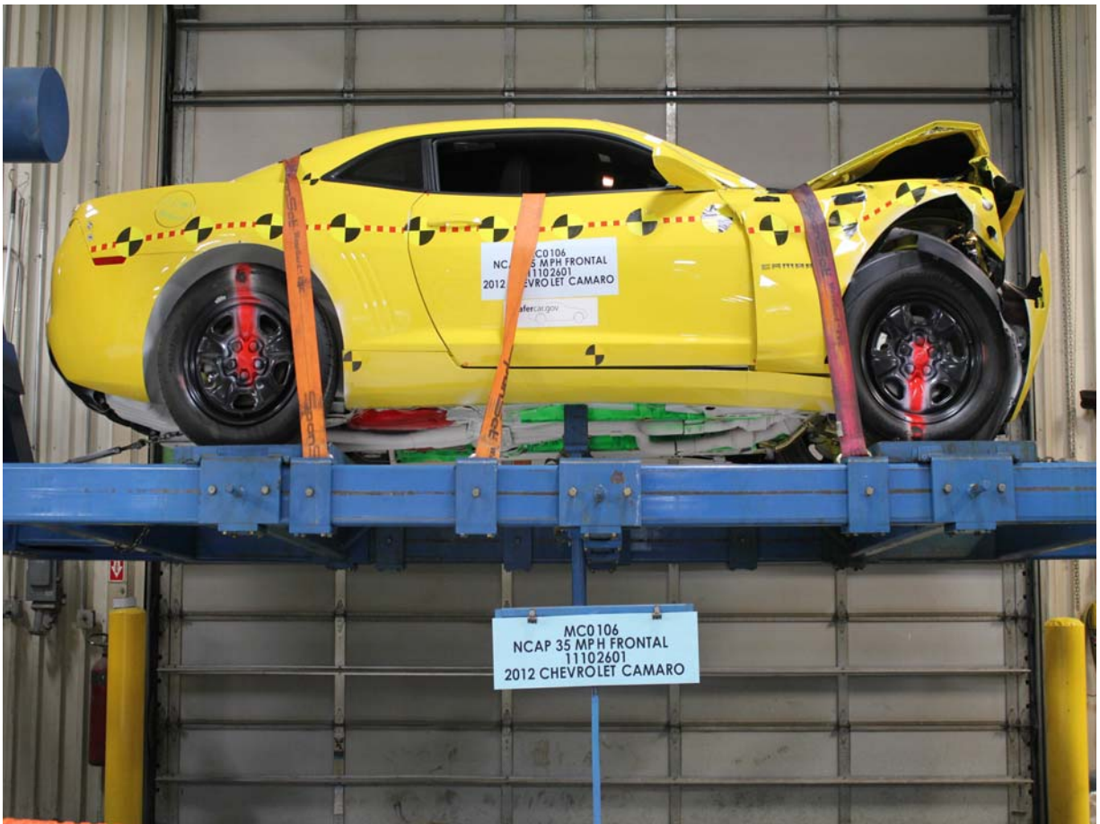
Vehicle at 0 Degrees on Static Rollover Device
