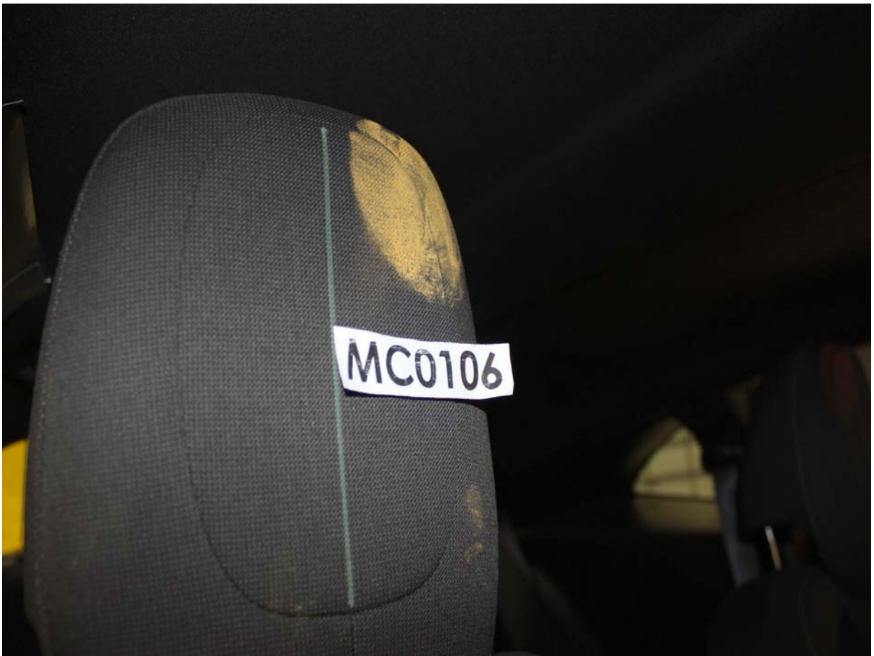
Post-Test Passenger Dummy Contact with Headrest
