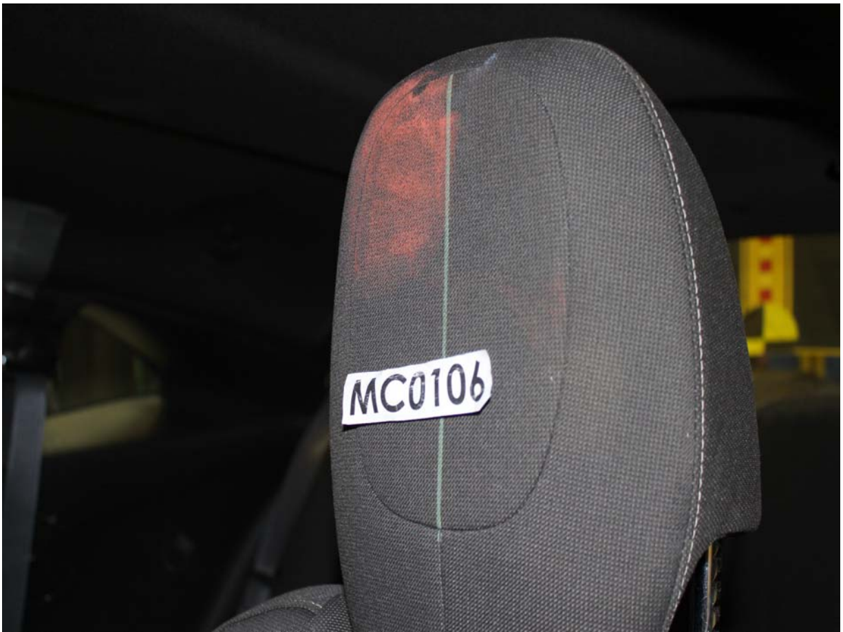
Post-Test Driver Dummy Contact with Headrest
