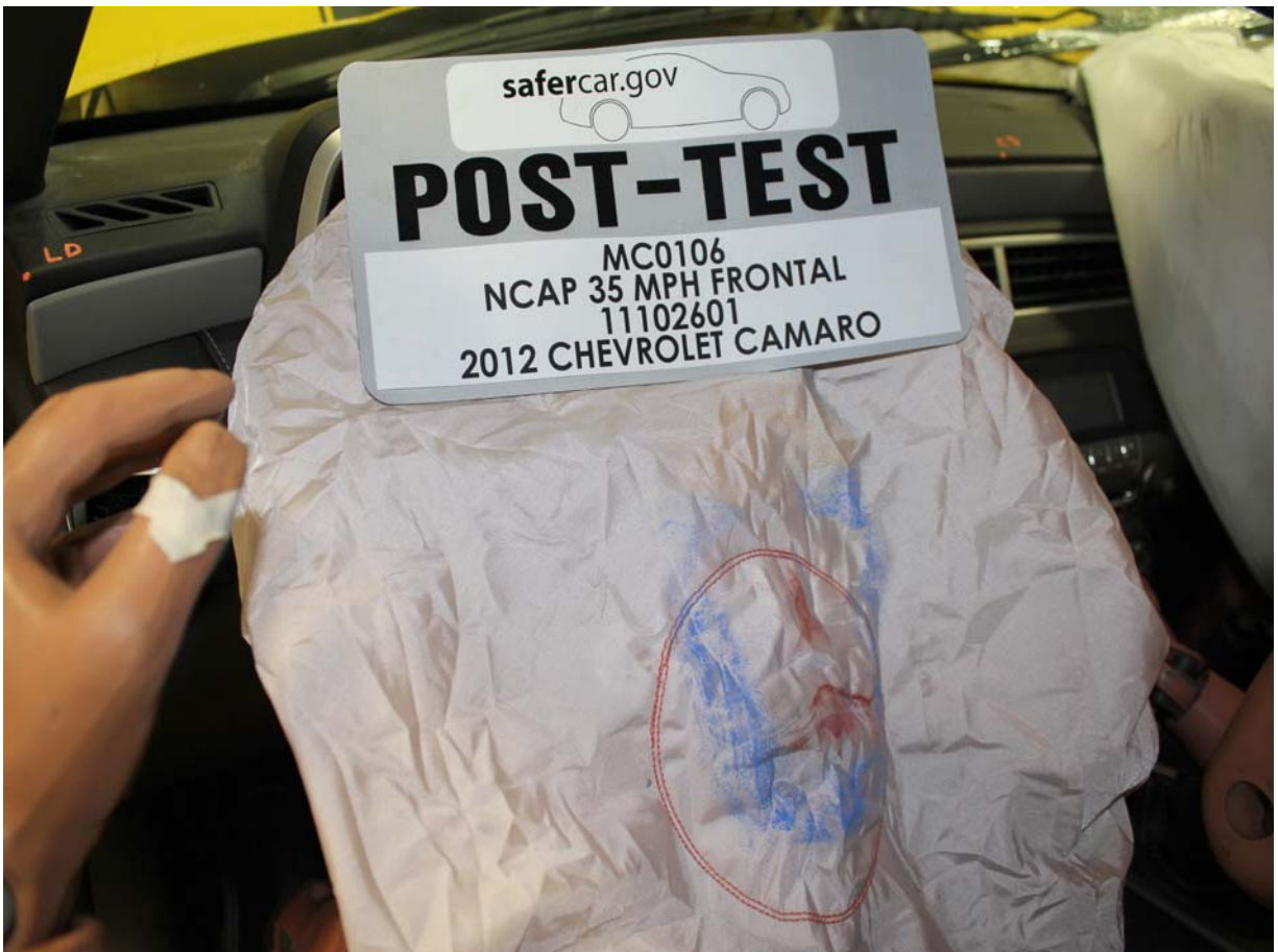
Post-Test Driver Dummy Contact with Airbag
