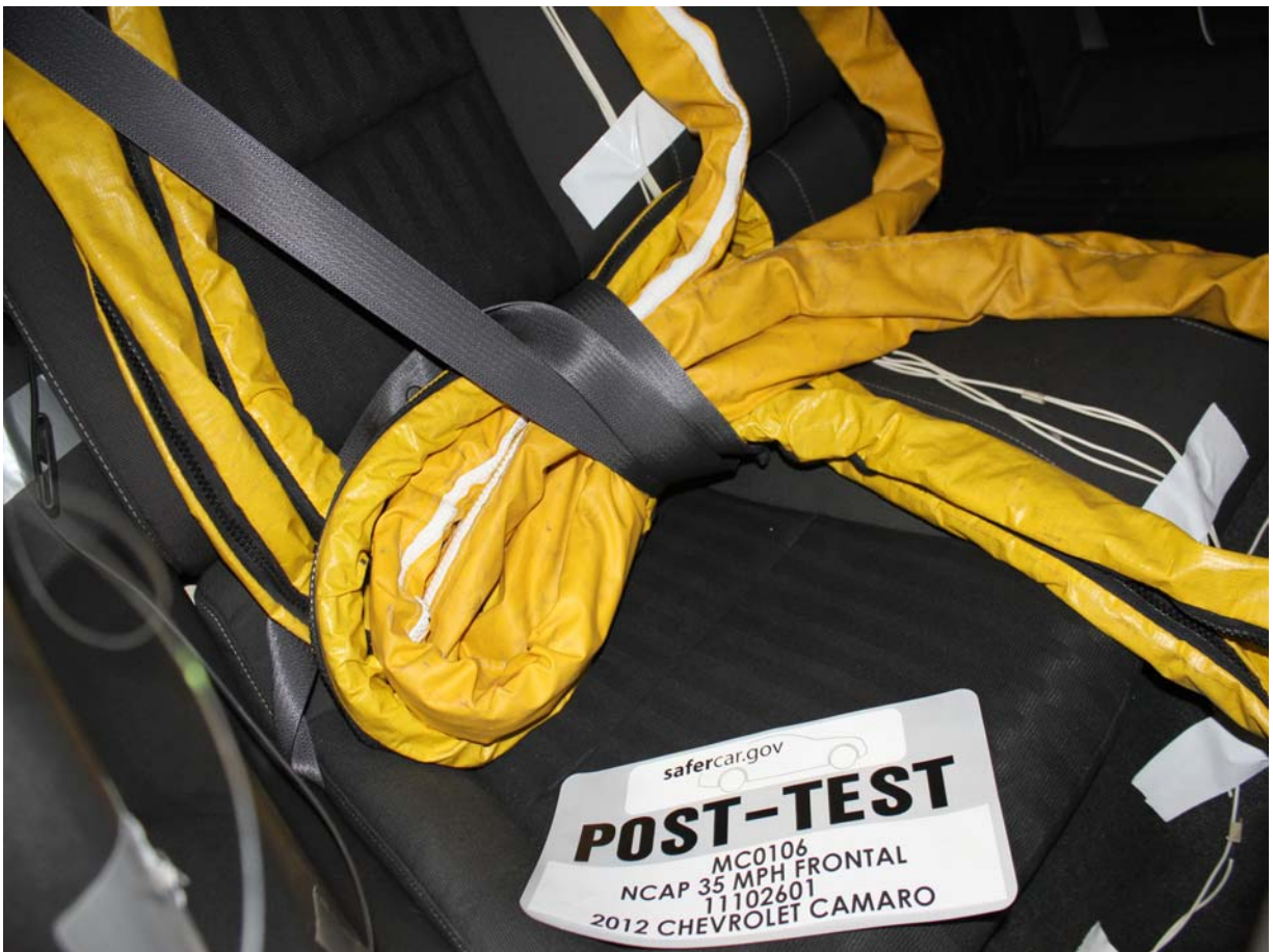
Post-Test Dummy Cable Routing
