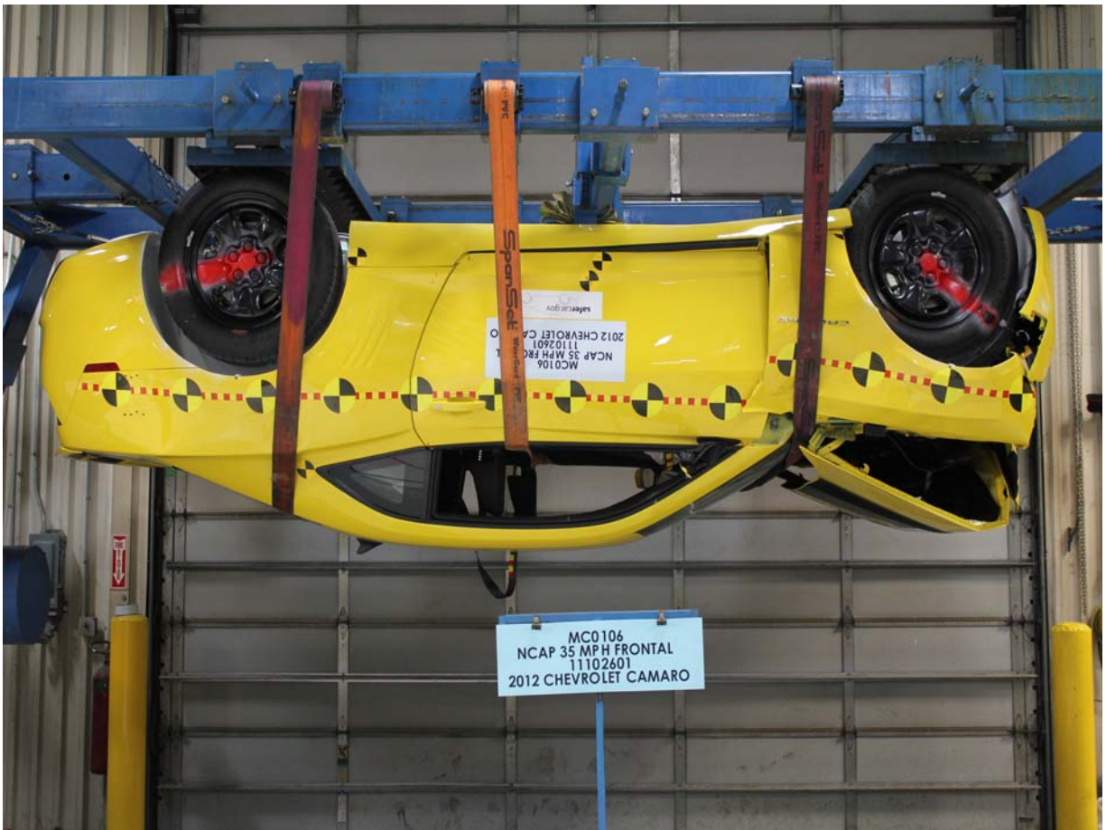
Vehicle at 180 Degrees on Static Rollover Device
