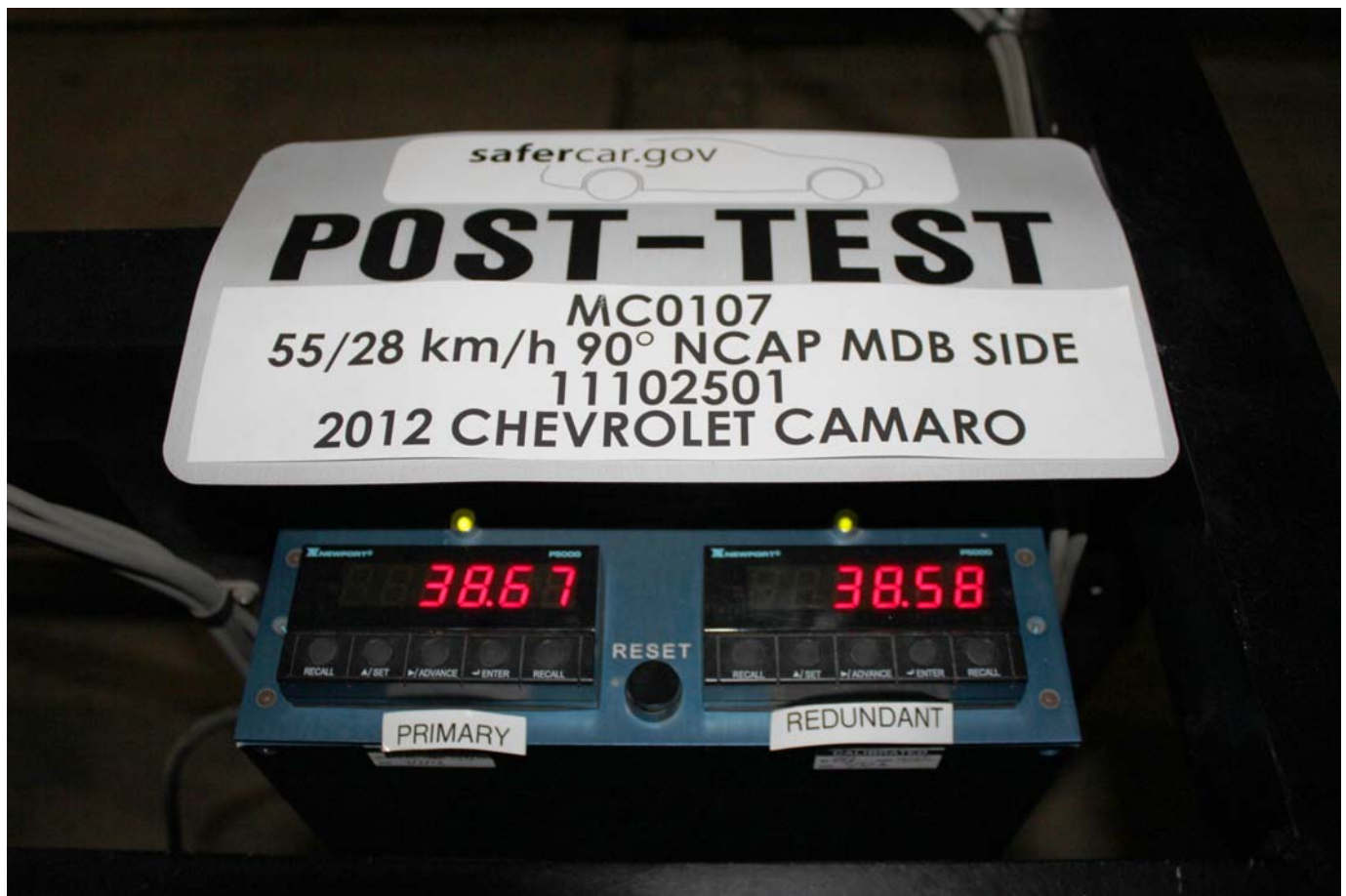
Post-Test Primary and Redundant Speed Trap Read-Out
