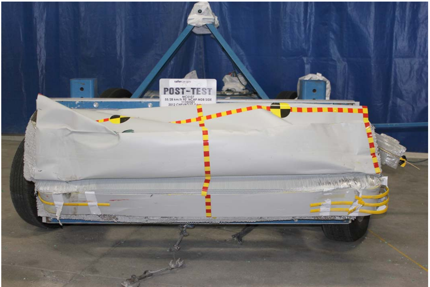
Post-Test Front View of MDB Impactor Face
