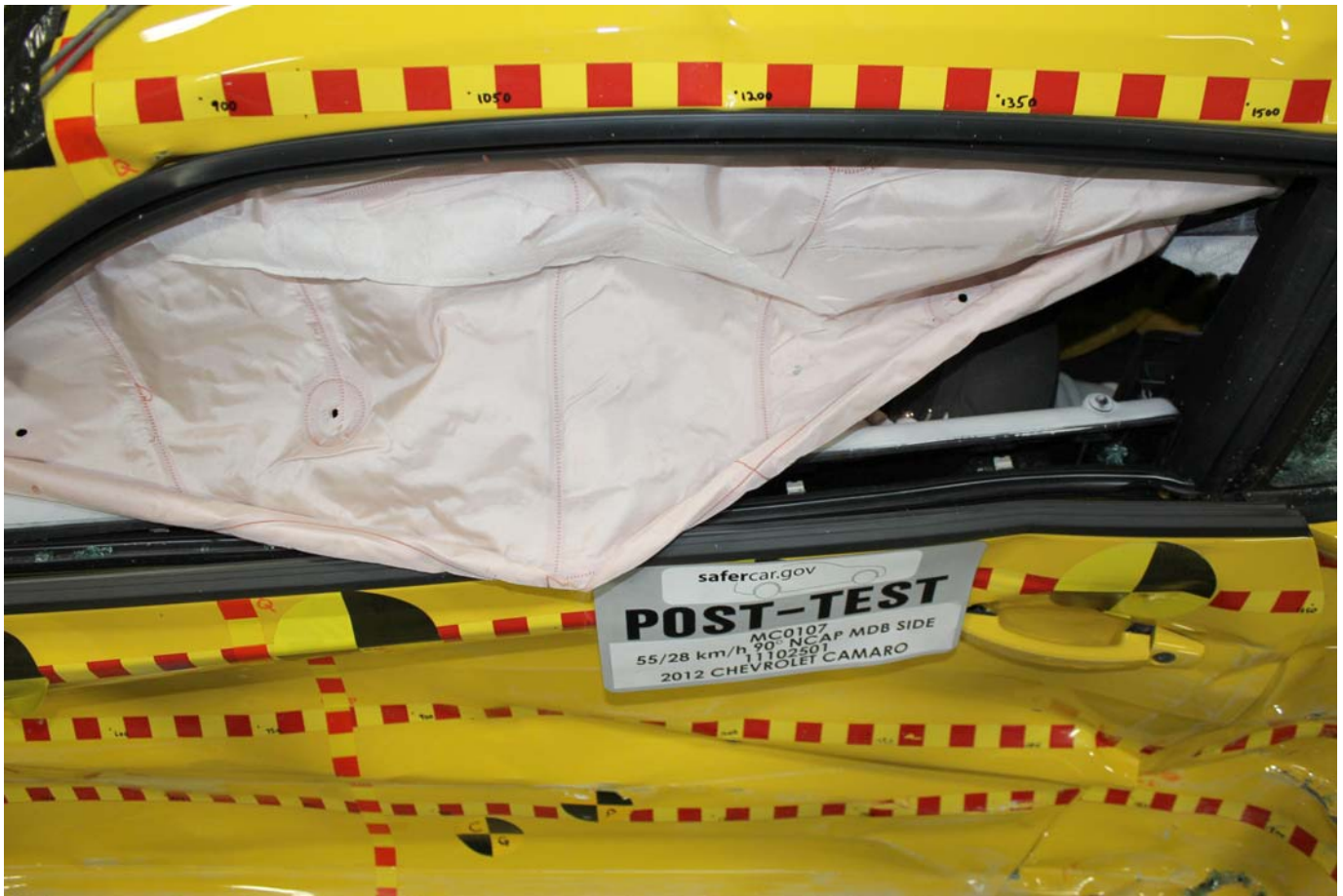
Post-Test Driver Dummy and Door Clearance View
