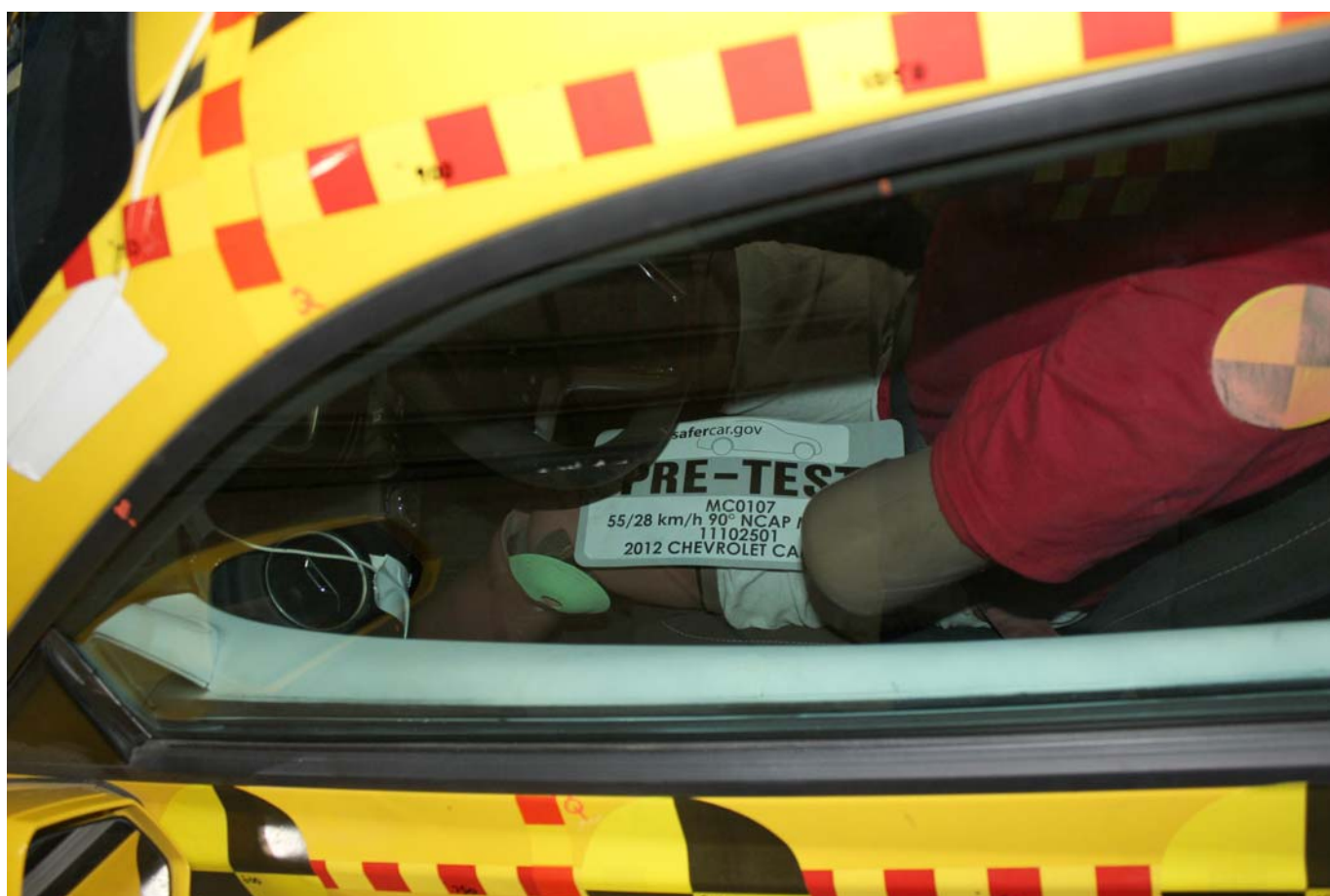
Pre-Test Driver Dummy and Door Clearance View
