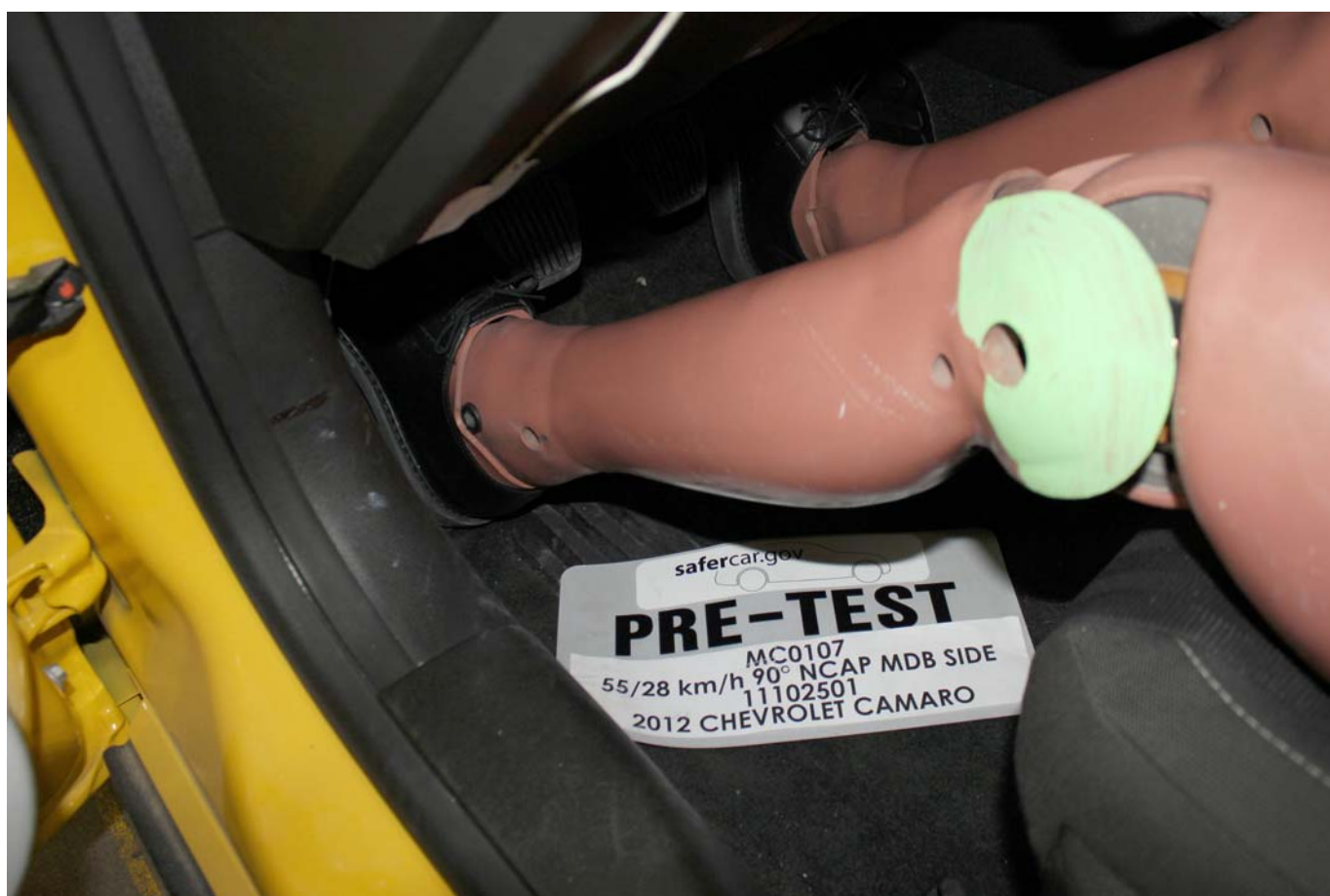
Pre-Test Placement of Driver Dummy's Feet
