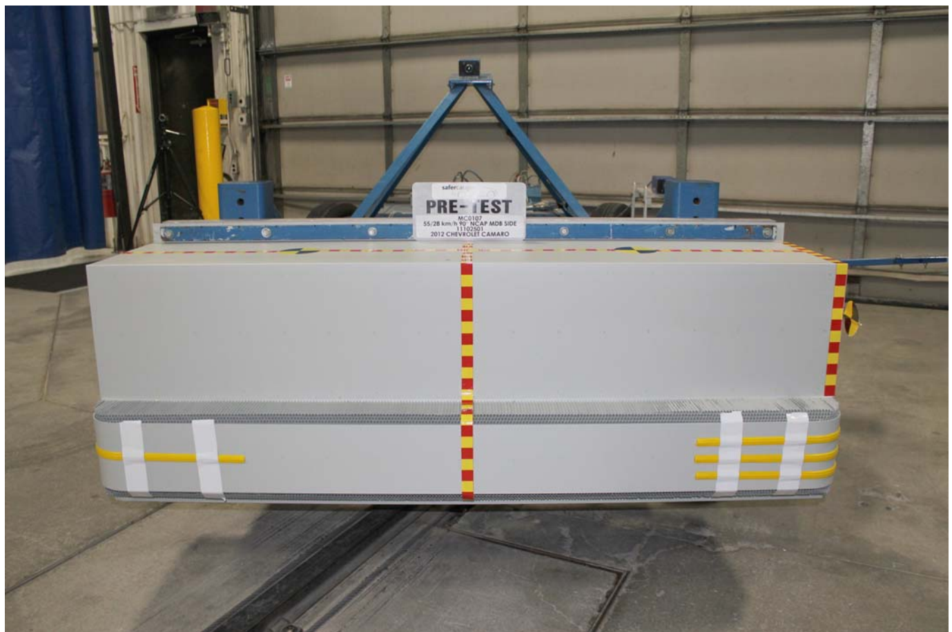
Pre-Test Front View of MDB Impactor Face
