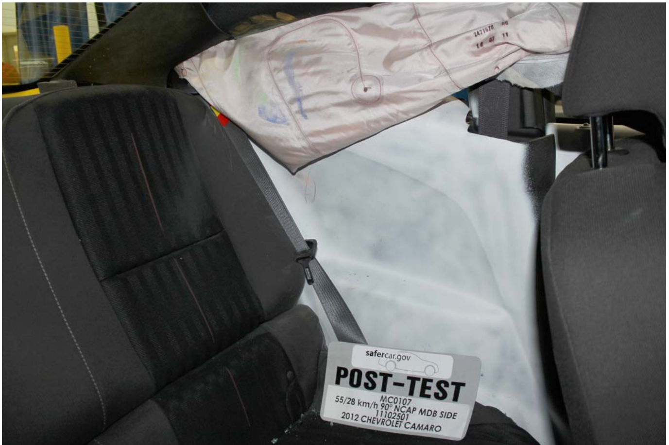
Post-Test Rear Passenger Inner Door Panel View
