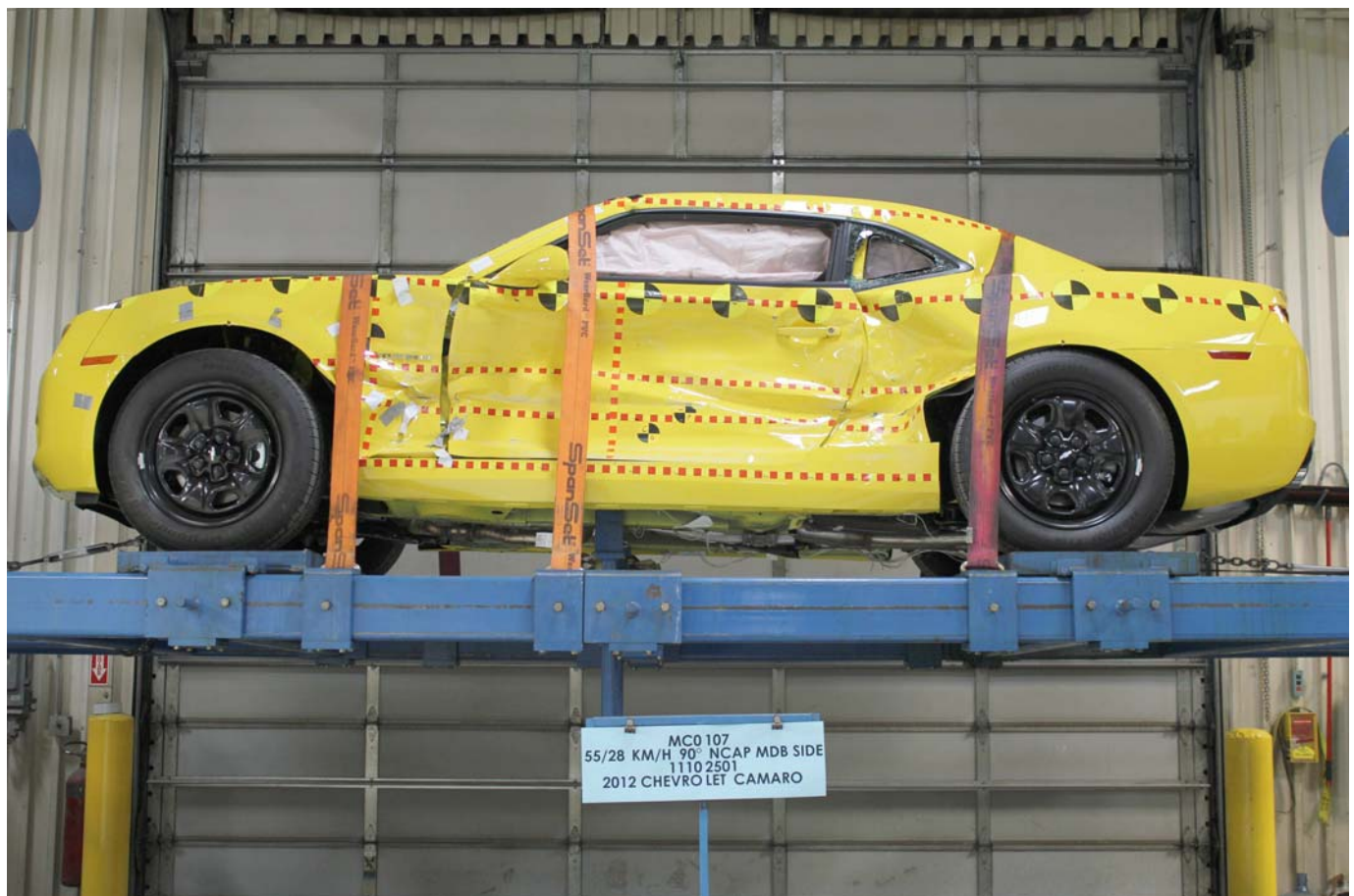
FMVSS No. 301 Static Rollover 0 Degrees
