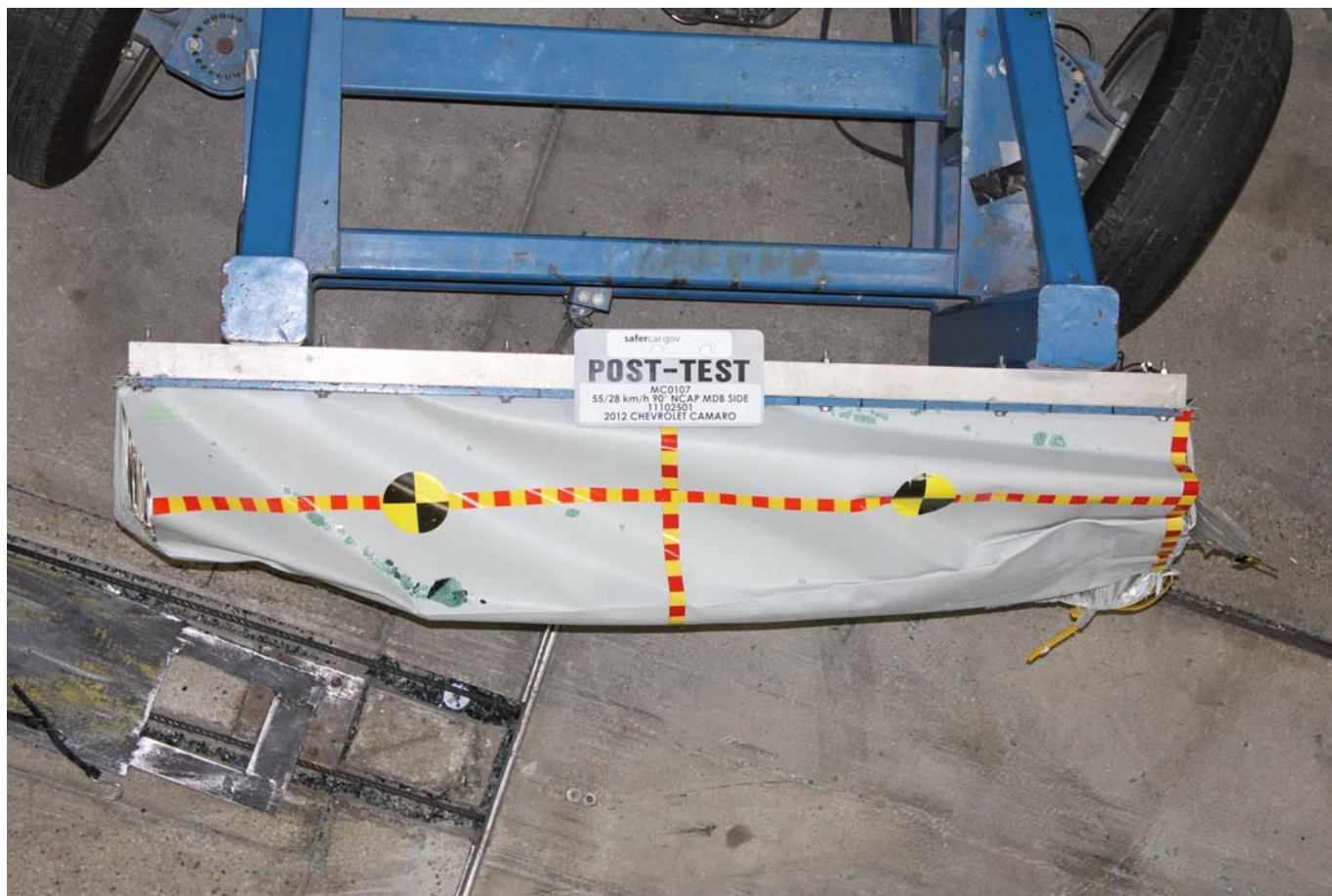
Post-Test Top View of MDB Impactor Face
