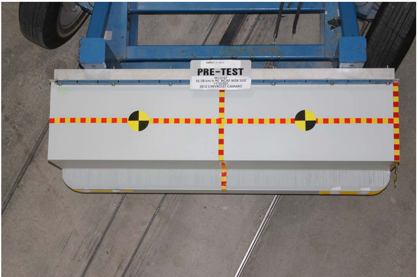
Pre-Test Top View of MDB Impactor Face
