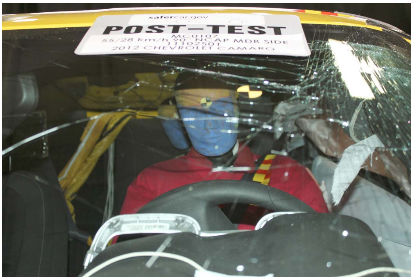
Post-Test Front Close-Up View of Driver Dummy
