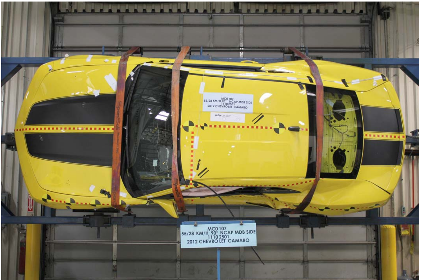
FMVSS No. 301 Static Rollover 270 Degrees
