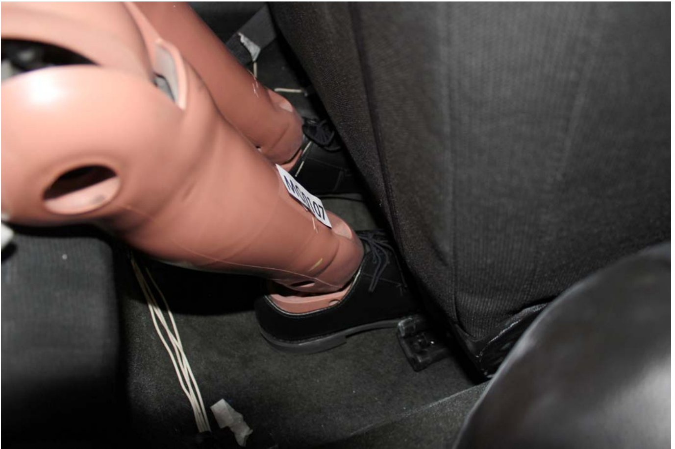
Pre-Test Placement of Rear Passenger Dummy's Feet
