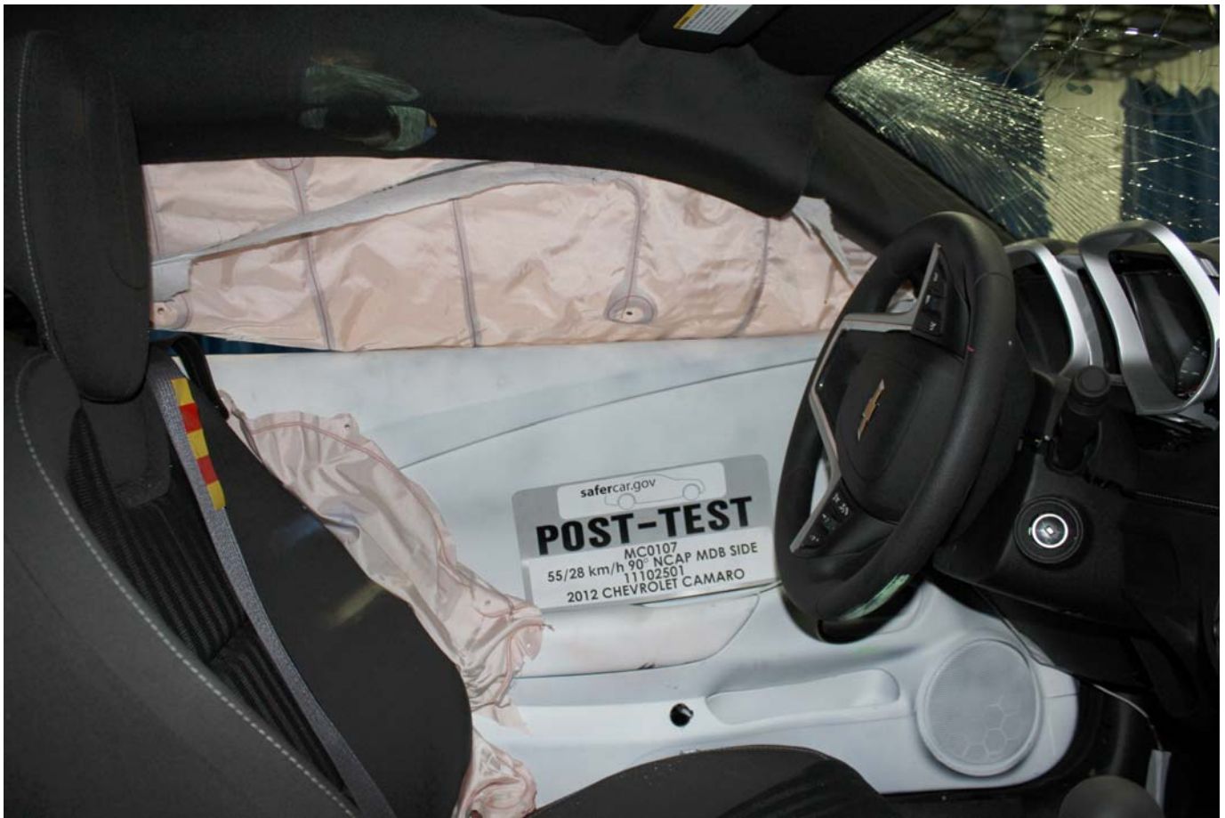
Post-Test Driver Inner Door Panel View
