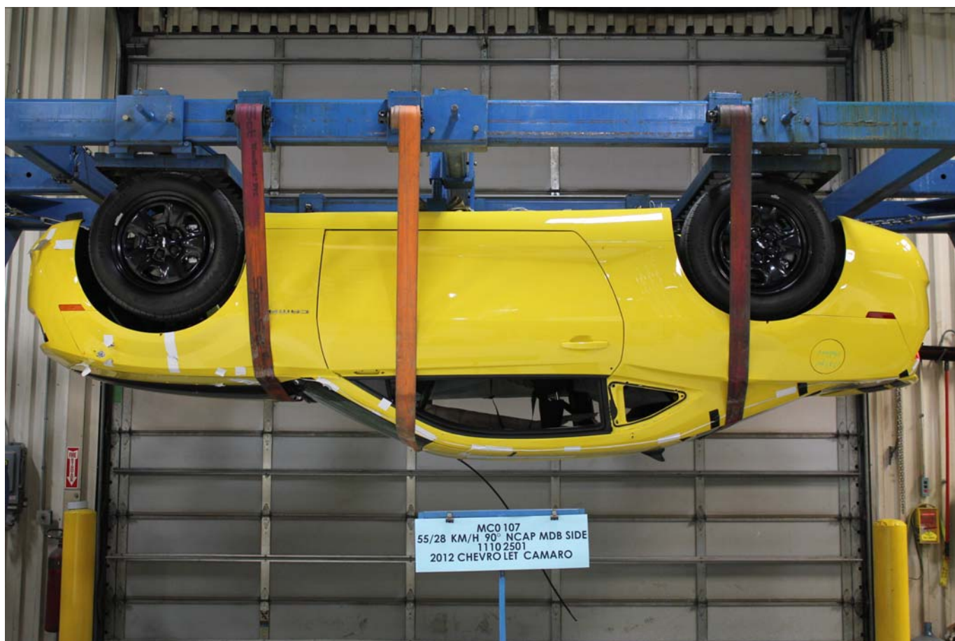
FMVSS No. 301 Static Rollover 180 Degrees
