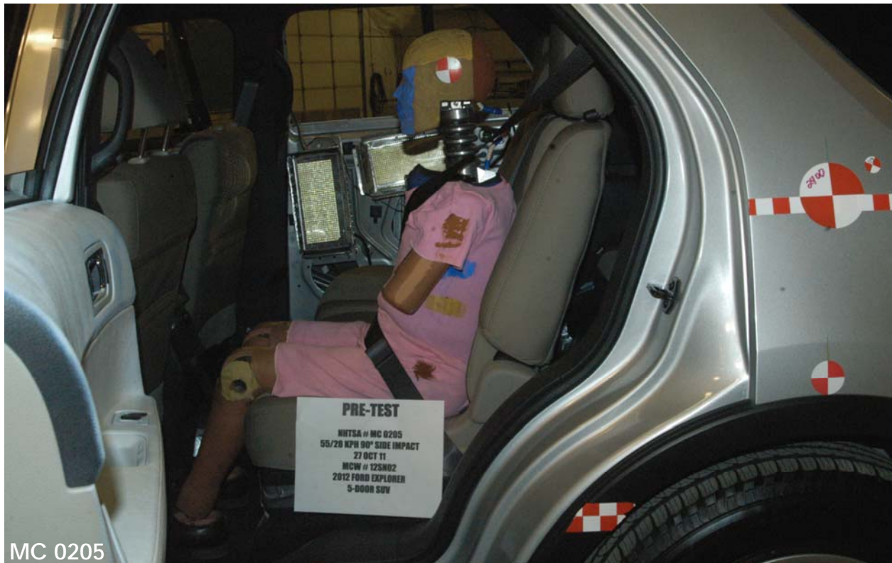
Figure A-54: Pre-Test Left Side View of Rear Passenger Dummy Showing Belt and Chalking
