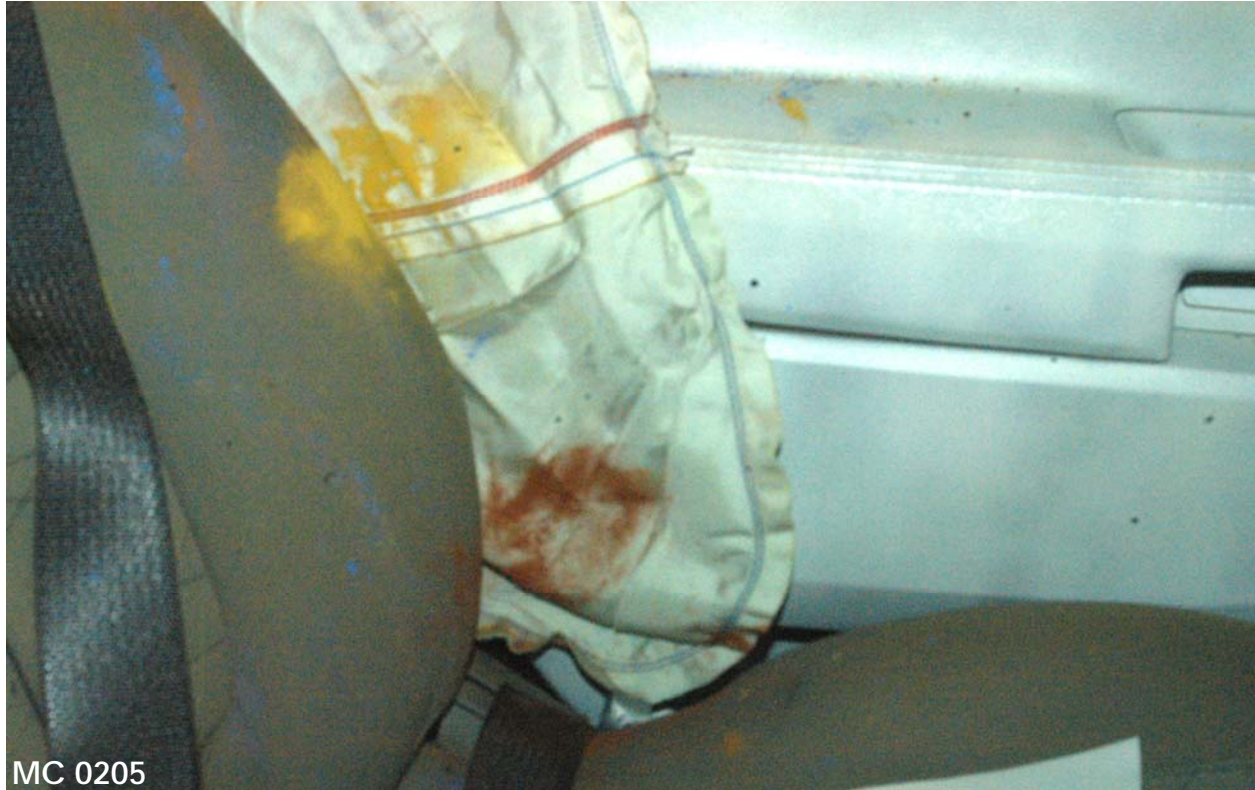
Figure A-53: Post-Test Driver Dummy Close-Up Pelvis Contact with Side Airbag View
