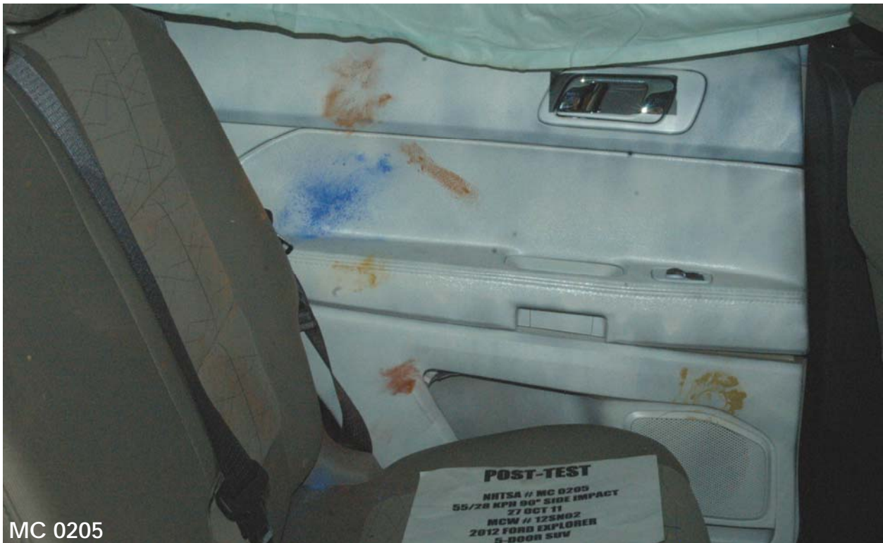
Figure A-76: Post-Test Rear Passenger Dummy Close-Up Torso Contact with Vehicle Interior View
