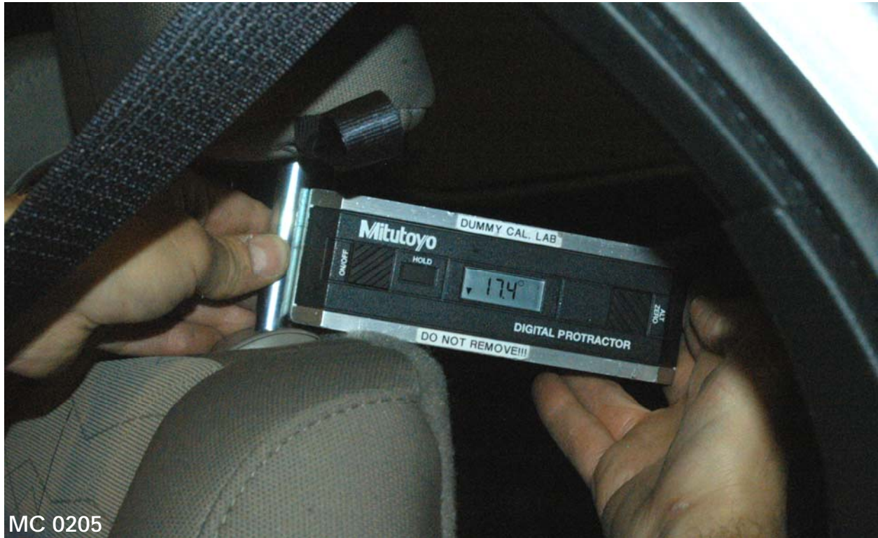
Figure A-41: Pre-Test Close-Up View of Driver Seat Back or Head Restraint
