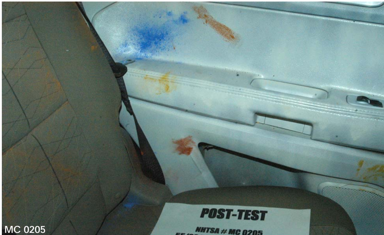
Figure A-78: Post-Test Rear Passenger Dummy Close-up Pelvis Contact with Vehicle Interior View
