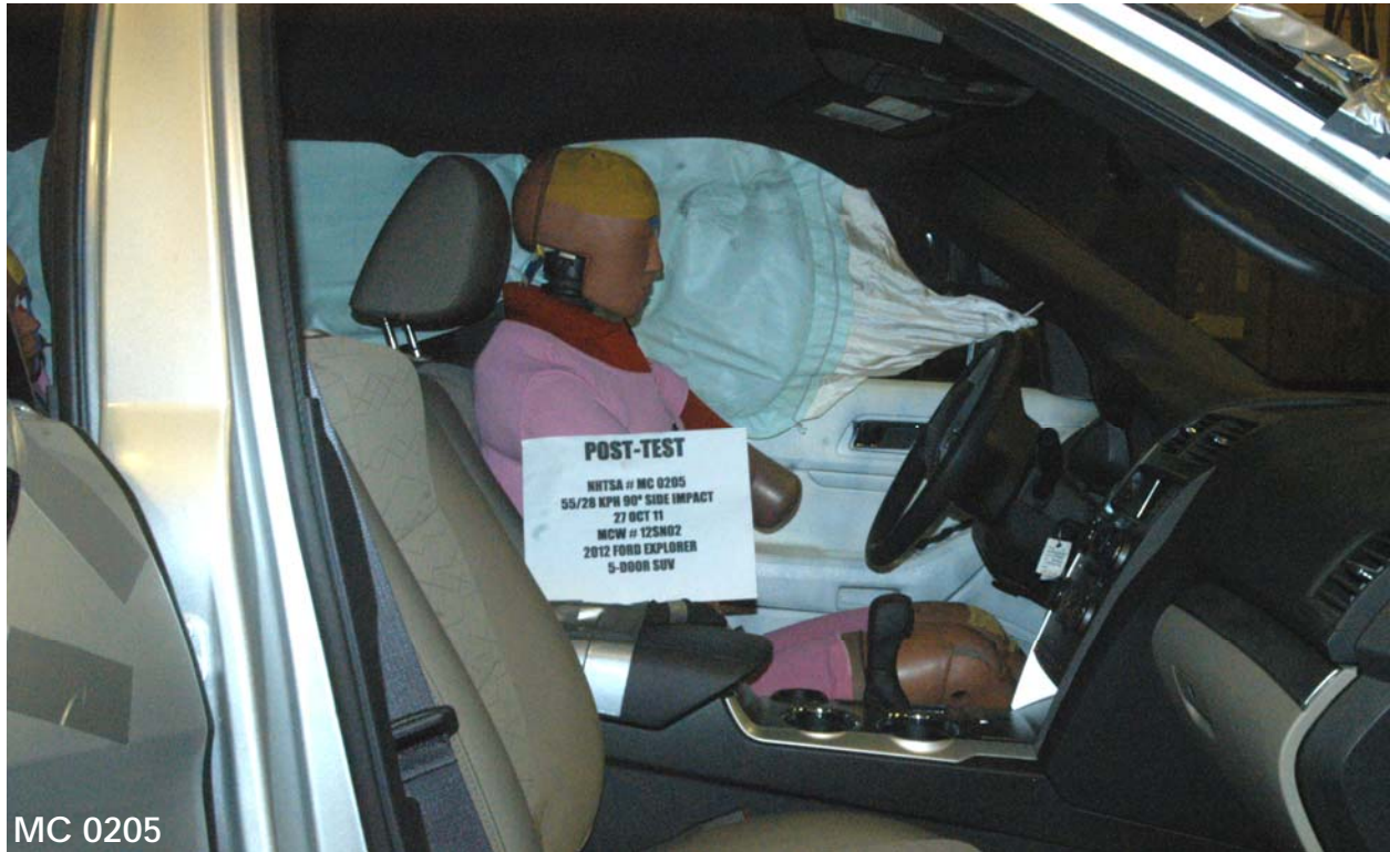
Figure A-45: Post-Test Right Side View of Driver Dummy and Front Seat Occupant Compartment
