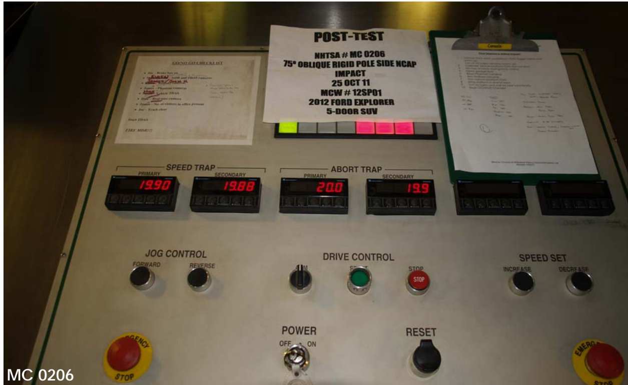
Figure 061: Post-Test Primary and Redundant Speed Trap Read-Out
