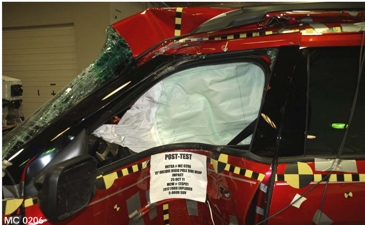
Figure 025: Post-Test Left Side View of Dummy Shoulder and Door Top View
