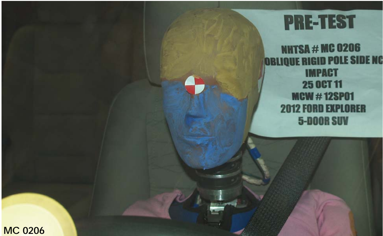
Figure 027: Pre-Test Frontal Close-Up View of Dummy Head and Shoulders in Relation to Head Restraint
