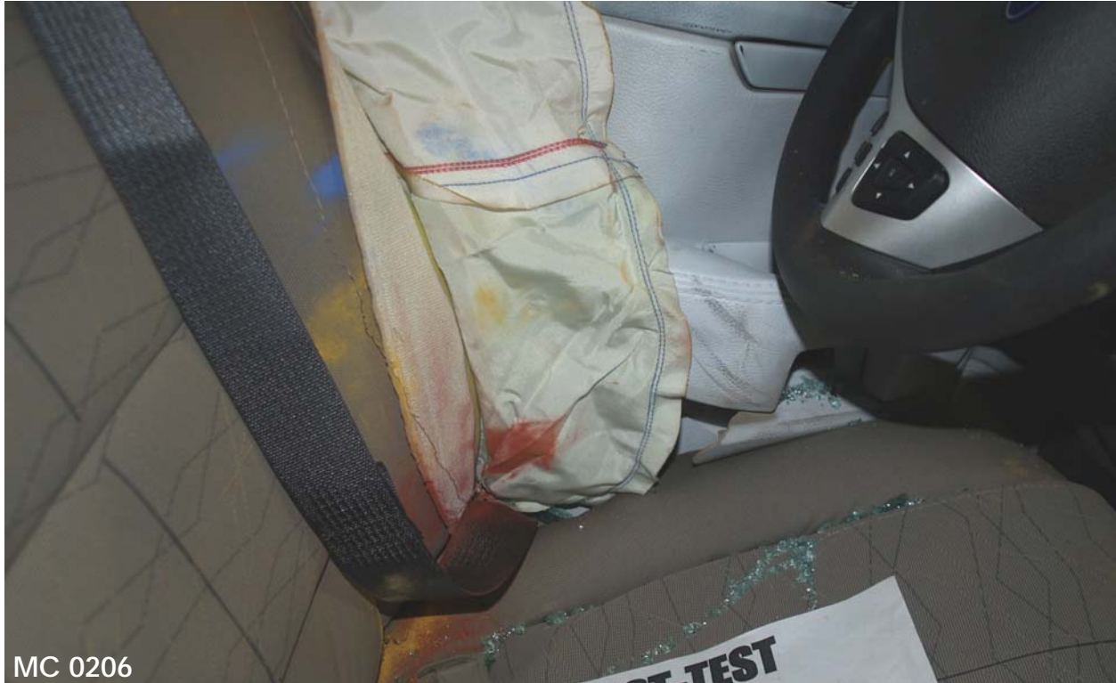
Figure 051: Post-Test Dummy Close-Up Pelvis Contact with Side Air bag View
