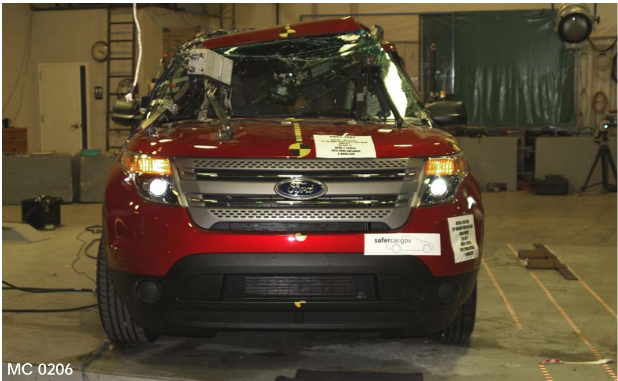
Figure 004: Post-Test Frontal View of Test Vehicle
