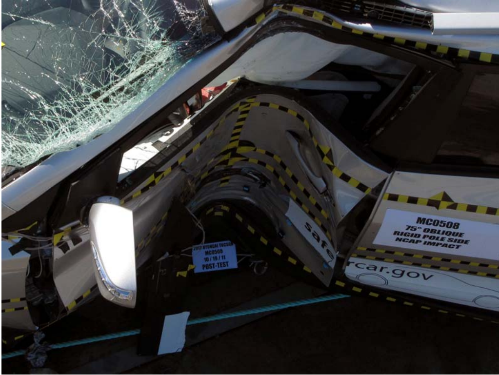
FIGURE 41. Post-Test Driver Dummy and Door Clearance
