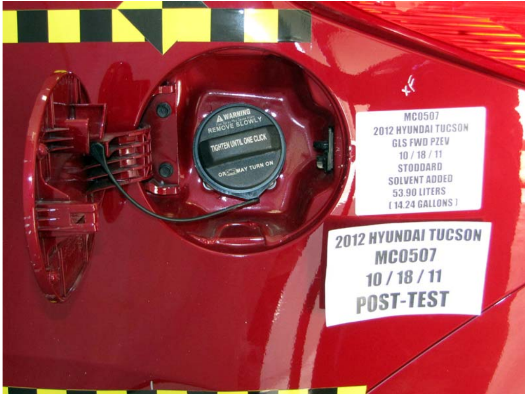
FIGURE 81. Post-Test View of Fuel Filler Cap
