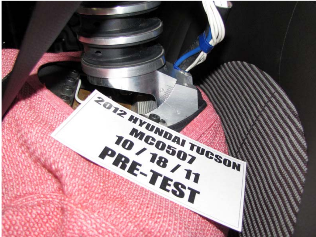
FIGURE 61. Pre-Test View of Rear Passenger Dummy's Neck Showing Position of Adjustable Neck Bracket
