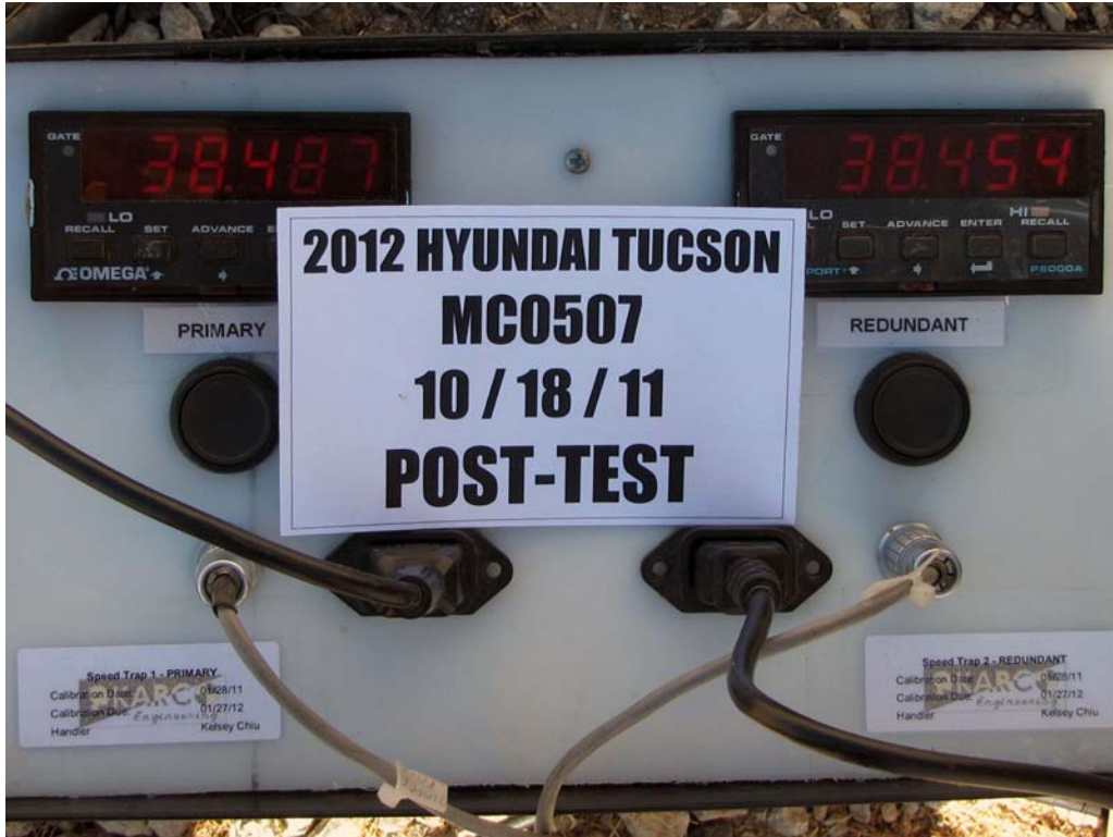
FIGURE 93. Post-Test Primary and Redundant Speed Trap Read-Out
