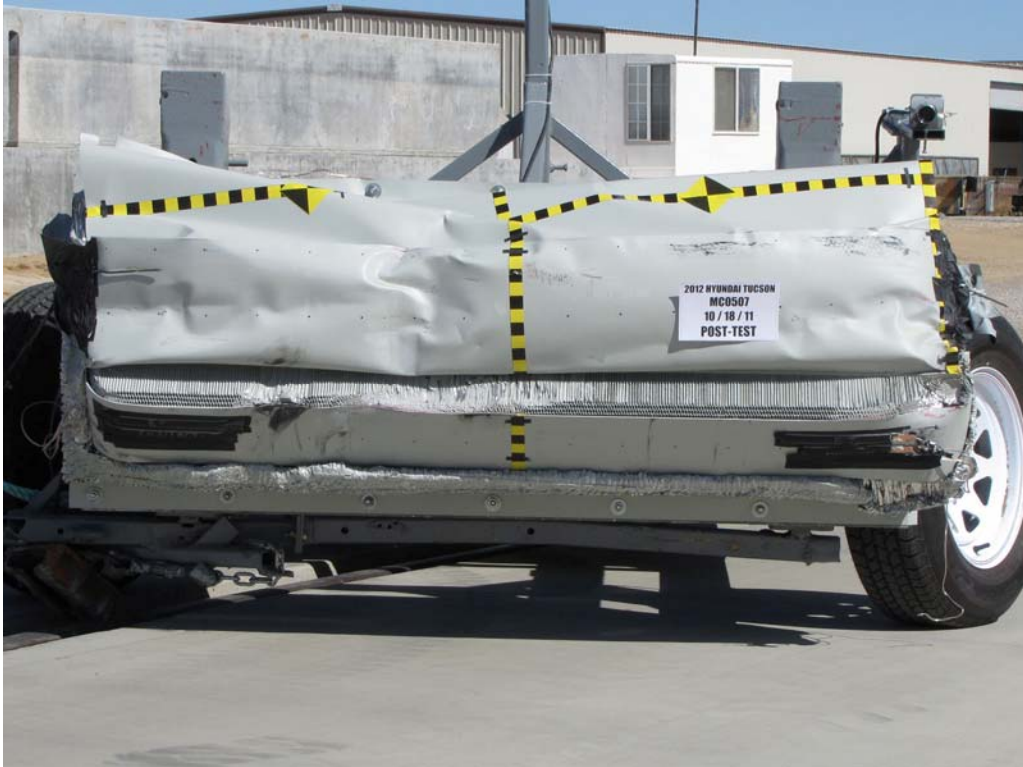
FIGURE 83. Post-Test Front View of MDB Impactor Face
