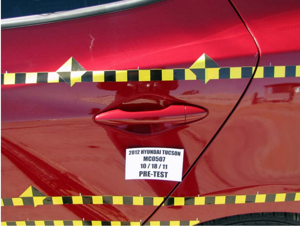
FIGURE 23. Pre-Test Left Rear Door Latch Close-Up
