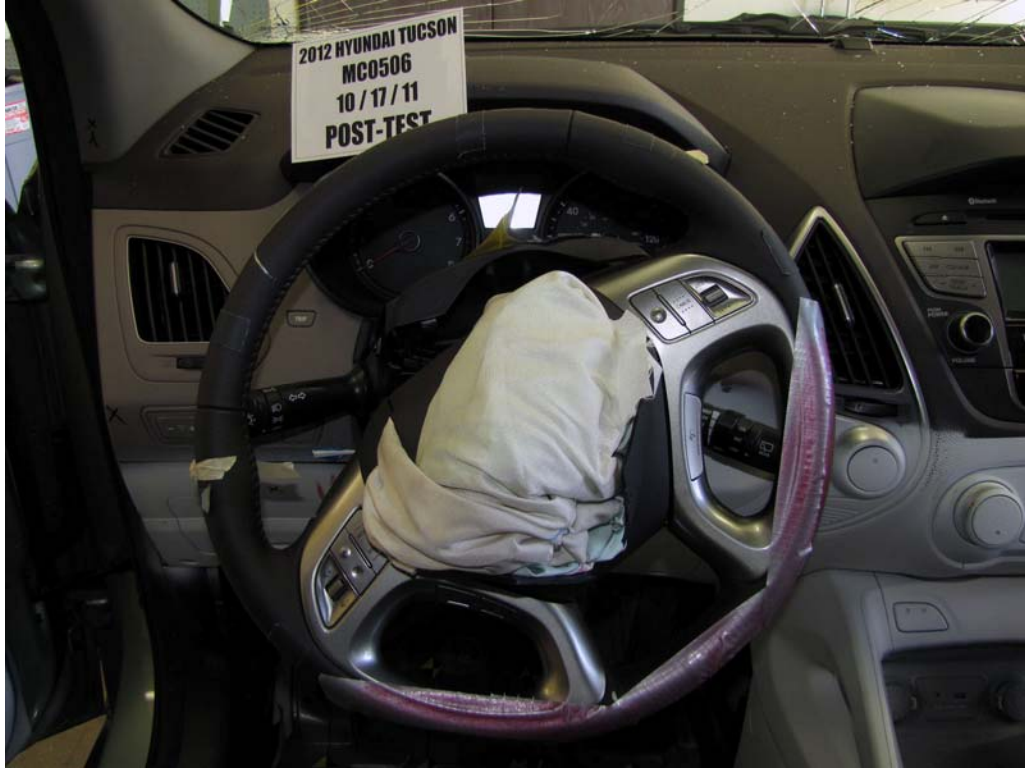
FIGURE 47. Post-Test View Of Steering Wheel
