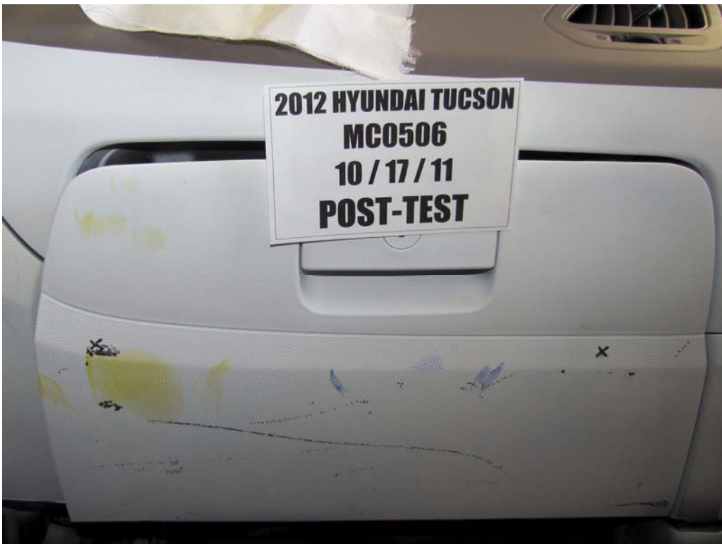
FIGURE 62b. Post-Test Passenger Dummy Contact With Glovebox
