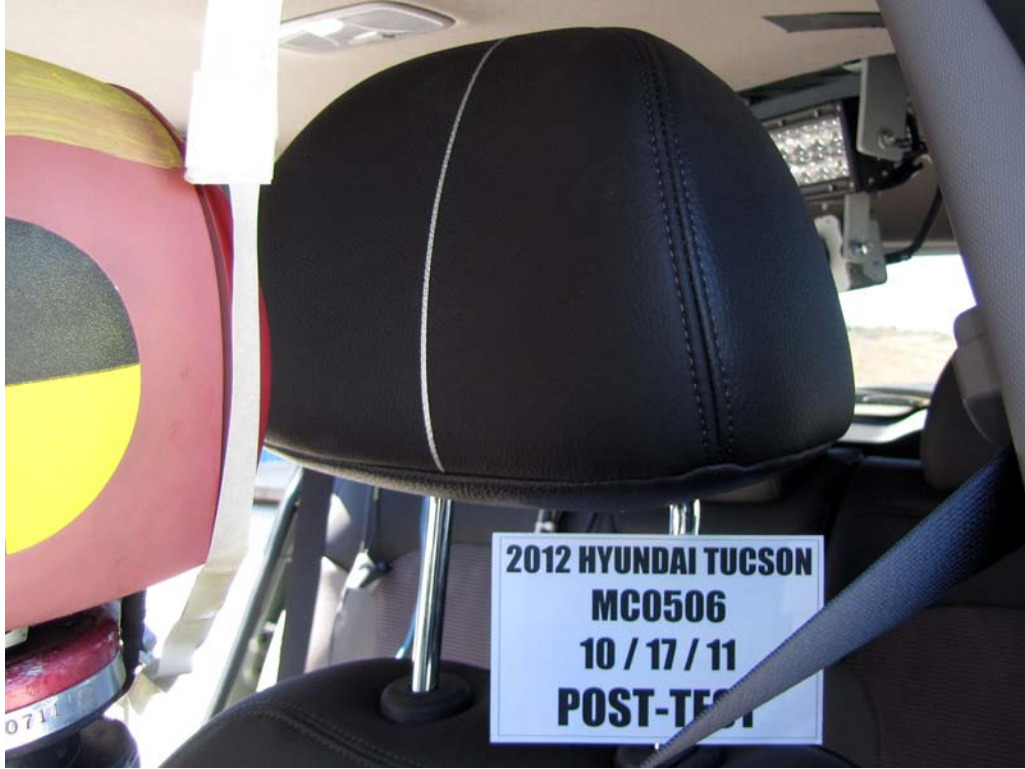
FIGURE 45. Post-Test Driver Dummy Contact With Head Rest
