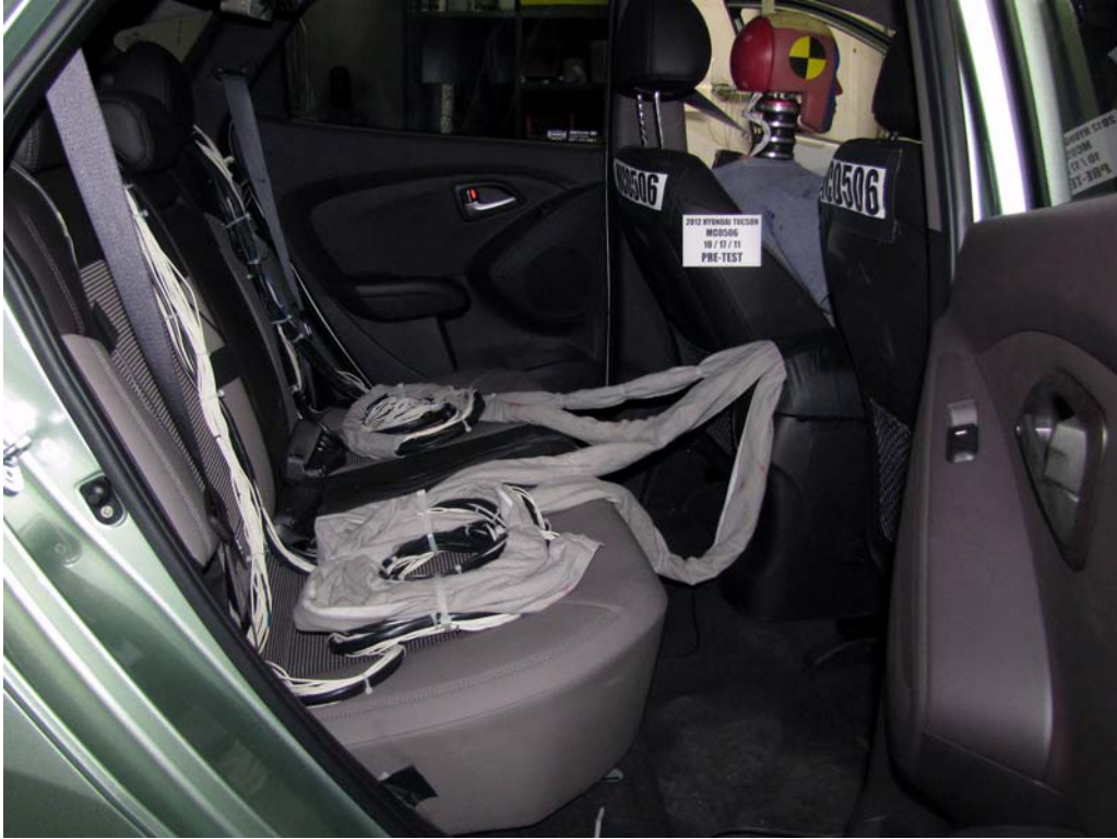
FIGURE 27. Pre-Test Dummy Cable Routing
