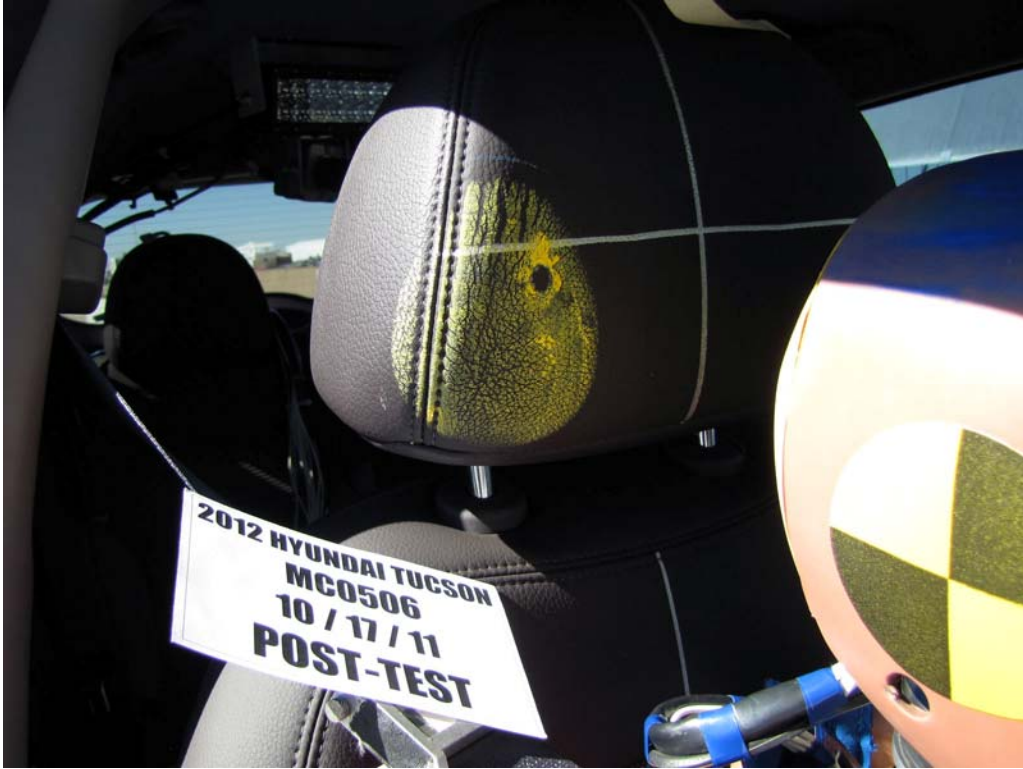
FIGURE 62a. Post-Test Passenger Dummy Contact With Headrest
