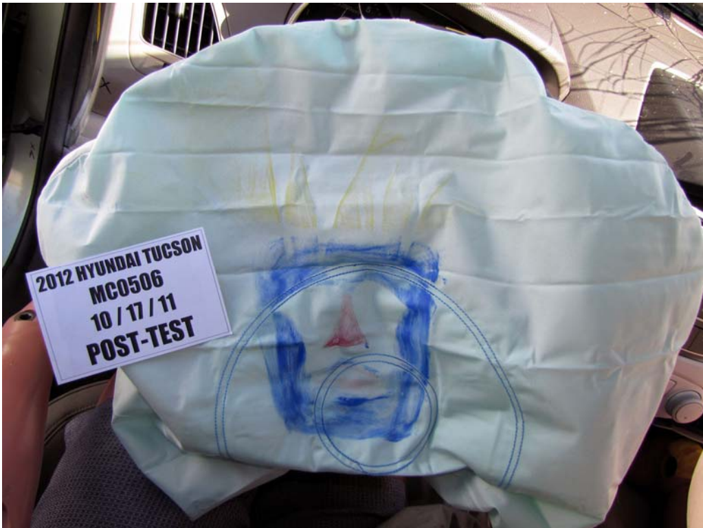
FIGURE 44. Post-Test Driver Dummy Contact With Airbag
