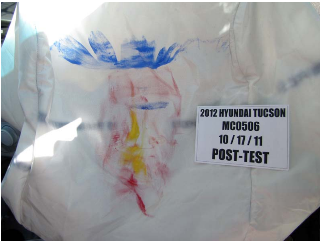
FIGURE 62. Post-Test Passenger Dummy Contact With Airbag
