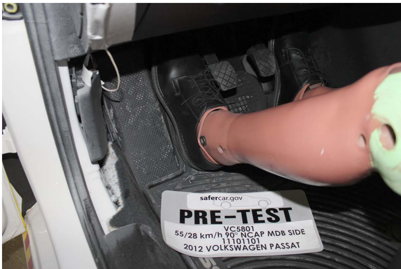
Pre-Test Placement of Driver Dummy's Feet
