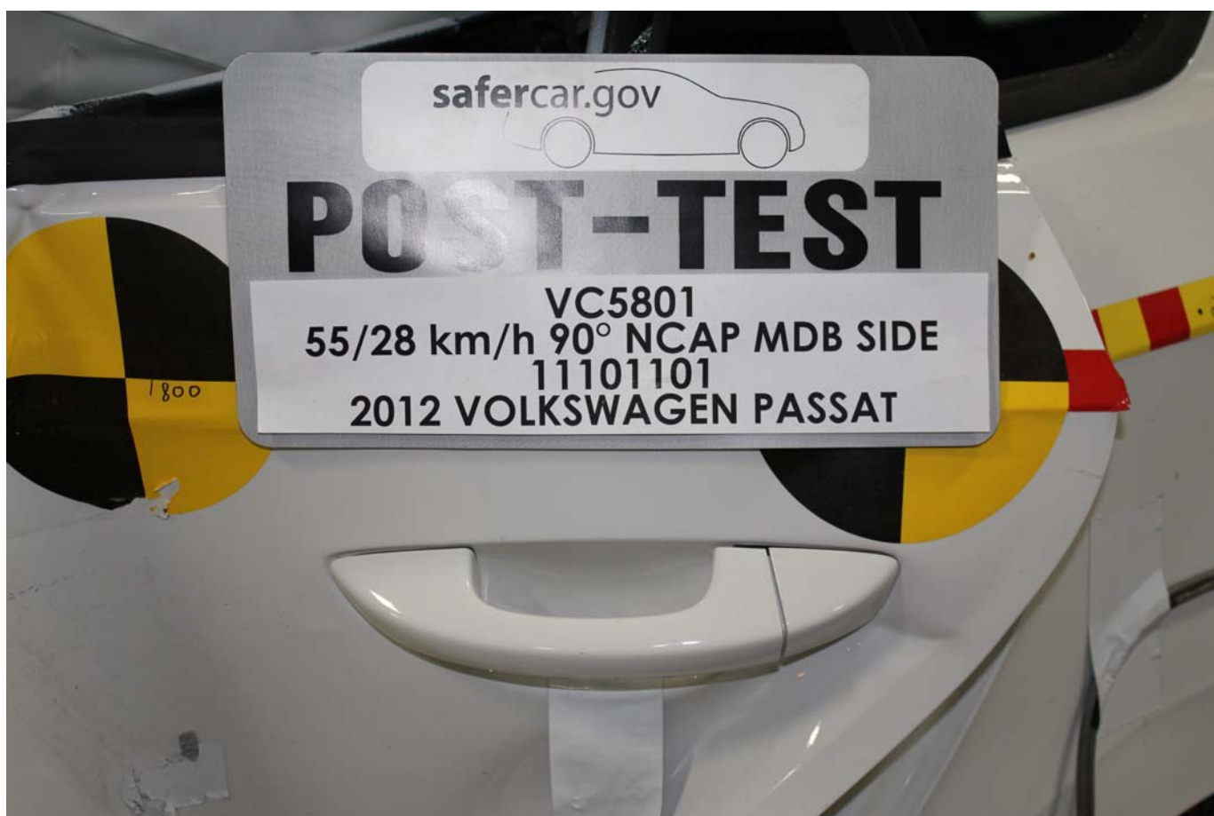
Post-Test Left Rear Door Latch Close-Up
