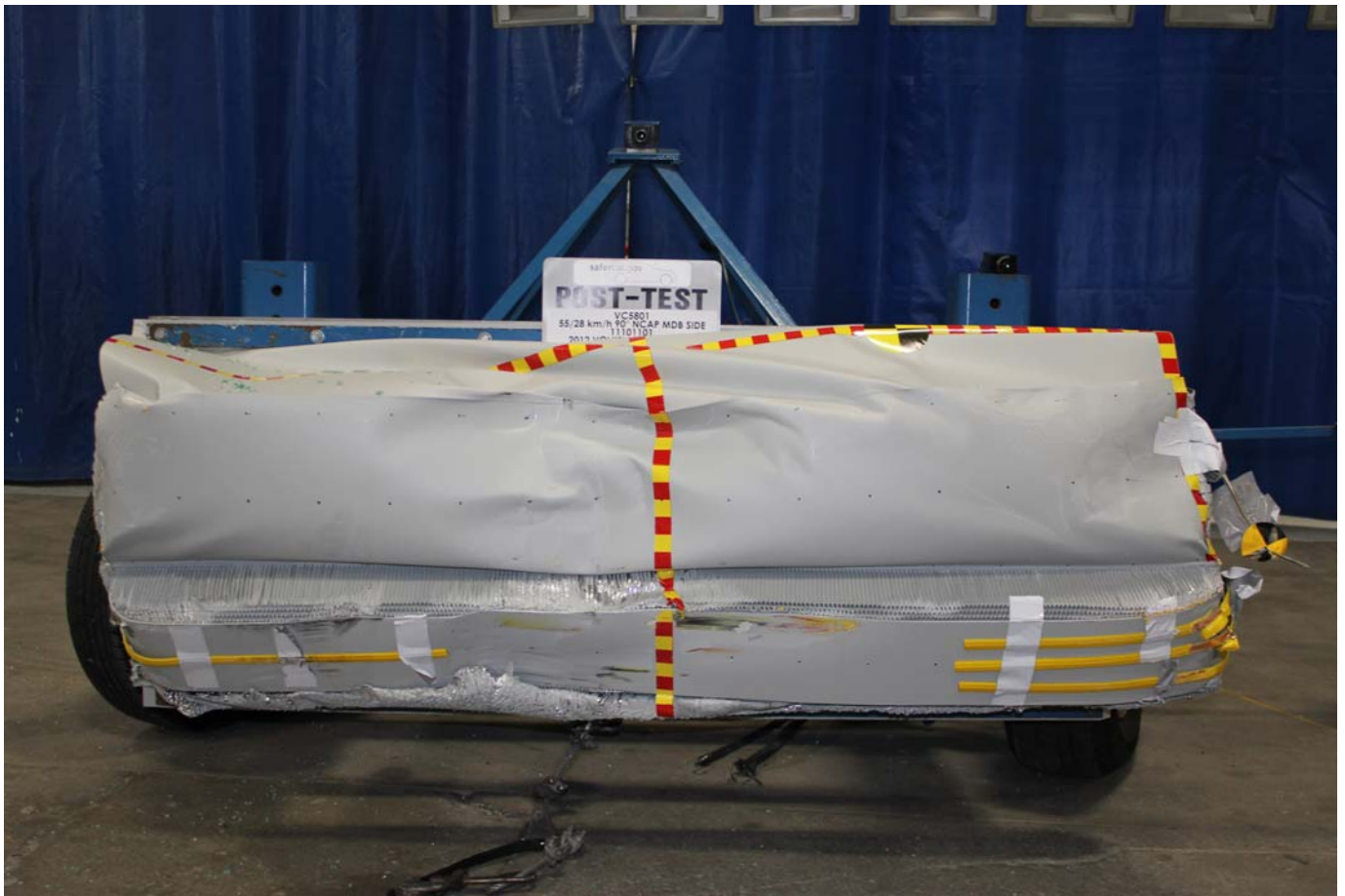
Post-Test Front View of MDB Impactor Face
