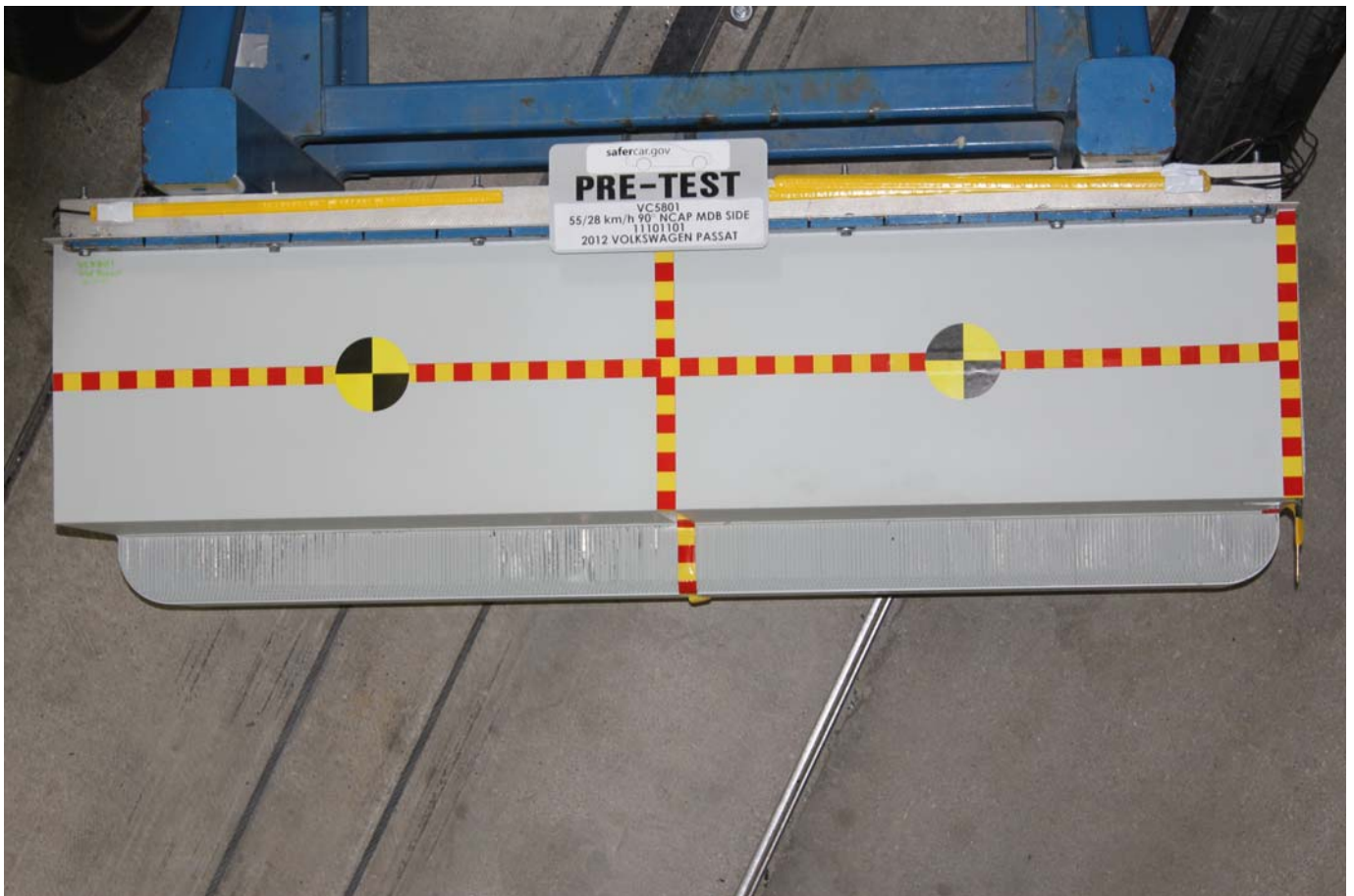
Pre-Test Top View of MDB Impactor Face
