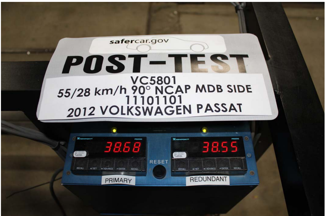
Post-Test Primary and Redundant Speed Trap Read-Out
