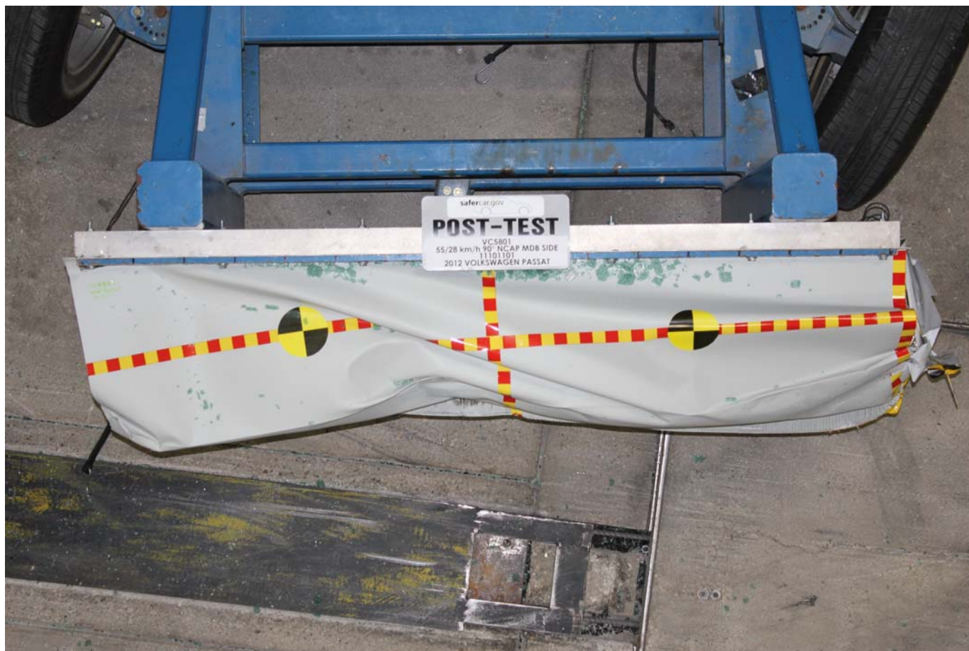
Post-Test Top View of MDB Impactor Face
