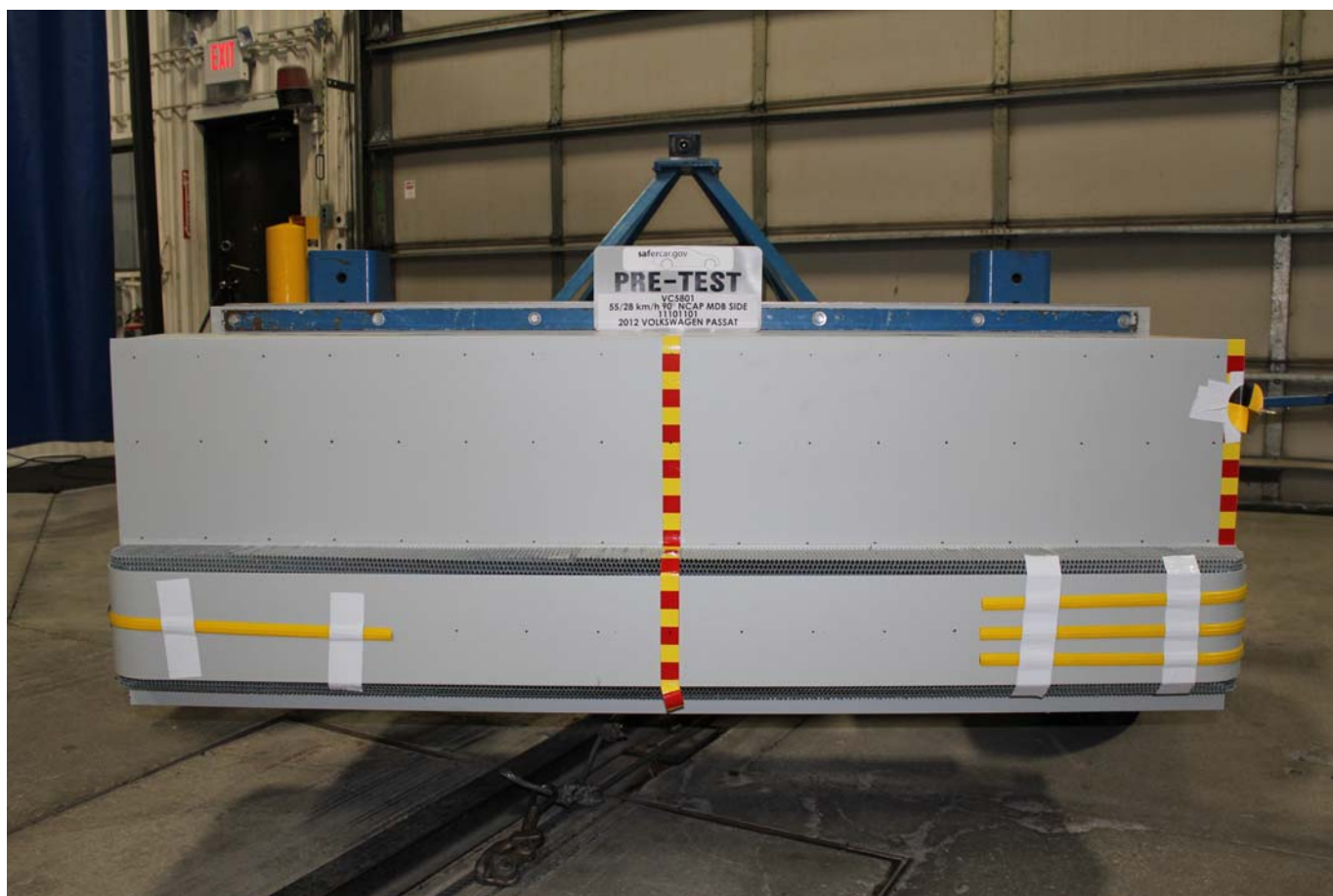
Pre-Test Front View of MDB Impactor Face
