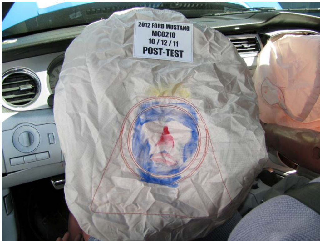
FIGURE 44. Post-Test Driver Dummy Contact With Airbag
