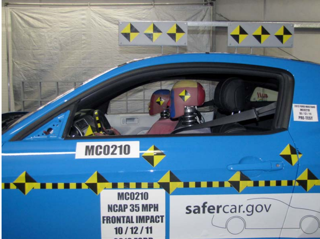
FIGURE 31. Pre-Test Driver Dummy Window View
