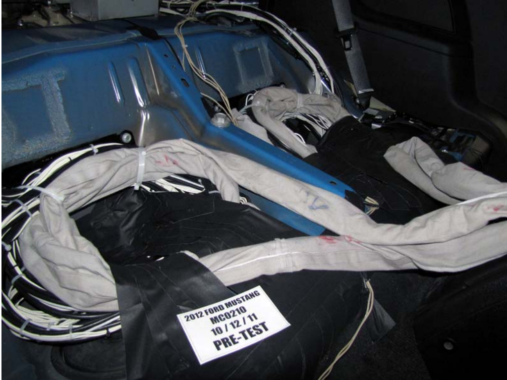
FIGURE 27. Pre-Test Dummy Cable Routing
