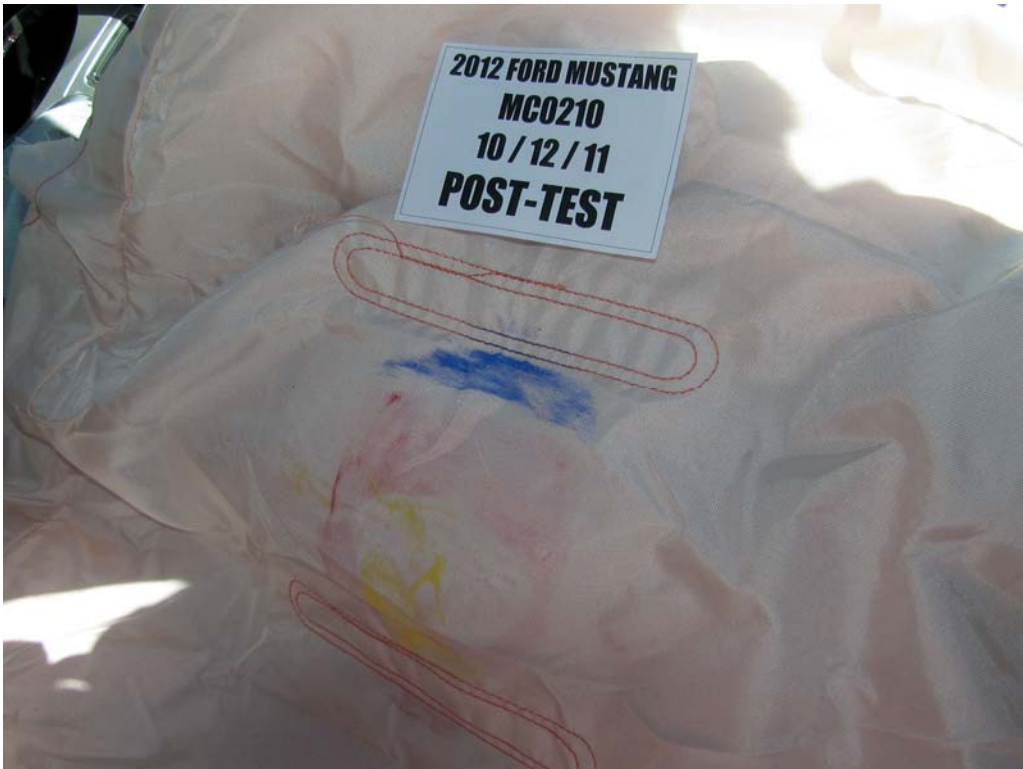
FIGURE 62. Post-Test Passenger Dummy Contact With Airbag
