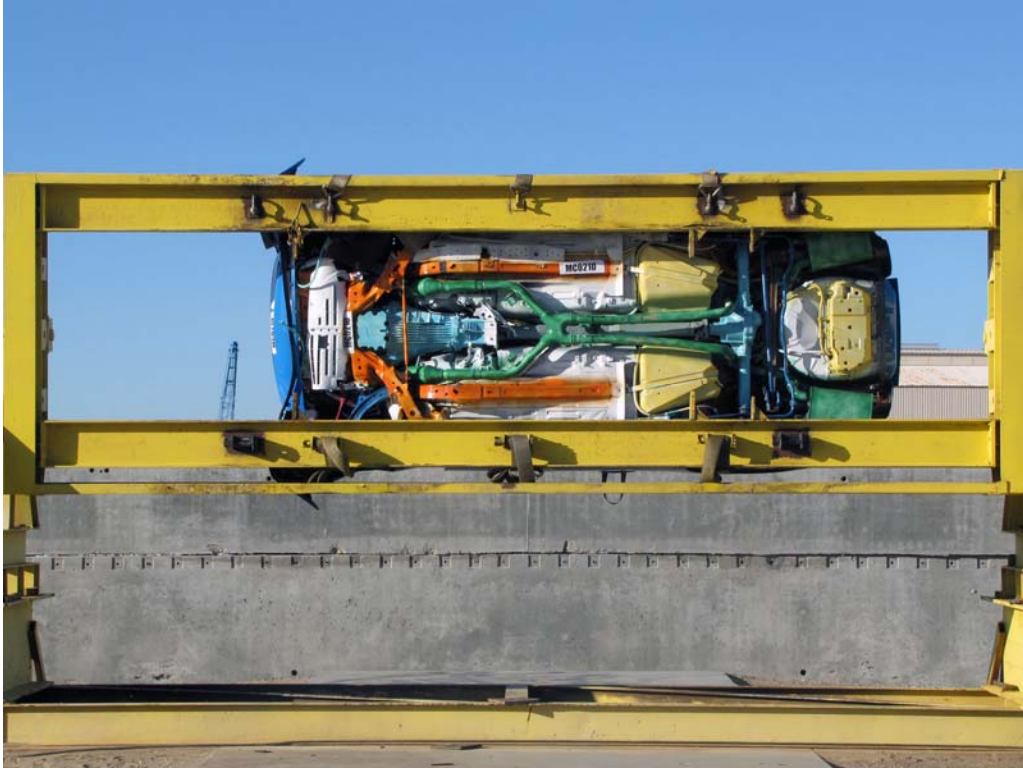
FIGURE 69. Vehicle at 270°on Static Rollover Device
