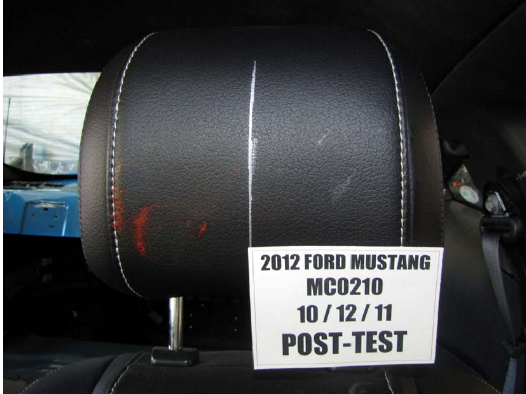
FIGURE 45. Post-Test Driver Dummy Contact With Head Rest
