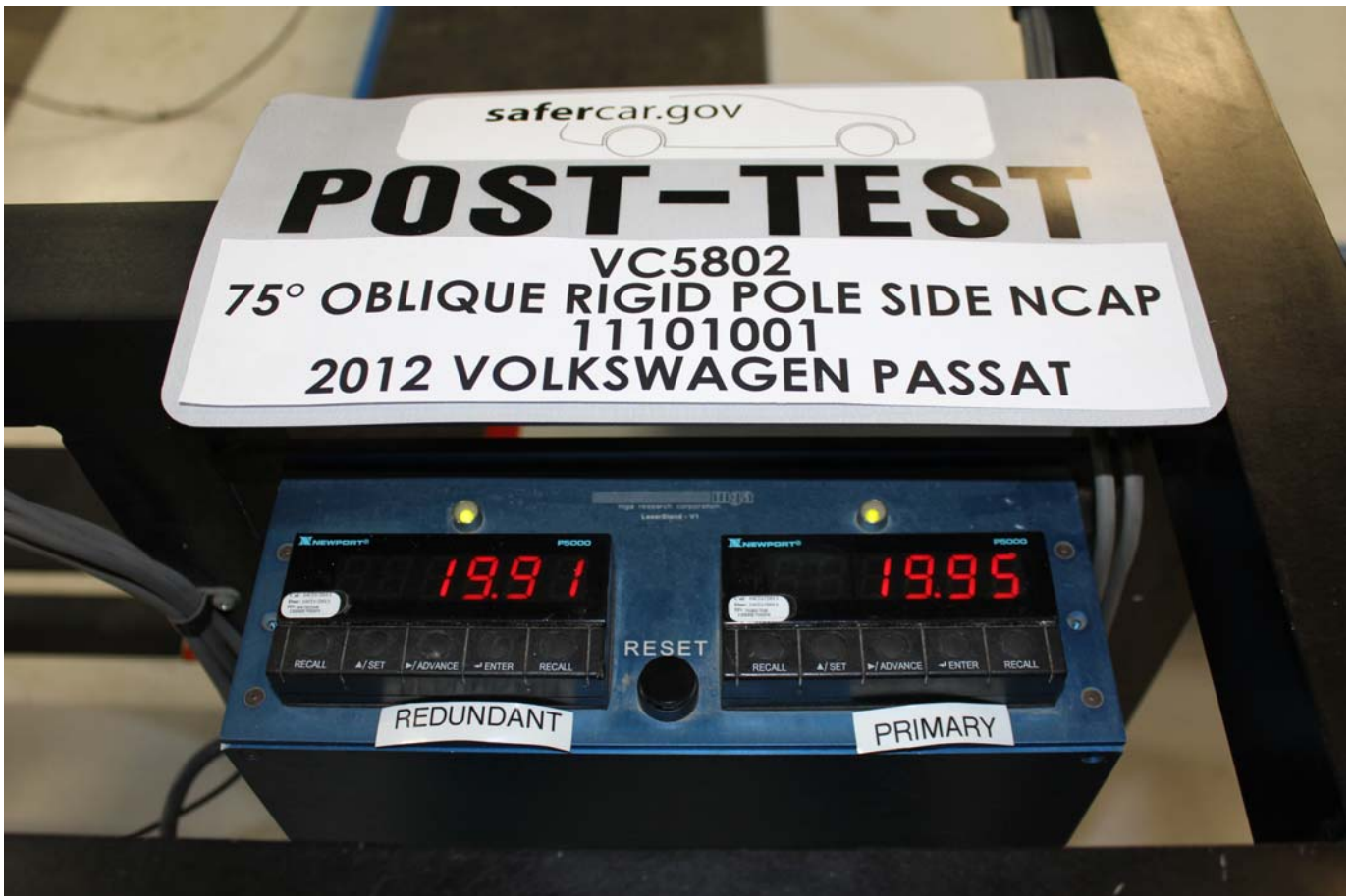
Post-Test Primary and Redundant Speed Trap Read-Out
