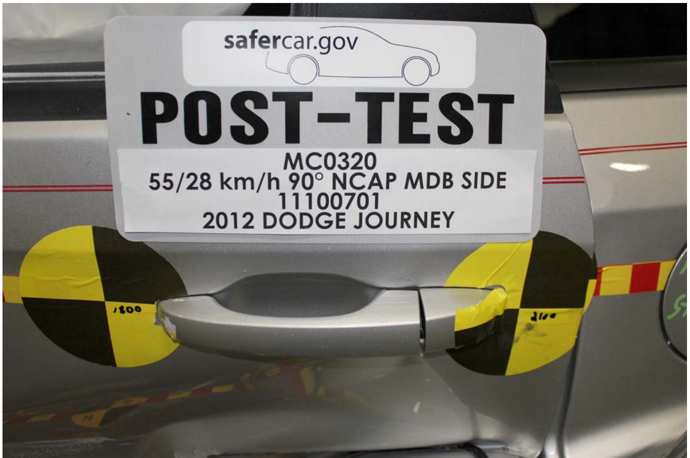
Post-Test Left Rear Door Latch Close-Up
