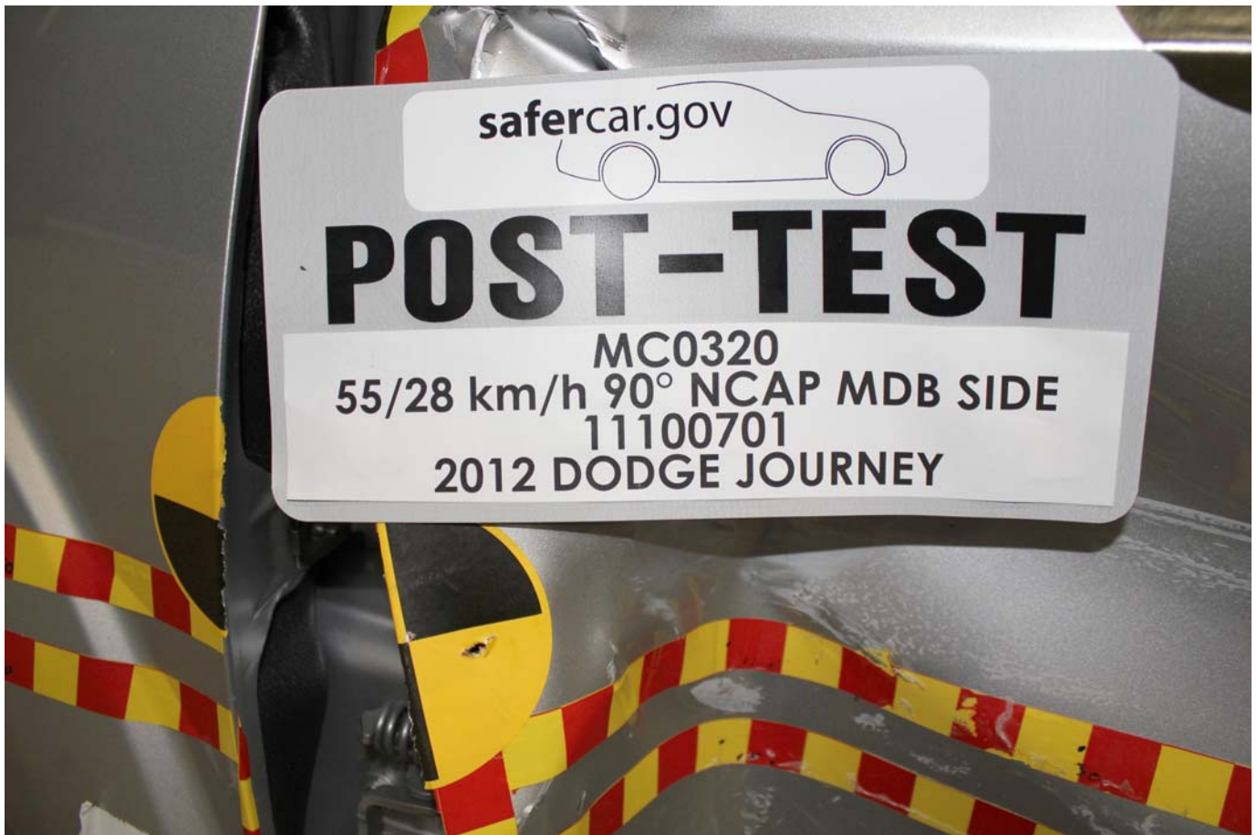
Post-Test Close-Up View of Impact Point Target
