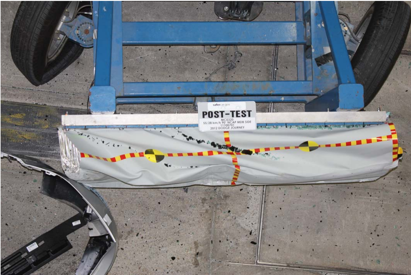
Post-Test Top View of MDB Impactor Face
