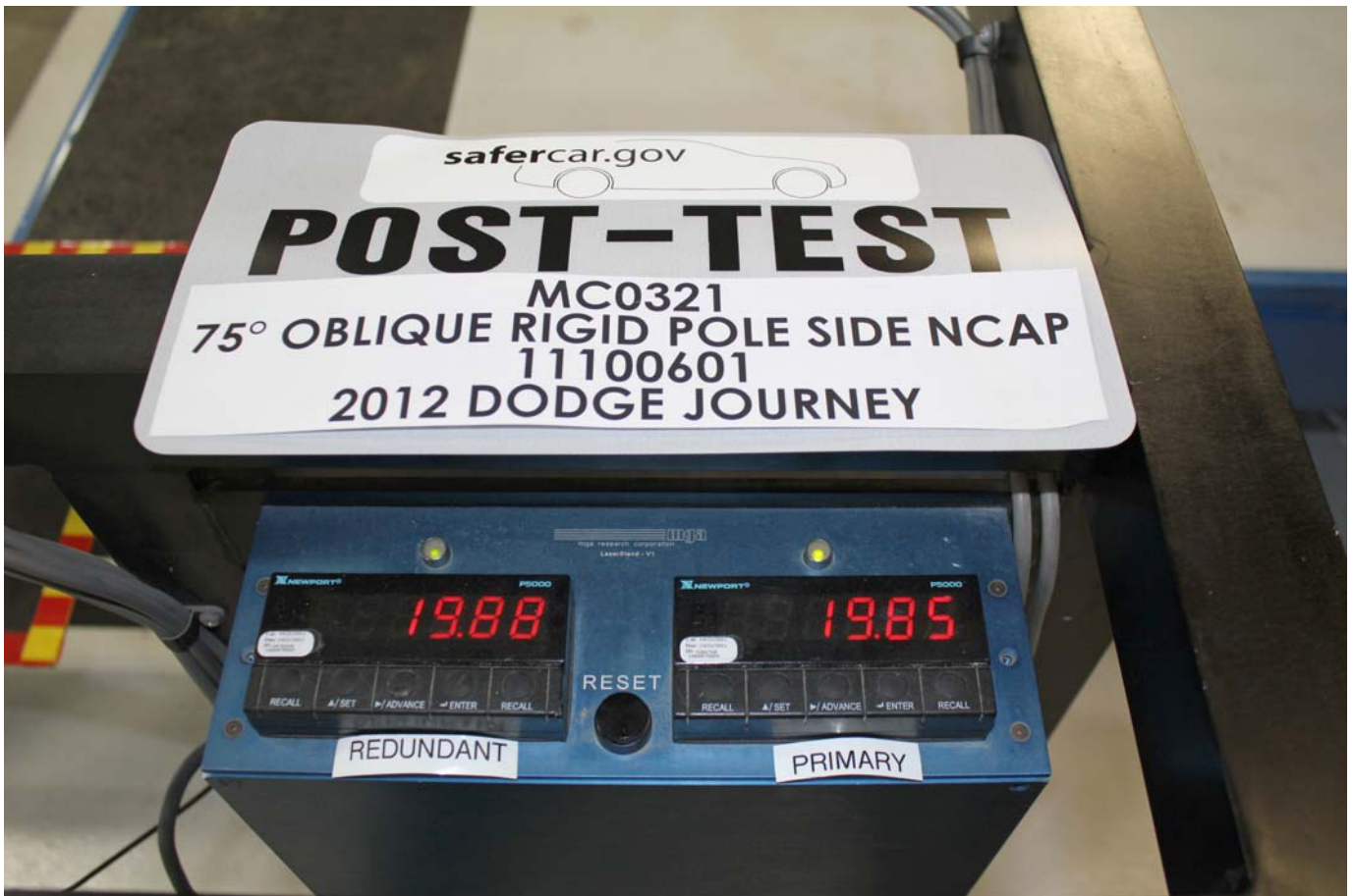
Post-Test Primary and Redundant Speed Trap Read-Out
