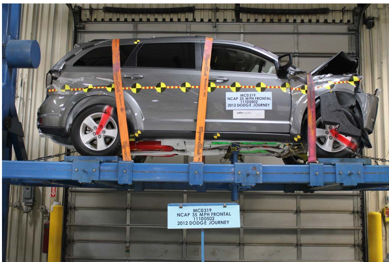
Vehicle at 0 Degrees on Static Rollover Device
