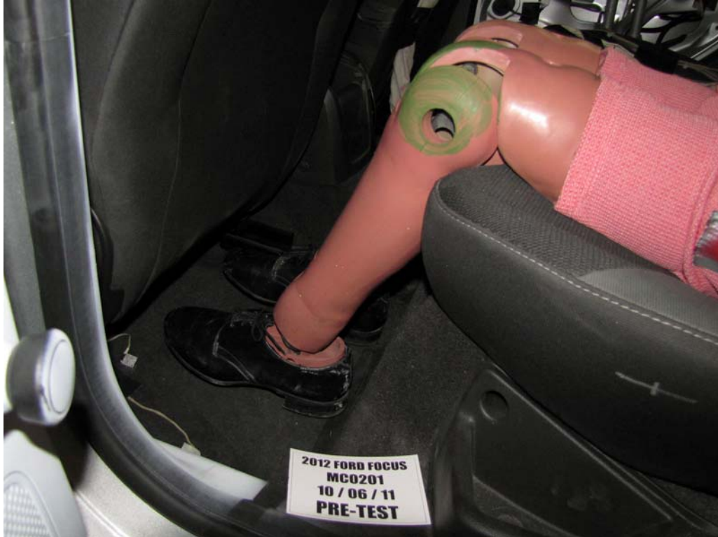
FIGURE 63. Pre-Test Placement of Rear Passenger Dummy's Feet
