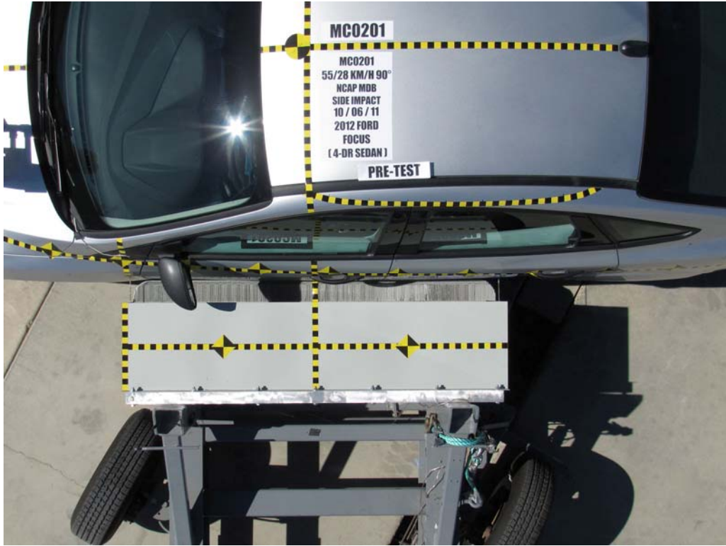
FIGURE 15. Pre-Test Overhead View of Test Area
