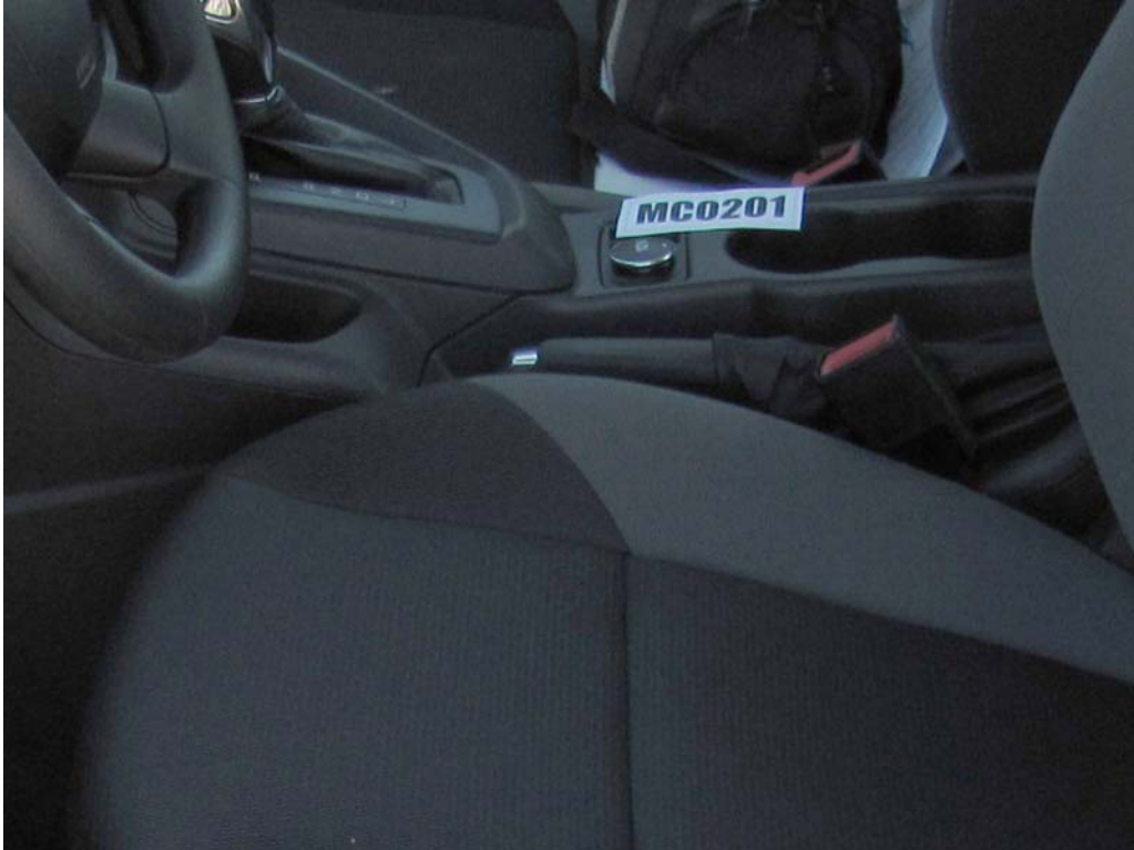
FIGURE 37. View of Disengaged Parking Brake
