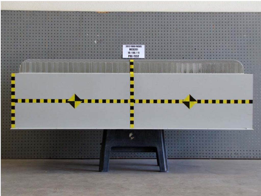
FIGURE 84. Pre-Test Top View of MDB Impactor Face
