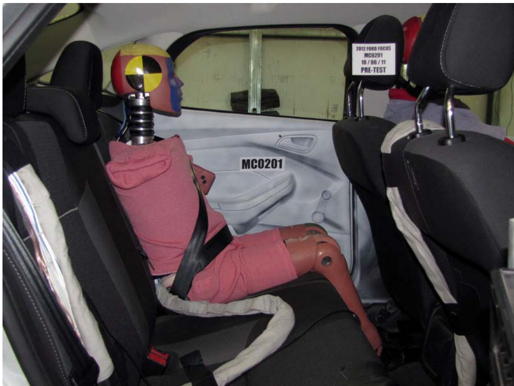
FIGURE 70. Pre-Test Right Side View of Rear Passenger Dummy and Rear Seat Occupant Compartment
