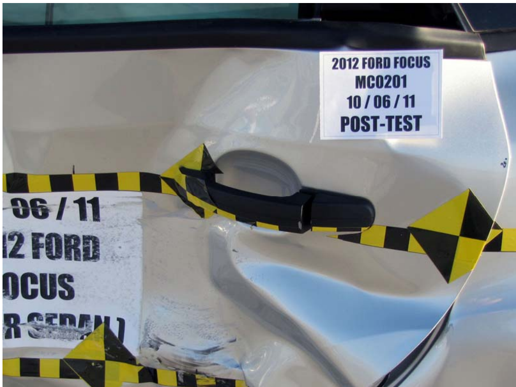
FIGURE 24. Post-Test Left Rear Door Latch Close-Up
