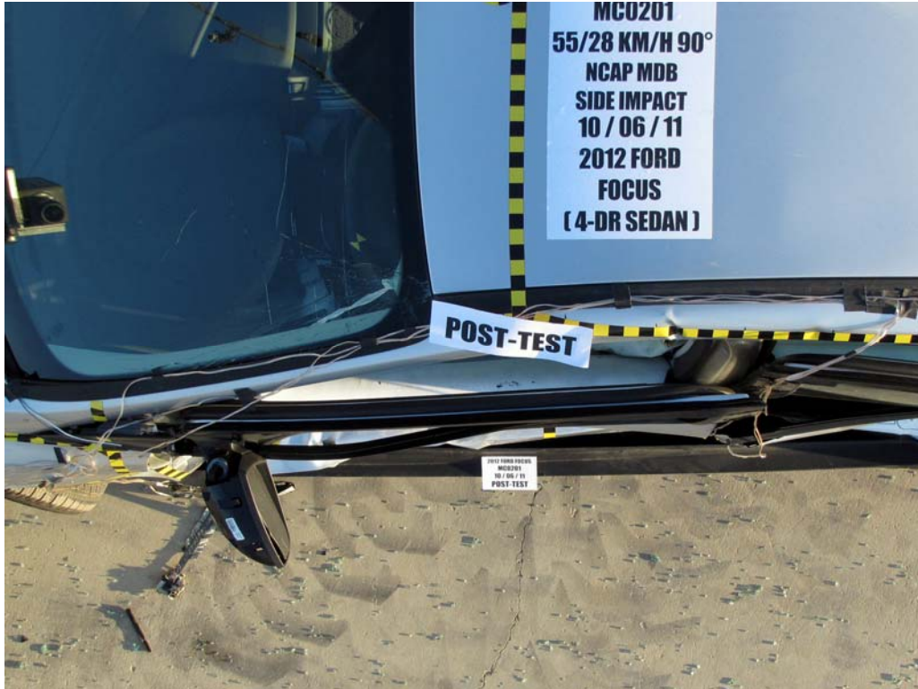
FIGURE 43. Post-Test Driver Dummy and Door Clearance View
