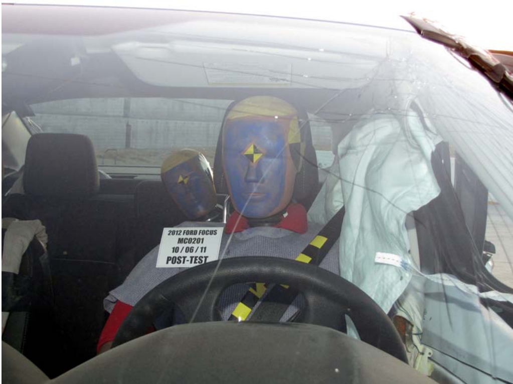
FIGURE 26. Post-Test Front Close-Up View of Driver Dummy
