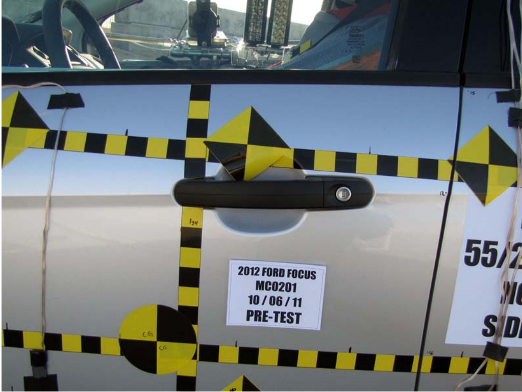
FIGURE 21. Pre-Test Left Front Door Latch Close-Up
