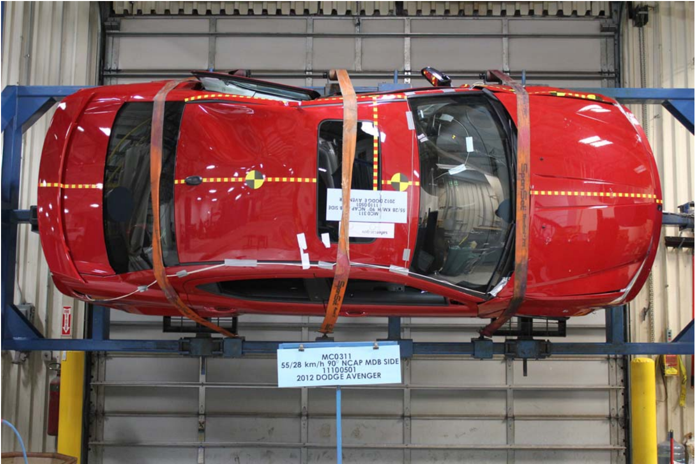
FMVSS No. 301 Static Rollover 270 Degrees
