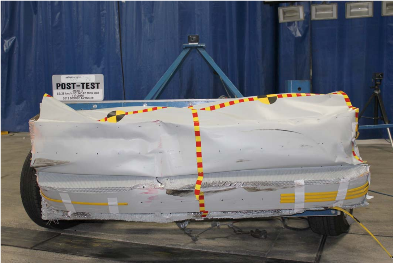
Post-Test Front View of MDB Impactor Face
