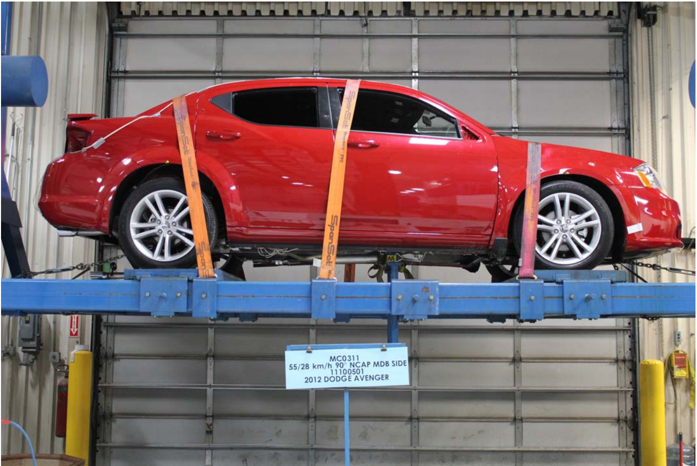
FMVSS No. 301 Static Rollover 0 Degrees
