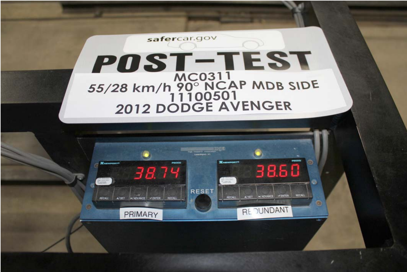
Post-Test Primary and Redundant Speed Trap Read-Out
