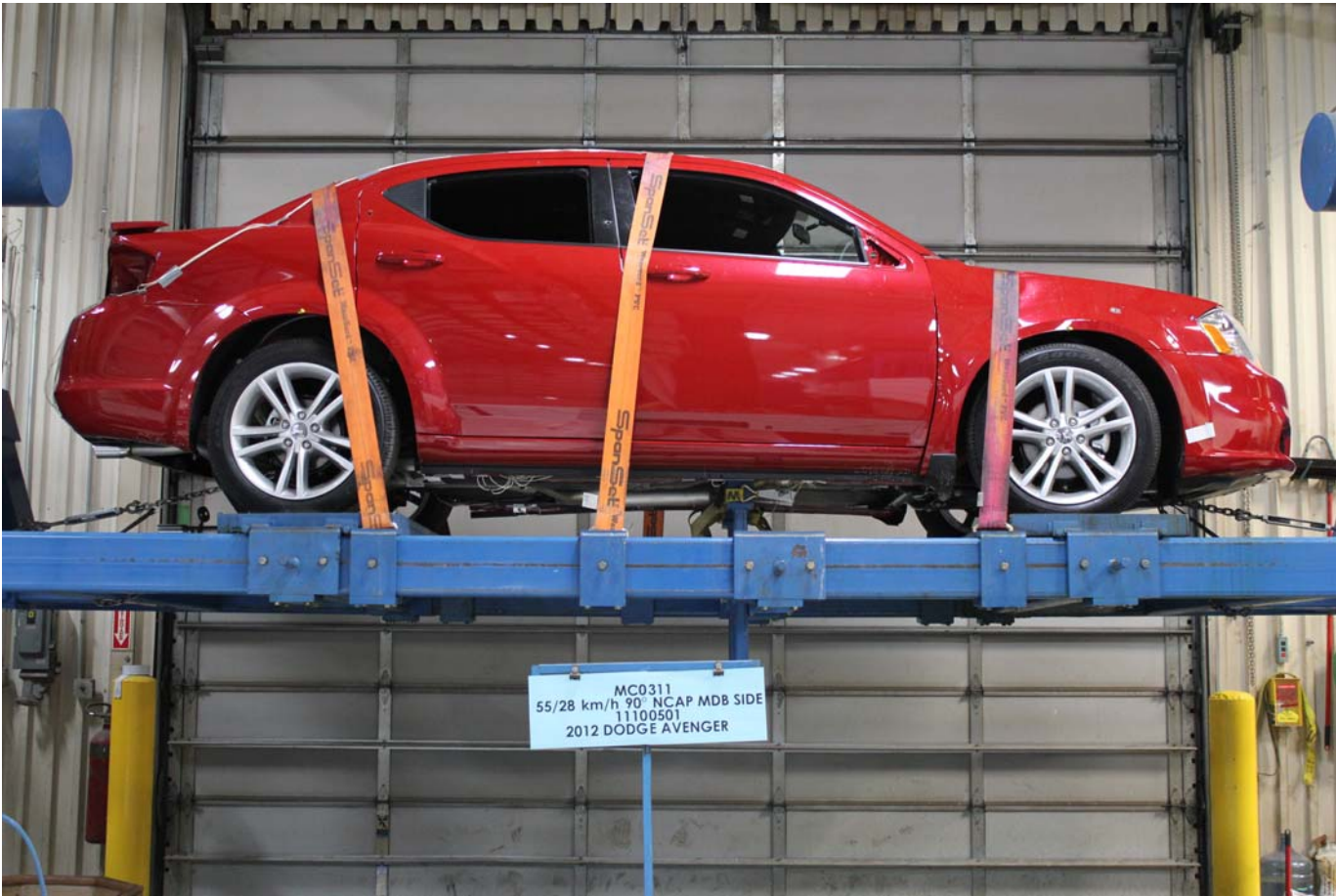
FMVSS No. 301 Static Rollover 360 Degrees
