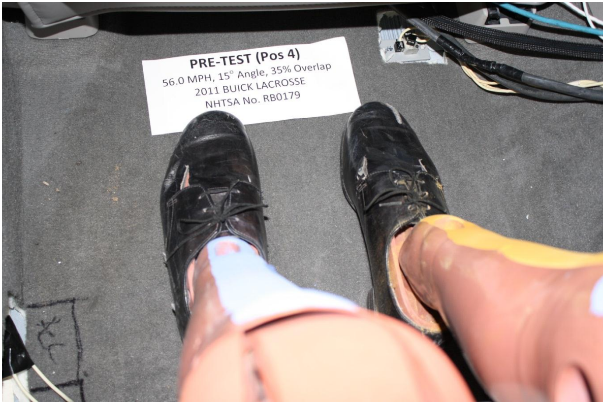
No. 098 Pre-Test View of Passenger Dummy Feet
