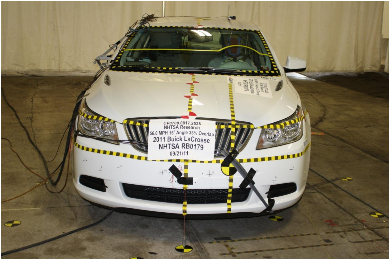
No. 005 Pre-Test Front View of Test Vehicle
