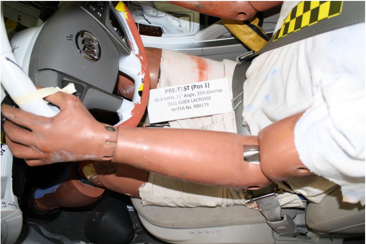
No. 077 Pre-Test View of Driver Dummy Abdomen
