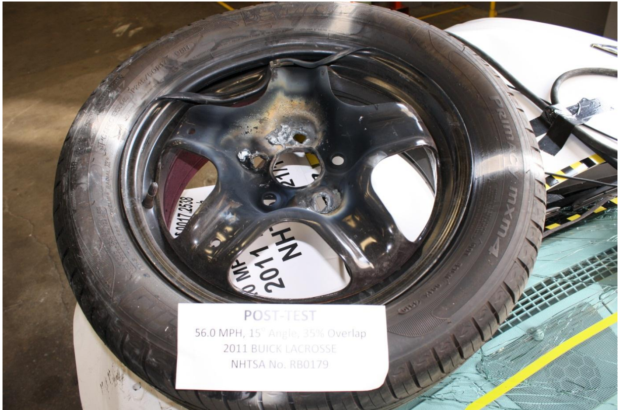
No. 125 Post-Test View of Wheel and or Tire Deformation
