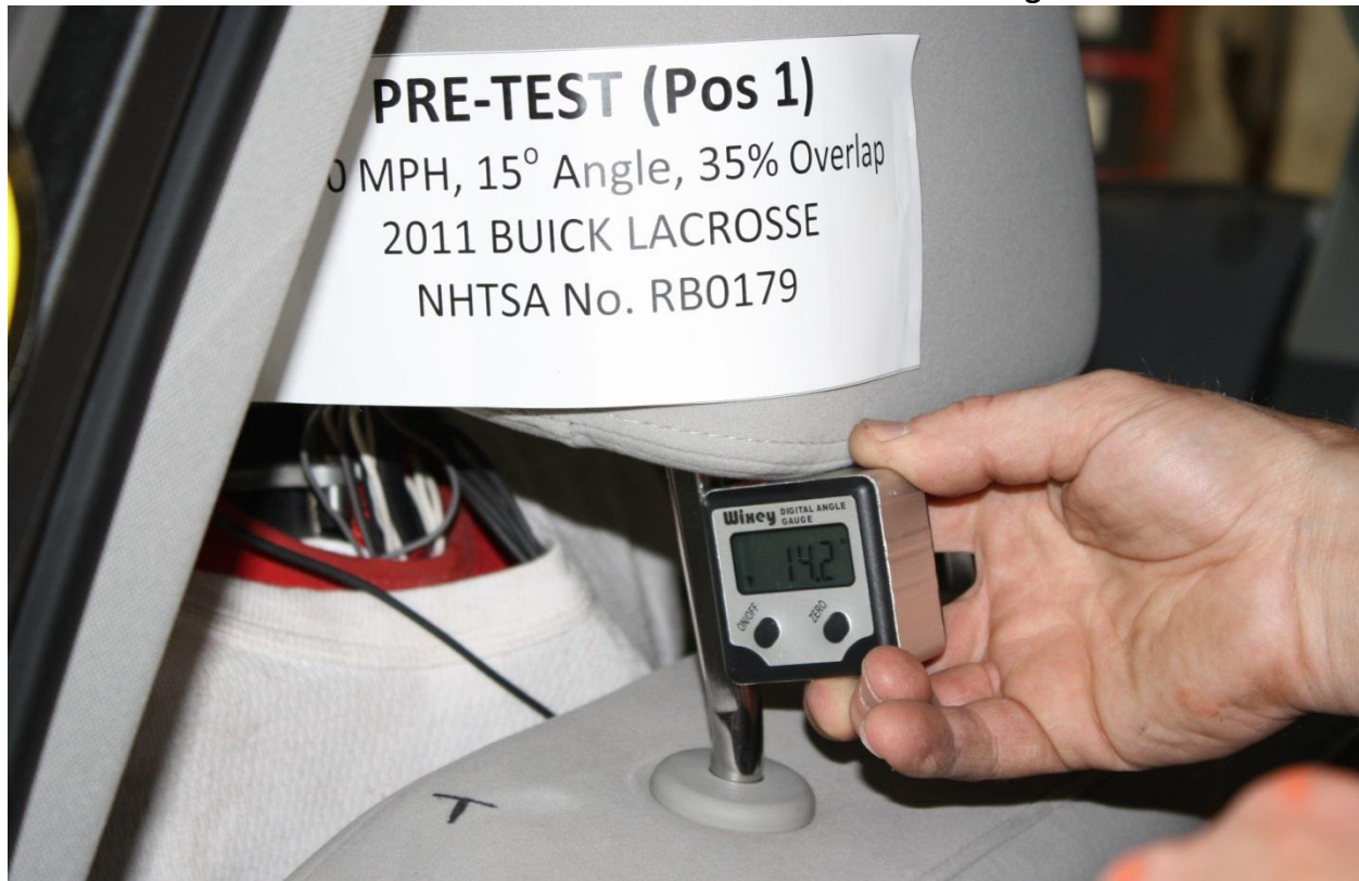
No. 065 Pre-Test Driver Seat Back Position with Level or Inclinator
