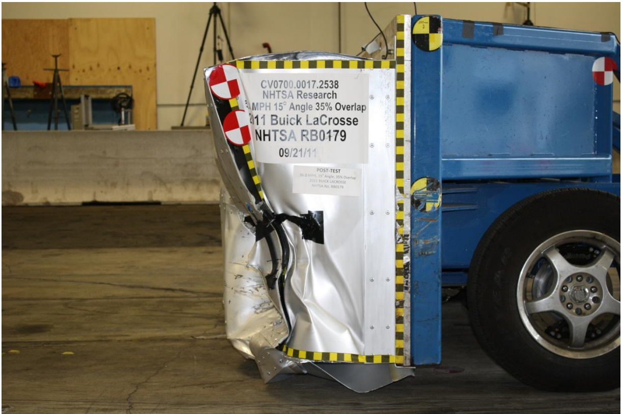
No. 129 Post-Test Left Side View of RMVB
