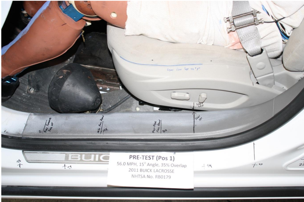
No. 066 Pre-Test Driver Seat Fore Aft Markings
