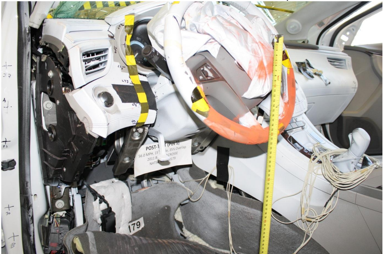
No. 045 Post-Test Left Side View of Driver Knee Bolsters with panel removed
