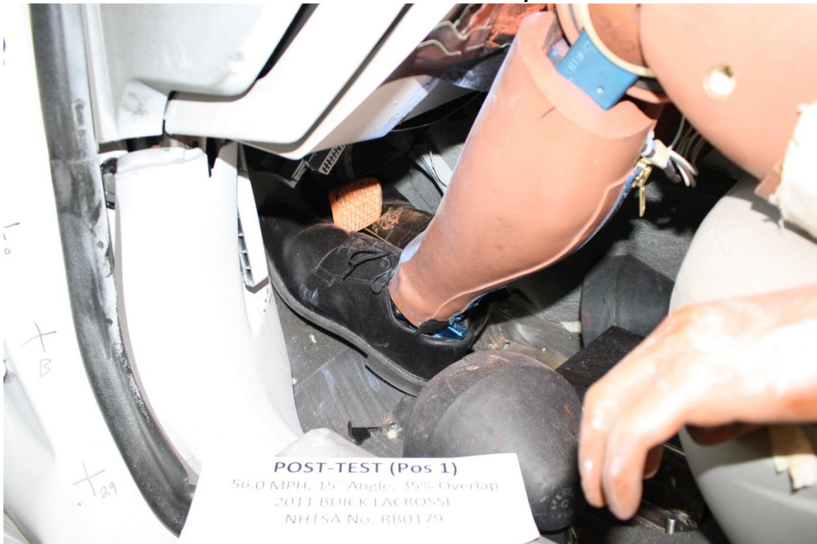
No. 072 Post-Test Driver Dummy Feet
