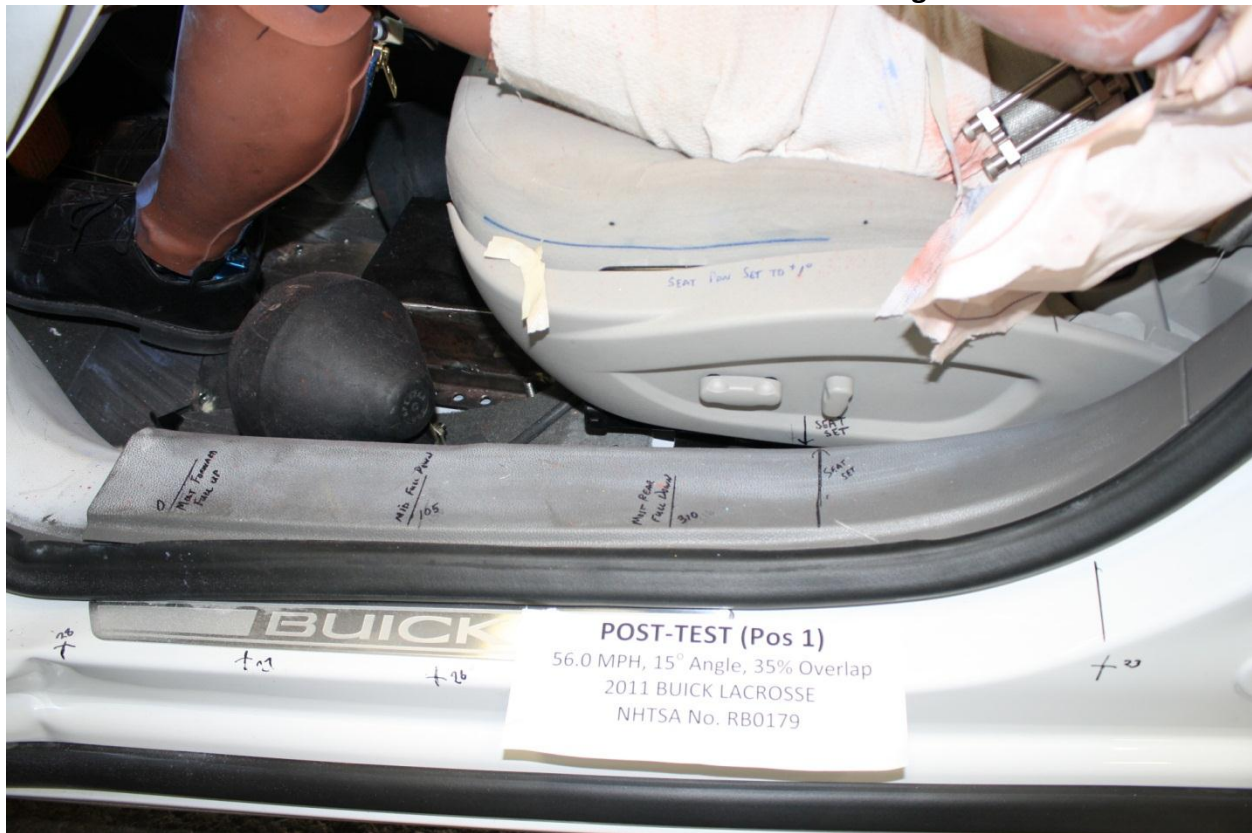
No. 067 Post-Test Driver Seat Fore Aft Markings
