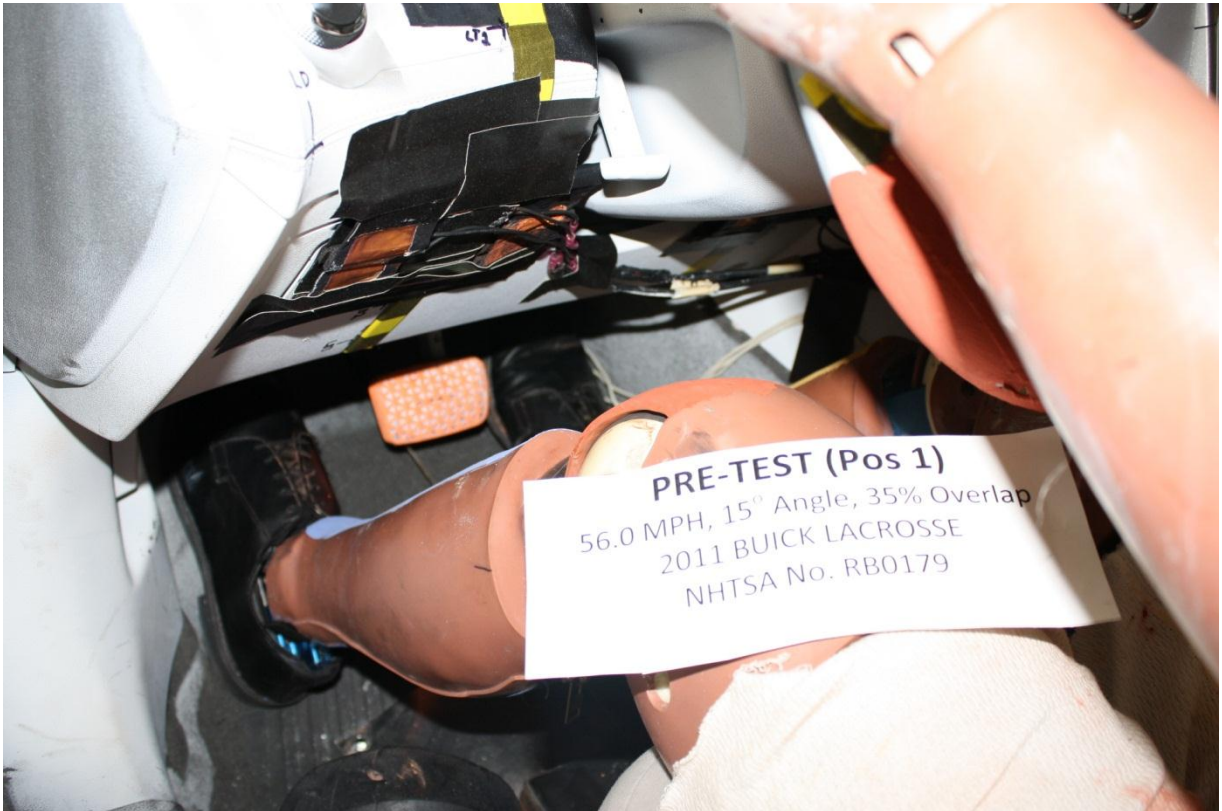
No. 075 Pre-Test View of Driver Dummy Left Knee and Bolster
