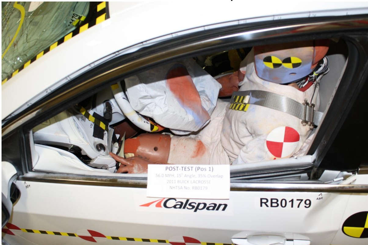
No. 063 Post-Test View of Driver Dummy Door Clearance
