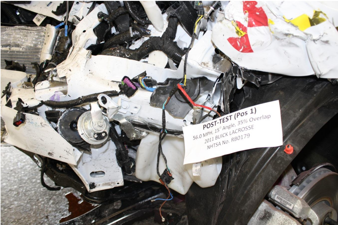
No. 118 Post-Test Frame Rail with tire removed
