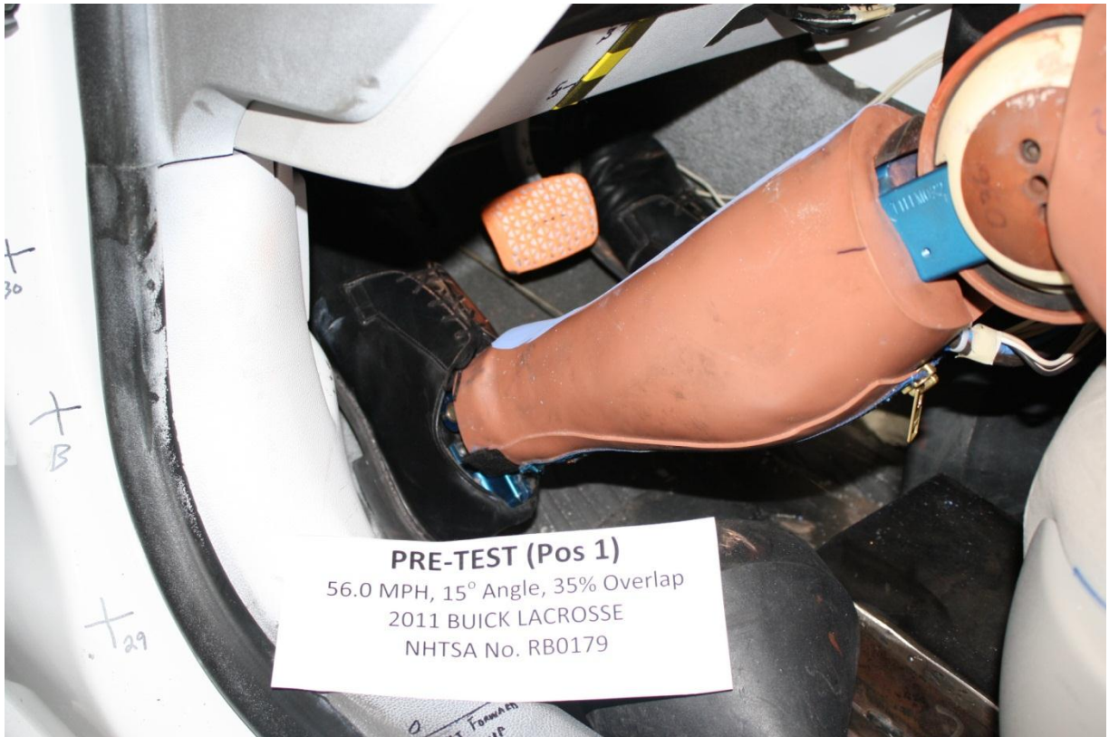
No. 071 Pre-Test Driver Dummy Feet
