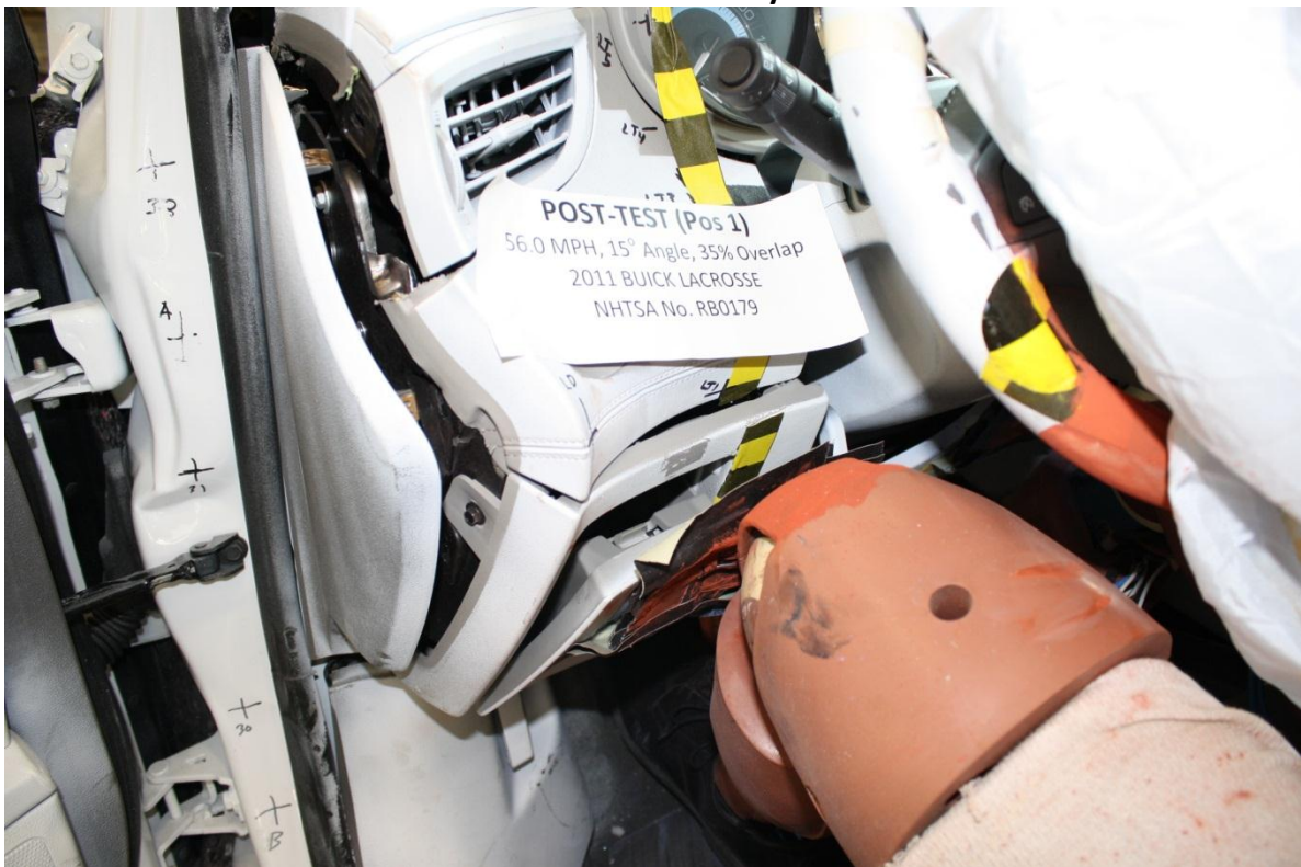
No. 076 Post-Test View of Driver Dummy Left Knee and Bolster
