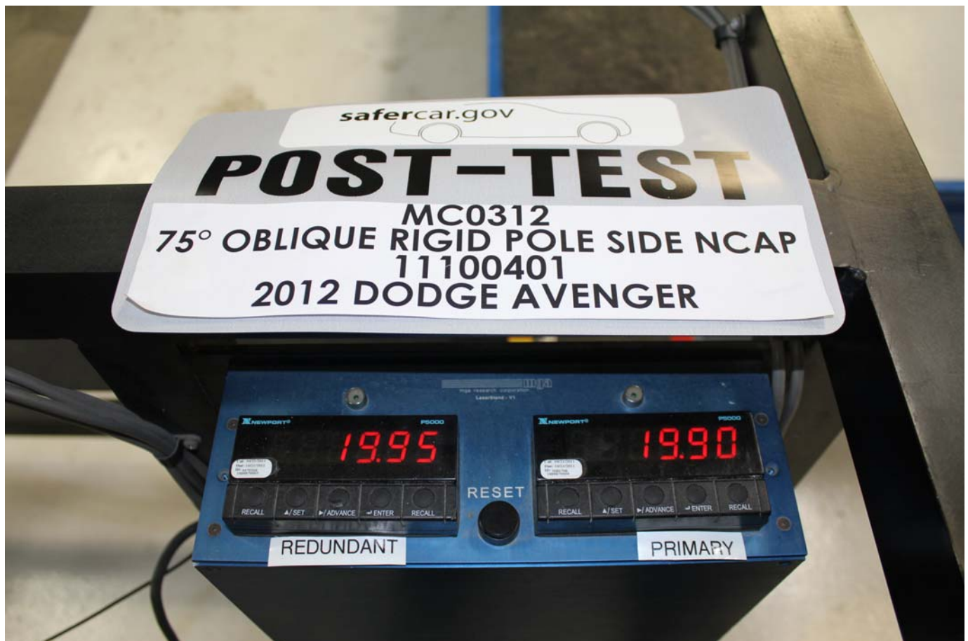
Post-Test Primary and Redundant Speed Trap Read-Out
