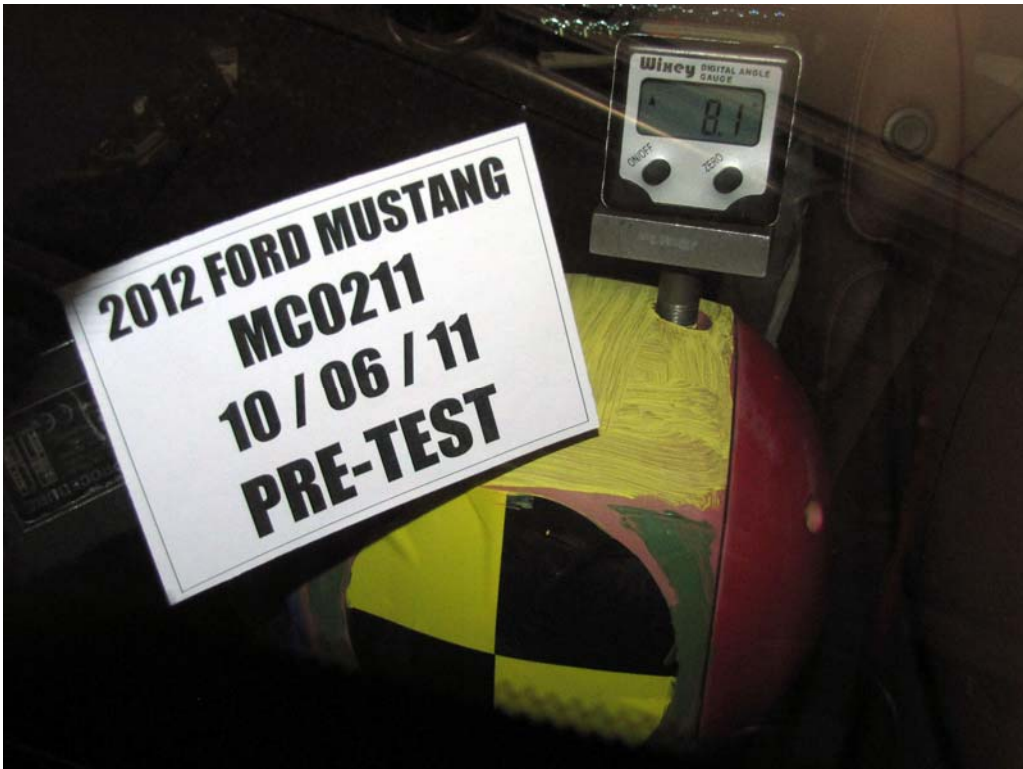
FIGURE 62. Pre-Test View of Rear Passenger Dummy's Head Showing Dummy's Head is Level
