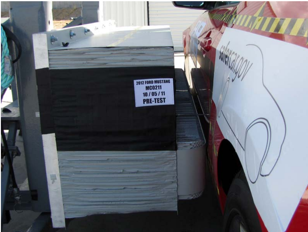
FIGURE 18. Pre-Test Right Side View of MDB Positioned Against Side of Test Vehicle at Ideal Impact Point
