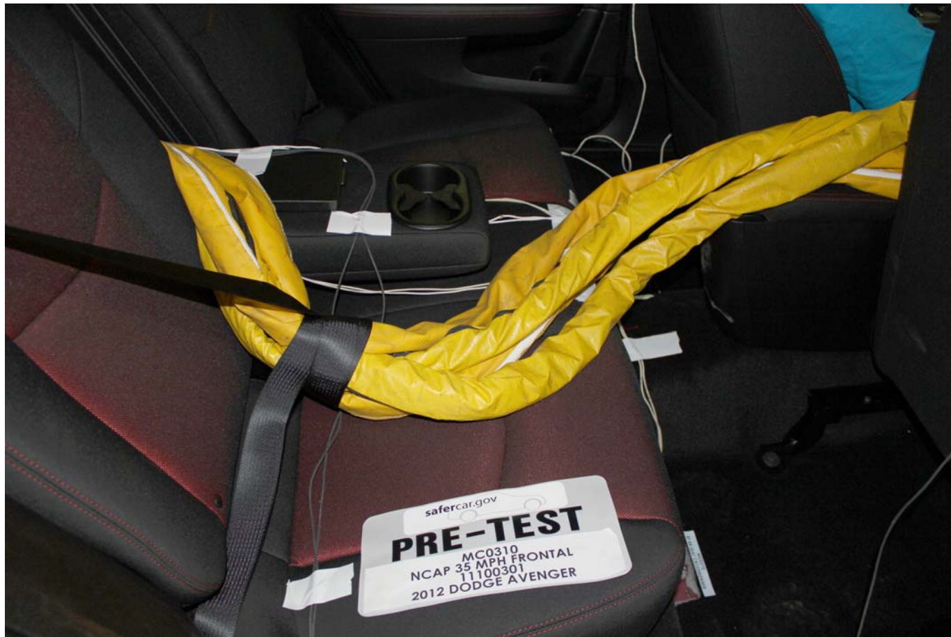
Pre-Test Dummy Cable Routing
