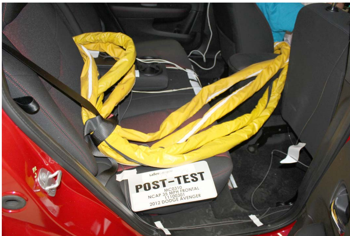
Post-Test Dummy Cable Routing
