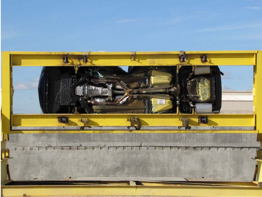
FIGURE 65. FMVSS No. 301-305 Rollover 270 Degrees
