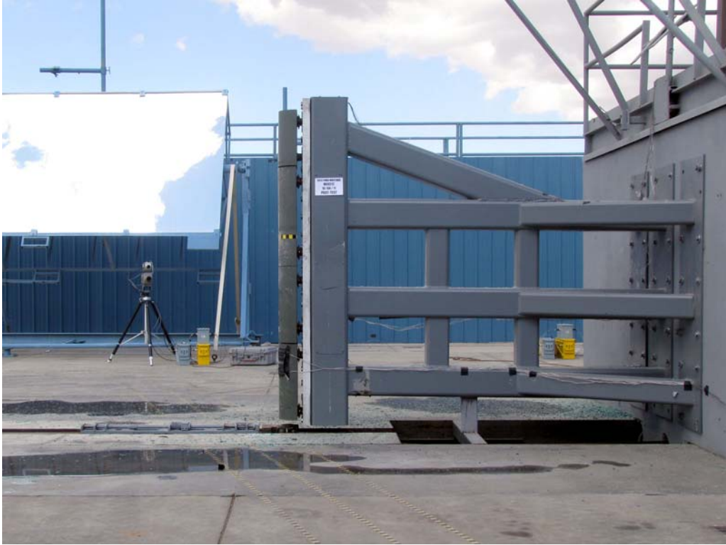
FIGURE 59. Post-Test Pole Barrier Side View
