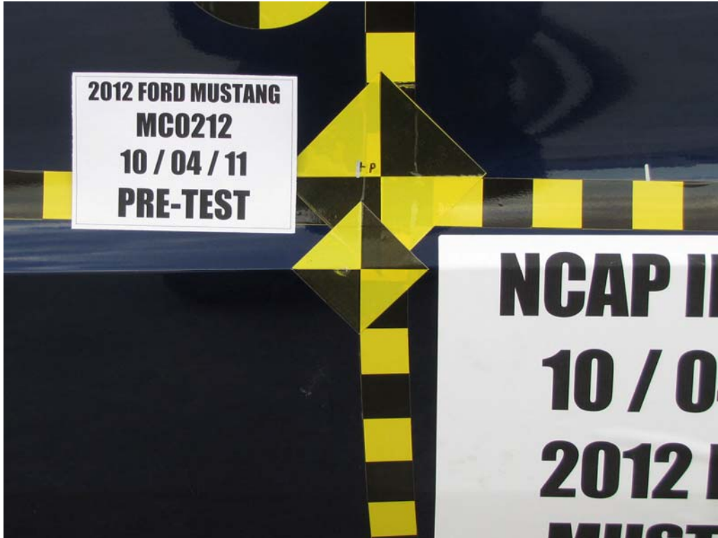
FIGURE 19. Pre-Test Close-Up View of Impact Point Target
