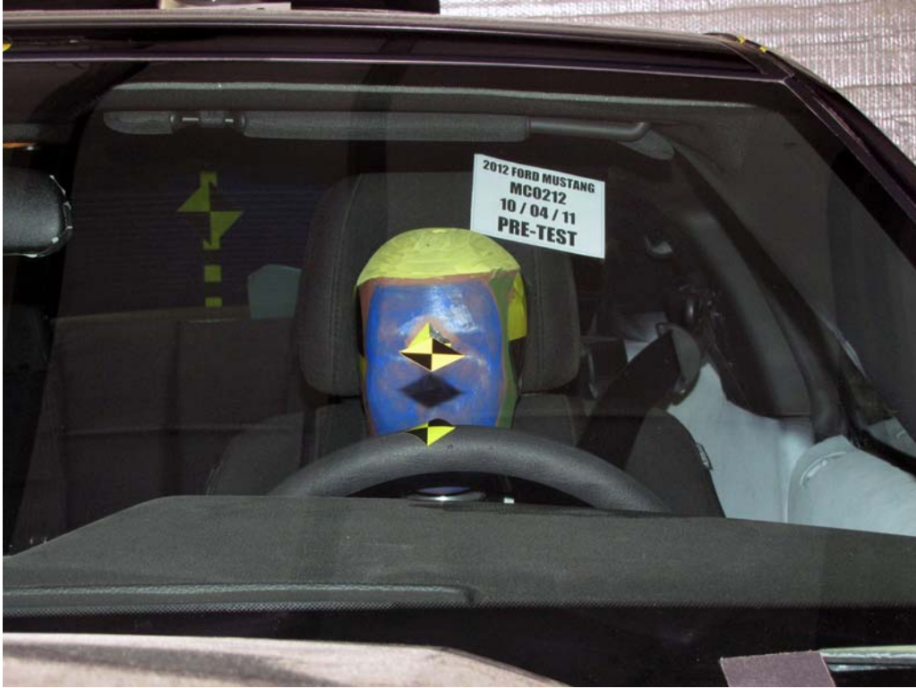
FIGURE 27. Pre-Test Frontal View of Dummy Head and Shoulders in Relation to Head Restraint
