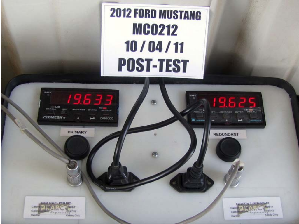
FIGURE 61. Post-Test Primary and Redundant Speed Trap Read-Out
