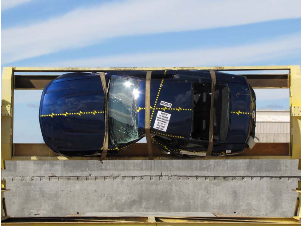
FIGURE 63. FMVSS No. 301-305 Rollover 90 Degrees
