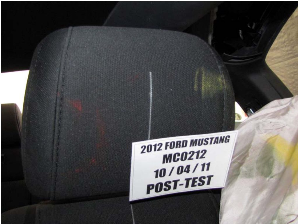
FIGURE 46. Post-Test Dummy Close-Up Head Contact with Vehicle Interior View
