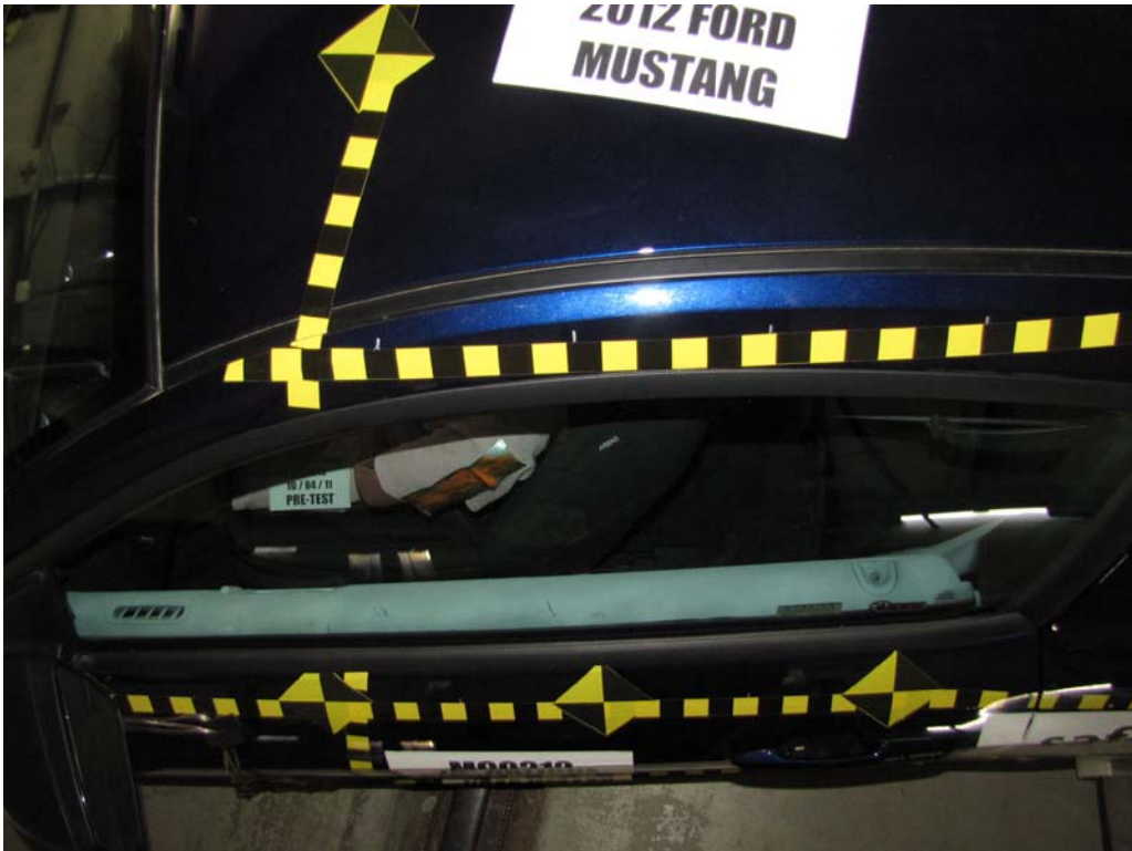
FIGURE 40. Pre-Test Driver Dummy and Door Clearance
