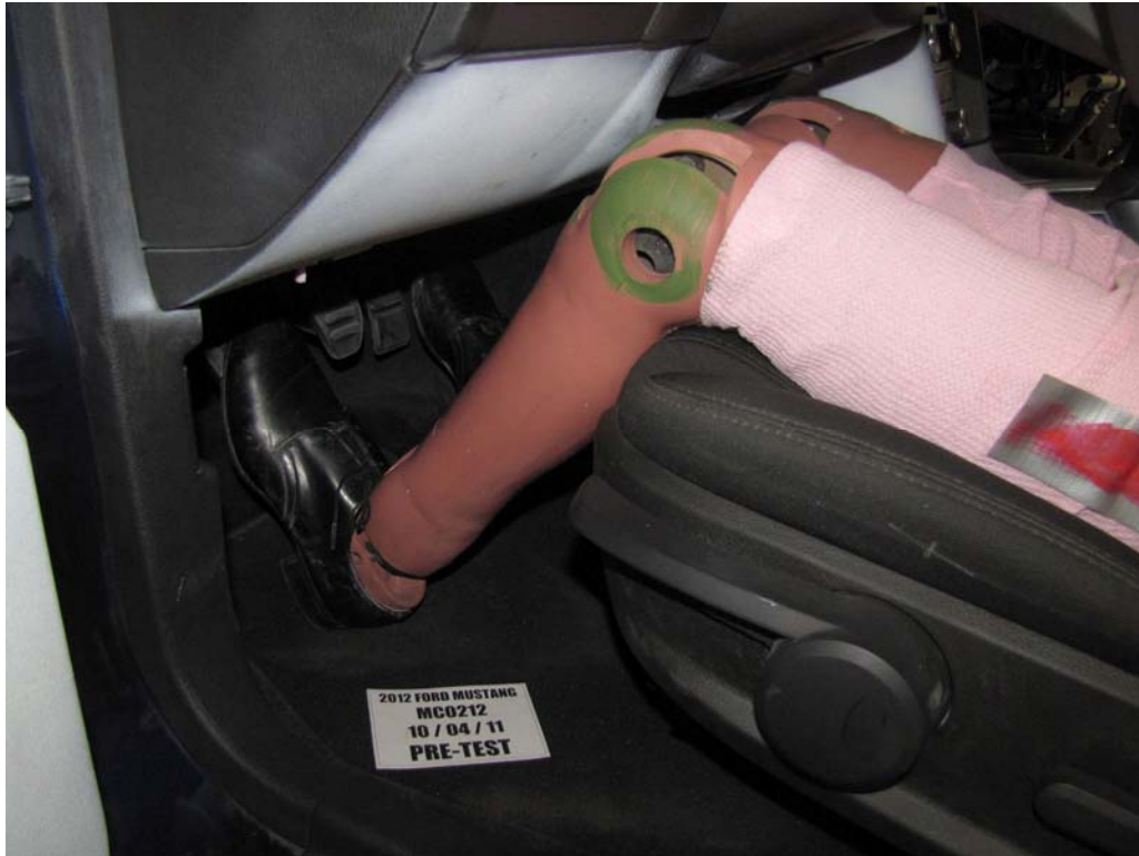
FIGURE 32. Pre-Test Placement of Dummy's Feet
