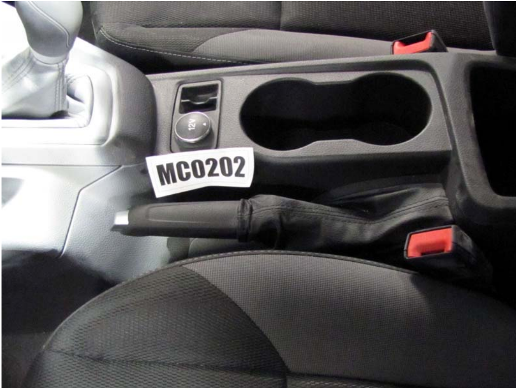
FIGURE 35. View of Disengaged Parking Brake
