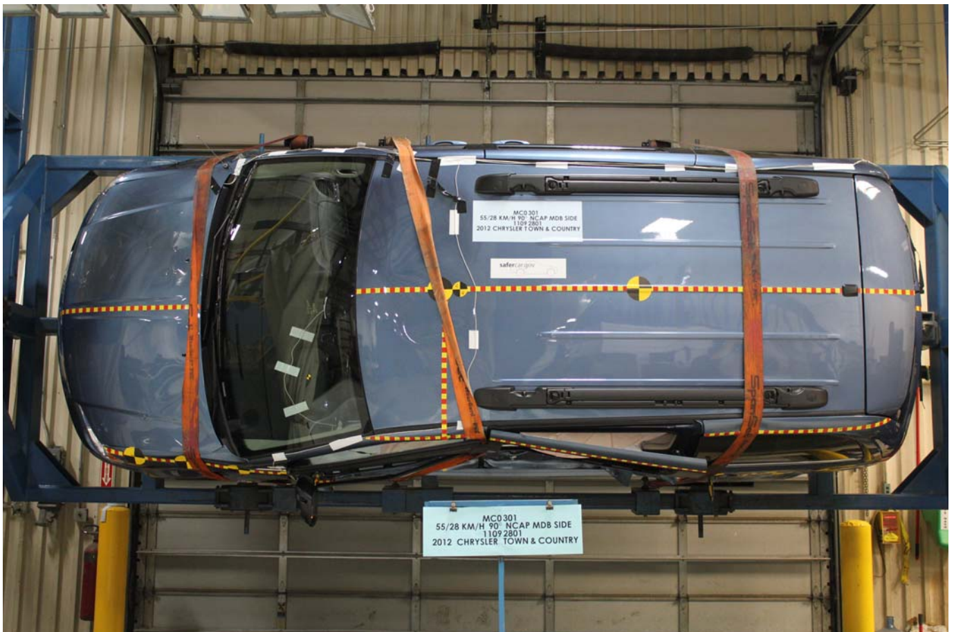
FMVSS No. 301 Static Rollover 90 Degrees
