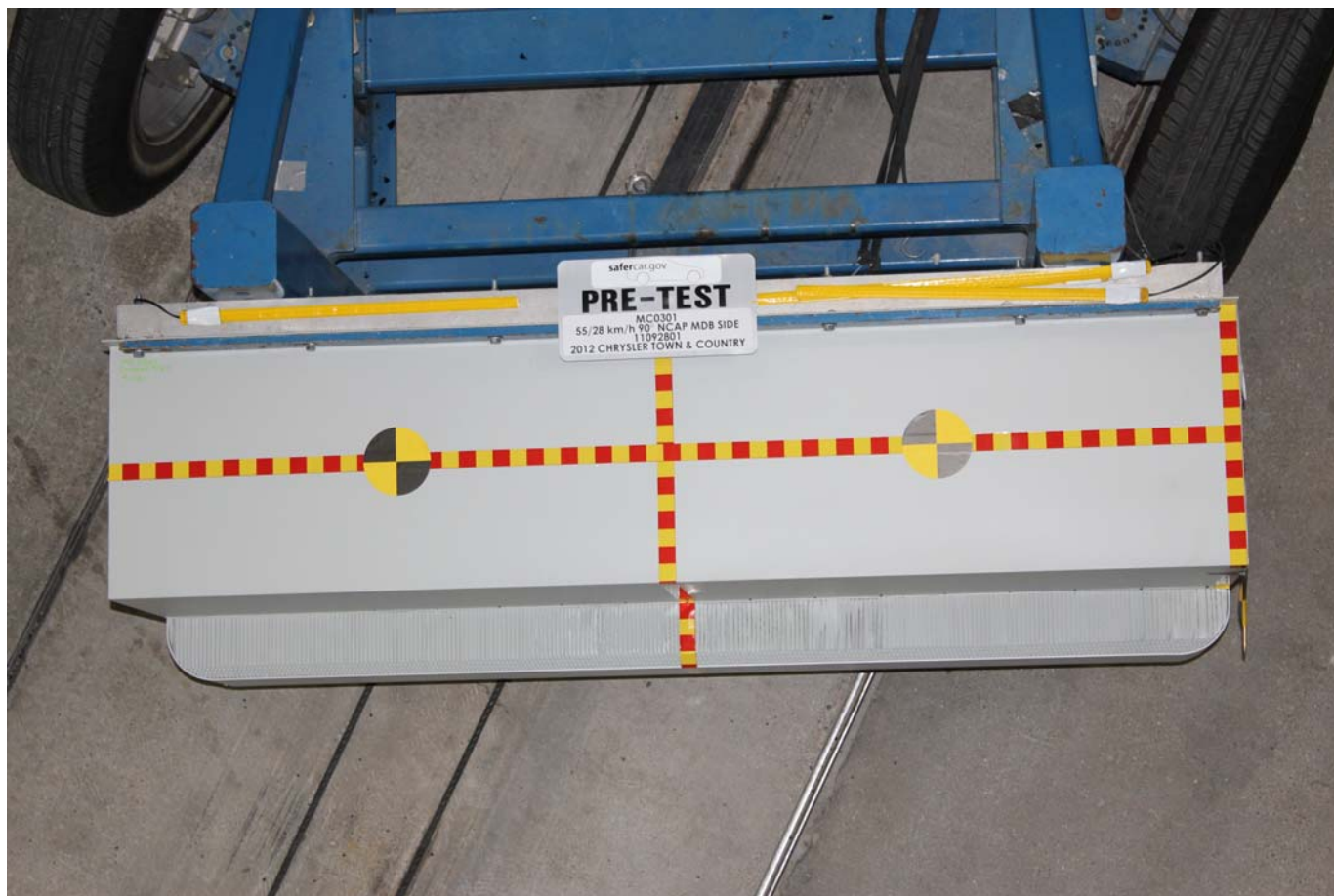
Pre-Test Top View of MDB Impactor Face
