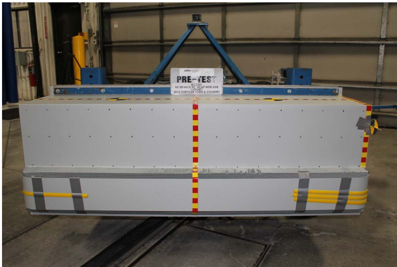
Pre-Test Front View of MDB Impactor Face
