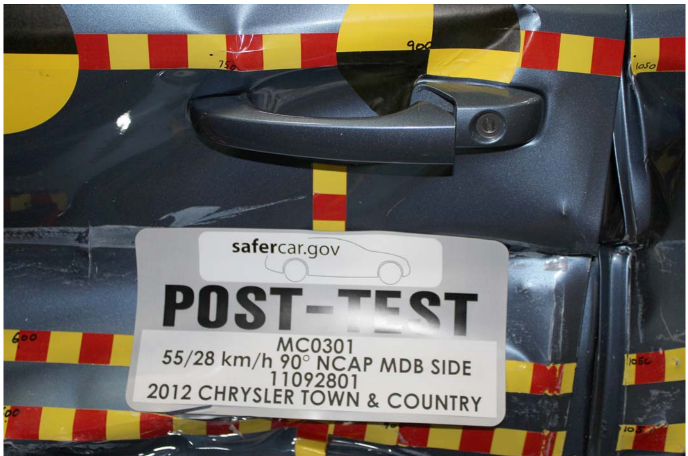
Post-Test Left Front Door Latch Close-Up
