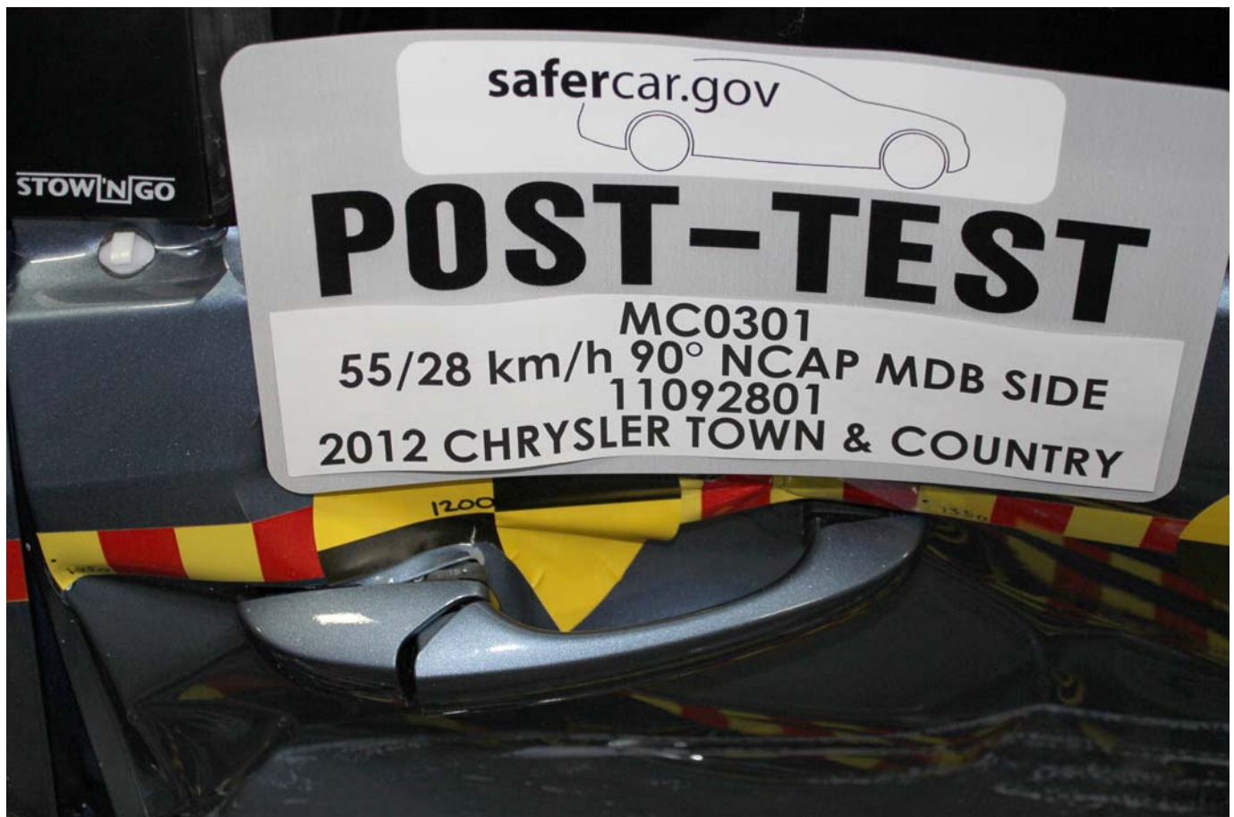
Post-Test Left Rear Door Latch Close-Up
