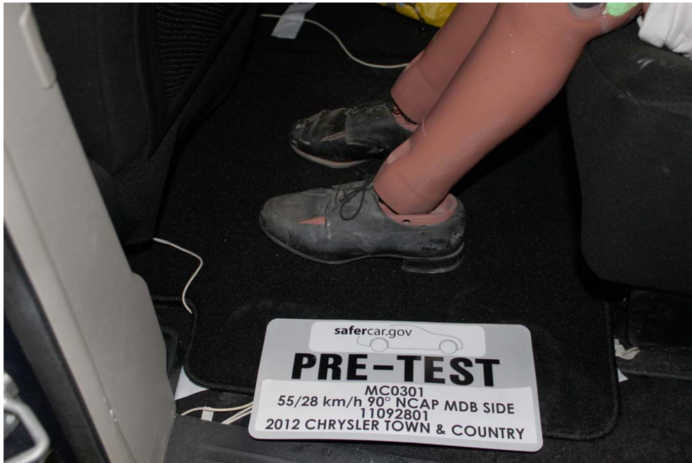
Pre-Test Placement of Rear Passenger Dummy's Feet
