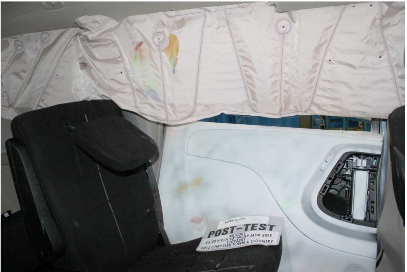
Post-Test Rear Passenger Inner Door Panel View
