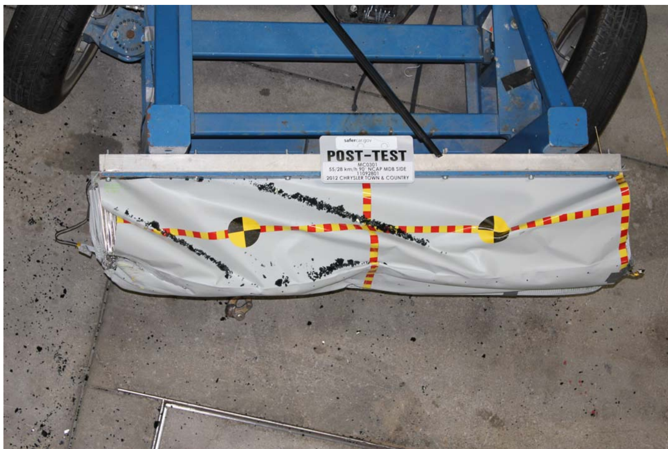
Post-Test Top View of MDB Impactor Face
