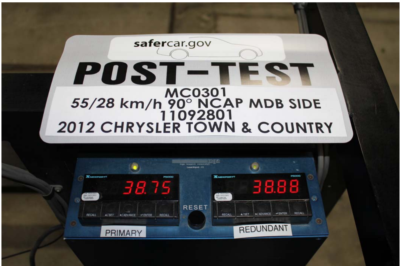
Post-Test Primary and Redundant Speed Trap Read-Out
