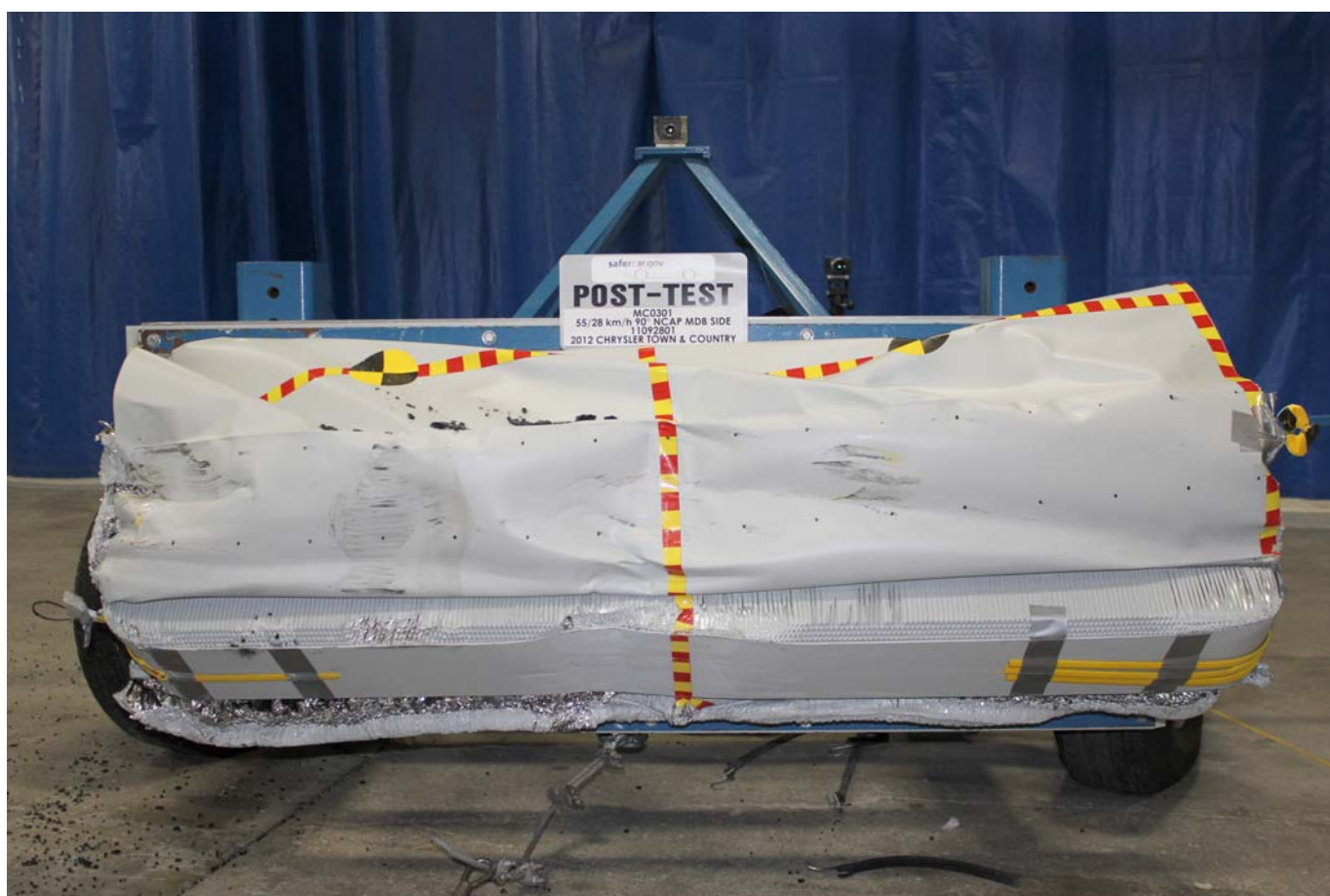
Post-Test Front View of MDB Impactor Face
