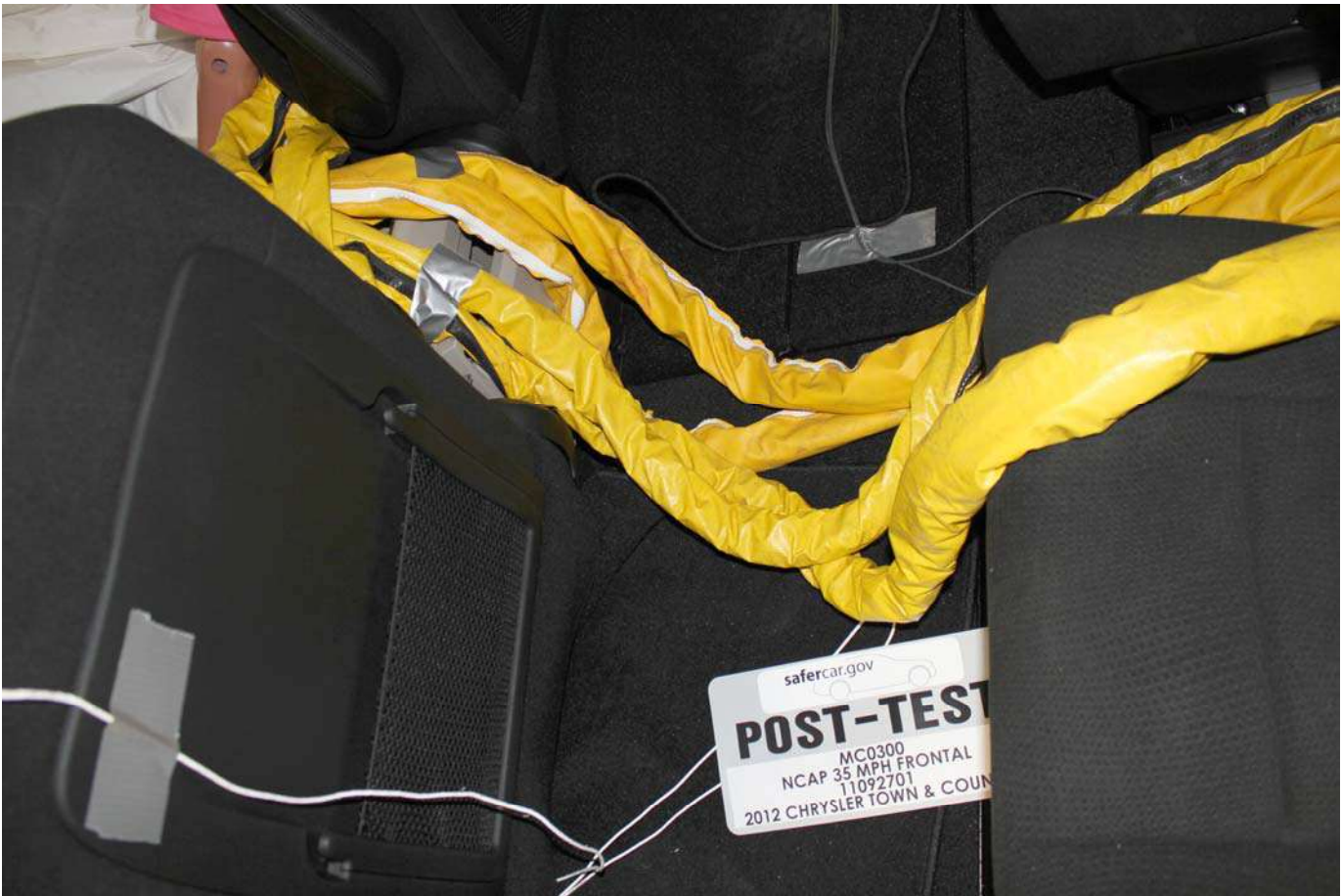
Post-Test Dummy Cable Routing
