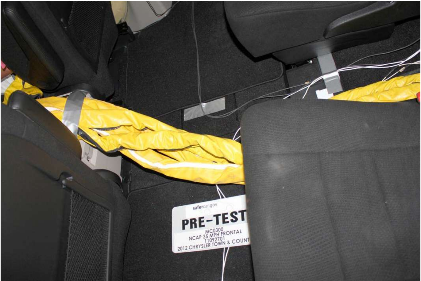
Pre-Test Dummy Cable Routing
