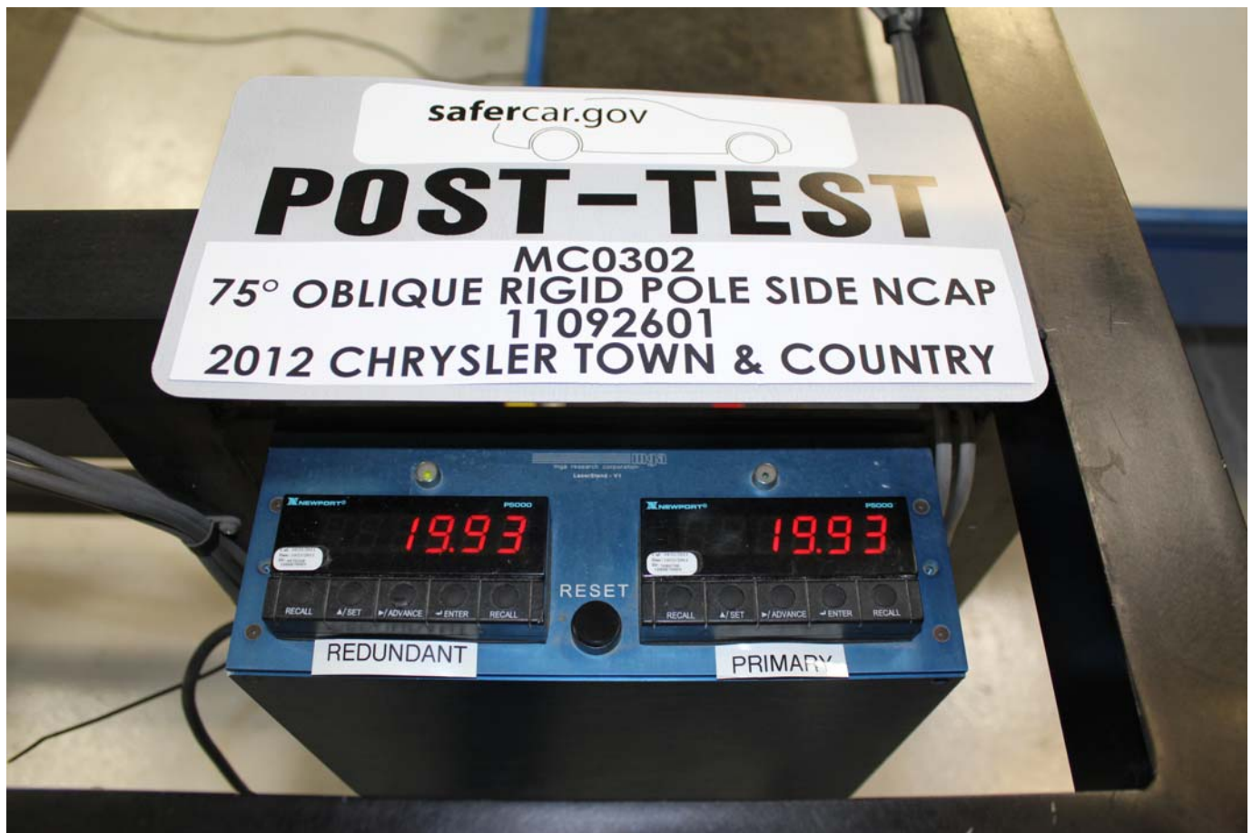
Post-Test Primary and Redundant Speed Trap Read-Out
