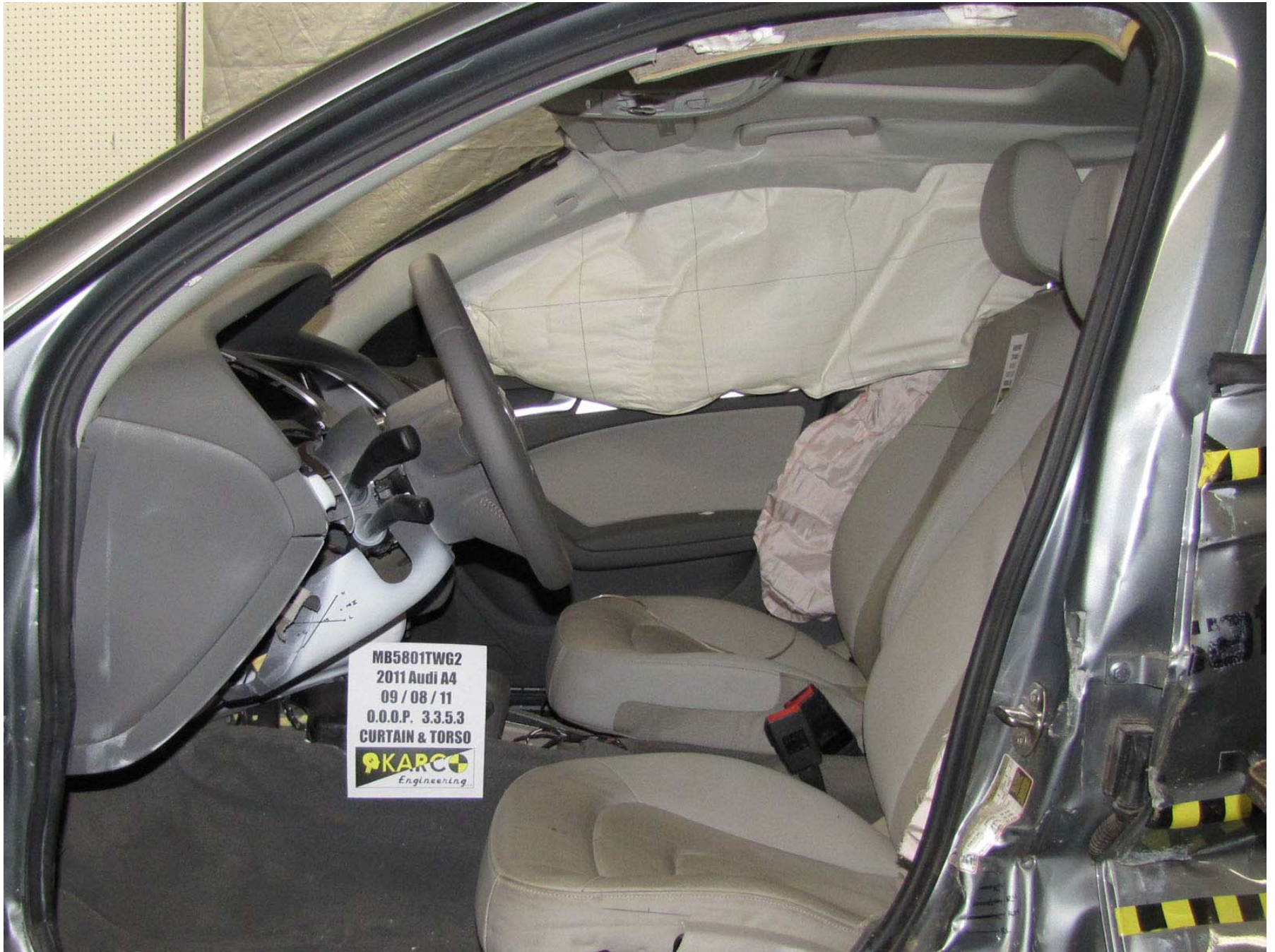
Figure A-9: Post-Test Airbags, Left Side View
