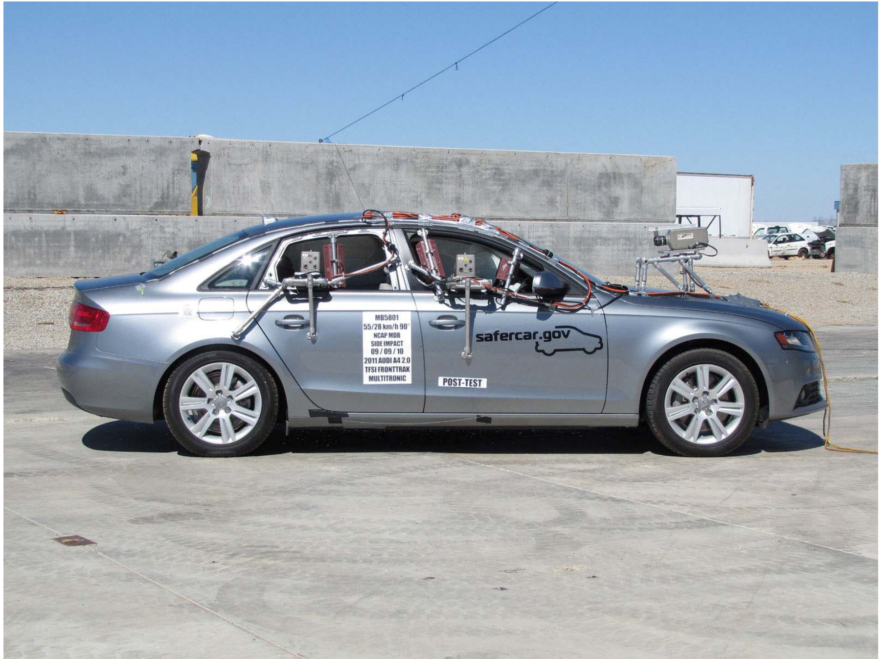
Figure A-4: Post-Test Right Side View of NCAP Side Impact Test
