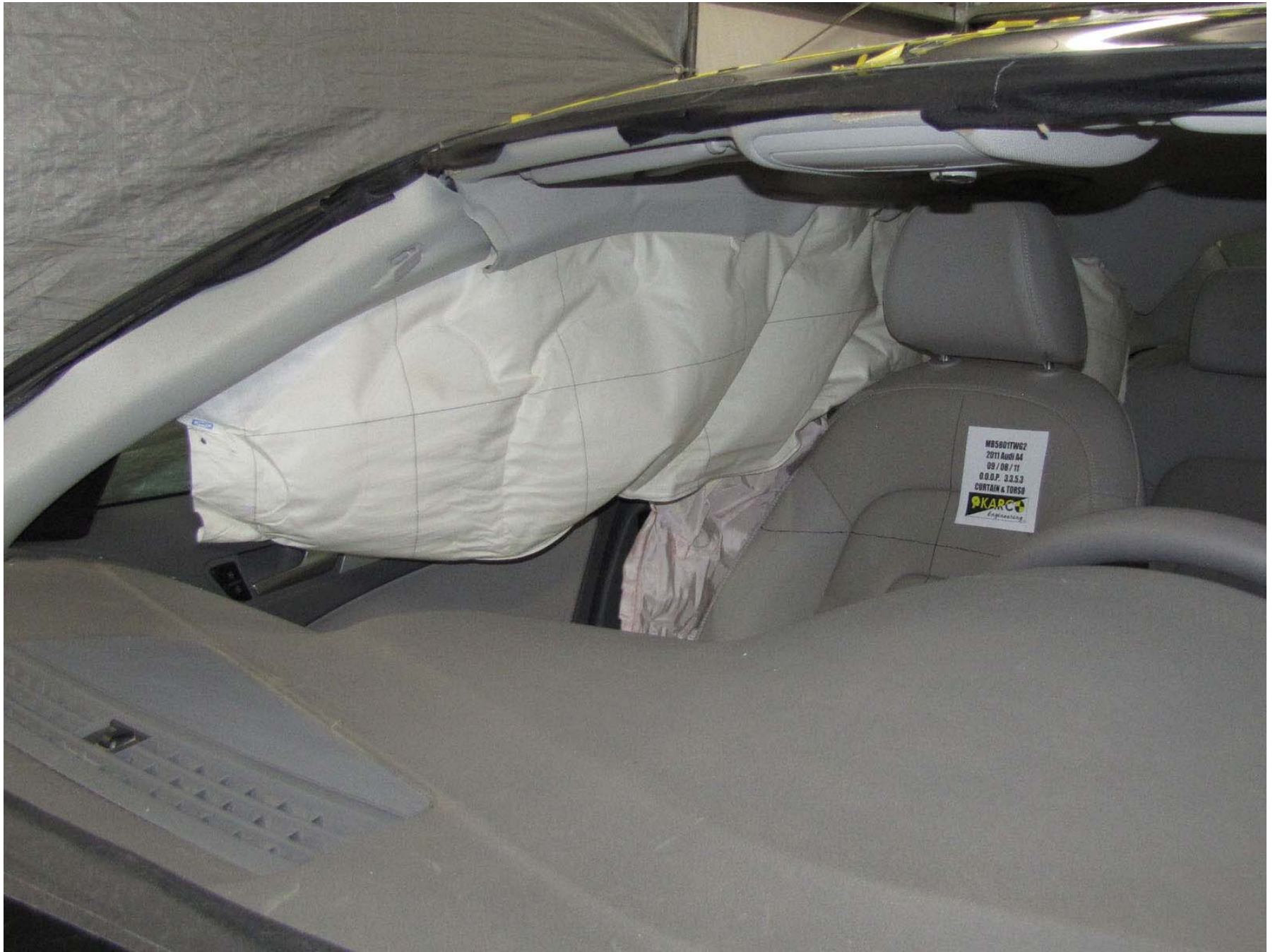
Figure A-10: Post-Test Airbags, Left Front ¾ View
