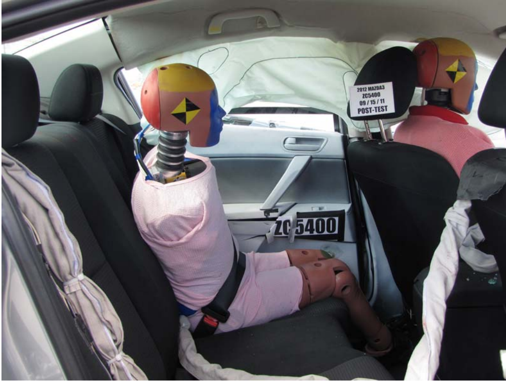
FIGURE 71. Post-Test Right Side View of Rear Passenger Dummy and Rear Seat Occupant Compartment
