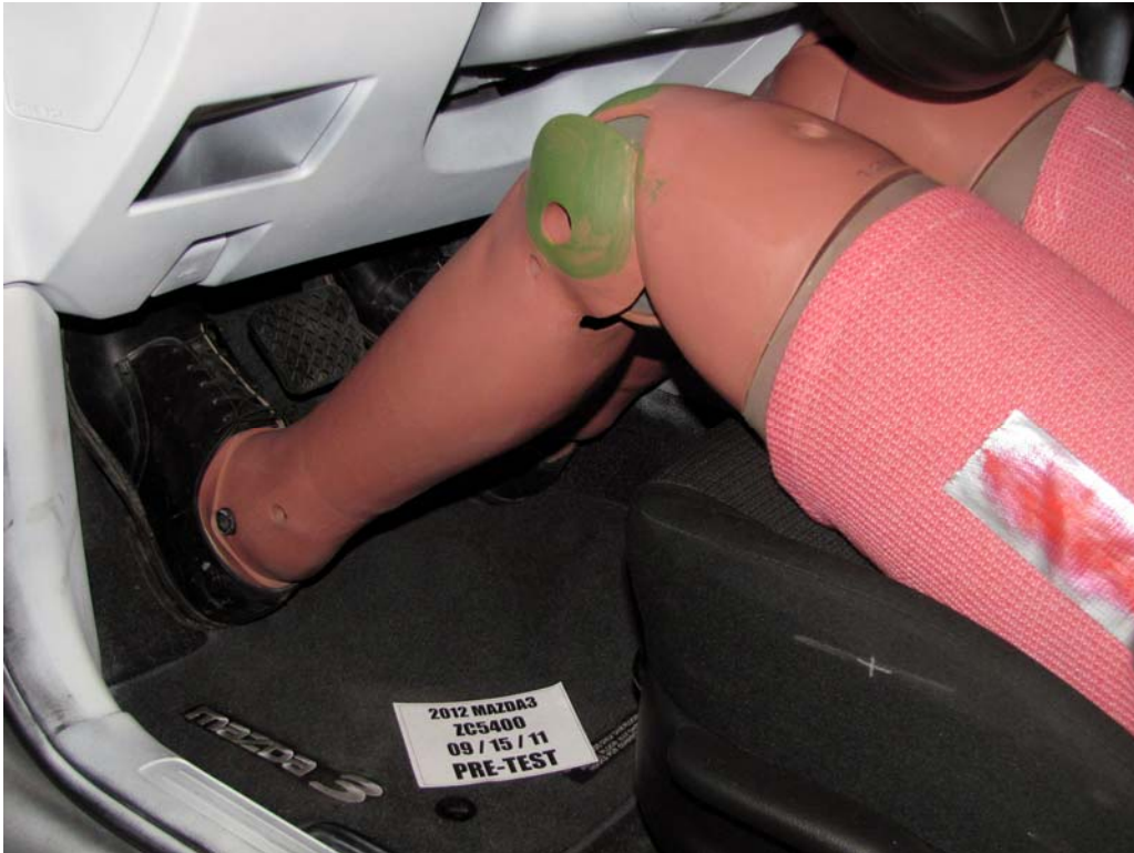
FIGURE 34. Pre-Test Placement of Driver Dummy's Feet
