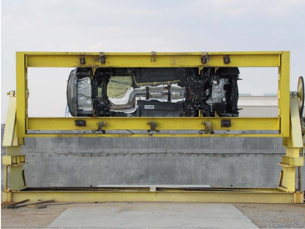
FIGURE 97. FMVSS No. 301 Static Rollover 270 Degrees
