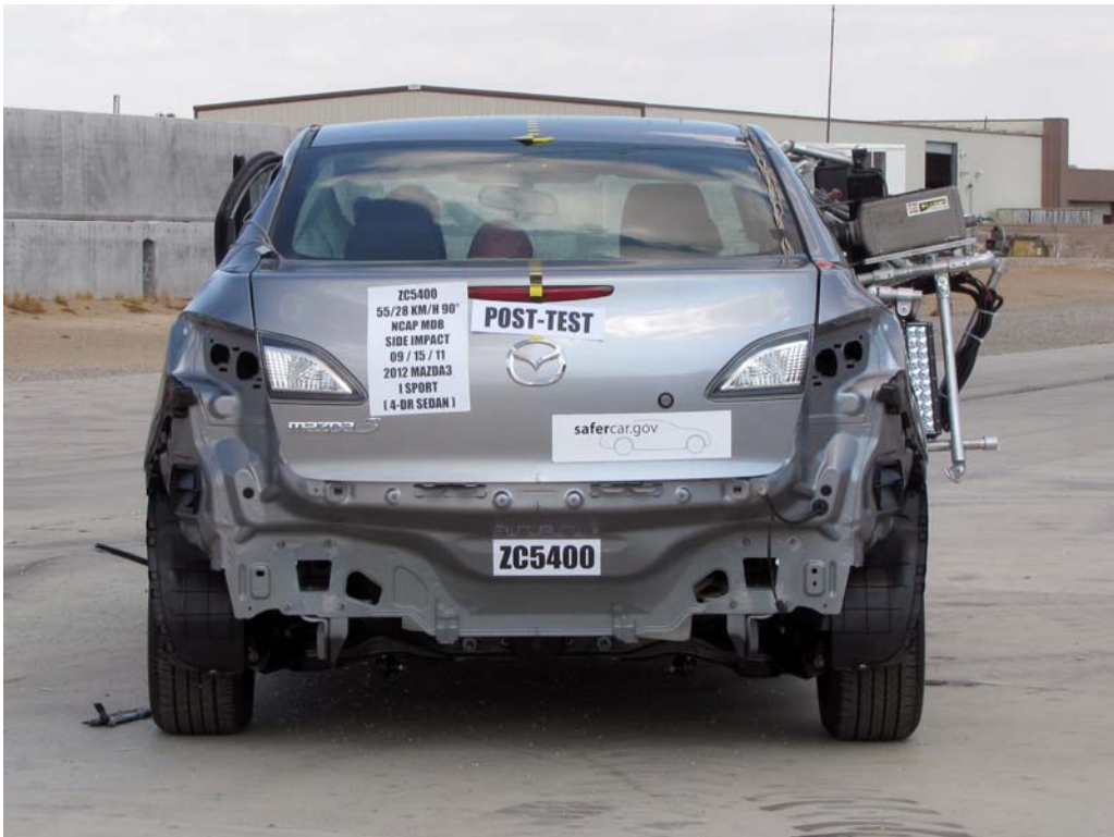
FIGURE 12. Post-Test Rear View of Test Vehicle
