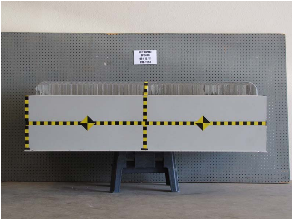
FIGURE 84. Pre-Test Top View of MDB Impactor Face
