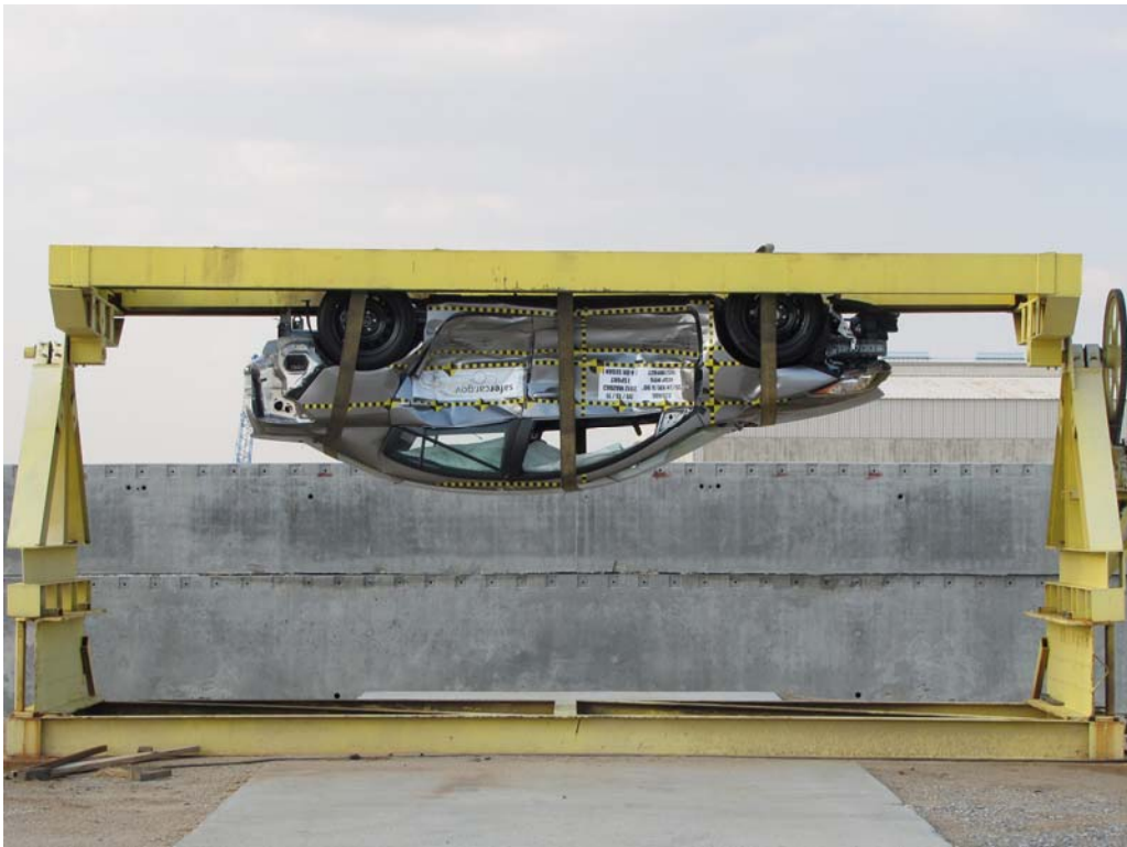
FIGURE 96. FMVSS No. 301 Static Rollover 180 Degrees
