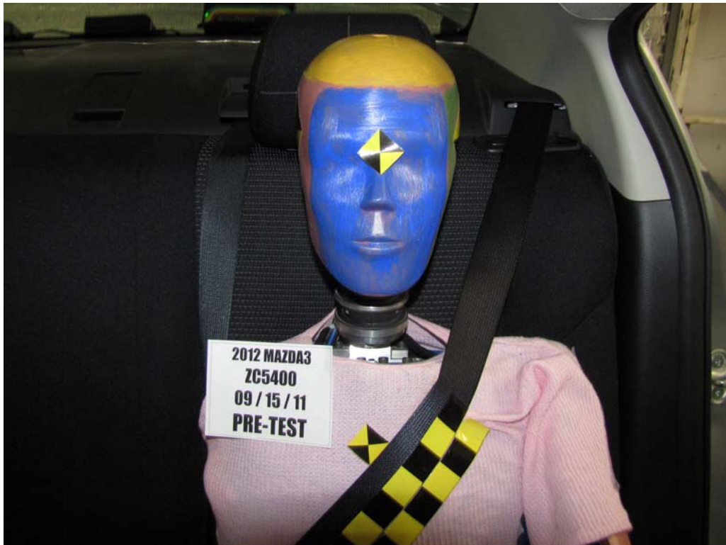
FIGURE 58. Pre-Test Frontal View of Rear Passenger Dummy Head and Shoulders in Relation to Head Restraint
