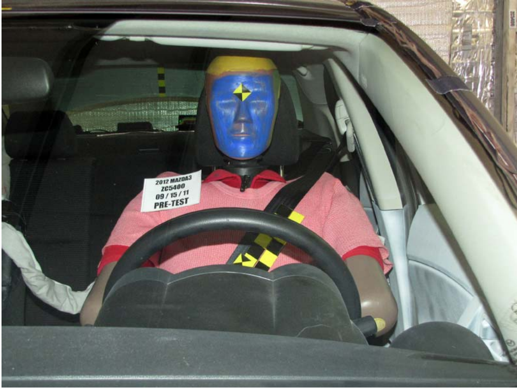
FIGURE 25. Pre-Test Front Close-Up View of Driver Dummy
