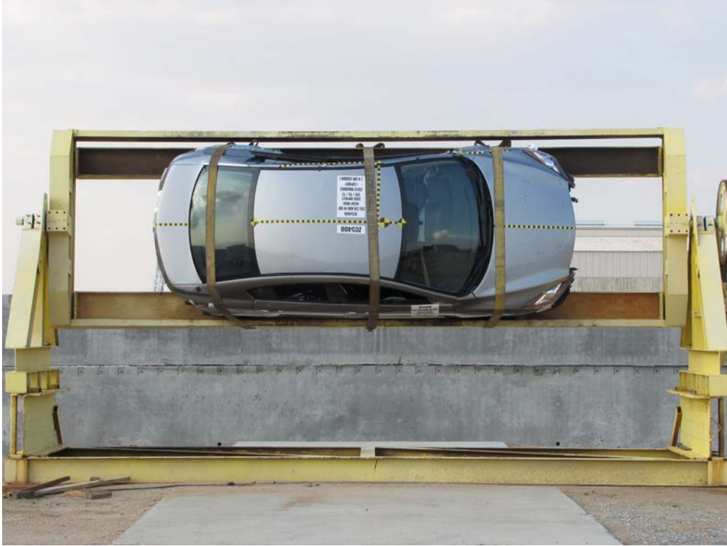
FIGURE 95. FMVSS No. 301 Static Rollover 90 Degrees
