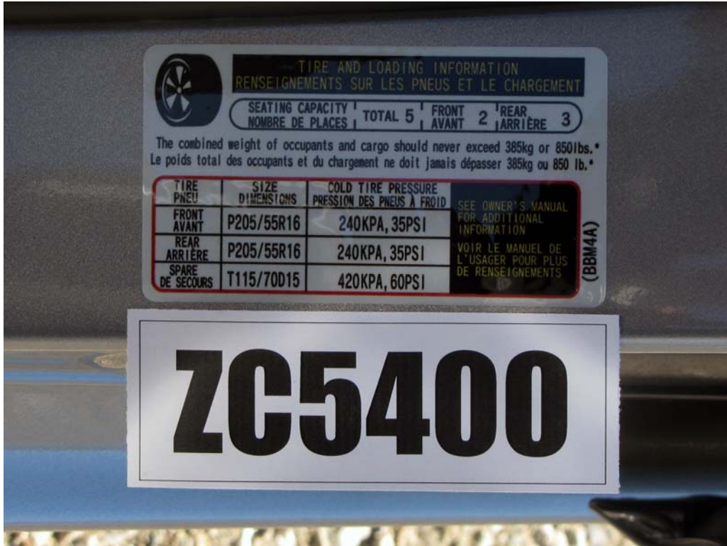
FIGURE 91. Close-Up View of Vehicle's Tire Information Placard
