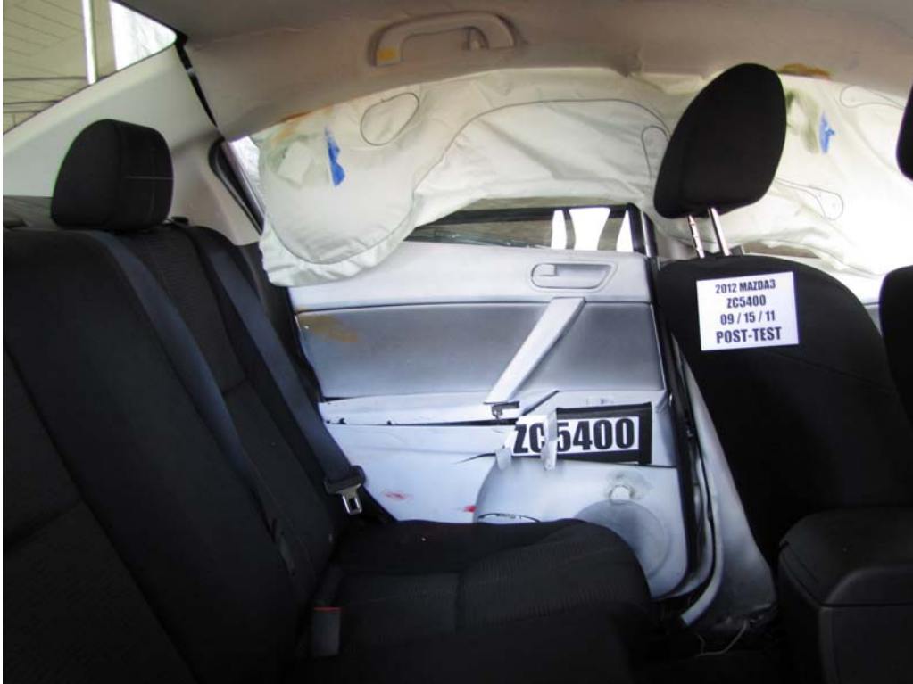
FIGURE 73. Post-Test Rear Passenger Inner Door Panel View
