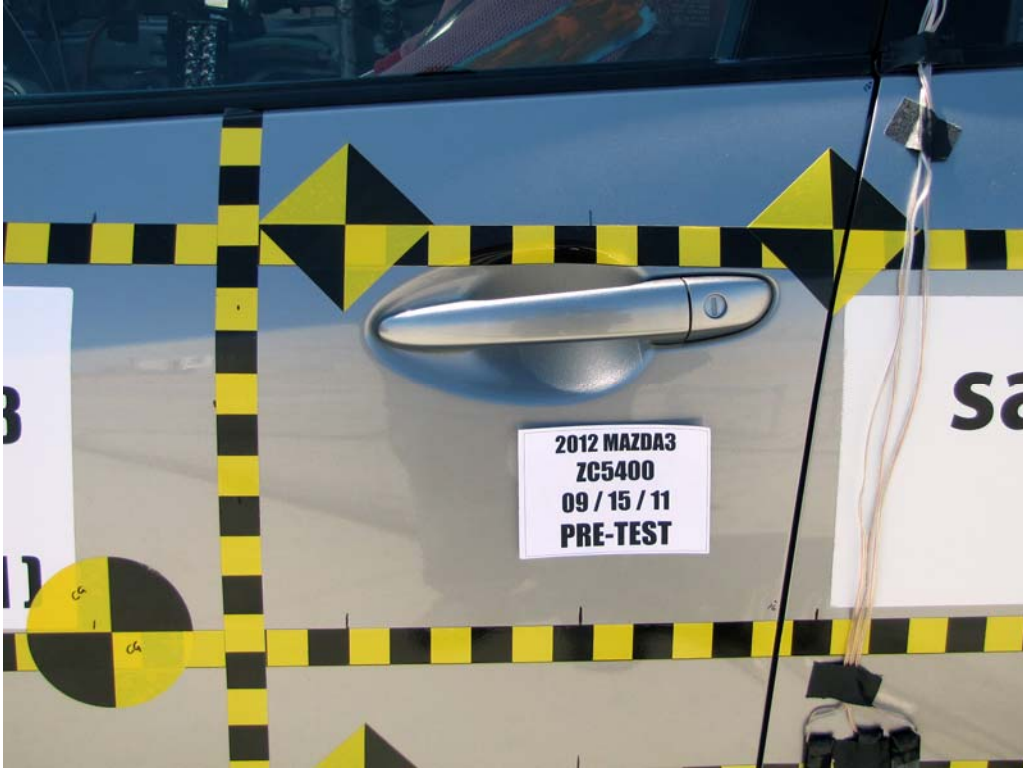
FIGURE 21. Pre-Test Left Front Door Latch Close-Up
