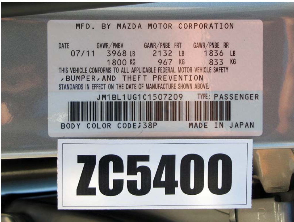
FIGURE 90. Close-Up View of Vehicle's Certification Label
