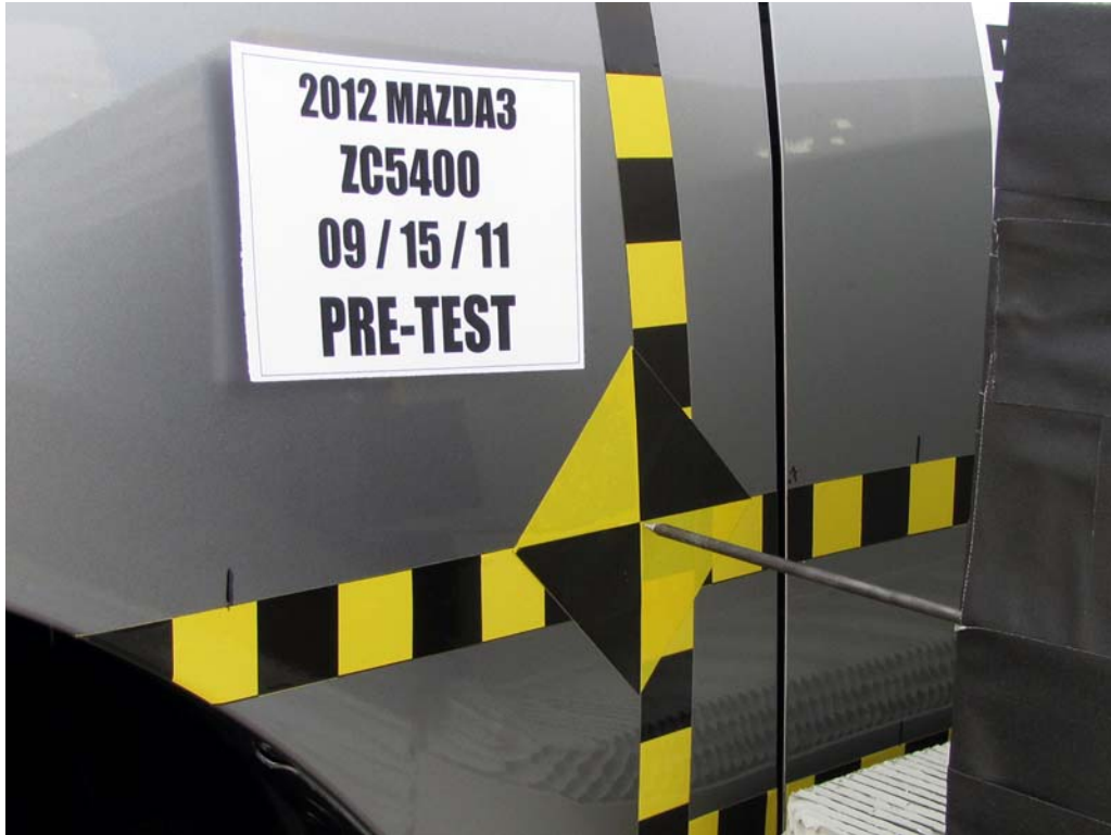
FIGURE 19. Pre-Test Close-Up View of Impact Point Target
