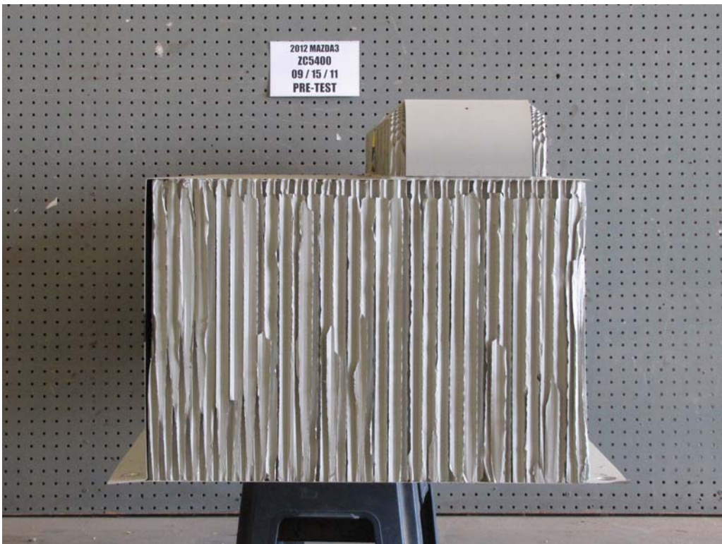
FIGURE 88. Pre-Test Right Side View of MDB Impactor Face
