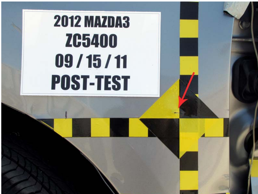
FIGURE 20. Post-Test Close-Up View of Impact Point Target Showing Impact Point Location
