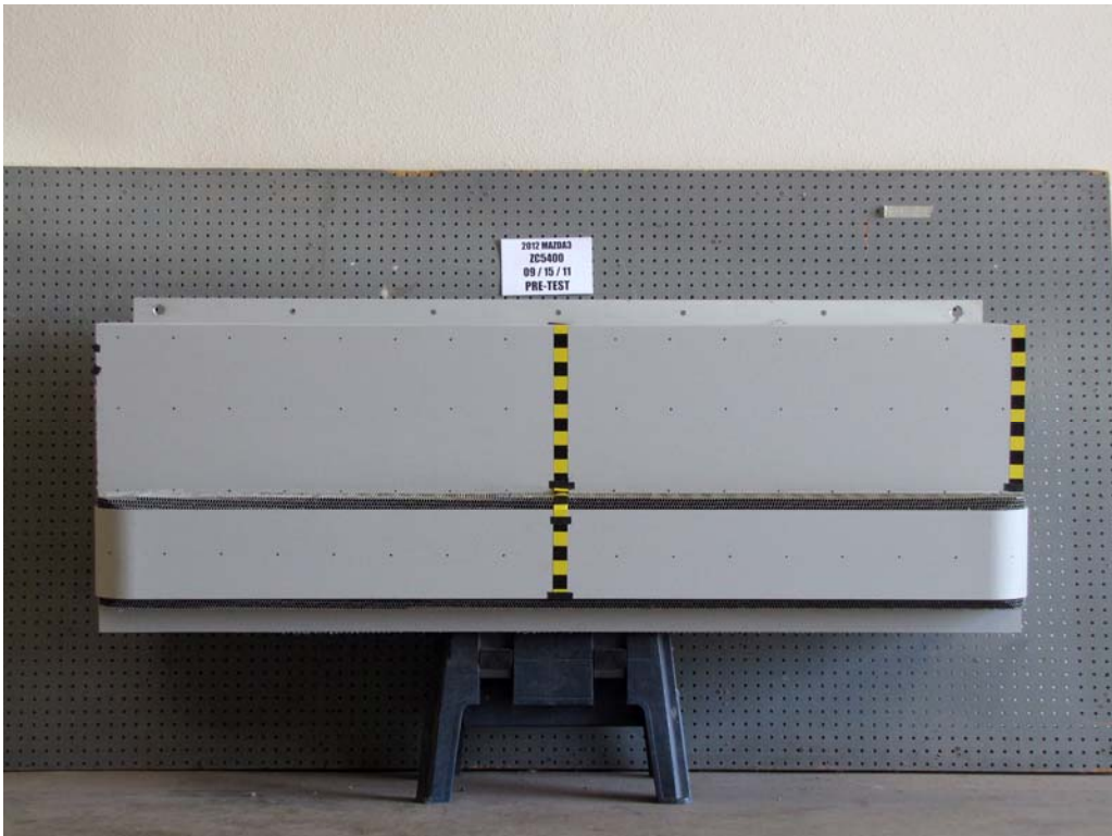
FIGURE 82. Pre-Test Front View of MDB Impactor Face
