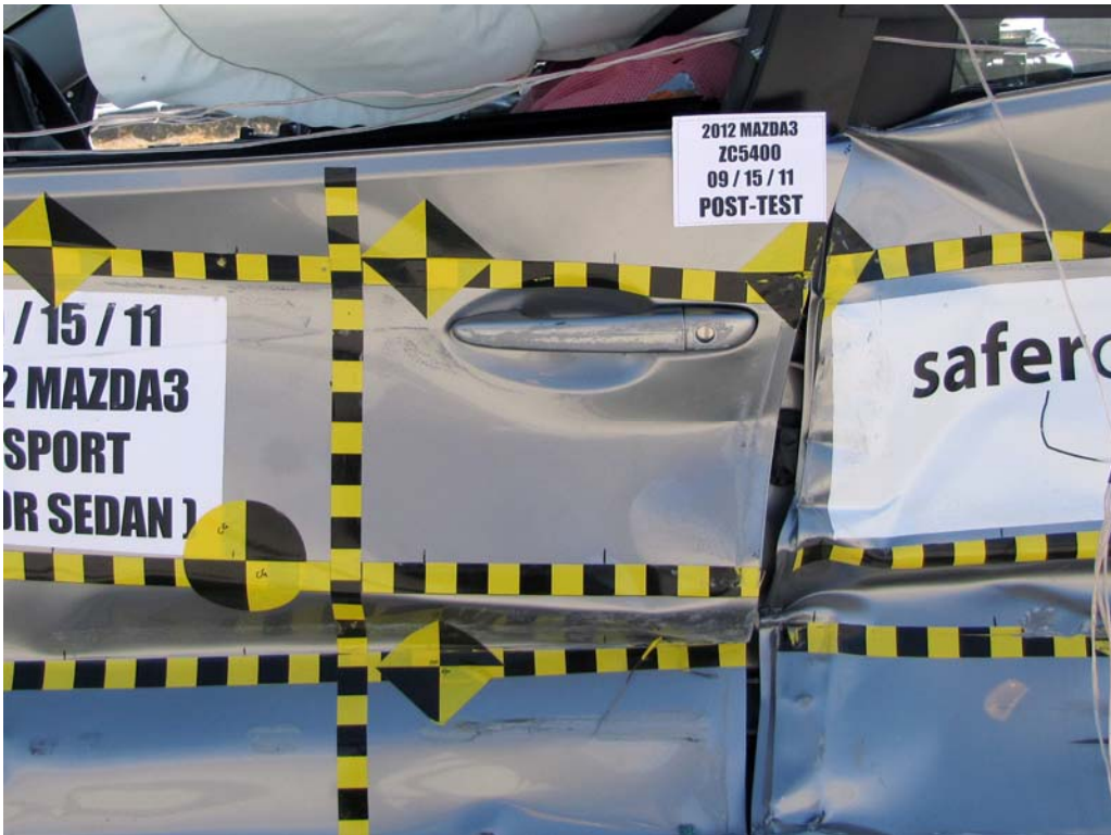
FIGURE 22. Post-Test Left Front Door Latch Close-Up
