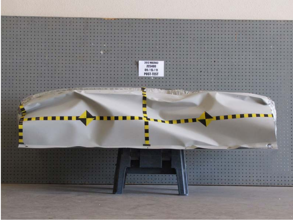
FIGURE 85. Post-Test Top View of MDB Impactor Face
