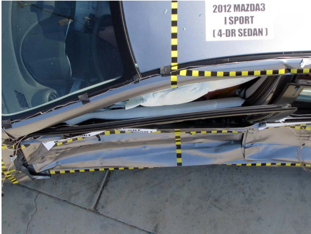
FIGURE 43. Post-Test Driver Dummy and Door Clearance View
