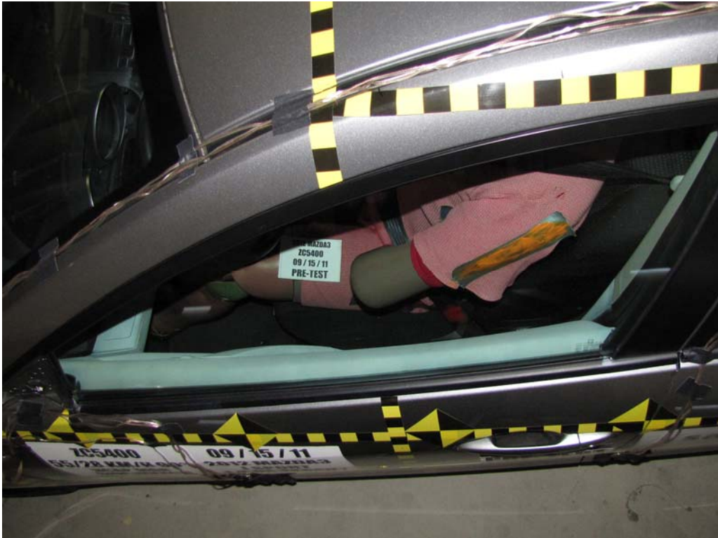
FIGURE 42. Pre-Test Driver Dummy and Door Clearance View
