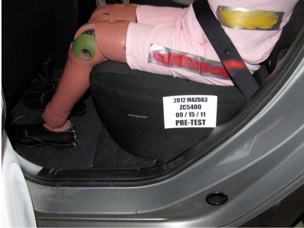
FIGURE 63. Pre-Test Placement of Rear Passenger Dummy's Feet
