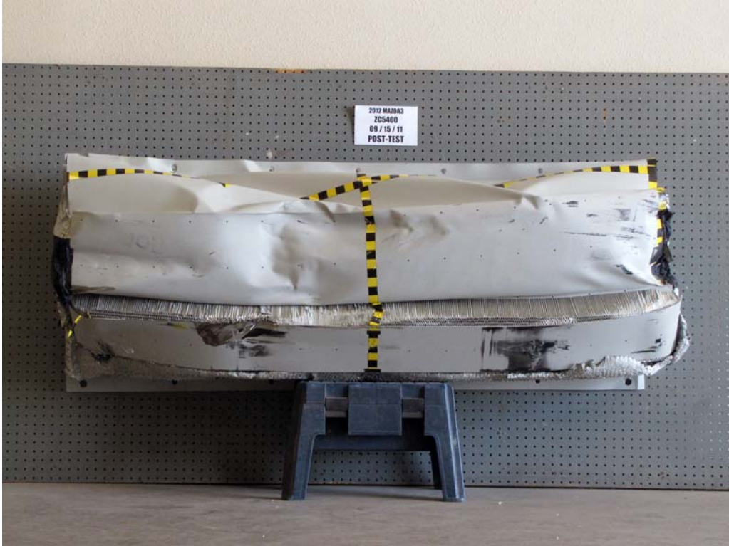
FIGURE 83. Post-Test Front View of MDB Impactor Face
