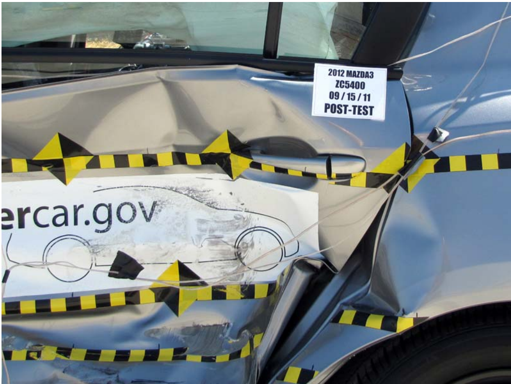
FIGURE 24. Post-Test Left Rear Door Latch Close-Up
